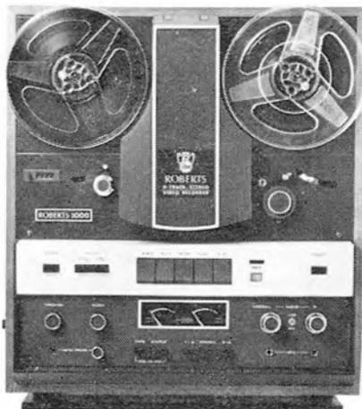
The helical scan system is used when operating video and the deck employs four motors, one three-speed motor for capstan drive, two outer rotor motor for reel drive and one video head motor. A full range of facilities is provided including remote control and a special "sensing" tape reversal system.
