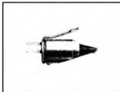
**S.P.6.** Response 20 - 20,000 Hz  $\pm$  2.5 dB. Compliance 15 x 10<sup>-6</sup> cm/dyne. Pressure 1.5 - 2.0 g. Stylus: 15  $\mu$  diamond. Output: 7 mV. 47K ohms. Price \*£7.19.6d.
