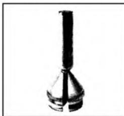
**Beomic 1000** Omni-directional moving coil microphone. Response 50 - 17,000 Hz  $\pm$  2-5 dB. Sensitivity 0.1 mV/ $\mu$ bar. Hum sensitivity -139 dB. Output: 200 ohms at 1 KHz. via 9ft lead, 5 pin DIN plug. Supplied with frequency response chart, lavalier cord, anti microphonic base, and packed in a futuristic container. Price \*£9.9.0d.
