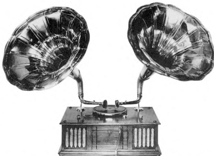
An enthusiasm for audio also implies an incurable optimism. The inventor of this device must surely have been the greatest optimist of them all! The two stylii have to be located in the same groove when the sound will have an echo effect produced by the time constant of the distance between them. We are indebted to the Tage Schouboe Museum, Copenhagen, for the use of this illustration and also for our front cover this month.
