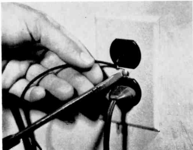
The Cornell-Dubilier AC line filter is shown at right. Into this is plugged a three-way adapter and all units, radio, TV and recorder plugged into it for best results. The terminal at the top of the case
