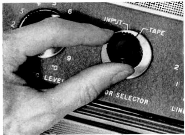
The Ampex 600 mode selector switch lets you make an instantaneous listening comparison between what is fed to the tape and what the tape plays back to you. (Ask your local Ampex distributor for this demonstration!)
