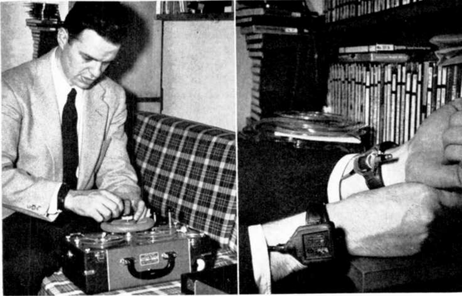
Left: the small Brush microphone is attached to the right wrist with a strap. The wire from the mike runs up the sleeve, across his back and down the left sleeve, terminating in a plug which fits the mike input on the recorder. Part of his huge tape collection can be seen in the background where racks extend from floor to ceiling. The next photo shows Tony setting up the self-powered Magnemite for outdoor work. He has made a few adaptations in the unit to suit his particular needs.
