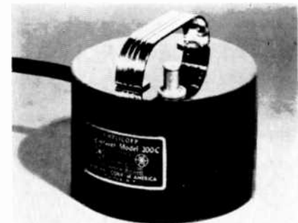
The Magneraser, a handy bulk eraser is used to wipe tapes clean for the next recording. The unit is plugged into the regular 110 volt line and brought into contact with both sides of the reel. It may also be used to demagnetize heads.
