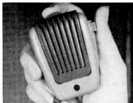
The microphone-speaker controls the machine. The bar on right starts and stops it, the button above rewinds and plays back.
