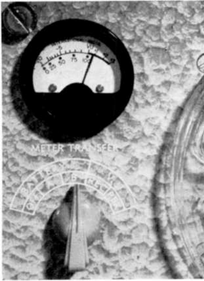
The VU meter and its function switch. The four position switch will allow the meter to indicate the condition of the A and B batteries as well as the modulation on both recording and playback.
