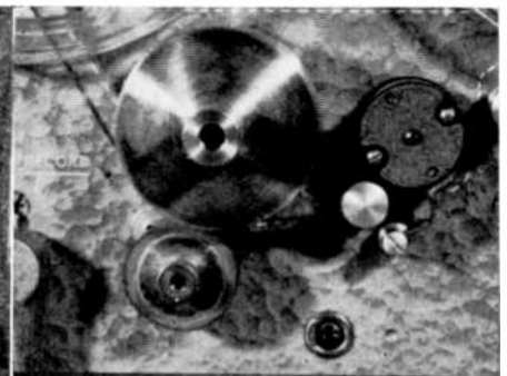
Tape threading is easy and straightforward, and should be done before the flywheel is put on. The reversible head can be seen at the right.
