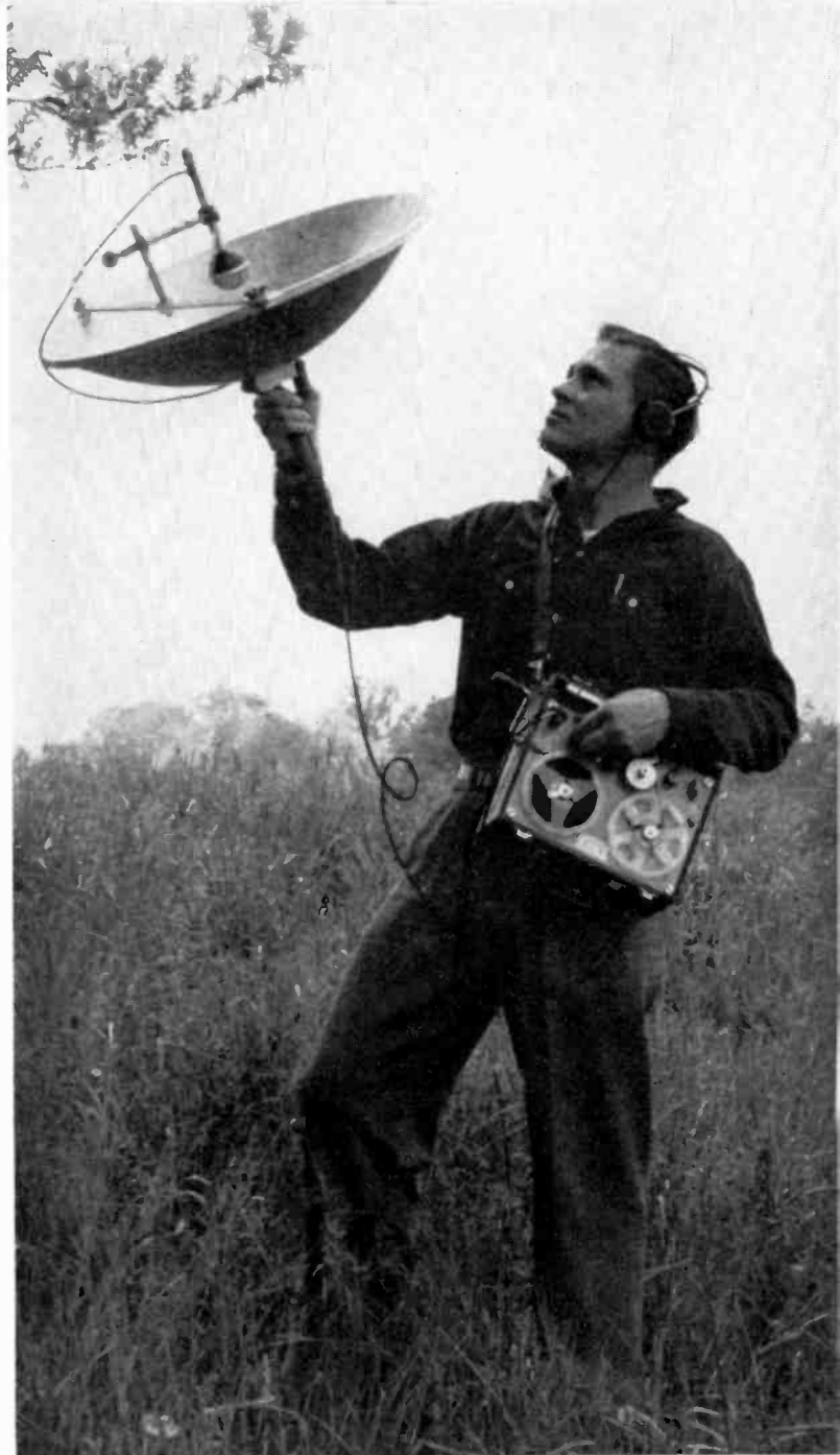
The author demonstrating the use of an aluminum parabolic reflector with the Magnemite Portable 610-E to record cicadas and other treetop singing insects.
