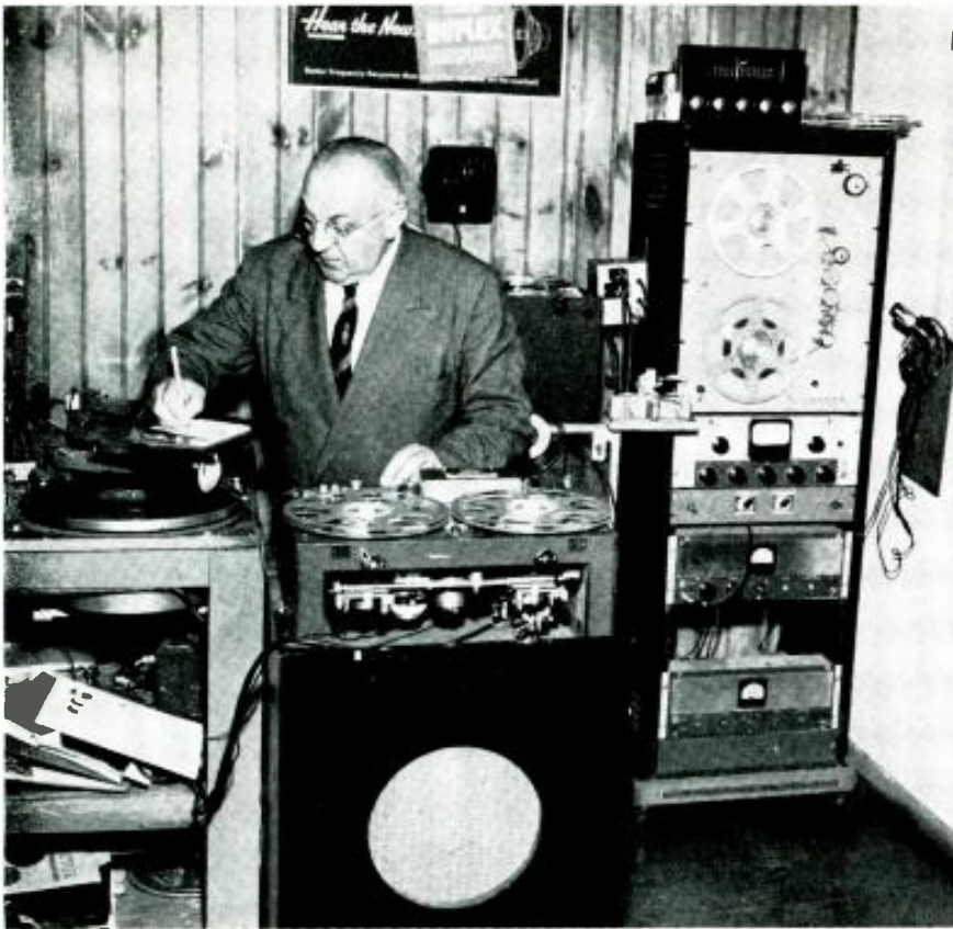
Sam Saltzman of the Masque Sound & Recording Corp. keeps notes on the time of tape sequence in the company lab where tapes are made. He is surrounded by a Presto recorder, two playback machines, and two turntables for records that are to be incorporated in the tape being made.
