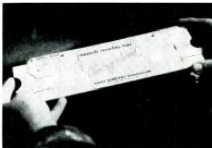
The Reeves Soundcraft Timing Chart gives the lengths of tape needed for any time and covers all thicknesses of tape. It works like a slide rule.
