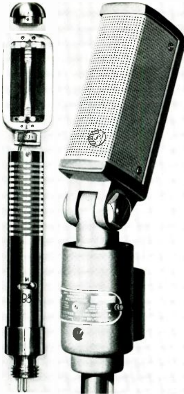
Left: Fentone Blue Ribbon mike, a 50 ohm velocity unit, made by Band and Olufsen in Denmark. Notice the tiny transformer below the magnet, which raises the ribbon impedance to 50 ohms. Right: Shure 333 velocity microphone, a ribbon mike with uni-directional pick-up pattern. This unit features three impedances, controlled by built-in switch.
