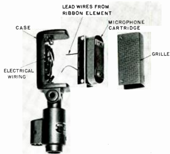
Exploded view of Shure "Concert-Line" 333 broadcast unidirectional microphone. The transformer for changing ribbon to line impedance is located in the base of the microphone, the switch is at the back, and is labeled "electrical wiring."
