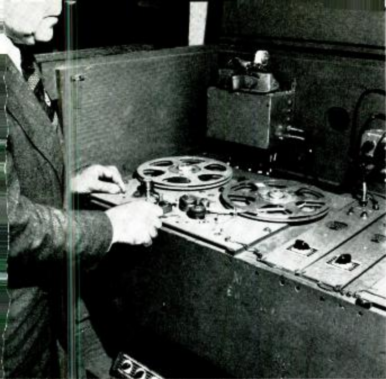
A closeup of the tape machines used at a performance, showing lead tape for next cue. The machine holds cue sheets and has a dim light that can illuminate the shelf even when the play's action demands a blackout behind the scenes.
