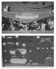
Upper: showing cover removed. Automatic cutoff is at left then two heads and capstan and roller at right. Lower: back panel with power input, octal socket output, erase link and fuses.
