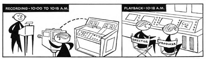
Here's how the new "Videotape" recorder works: As TV camera captures the action, it is recorded on magnetic tape along with the sound. The tape can then be played back *immediately*. This enables the producer and director to check the performance immediately without tying up costly talent and studio time.
