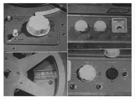
Top left: control panel showing function selector knob and stop and start buttons. Lower left: lock-on reel and timing scale. Top right: bass and treble control knobs and VU meter. Jack at left is mike input. Lower right: gain control and octal socket. Jack at left is radio input, at right 15 ohm output. On-off switch is at far right.
