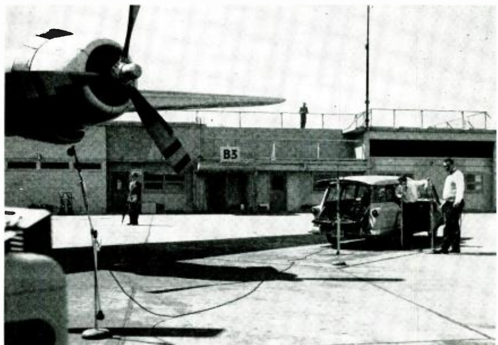
Waiting for a United Airlines DC-6 to warm up prior to takeoff, James Cunningham and Robert Oakes Jordan stand by with their recording equipment. The recording was made in three dimensional stereo, with the plane starting up one engine at a time across the mikes.
