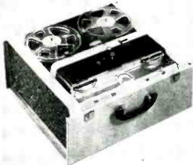
PENTRON STREOMAGIC EMPEROR. Records and plays back monaural tapes at 3 3/4 and 7 1/2 ips. Frequency response 40 to 12,000 cps. Plays staggered head tapes using radio, TV or amplifier for second channel. Price $269.95. Also model HFW 500-S at $319.95 and Stereomagic Pacer-maker, Model T-90S, staggered head at $219.95.
