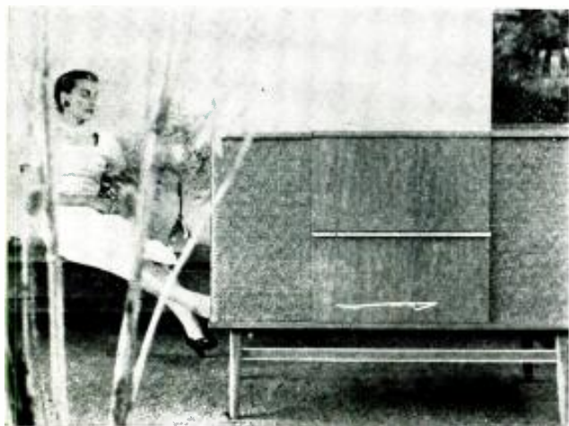
The only stereo outfit all in one cabinet is made by Ampex. Speakers throw the sound to inclined baffle boards which spread it through the room. This console also contains an AM-FM radio and a record changer. All are interconnected so that any function can be selected at the touch of a button.
