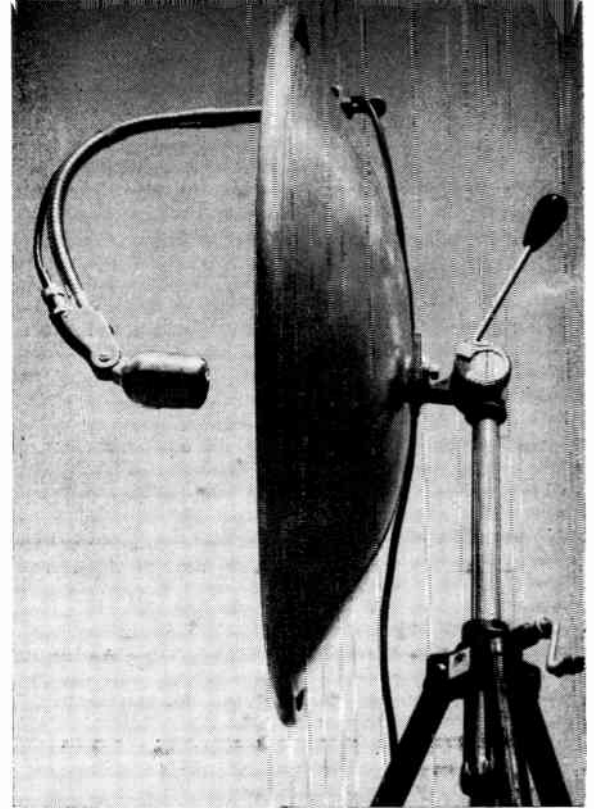
The Atlas clamp and flexible microphone stand are used to hold the mike as shown. The assembly should be well tightened and suspended from the top of the reflector.
