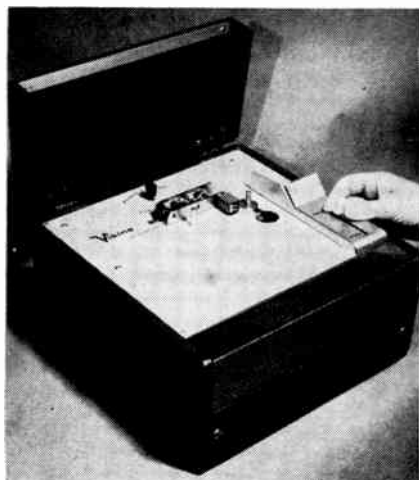
Left: single lever is only control mechanism and has two positions, release and play. Pressure roller is brought up from beneath deck and clamps tape, pulling it through cartridge. Below: unit with single head for stereo playback. Right: head lineup for erase, record and stereo playback in conjunction with Viking PB 60 record/playback amplifier.
