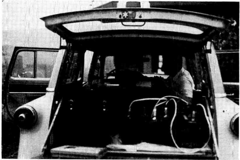
Mobile set-up showing battery hook-up for rotary converter. This type converter with some form of frequency control is recommended for out-door stereo recording.
