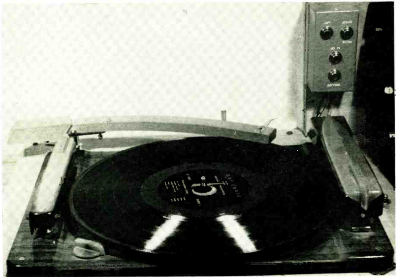
The illustration shows a setup for handling either hi-fi, lo-fi or stereo. The base is an old Wilcox-Gay unit with a Livingston tone arm added containing a stereo cartridge. For lo-fi copying, the small arm is used with a steel needle, for hi-fi, the large arm is employed and the output taken from the right hand jack which connects both channels together. For stereo, separate cords are run to right and left jacks.
