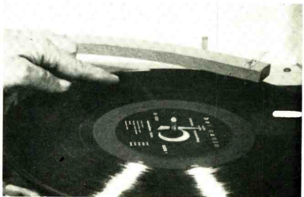
Cuing a record. The needle is placed in the groove and the record run until the first note starts. The finger is then placed on the record and the disc backed off a half turn. If the turntable motor is strong enough it will spin the turntable while the record is held still with the finger. On cue, lift the finger and the record will play.
