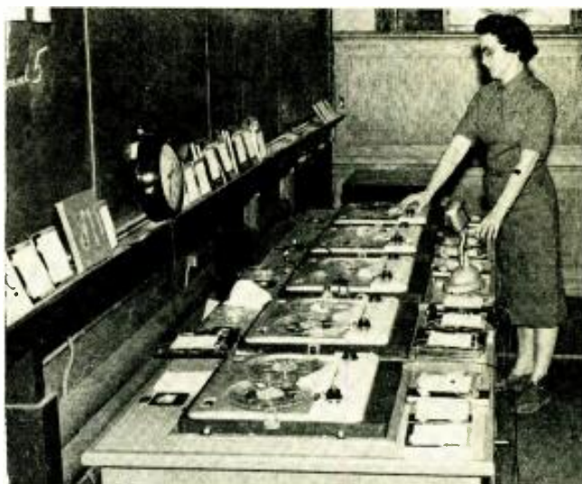
The master console at the Language Laboratory has five Webcor Royals which can handle five different languages simultaneously. Laboratory technician, Mrs. Gertrude LeBlanc, is shown in background.
