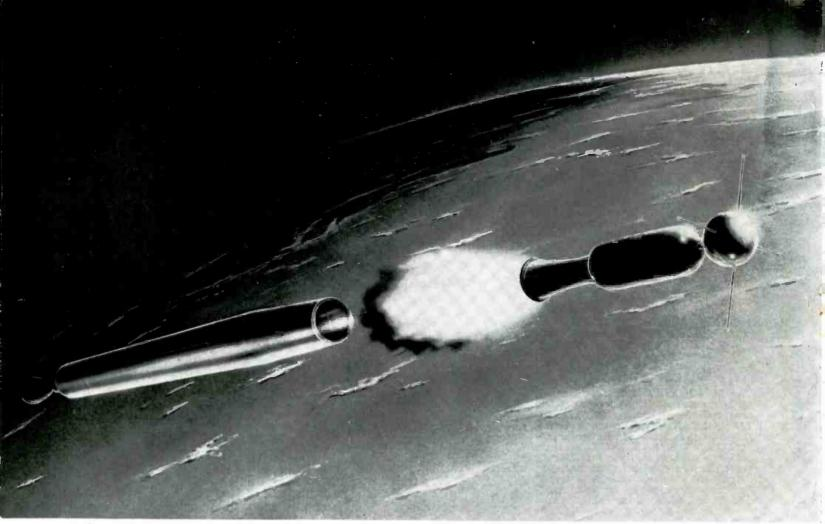
Once orbital velocity is reached the satellite is separated from the third stage rocket by a spring mechanism. For a time the empty third stage trails along as a second satellite. Satellite signals from U. S. Vanguard will be broadcast on 108 megacycles.
