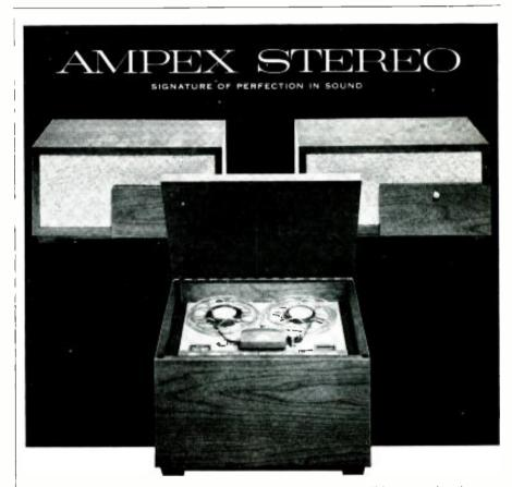
Recorder-Stereophonic Reproducer — Two-speed, precision-built tope transport, copoble of playing over 4 hours from a single 7" reel of tope; sustained frequency response 30-16,000 cps (7½ ips), with dynomic range over 55 db; Flutter and wow under 0.25% rms at 7½ ips; Precision timing occuracy affords perfection of pitch held to talerances of less than ½ of a holf tone of highest frequencies.
