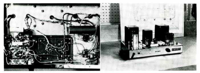
Left, the underside of the amplifier showing the printed circuit board and its connections to other components on the chassis. At right can be seen the completed amplifier and behind it one of the large detailed drawings on which the wiring is checked off as it is accomplished.
