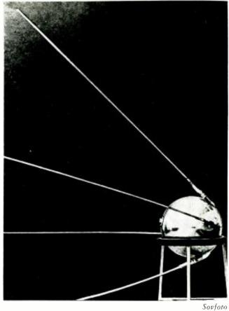
This is the first official photograph of the Russian satellite "sputnik." The weight has been given as 184.3 lbs. and it has a velocity of 18,000 miles an hour. Messages were sent out on 20.005 and 40.002 megacycles.
