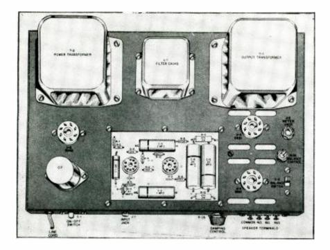
The diagrams furnished with all of the kits are very complete and detailed. This layout shows the diagram of parts placement for the Knight Linear Amplifier, made by the Allied Radio Corporation. In addition to general diagrams such as this there are specific closeup diagrams at any points where wiring is complicated. The use of printed circuits in kits such as this has eliminated possible mistakes in wiring and speeded up the construction.
