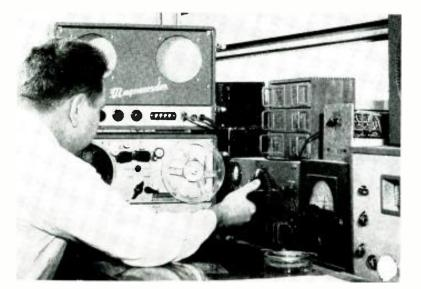
Melvin Hastings tunes the HRO receiver on 20.005 megacycles to catch the beep, beep signals from the Russian satellite sputnik. The output from the radio receiver was fed into the Magnecorder shown and results of the recording were excellent. At one point the signal was picked up while the satellite was 3,000 miles from the station. When almost overhead the signal from the one watt transmitter on the satellite was so loud volume had to be turned down for recording.
