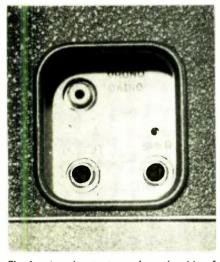
The input and output panel on the side of the recorder contains a phonojack for radio and phono recording and the standard phone jack for the output and the external speaker connections.
