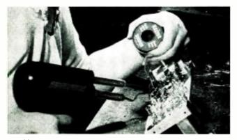
A soldering gun and rosin core wire solder is the most effective combination in assembling one of the regular kits. Making the soldered connection is easier than pasting pieces of paper together. Wives or sweethearts enjoy soldering components in a chassis.
