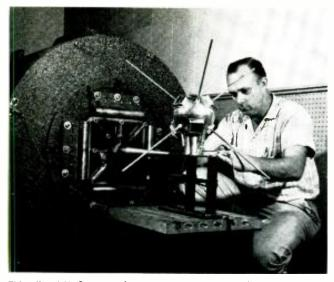
This official U. S. Navy photo shows an experimental six inch Satellite being tested by vibrations up to 25 G's at the Naval Research Laboratory, Washington, D. C. Units similar to this will be fired this year.
