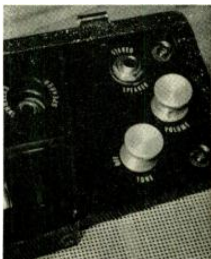
Stereo controls are grouped at right side of case. Photo shows tone and volume controls and jack connection for stereo speaker.
