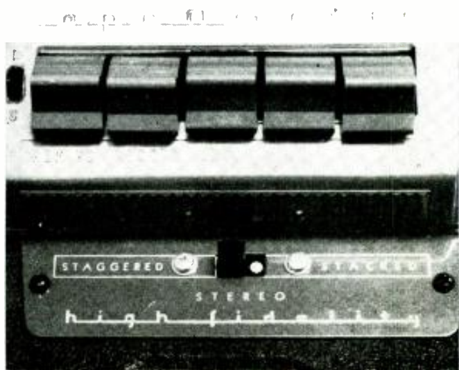
Top: speaker yellow lead is grounded to speaker frame by soldering short jumper wire to speaker rivet. Upper center: head socket and switches which must be rewired are exposed by removing metal bottom plate. Drawing shows position of heads with new stacked head in place. Lower: the switch installed on the top of the recorder in front of the operation buttons.
