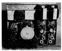
Rear view of tape deck showing three motors Preamps are mounted at right side in picture. Deck has no belts, pulleys or clutches.
