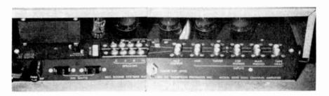
Above: rear view of amplifier showing inputs and outputs. The unit contains 11 tubes. Below: possible hookups for tape deck and amplifier plus associated equipment.
