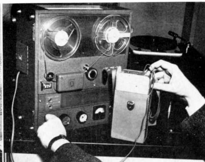
Left: Recorded reels of the Cub-Corder can be removed and used directly for broadcast. Right: Recordings made on the Mohawk must be transferred from the magazine tape to reels for broadcast.
