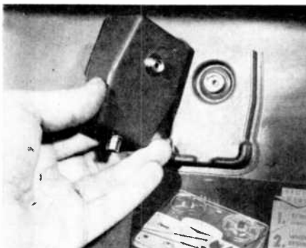
Left: the microphone does not have a cord attached and is snapped into its holder in the lid by means of a button on the back of the mike case as shown. Mike cord also serves as an output cord for the recorder. Right: rubber reel locks insure quiet operation and permit the recorder to be used in any position.
