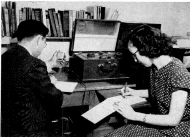
Below: one of the first dual track machines was the Eicor, shown below. Revere, Webcor, Pentron, Ekotape and a few others made their debut about the same time and came on the market as dual track machines. At right is shown the Brush Soundmirror which had a single track down the middle of the tape.
