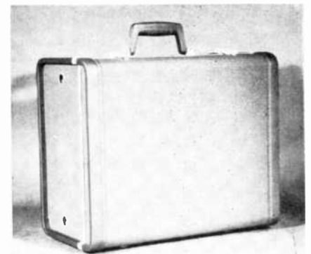
The recorder with the case closed. The openings in the end of the case take the microphone plugs when stereo recording is done.
