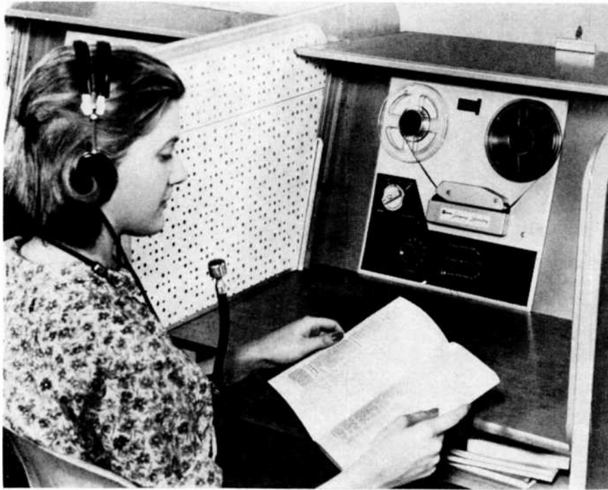
An individual language lab booth installation made by the Edwards Company. Booth has headphones, microphone, and tape deck. The student can record the lessons from the master console then compare his performance with the master tape. In this way, using the modern language laboratory, students learn to speak, understand and use the foreign language.
