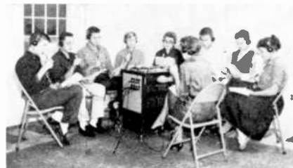
A complete self-contained language laboratory for one to eight students and teacher with headsets, microphones and monitor station on wheels.
