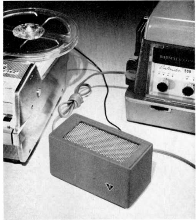
Above: the Cavalcade Programmer by Eastman Kodak acts as a mixer as well as a synchronizer. It uses a 6000 cycle tone placed on the same track as the narration. Right: the Bausch and Lomb Balsync puts the signal on the second track of a stereo pair to operate the projector.
