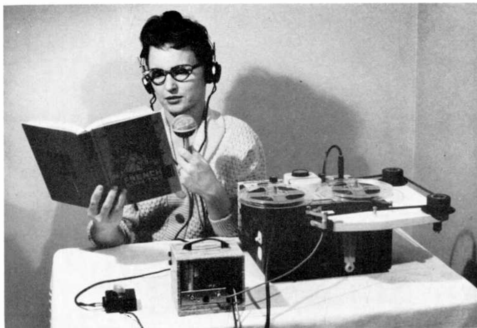
Fig. 10: An excellent use for the Echo Master is as a supplementary aid in studying a foreign language. And to still further enhance its value, it is necessary to extend the delay period of the "echo" so that more can be said . . . hence the use of a system that furthers the distance between the record and the playback heads.
