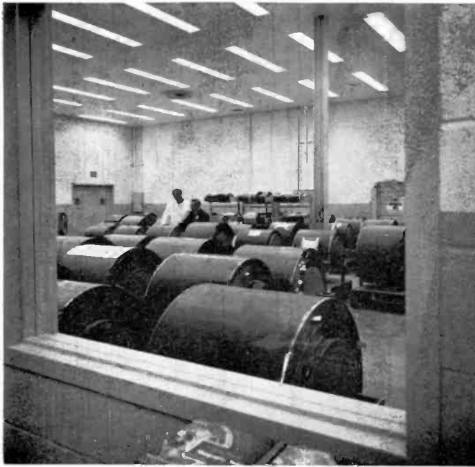
After the tape has been made it is stored in hospital-clean storage rooms to await slitting to commercial widths. Hundreds of thousands of listening hours are represented by these jumbo rolls at the Minnesota Mining plant. Right: the slitting process which cuts the jumbos to the size desired and spools the tape on the hubs or reels for delivery to the customer. Slitting is another in the many critical processes in tape making for the width must be maintained within a few thousandths of an inch, the tape edge must be smooth and even with no nicks and it must not cause the edge to waver or fray. This slitter is at the Audio Devices plant.
