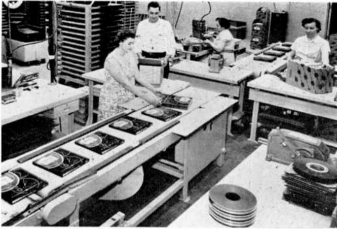
The end of the line in tape manufacture is the degaussing and packaging. Bulk erasers under the belt provide tape completely signal free. Care is also taken to provide packages which will insure that the tape reaches the customer in the same perfect condition in which it left the plant. Upper left is the Minnesota Mining packaging department, upper right, Reeves Soundcraft and lower, Audio Devices.
