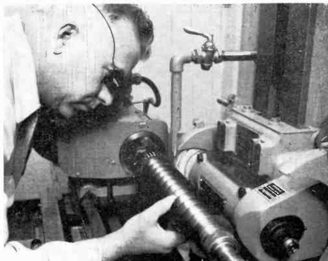
Grinding the slitter blades at the Ampex plant. A jeweler's loupe is used to examine the circular blade edges to make sure they are perfect. A dull or imperfect blade will leave its mark on every foot of tape it cuts.
