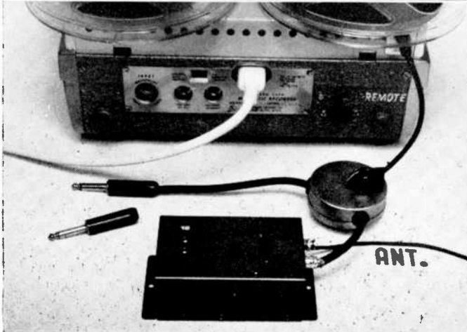
Upper left: the simplest system is just to set the Stereo Bug behind the recorder and plug it in. Then stretch out the radiation wire, turn the unit on and you're "on the air." The short cable shown here is the A-to-C cable more clearly illustrated in the following photo. Upper right: the simple shielded cables A-B and A-C may be all you will need. But if it is necessary to reduce an excessive preamp output, or if you want to combine the two separate channels for a single balanced monaural output, then the easy-to-make special K-ABC "octopus" control is worth having . . . inside a typewriter ribbon can. Lower left: this is the hookup for stereo (broadcasting to a nearby AM radio for the second channel), similar to the hookup in above except with a potentiometer added. The signal coming from the 2nd channel preamp is without a recorder volume control, so adding a "pot" gives you the proper stereo balance control so often needed. Lower right: this is the hookup for converting stereo to monaural, necessary when you want to broadcast a taped stereo "program" around the house for other members of the family to pick up monaurally on their AM radios. The potentiometer control knob is adjusted so that both channels combine and come "through" equally.
