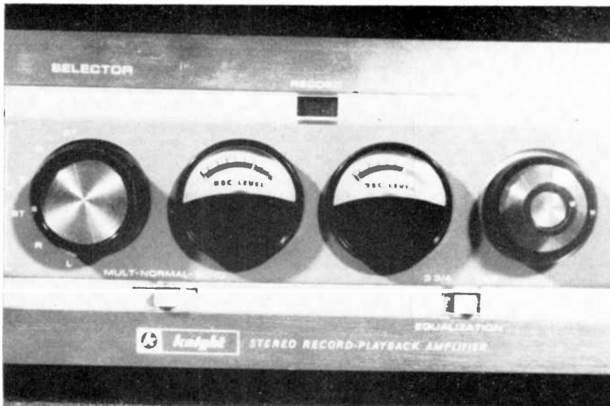
Center portion of control panel showing twin VU meters which function on both record and playback. Knob at left of meters is selector switch, one on right controls right and left volume to auxiliary jack. Left switch below meters controls mode of recording (multi-normal-echo) and switch to right is for equalization.
