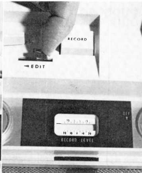
Center section of deck has edit key for stopping tape, record interlock button and record level indicator.
