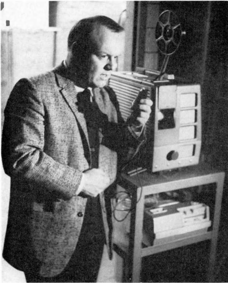
Left: While silent 16 mm film is being projected on screen, a tape recording can be made explaining or instructing in conjunction with the film. For all practical purposes this makes a good substitute for sound on film—and is less expensive.
