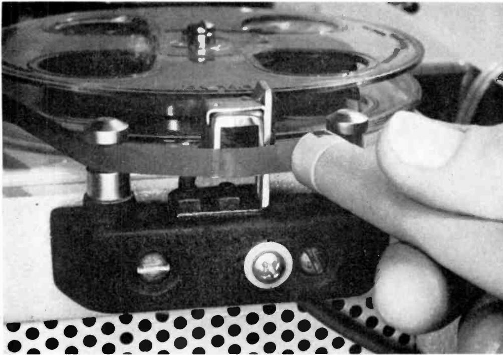
Fig. 9: Now the magnet (fastened to a wooden dowel for ease of handling) is being used on the other side of the auxiliary play-head. This way you can hear the recording immediately before you erase, making it a simple matter (with practice) to hold the magnet against the tape during the exact times you want to make an erasure.
