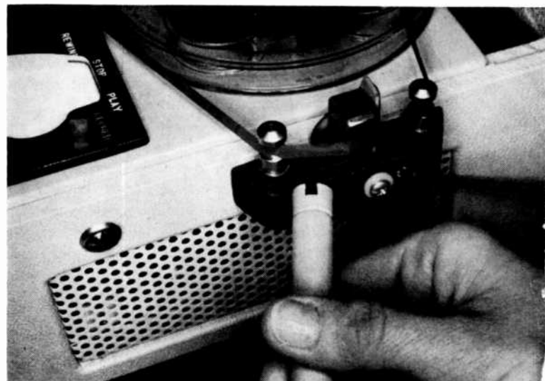
Fig. 8: With the auxiliary play-head assembly back on your recorder and a small, powerful permanent magnet to aid you, it's possible to edit your tapes without cutting them . . . by varying the distance of the magnet from the passing tape. With the magnet used as shown here, you can immediately hear the results of your editing.
