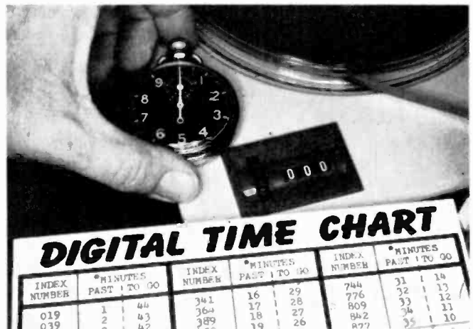
Fig. 2: For utmost use of your digital counter you should make up a few Conversion Charts relating the reading to actual playing time. First write the numbers from 1 to 30 on paper (or beyond 30 if you're using extended-play tape as I do), and then play a complete reel of tape as you make note of the digital reading every minute.
