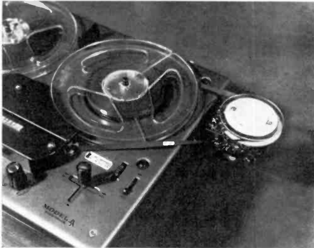
Top: Typical projector, amplifier, tape deck and synchronizer set up in operating position. Bottom: Synchronizer attached to tape deck. Note half twist in tape and approaching aluminum tab which will actuate the slide change.
