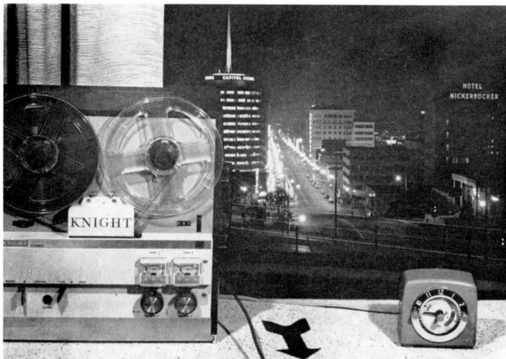
Fig. 1: All set for a "Knight" on the town, with your recorder hooked up to a timer clock and also (arrow) plugged into a radio or TV that turns automatically on and then off again, to record your favorite programs even though you're not actually at home yourself.
