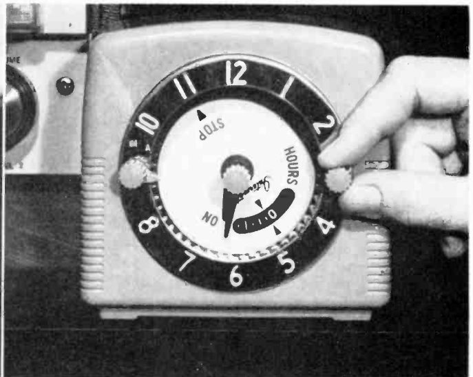
Fig. 6: Let's say you want your recorder (as well as the TV) to turn back on again so you can record a full musical hour from ten to eleven o'clock. So now turn the right-hand knob in a counter-clockwise direction until the little red "Stop" arrow points exactly to eleven as shown here (and note that this is the STOPPING time).
