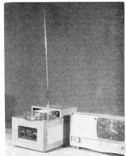
The antenna can be extended for about two feet which broadcasts the signal to any nearby AM radio.
