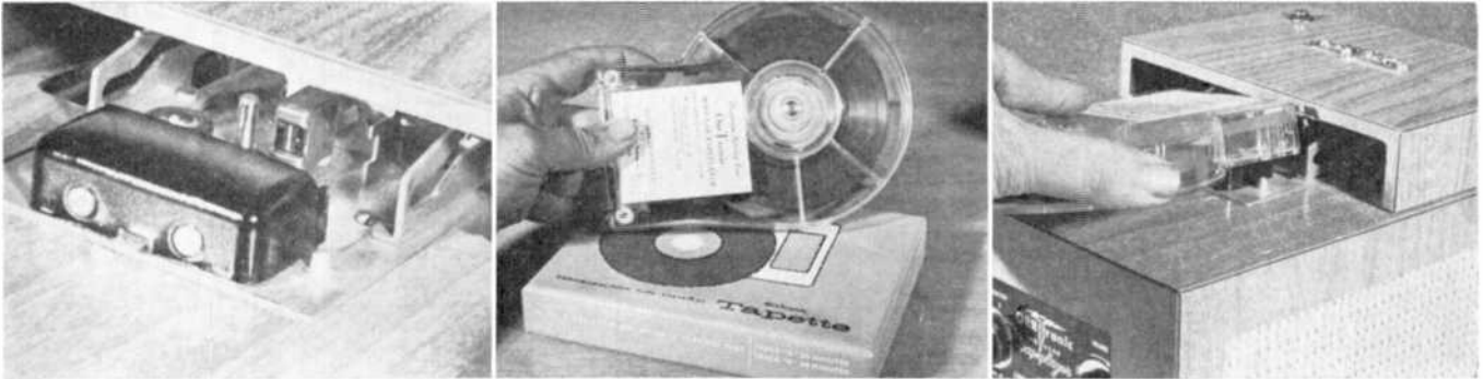
Left: showing the two track head, capstan and roller. The cartridge nests over the black housing in the foreground and is pushed in to play. Center: the Orrrtronic Tapette which holds 600' of 1 mil Mylar tape. Right: showing how the Tapette cartridge is placed over the housing and onto the pins on the deck of the player.
