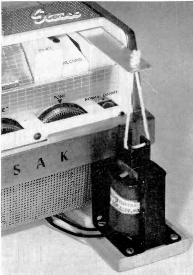
Fig. 8: Another mode control system is via push buttons, as with this Wollensak recorder. As shown here, a short "lever" of metal is placed over the STOP key, with the key itself acting as the fulcrum. The up-ended solenoid plunger attaches to the other end of the lever, to effectively push the key when solenoid power is applied.
