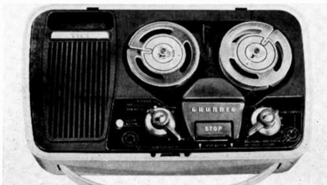
The Grundig portable has a DC motor and moves the tape by powering the take-up reel. It has no capstan and roller. This makes the speed of the tape vary, depending upon the amount on the take-up reel. It records and plays back satisfactorily, but its tapes cannot be played on standard machines.
