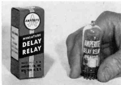
Fig. 2: The "heart" of the unit is this Amperite thermostatic delay relay which comes in tube form. The relay is hermetically sealed in a glass envelope, with SPST normally-open 3 amp. contacts that close automatically by heater action after a delay of so many seconds. The tiny 2-watt heater element works off 115-volts AC-DC.
