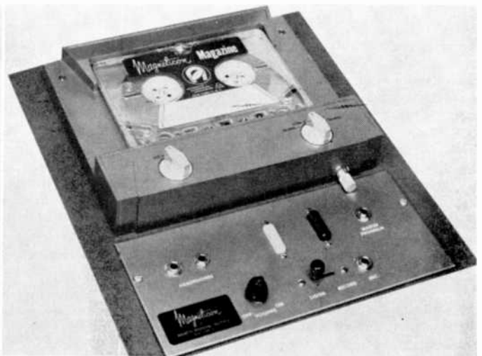
Left: the typical home tape recorder is exemplified by this V-M model having two reels and using a capstan and roller tape drive. Right: the Magneticon, a machine designed for school language labs uses the RCA type cartridge. The principle is still reel-to-reel.
