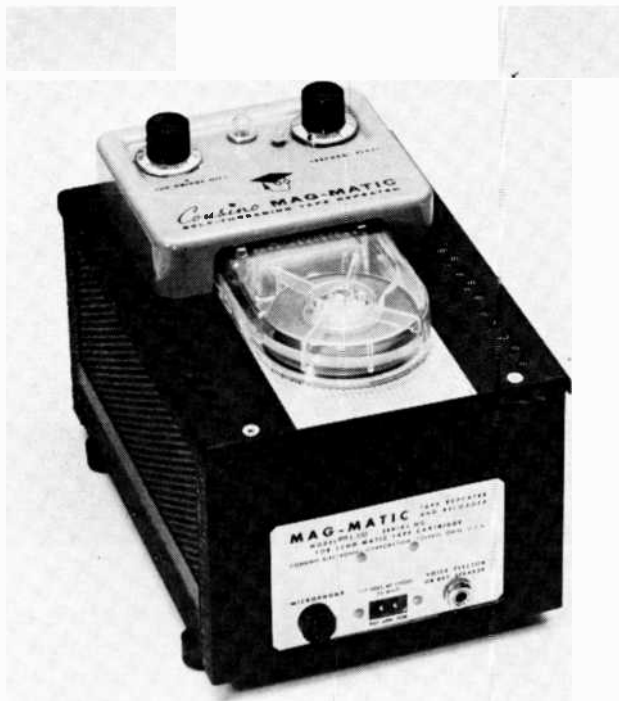
The Cousino machine uses a Cousino cartridge which is a continuous loop of tape. Up to an hour of playing time may be had. A capstan and roller furnish the drive.
