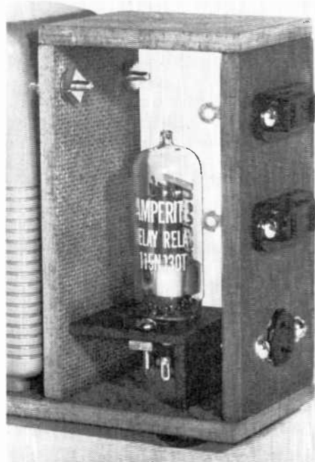
Fig. 5: Although the exact shape and size of the little housing is not too important, be sure to leave adequate room around the relay tube to allow for proper ventilation. The upper two receptacles are regular solder-lug AC chassis sockets, while the lower one is purposely different as it connects directly to the recorder motor.
