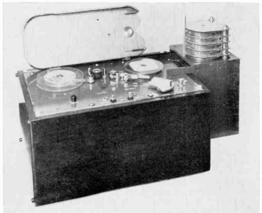
This machine was developed by the Armour Research Foundation but so far has not seen any commercial use. The tape is held on the reel by means of beaded flanges and a wide leader strip attached to the end of the tape. The strip has a hook on it which engages an eye on the machine which then threads the tape past the heads. Rewind is automatic.
