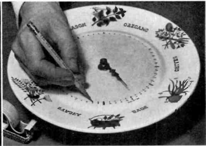
Fig. 4: Exactly center and then fasten down the 5 1/2" Minute Guide paper atop the clock's inner dial by means of double-faced Scotch tape. Go completely around the rim of the guide, marking off the sixty divisions. You'll find the clock's markings a bit less than perfectly accurate, but your later calibration will make up for this.
