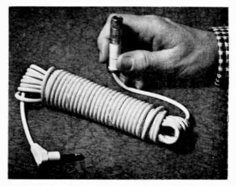
Fig. 8, left, top: These are Amphenol "Series 75" cable connectors used for making a strong, reliable joint between two singleconductor shielded cables. The female connector "A" is at the end of the cable coming from the microphone, with "B" representing this same connection, but with a phone plug adapter screwed on for direct use.
