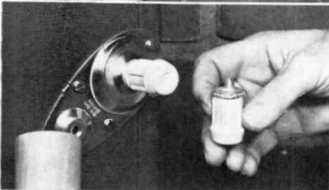
Fig. 5-a, top: If your recorder is a large one, a set of long legs can be quite elegant looking (and table saving). But there will be times when you'll want to unscrew the long legs and replace them with shorter ones for table top—or, in this case, fireside—use.
