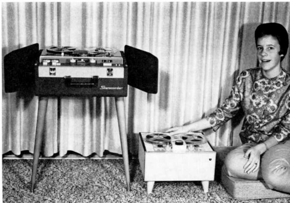
Fig. 1: Putting legs on your recorder can not only add to its convenience and attractiveness, but this may completely solve your cooling problem as well. Being higher up, the cooling fan underneath the motor has a better chance to draw in an adequate supply of air.
