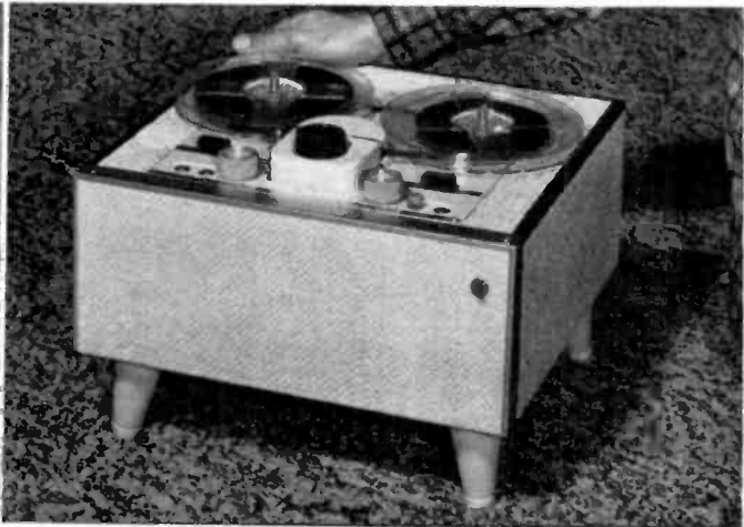
Fig. 4: Then, if raising up the recorder solves your problem, permanently substitute regular screw-on table legs. You may wish "shortie" legs as shown here—which are the perfect answer for those of you who like to set your recorder down on a deep-piled rug to operate—or longer 21" legs as sported by the Sony in Fig. 1.
