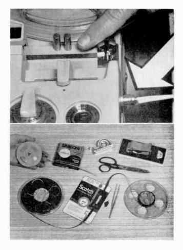
wraps itself around at about a  $90^{\circ}$  angle before going on to the pickup reel. You can guide your own tape this same way simply by fastening a single *Nortronics* TG-5 Tape Guide Post (see last month) at a point on your own tape deck that more or less duplicates the Revere setup. Either fasten the Guide from below deck with a machine screw or Epoxy it in place from above. And it needn't be insulated from the metal deck.
