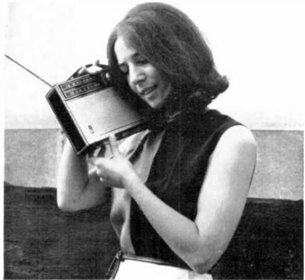
Test reception before doing any actual recording. FM signals are highly directional and reception will depend on orientation of antennas at both the receiver and the transmitter. Experiment for optimum results.
