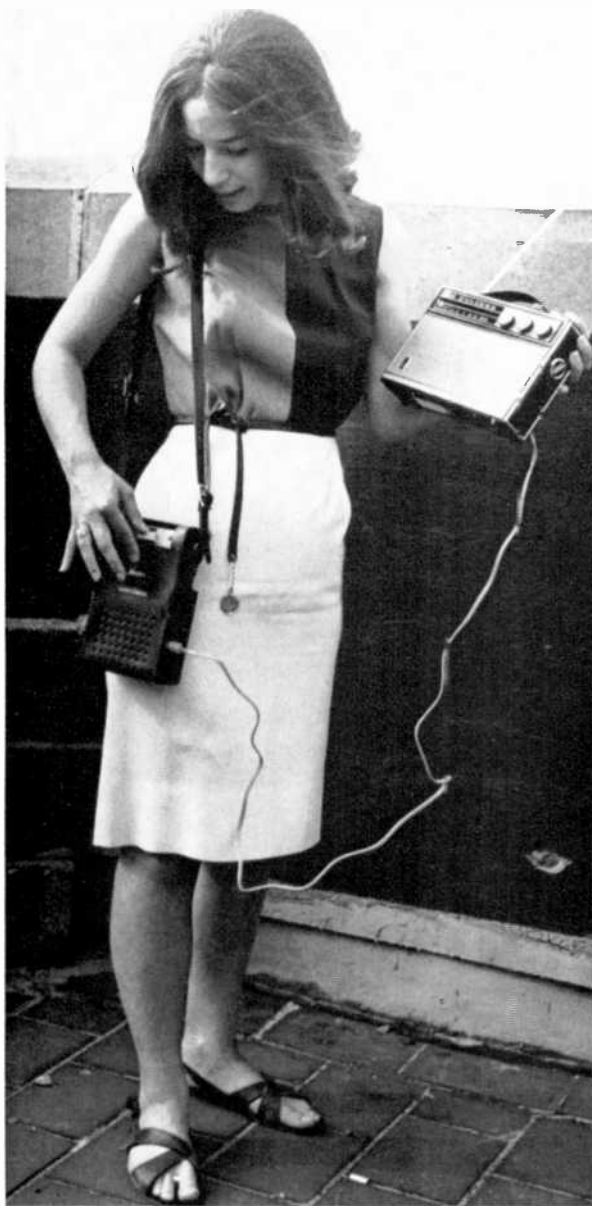
Recording station on the go comprises FM portable radio (by Sylvania) and Norelco 150 battery tape recorder. Recorder is patched into radio's earphone jack, but direct connection to radio's audio transistors can be made if preferred.
