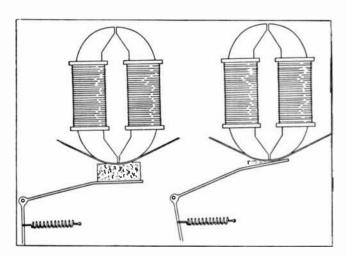
Above is typical record head. Note narrow gap. At right is same head when badly worn. Note that constant wear and abrasion has worn away the narrow gap, destroying high frequency response and increasing signal-to-noise ratio.
