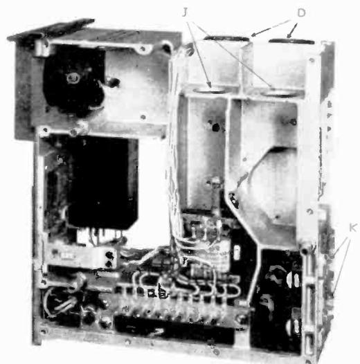
Aerial ammeter and audio components for the F.U.G.-10. Note the extra compartments and the mounting brackets, which are part of the die-casting
