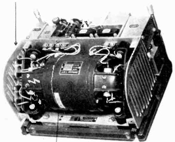
F.U.G.-16 power unit including rectifier and filter circuits. The warning arrow on dynamotor indicates high-voltage terminals
