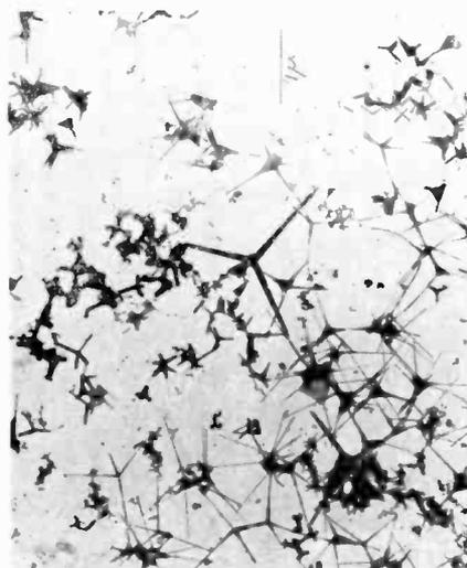
Electron micrograph of zinc oxide smoke
