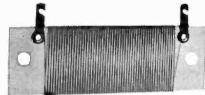
**TYPE JN**—mica card, standard tolerance 1%, maximum resistance—100,000 ohms, size 1" wide x 3 1/4" long x 1/16" thick. Mounting by insulated holes to clear 6/32 screw. Terminals: hot tinned copper lug.
