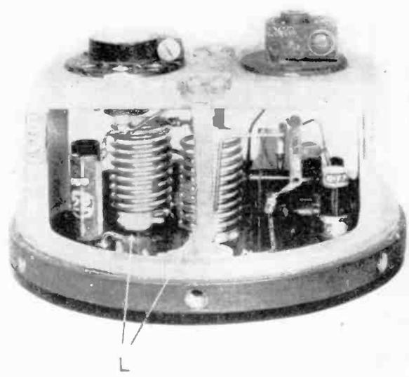
Cast alloy base on which F.U.G.-16 set and power unit are carried. The female outlets shown in the picture, connect with male contacts of other units
