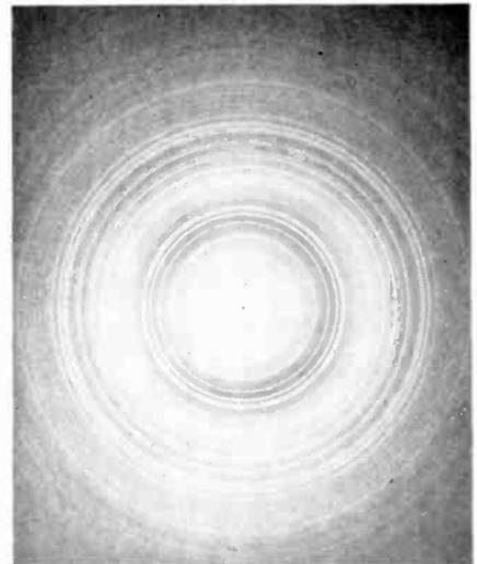
Diffraction pattern of zinc oxide smoke
