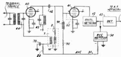
circuit and simulates a negative capacity in shunt with the input capacity, the avc being connected also across this preceding amplifier circuit and varying the negative capacity in such a manner as to compensate input capacity variations and the detuning of the tuned circuit resulting from it. Walter van B. Roberts, R.C.A., (F) January 27, 1940, (I) Sept. 15, 1942. No. 2,296,057.
