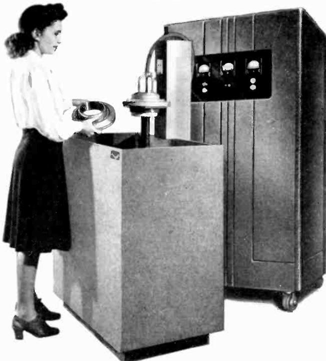
Set up for multiple brazing of bomb fuse liners with 20 kw "Thermonic" induction heating equipment
