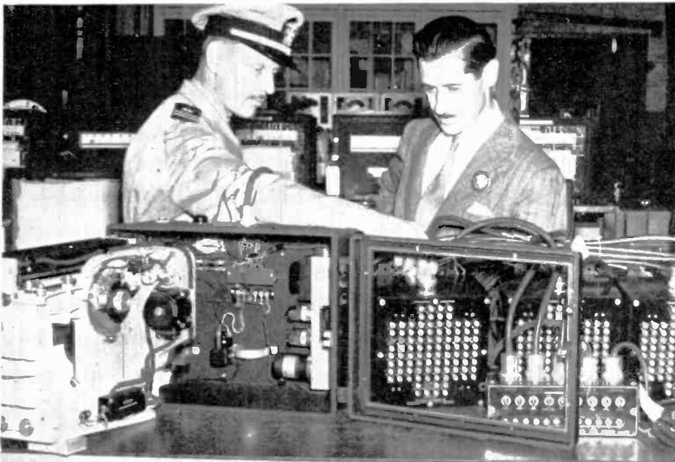
Self-balancing electronic potentiometer and recorder equipment to graph changing temperatures of up to 14 different points at once, in aircraft flight tests. Developed by Brown Instrument Company, the recorder is being widely used on Douglas B-19 and other planes. It records data faster than three or more men with pads and pencils and with ten times annual accuracy.
