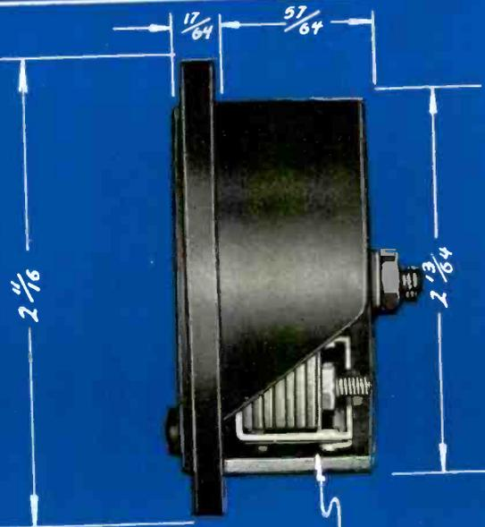
NOTE - THIN MOLDED CASE WITH FULL SIZE TRIPLETT MECHANISM.
