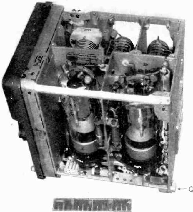
F.U.G.-16 transmitter for German fighter plane. Note the ceramic coil form with keyed-on winding in the master oscillator of this Luftwaffe transmitter. The unit uses an MO-PA unit with grid modulation, has an output of about 2½ watts and a frequency range from 2.9 to 3.5 mc
