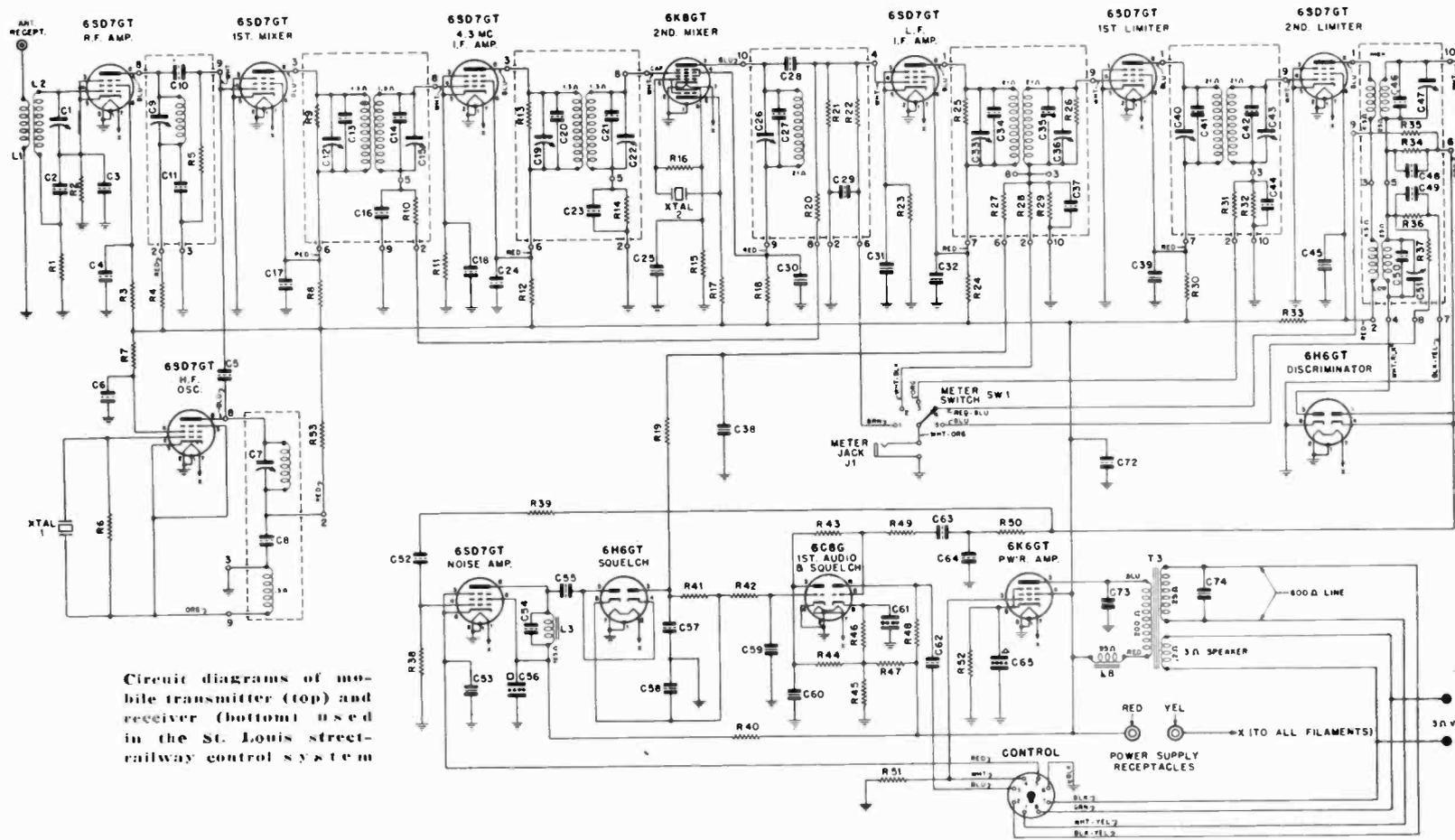
Circuit diagrams of mobile transmitter (top) and receiver (bottom) used in the St. Louis street-railway control system
