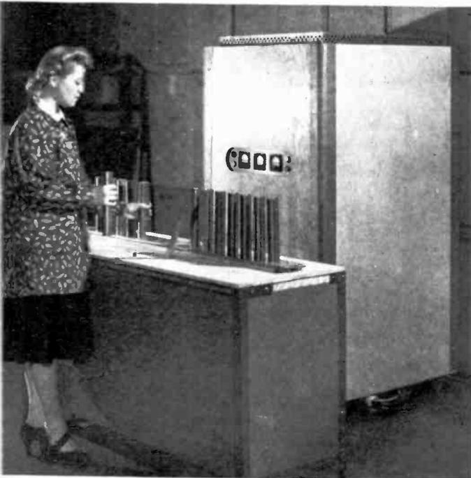
Above, the incendiary bombs in this photograph were among those Doolittle dropped on Tokio. The girl is inserting bombs in a special heating coil for quick, multiple brazing operation with induction heating.
