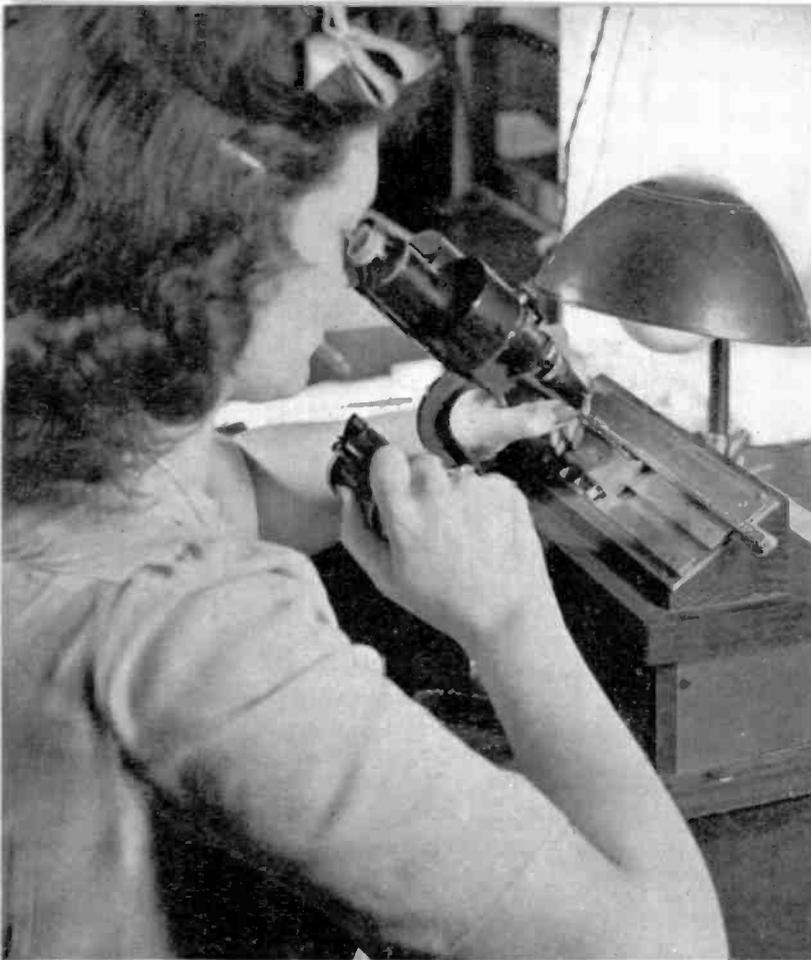
Microscopic inspection of glass V-jewel bearings, for all types of electrical measuring instruments, at West Lynn General Electric plant. Special-glass jewels, now in mass production, replace natural and synthetic amethyst previously imported.
