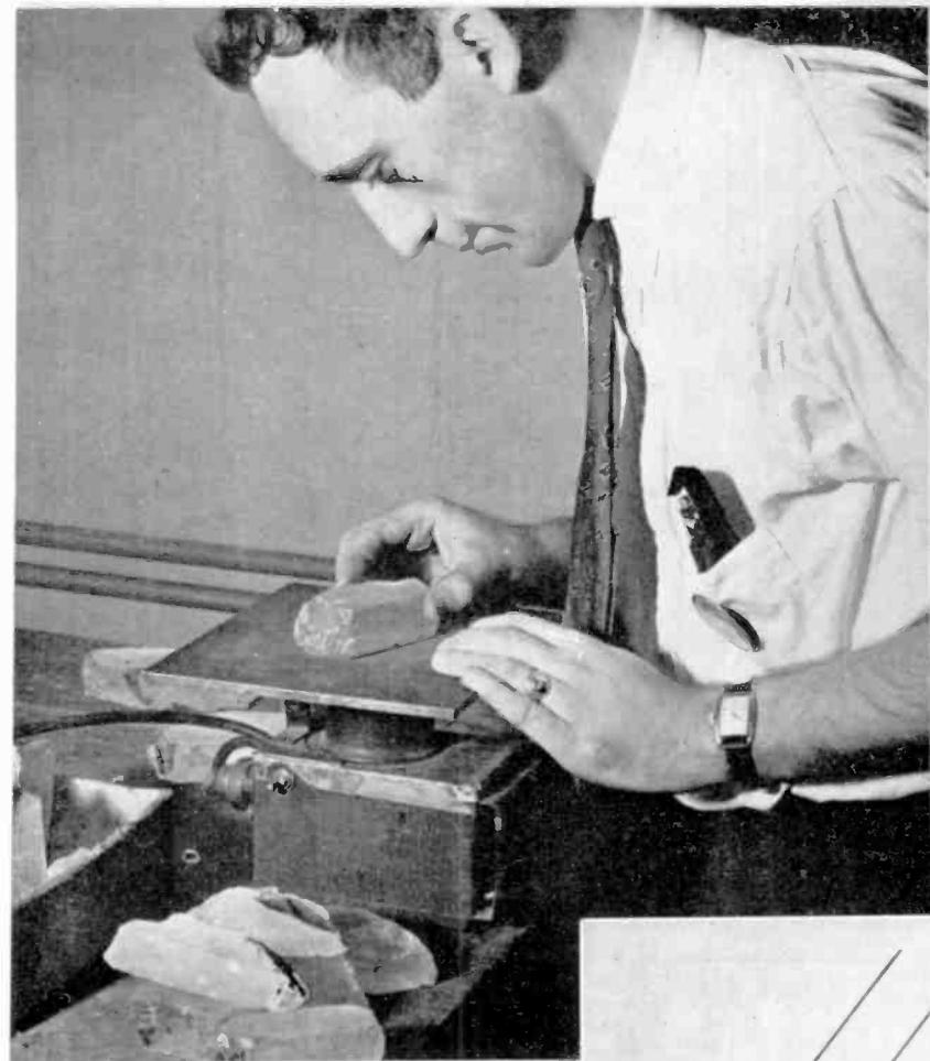
In cutting quartz bars, considerable savings are effected by a special mounting fixture designed by Joseph Eckert, RCA X-ray operator, above. The bars are mounted as shown in his shop sketch. Each bar is sampled during blanks set up without cutting intermediate wedge blanks. In addition to savings of quartz, special mounting saves saw set up time, X-ray measurement time, and orientation time.
