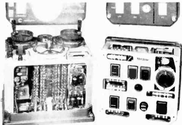
F.U.G.-10 aerial set controller, and interphone switch box. A button is provided on switch box for "cutting out" rear gunner
