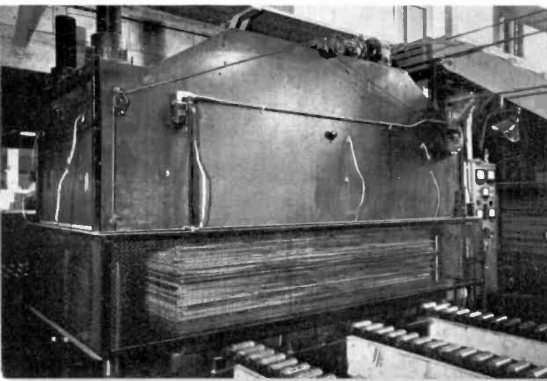
Close-up of electrode centered in stack of plywood panels of various thicknesses. Top and bottom press plates, or followers, are grounded
