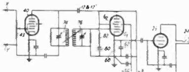
signal energy and a small reactance for the demodulation of FM. The output circuit includes a load resistor connected between cathode and a point of relatively fixed a-c potential. M. G. Crosby, RCA, (F) April 6, 1940, (I) September 15, 1942. No. 2,296,090.
