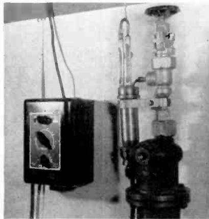
A sample cooler is available for attachment to steam or hot sample source with a needle valve for adjustment of flow, and a thermometer for measuring temperature of cooled sample. The conductivity cell contains two platinized electrodes and measures resistance.
