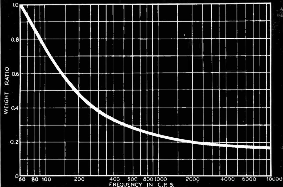
Fig. 5. Relative size of transformers for different frequencies
