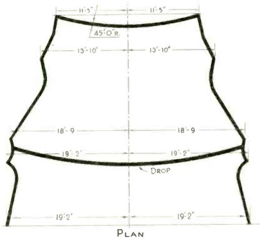
**EXPONENTIAL-HORN FORM** given the stage section is clearly shown in both sketches and photographs. These also reveal details of the 2-ton curved "drop" which can be lowered to cut off the backstage, when entire space is not needed for a 125-piece orchestra
