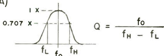
$f_L$  AND  $f_H$  ARE FREQUENCIES AT WHICH GAIN IS 0.707 OF PEAK VALUE
