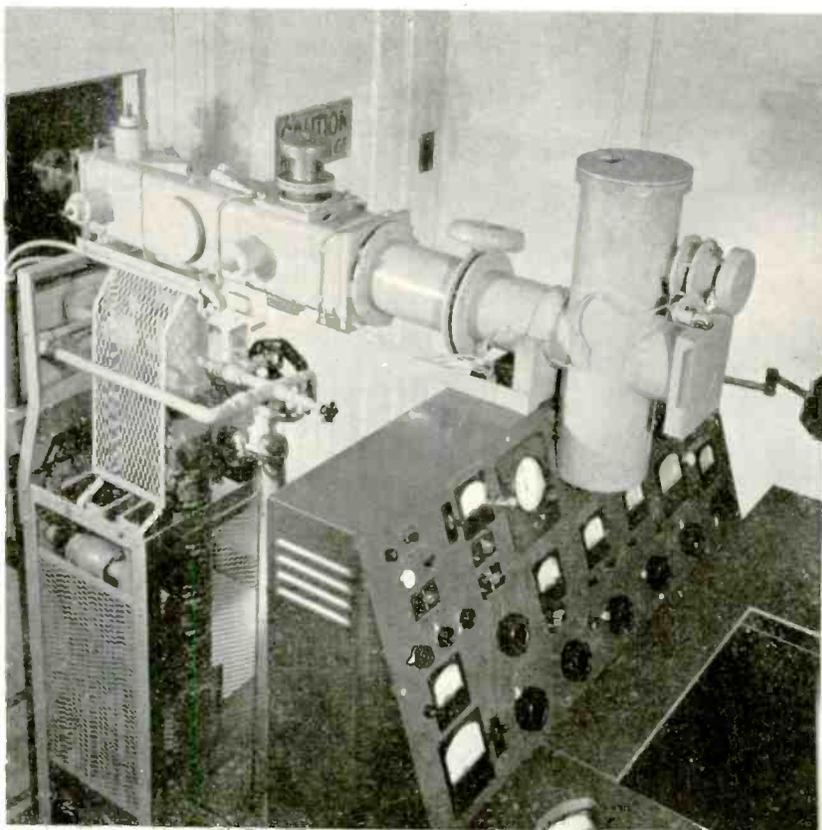
**THE STUDY OF ATOMIC STRUCTURE** is one phase of research activity at Murray Hill. Above an electron-diffraction camera is set up for investigating the crystal structure of surface films. A beam of high-speed electrons, scattered from the surface of the material being studied, records its diffraction-pattern on a photographic plate
