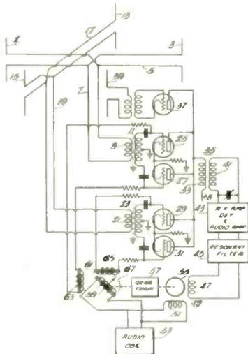
move. If the received waves do not apply equal currents to the antennas, unequally modulated components will modulate the carrier and will be applied to the receiver which, upon demodulation, will cause rotation of rotor 55 until equal and opposite modulation components are produced in the pairs of balanced modulators 25, 27 and 29, 31. The bearing of the waves will be indicated by pointer 67. V. D. Landon, RCA, (F) June 28, 1940, (I) March 16, 1943, No. 2,314,093.
