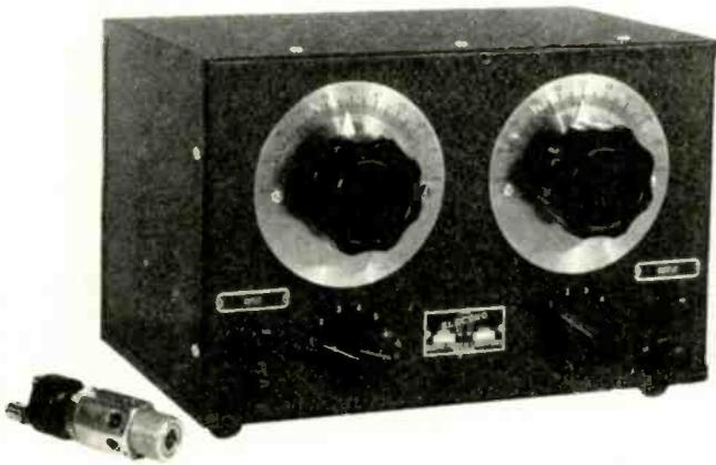
Analysis of the oscillograms of detonation effects is readily carried out with the above equipment (Fig. 1) developed by Electro Products Labs, 549 W. Randolph St., Chicago
