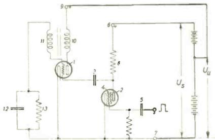
**Saw-Tooth Generator**—As will be seen from the drawing, the voltage  $U_s$  applied to condenser 3 is higher than plate voltage  $U_u$  of generator tube 1. By this provision a high negative grid-potential is obtained, blocking the generator tube immediately upon discharge of condenser 3 through synchronizing tube 2, and correct synchronization is effected. H. Baehring et al, Alien Property Custodian, (F) March 20, (I) Feb. 2, 1943, No. 2,310,198.
