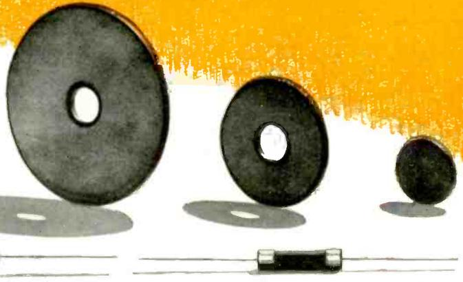
**THYRITE\*** is a silicon-carbide ceramic material, dense and mechanically strong, having nonlinear resistance characteristics—the resistance varying as a power of the applied voltage. Its resistance characteristic is stable, and substantially independent of polarity or frequency. Thyrite has been used for many years in many important applications, including electronic. Thyrite can be produced in various shapes and sizes (those which can be successfully molded).
