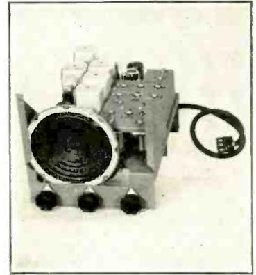
Series 6, five channel fixed tuned receiver. Model illustrated not crystal controlled.
