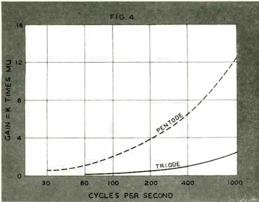
Fig. 4. Gain expectancy when optimum ratio is employed
