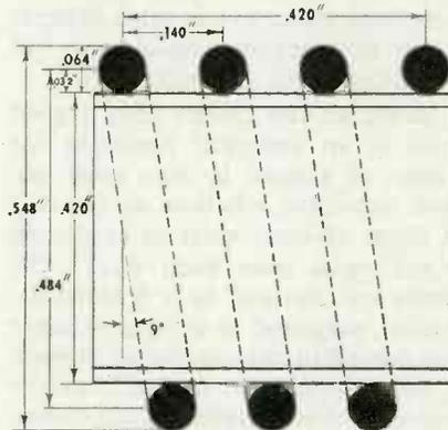
Fig. 2. Three turn wire-wound coil
