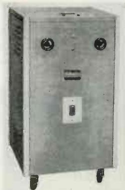
in the article or molecule itself by reason of its molecular resistance to the high-voltage, high-frequency current passed through it from flat electrode plates covering opposite sides or top and bottom of the mass to be heated. All coils, tubes, controls, etc., are encased in a compact safety cabinet.
