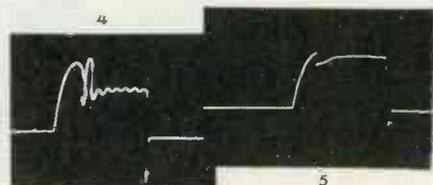
Curve (4) shows an average amount of bounce attendant on the closing of relay contacts. Curve (5) was obtained from a similar relay operating under conditions wherein the bounce has been eliminated.
