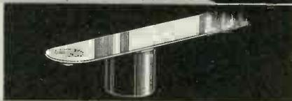
Heelpiece and coil core of magnetic metal, carefully annealed.
