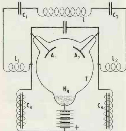
determined by these constants. Stable operation is aided by the inductive chokes in the anode supply leads, shown as  $C_H$ . The Vreeland tube is thus, basically, a synchronous switch.
