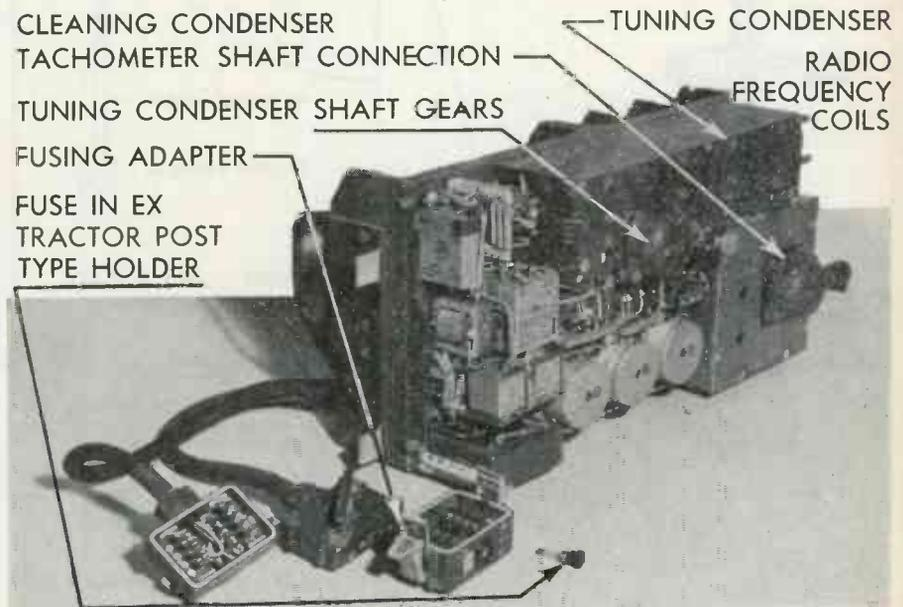
RADIO compass receiver is trf unit covering two bands for aural and visual use
