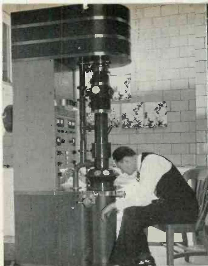
**ELECTRON MICROSCOPE** at Goodyear research laboratory aids in study of natural and synthetic rubber structure. Note photos on wall.
