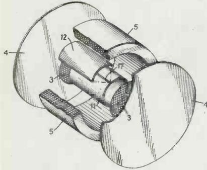
of the cycle, but electrons continuously withdrawn from cathode 12 are stored up within cylinder 11 as rotating space charge and are extracted as they are needed by the main oscillating circuit. W. T. Gibson, International Standard Electric Corp., (F) May 8, 1940, (I) July 20, 1943, No. 2,324,772.
