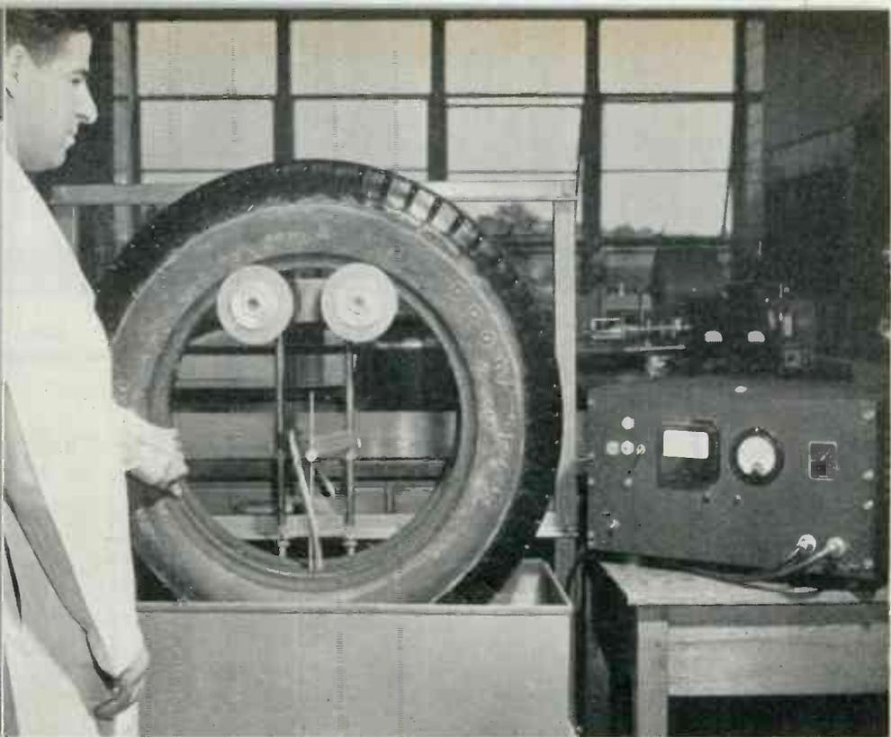
**ULTRASONIC** waves test tires in Goodyear Laboratory, Akron, Ohio. Magnetostriction generator in water feeds mike inside casing. Red light on panel indicates ply-separation. If tire is soild, mike receives signal and green lamp lights
