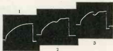
Oscillograms demonstrating (1) current rise in relay coil, armature not moving, (2) current rise with dip caused by increasing reactance when armature moves to close contacts, (3) current rise curve displaced by introduction of a voltage through contact circuit when contacts are not closed. Indicates time of operation, and whether or not bounce is present.
