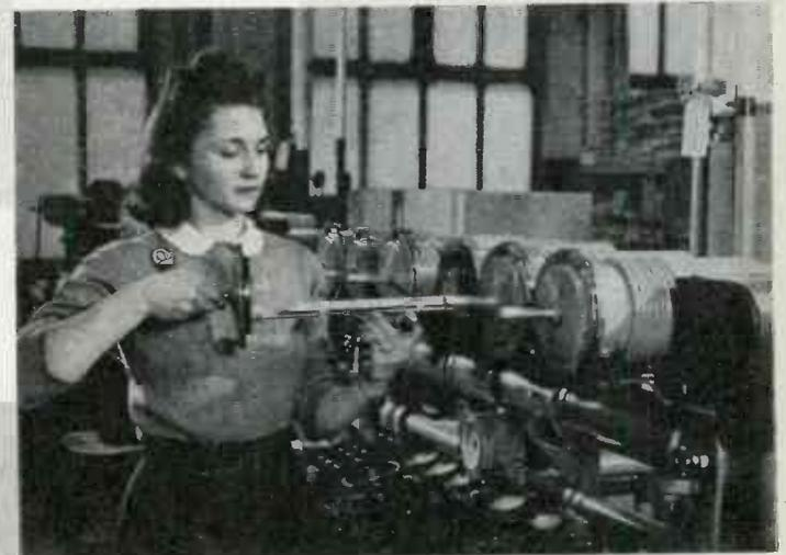
**SILVER SUBLIMATION** method efficiently plates quartz crystals in Western Electric Chicago works. Operator inserts tray of finished blanks into vacuum chamber for evaporation and deposition of protective silver film
