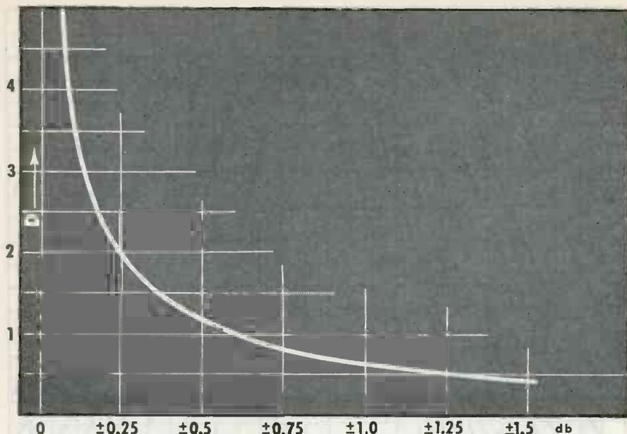
Fig. 3. Values of the Dip Function,  $D$ , as a pure number for various departures from flatness, in decibels
