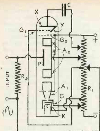
Fig. 6. Scanning wave generator directly synchronized
