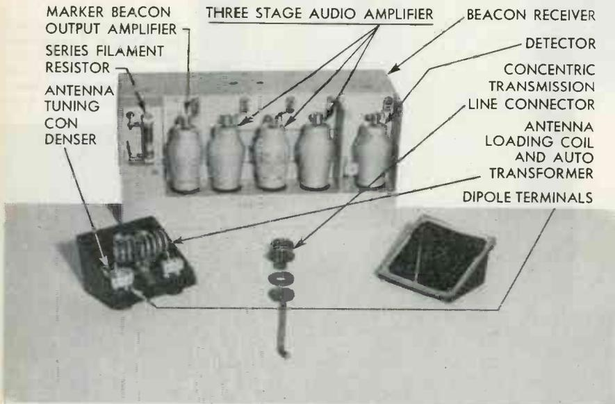
BLIND landing equipment removed from case to show arrangement of the tubes
