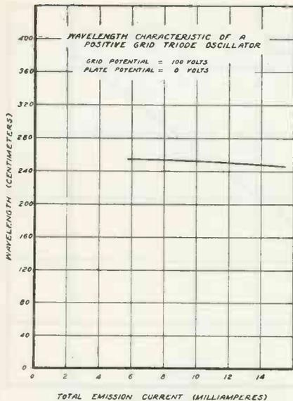
Fig. 5. Frequency is varied only slightly by change in cathode current
