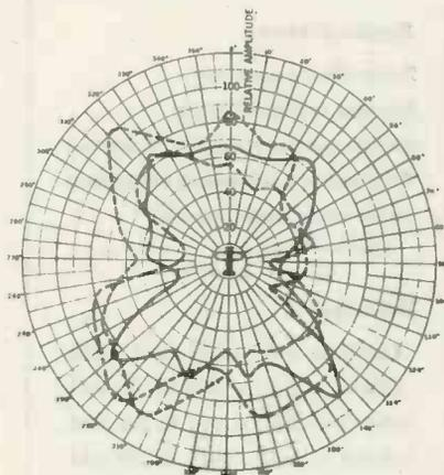
**Horizontal pattern obtained with airplane in level flight over a fixed point at various headings**
