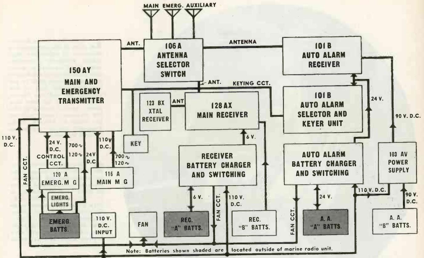
Block diagram of the complete circuits used in the Federal marine transmitter unit which provides for telegraph communication and an automatic alarm system
