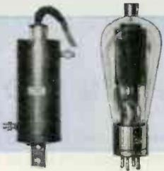
The G-E ignitron is the power tube and the G-E thyatron is the timer
