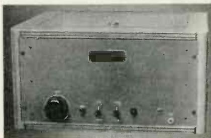
to 60 wpm by means of a Leach relay, relays disconnect the modulators and make other adjustments to insure clean, chirpless keying. The key is in the cathode circuit of the oscillator, with the relay operated by a self-contained 12-v dc source. Modulation capacity is 100 per cent, audio fidelity 100-6000 cps with low distortion. The output coupling circuit is self-contained, and may be matched to available antenna equipment. Manufacturer is Gates Radio & Supply Co., Quincy, Ill.
