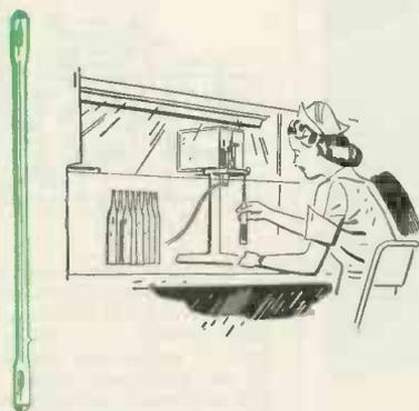
**Bacteria and Mold are Destroyed** by ultra-violet radiation produced by the Westinghouse Sterilamp, an electronic tube. Sterilamps are widely used to sanitize the air in rooms or working areas where pharmaceuticals, medical supplies or foods are prepared, processed or stored.
