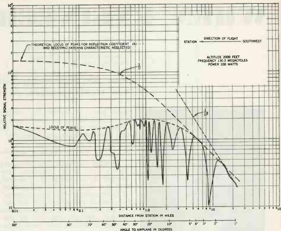
Recording of signals received from Floyd Bennett field during a flight at a constant altitude of 2000 feet
