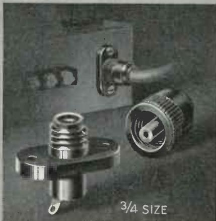
Another exclusive Millen "Designed for Application" product. Combination high voltage terminal and thru-bushing. Tapered contact pin fits firmly into conical socket providing large area, low resistance connection. Pin is swivel mounted in cap to prevent twisting of lead wire. Easy to use.  $\frac{1}{4}$ " o.d. insulation high voltage cable fits into opening in cap. Bored conductor passes thru pin for easy soldering to pre-tinned tip of contact plug.
