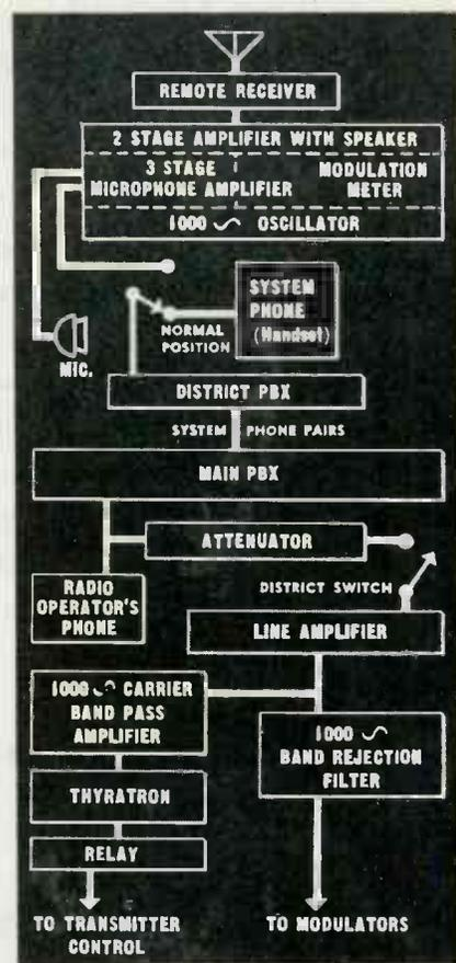
Block diagram showing method used by Detroit Edison in controlling transmitter over regular telephone circuits. Tone remains on the line all the time the transmitter is in use but filter attenuation results in its reduction to the point where it is barely audible
