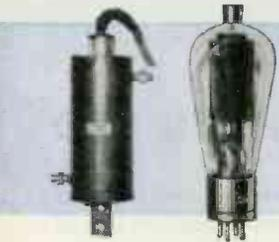
**The G-E ignitron is the power tube and the G-E thyatron is the timer**
