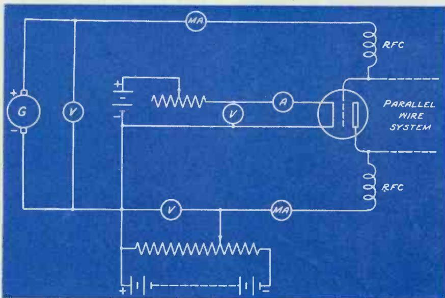
Fig. 2. Test circuit of positive-grid oscillator using transmission line tank. Line should be approximately 1/2 wavelength
