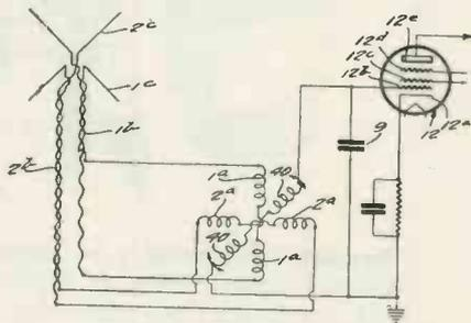
both antennas at a continuously varying degree. The directional effect obtained is the same as if one doublet were rotated. H. C. Forbes, Colonial Radio Corp., (F) Jan. 18, 1941, (I) May 25, 1943, No. 2,320,124.
