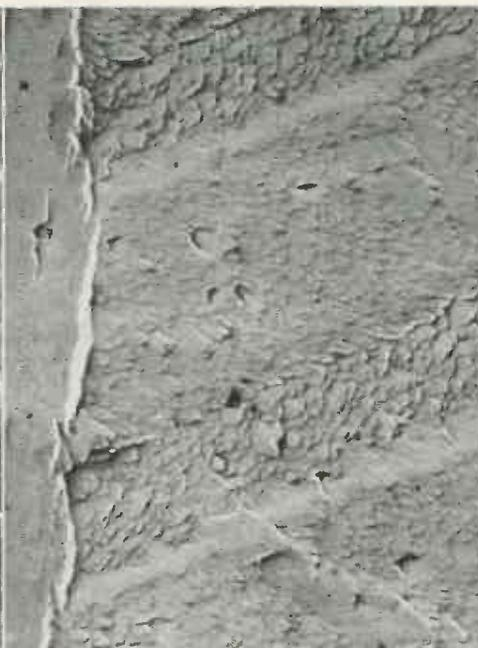
Etched copper viewed through polystyrene - silica technique
