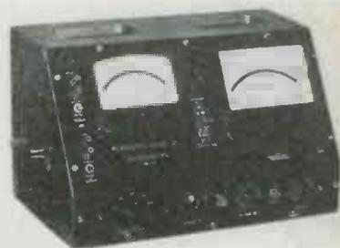
Fig. 1. Coil disjuncter oscillator unit houses rectifier and first three tubes shown in schematic. Three typical coils shown range in size from 1-in. to 8-in.
