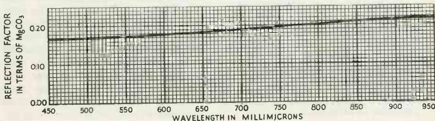
Spectral reflection of polished graphite film in the visible and infra-red regions. Below, curve for matte film
