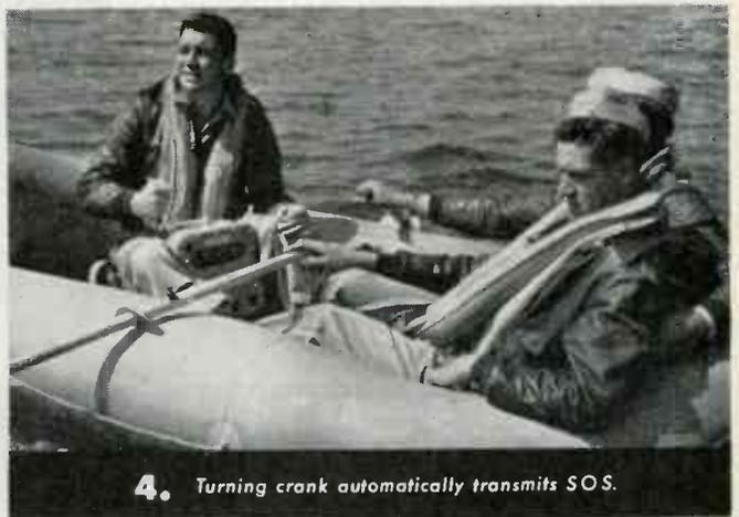
4. Turning crank automatically transmits SOS.
