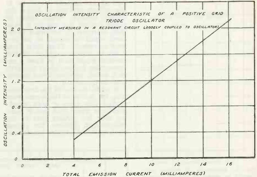
Fig. 3. Strength of oscillations is linear function of total cathode current over range observed
