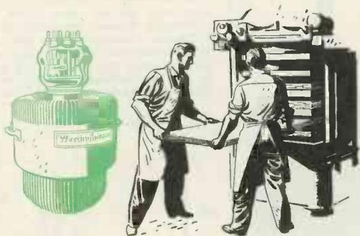
**"Bonding" Plywood** is an important new application of high-frequency heating. Operations which formerly took hours are now performed in minutes. Vacuum tube oscillators, similar to radio broadcasting tubes, are used to produce uniform heating throughout the piece—without injury to finish or structural qualities.
