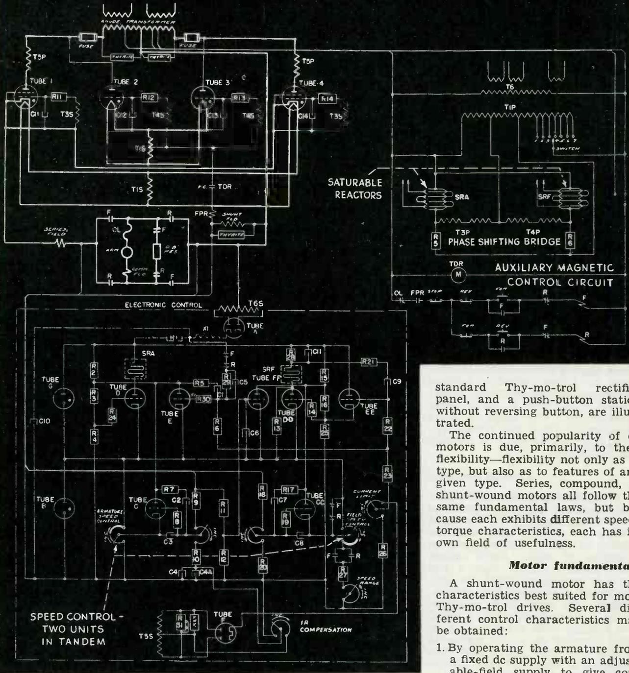
Basic equipment connections for the Thy-mo-trol electronically controlled variable speed motor drive, with auxiliary control features applicable to a 1 hp dc motor
