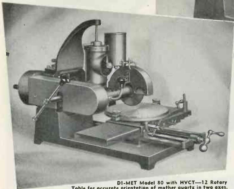
DI-MET Model 80 with HVCT—12 Rotary Table for accurate orientation of mother quartz in two axes.
