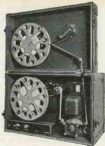
Men in our Armed Forces quickly learn how to receive international code on this Portable Keyer made by Waters Conley. It takes an inked record from paper tape and converts it, by the magic of electronics, into audible code signals.
