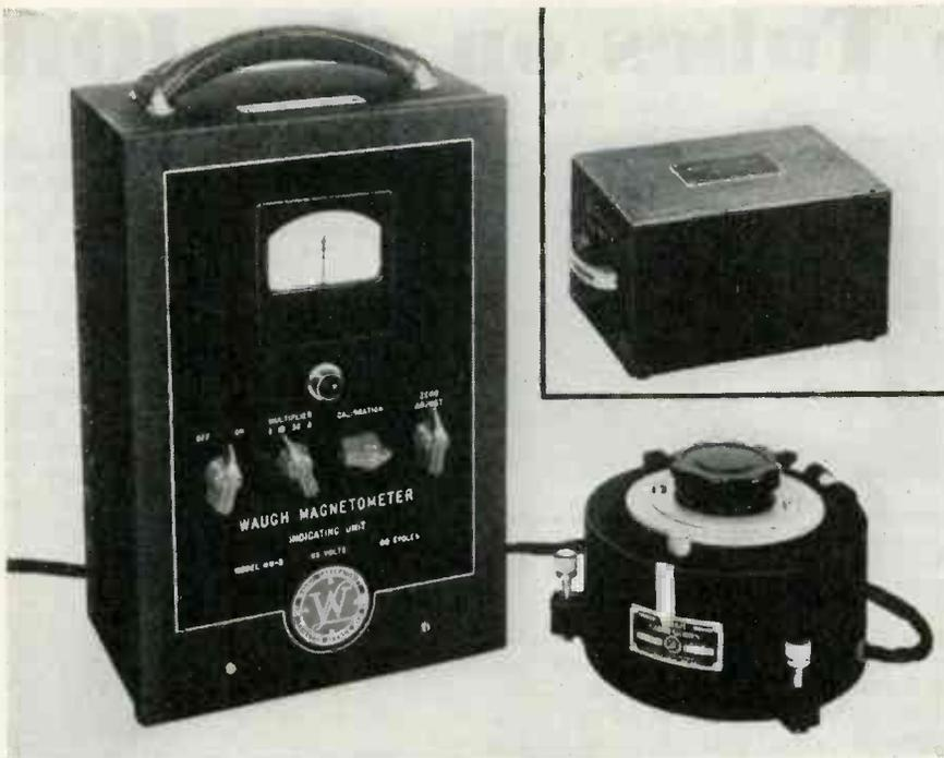
Field strength indicator and two styles of pickup units for measuring residual field of a part (upper) and field strength (lower)
