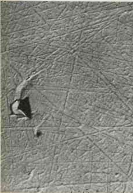
Slip bands in a calcite crystal viewed through polystyrene-silica technic
