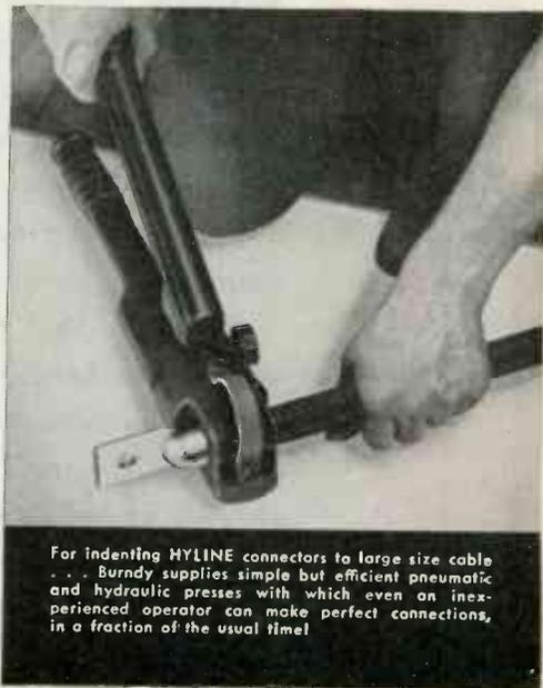
For indenting HYLIN connectors to large size cable . . . Burndy supplies simple but efficient pneumatic and hydraulic presses with which even an inexperienced operator can make perfect connections, in a fraction of the usual time!
