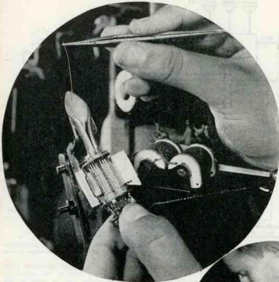
**1.** "Lilly jig" broke bottle-neck in the placement of filaments in miniature type tubes. Formerly a troublesome hand operation, accurate positioning of the fragile filaments is now done in far less time with help of the guiding jig and the buzzer which vibrates the wire into place. Annual saving of 12,600 "woman hours" will be the result in Newark, N. J., Tung-Sol plant. Device is covered by patents
