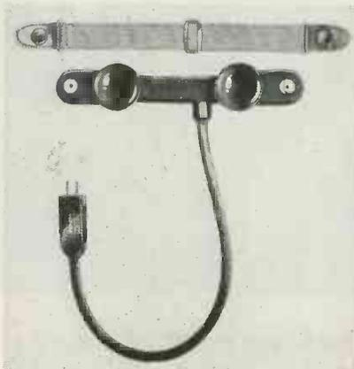
tic neckband. The plug is a non-locking breakaway type PL-291. Complete equipment requires the addition of an extension cord (CD354) and switch assembly (CD318 or CD308) containing the press-to-talk switch.
