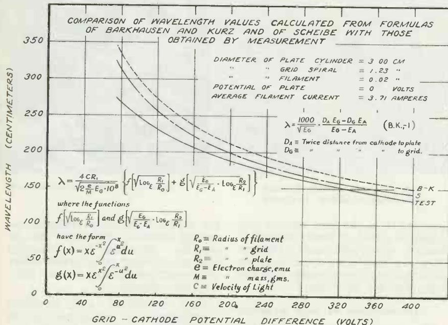
Fig. 1. Wavelength and positive grid-cathode voltage relations as computed and observed. Curve S is plot of formula at lower left
