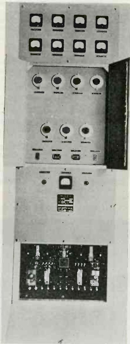
1. An airport traffic control transmitting system greatly superior to the present low frequency system has been realized by the application of ultra-high frequencies to this service.
