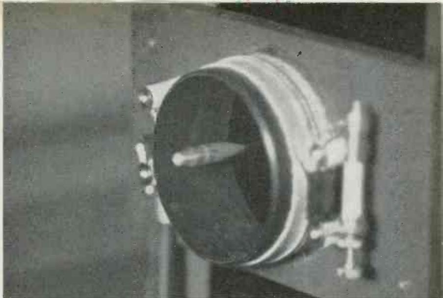
Fig. 2. High speed picture of a caliber .30 bullet at tripping position in a 3-in. coil
