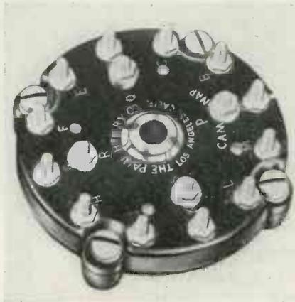
Any type of cam operating member can be used. Opening and closing of circuits requires but three or four degrees motion of the cam. Conservative current rating is 10 amperes at 29 volts, inductive load. The case is fully enclosed macerated phenolic; detent action can be furnished.
