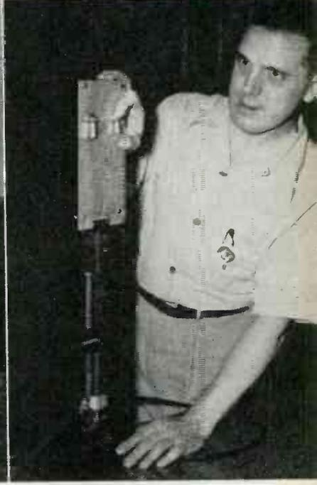
**7.** Differential pressure gage developed by Francis E. Pratt, Stromberg Carlson Co., Rochester, N. Y., for leak-test of pressure-sealed electronic equipment, detects changes of .001 lb. and cuts test from 4 hours to 7 minutes
