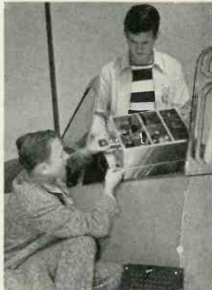
WHEN CONSOLIDATED VULTEE developed this superhuman radio flight reporter, the need for compact, reliable, portable power was met by Burgess Batteries—also used in all laboratory testing and development work at Vultee Field. When a plane is test-flown, stress and strain conditions at 70 key points equipped with gauges are relayed continuously to the ground station.
