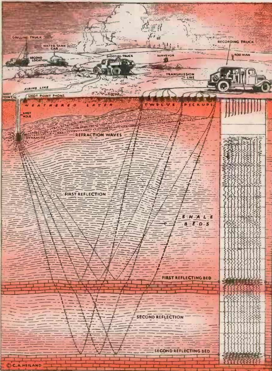
↑ Seismic reflection technic, showing wave-paths and record
