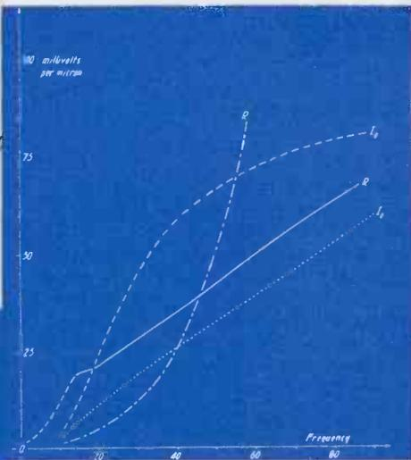
Voltage at grid of first amplifier tube in millivolts per micron ground motion (through impedance matching transformer) of commercial reflection detectors at various frequencies. R, reluctance types;  $I_0$ , inductive with oil damping;  $I_0$ , inductive detector electromagnetically damped. Heiland Research Corp.
