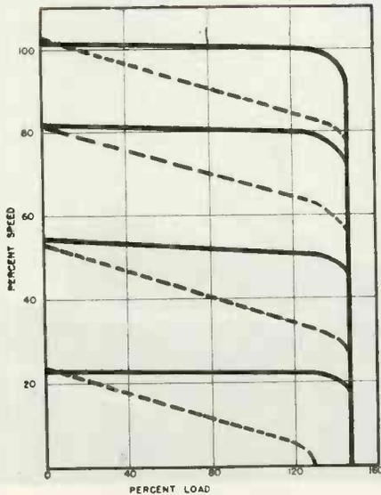
Speed regulation curves with (solid line) and without (dotted line) IR drop compensation
