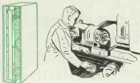
Where **Precision Work** is carried on, PRECIPITRON\* electric air cleaners remove tiny abrasive and corrosive particles that might damage highly finished surfaces. Electronic tubes rectify current, which charges every dust-bearing particle. These particles are drawn to, and precipitated on, charged collector plates.
