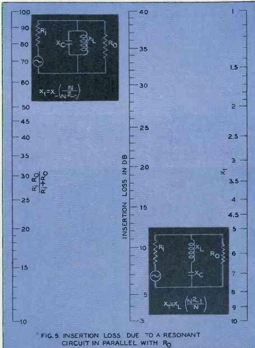
FIG. 5 INSERTION LOSS DUE TO A RESONANT CIRCUIT IN PARALLEL WITH  $R_o$
