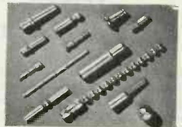
*These are typical **MULTI-SWAGE** products. Most of the electronic tube contacts used today are made by **MULTI-SWAGE**. This process will turn out large volume speedily, while maintaining close tolerances accurately.*
