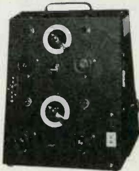
Coleman Universal Spectrophotometer Model 11 selects a monochromatic light band 35 mu wide, anywhere from 300-800 mu, with better than 2 mu precision. It passes light bands of any hue, including invisible bands at end of the spectrum, through any translucent product. Operation is simple.
