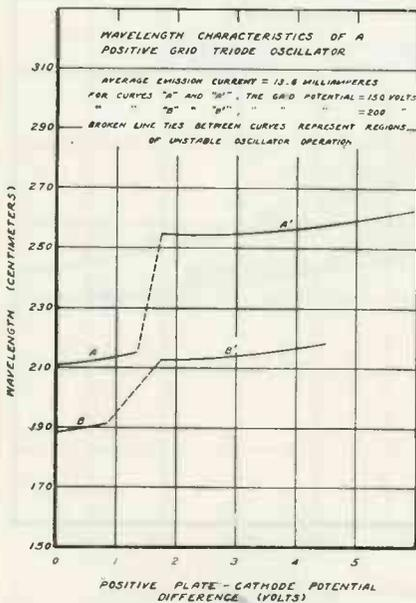
Fig. 6. Effect of positive plate voltage on frequency of oscillation
