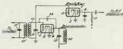
used for discriminator action. In the embodiment shown a separate rectifier tube 1 is included in the circuit. However, when suitably connected, the discriminator tube may at the same time act as rectifier. S. Hunt, RCA, (F) Aug. 26, 1941, (I) July 6, 1943, No. 2,323,603.
