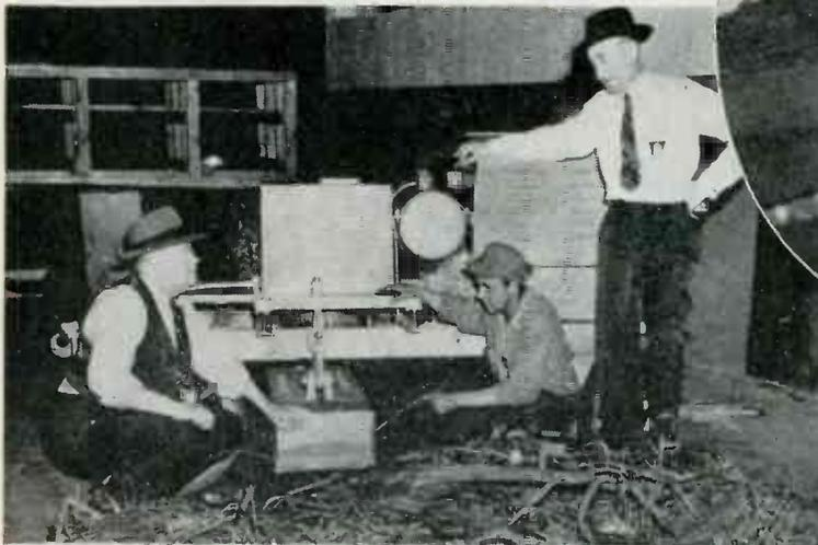
**3.** Factory scrap-hound, consisting of a trailer-mounted 16 x 54 in. electro-magnet energized by a "Jeep" motor, picks up as much as 700 pounds of ferrous scrap, and saves on sweeping costs as well as reducing hazard to personnel and factory truck tires in Willys-Overland, Toledo, Ohio, plant
