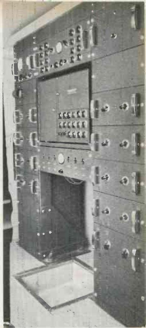
Nine dual amplifiers (one a spare) in 16-trace recording-truck installation of the Heiland Research Corp., Denver, Colo.
