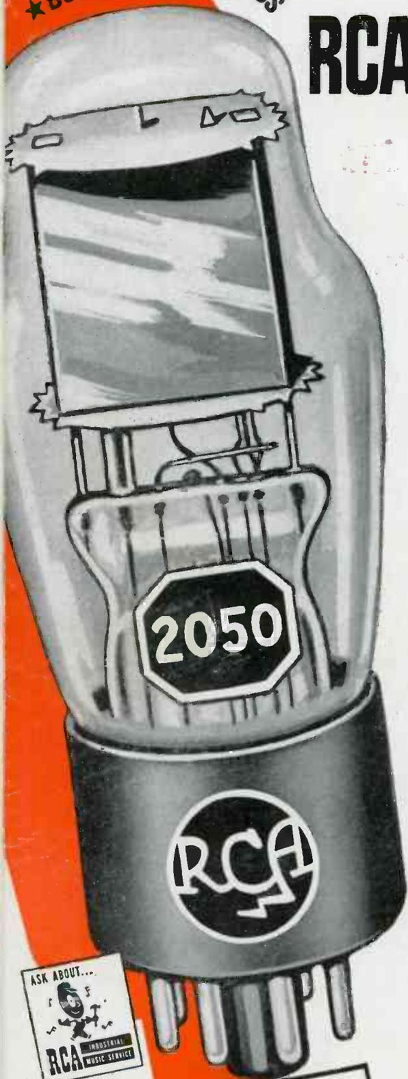
A THYATRAN is a "trigger" tube—a grid-controlled rectifier—which can "switch" power from full OFF to full ON with a very small change in control voltage.
