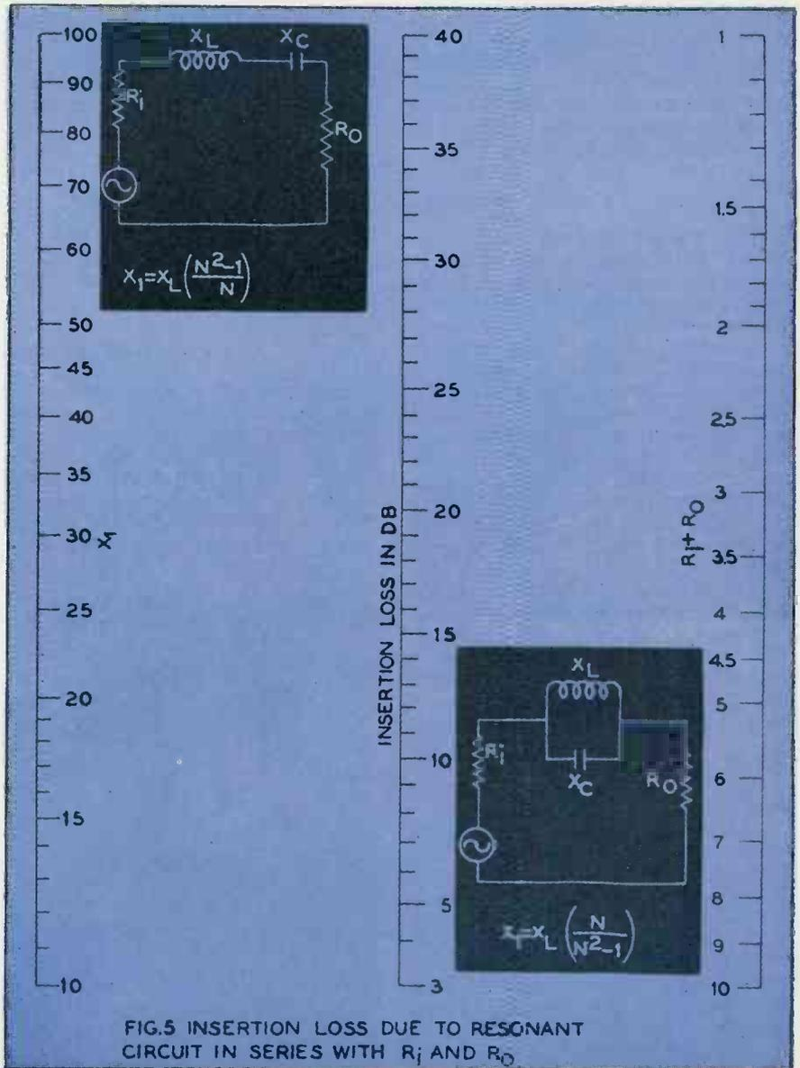
FIG. 5 INSERTION LOSS DUE TO RESONANT CIRCUIT IN SERIES WITH  $R_i$  AND  $R_o$
