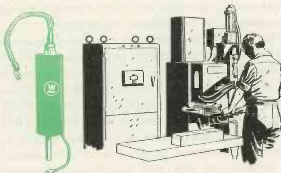
**Storing Electrical Energy** for resistance welding operations permits current to be drawn slowly from the a-c line—and applied in exactly equal amounts to produce strong, uniform welds. As the operator presses the switch, an exactly uniform amount of current is delivered for each weld by Ignitron tubes.
