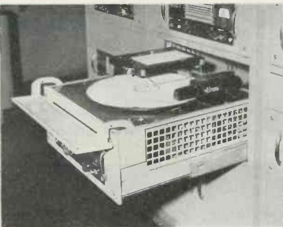
Memovox machines function in pairs with automatic signal to operator to start alternate
