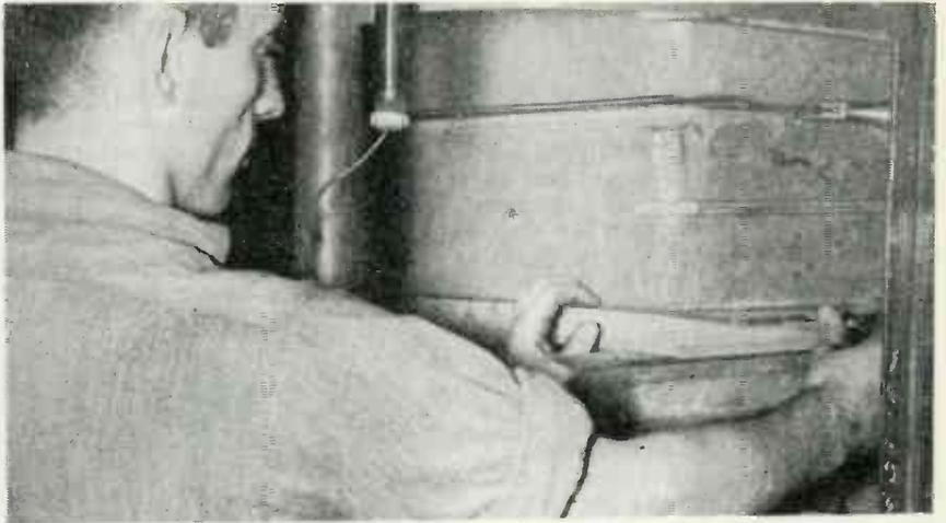
Showing position of copper plates on each side of block
