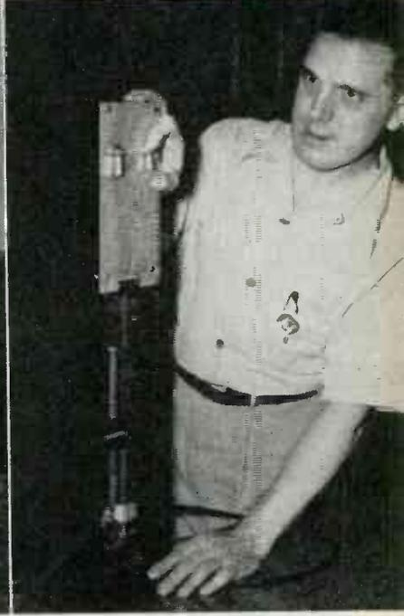
**7.** Differential pressure gage developed by Francis E. Pratt, Stromberg Carlson Co., Rochester, N. Y., for leak-test of pressure-sealed electronic equipment, detects changes of .001 lb. and cuts test from 4 hours to 7 minutes
