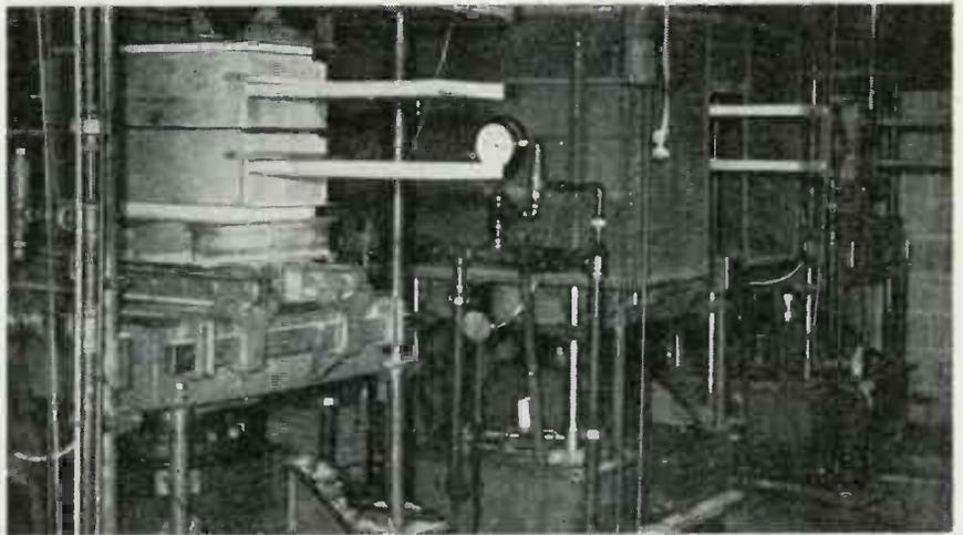
Battery of hydraulic presses with Pregwood blocks surrounded with thermal installation ready for gluing
