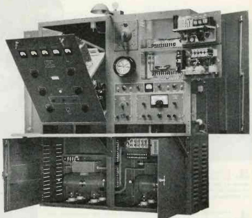
Self-contained, the new marine unit is designed for maximum accessibility and the easy replacement of essential operating components
