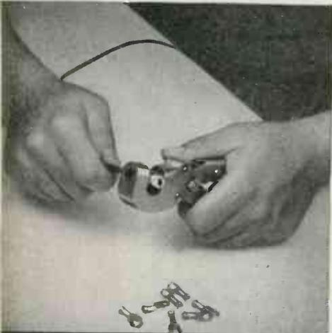
For small wire connections . . . Simply indent the HYLIN connector to the wire with the Burndy MYTOOL (pliers). A quick, simple operation requiring no skill.
