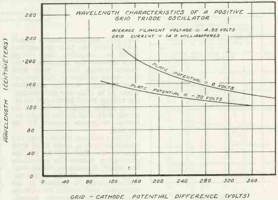
Fig. 4. Higher frequencies are reached when larger negative plate voltages and positive grid voltages are applied
