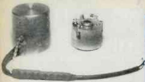
Electromagnetic inductance-type geophone, or ground-motion detector, used by National Geophysical Co., Dallas, Tex.
