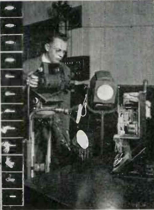
**6.** Fastax motion picture camera developed and improved by Bell Telephone Labs., N. Y. C., exposes 8,000 frames (200 ft. 16mm. film) in a second, for study of mechanical and other phenomena. Strip shows fuse blowing out
