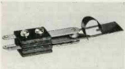
on 125 volts ac. Overall size is 3-1/16 x 11/16 x 1/2 in. It is made in single pole, single or double throw, set and return types, and also assembled to suit the needs of relay builders. It is manufactured by the Acro Electric Co., 1308 Superior Ave., Cleveland, O.
