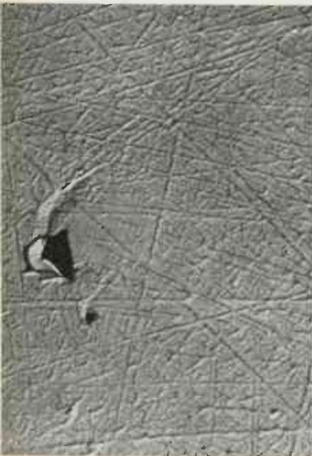
Slip bands in a calcite crystal viewed through polystyrene-silica technic
