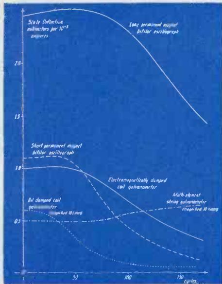
Response of various commercial recording-galvanometers
