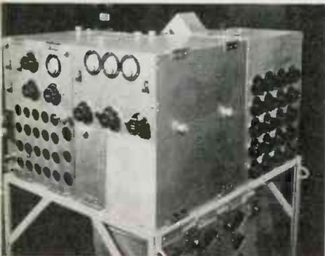
Control panel and timing system of Continental Oil Co. recording unit. Amplifiers mount in rack below
