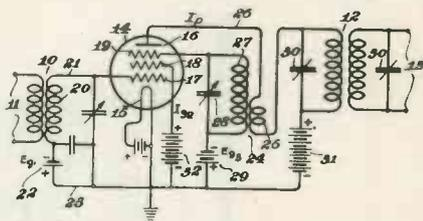
grid 18 shields negative grid 17 from negative grid 19 and prevents interaction between radio frequency and local oscillator circuit. In other examples shown grid 17 serves as oscillator grid and grid 19 as modulator grid. A way of effecting automatic volume control is described. The arrangement works as detector-oscillator if the generated frequency equals the carrier frequency of the modulated input wave. J. C. Smith, RCA, (F) Jan. 31, 1933, (I) June 29, 1943, No. 2,323,250.
