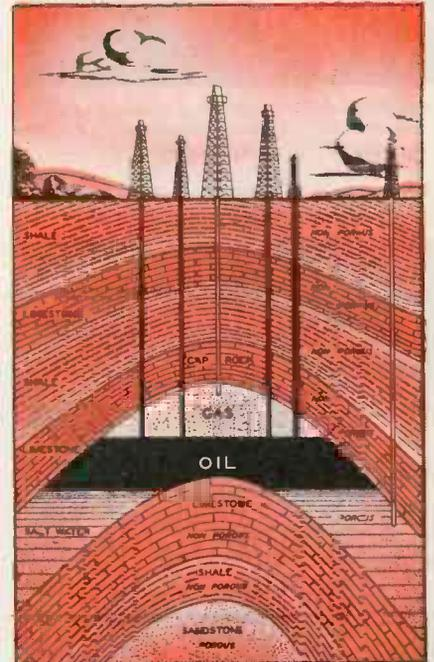
"Dome" or subsurface fold forming an oil-pool. "Dry hole" at right shows how easy it is to miss
