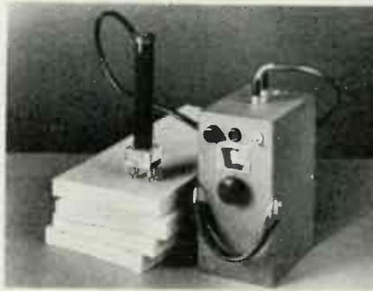
Method of electronically determining moisture content of wood using spiked instrument which is hammered in
