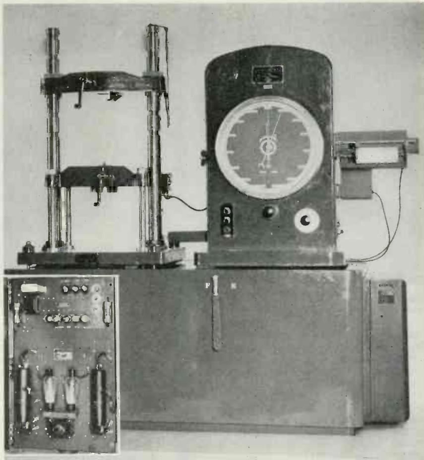
**Heavy materials testing machine powered by 2 horsepower motor and Thy-mo-trol drive. Inset shows control for start, stop and speed changes**
