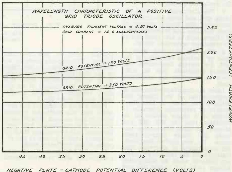
Fig. 7. Frequency of positive-grid oscillator is varied to greater extent by grid voltage than by plate voltage
