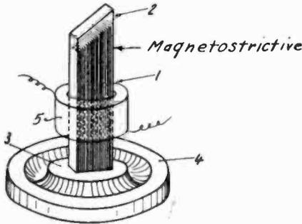
ity of narrow bars of unequal lengths and may have a mass 2 soldered to it. Experience shows that the microphone using the resonance of such a bar retains its sensitivity with an increase in the width of the pass band of 50 per cent to 100 per cent, useful in listening to submarine noises. Y. Rocard, Allen Property Custodian, (F) Feb. 24, 1940, (I) Aug. 31, 1943, No. 2,328,496.
