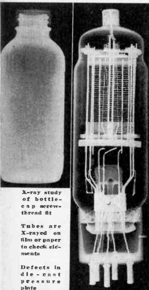
X-ray study of bottle-cap screw-thread fit
