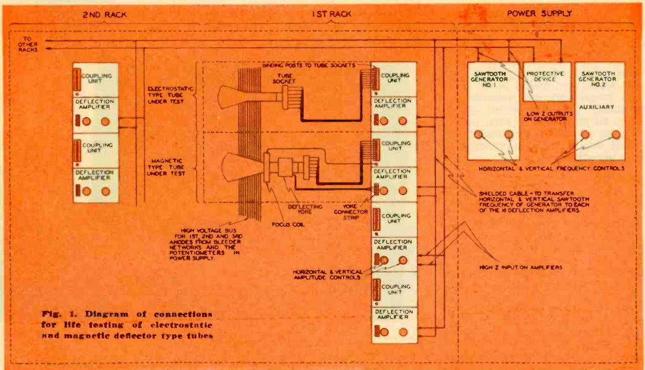
Fig. 1. Diagram of connections for life testing of electrostatic and magnetic deflector type tubes
