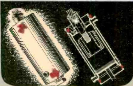
STAINLESS STEEL END HEADERS OF IGNITRON ITSELF IS SEAM WELDED VACUUM TIGHT TO WALLS.
