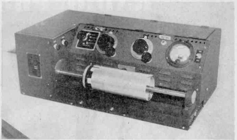
Transceiver unit of the FM sub-carrier radio photo equipment scans pictures 96 lines per inch, is synchronized by means of a fork oscillator
