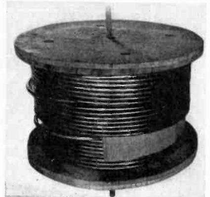
continuous lengths up to several thousand feet. The cable is wound on wooden reels and is electrically identical to rigid cables of the same size. It is easily uncoiled and bent by hand to the desired contour; connectors, junction boxes and expansion fittings are not necessary. The cable may be fitted at the factory with special glass-insulated terminals and shipped under pressure.
