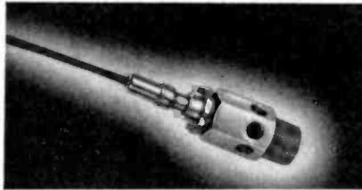
provides quick, reliable contact between connection cable and pickup. Adapter adjustments are much simpler because of the use of two set-screws which replace the older type hexagonal nut. The pickup coil has special impregnation to withstand operating temperatures of 350 deg. It is engineered to provide quick replacement of either diaphragm or coil and operates at constant polarity. Manufactured by Electro Products Laboratories, 549 West Randolph St., Chicago 6, Ill.
