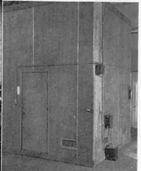
person using it at a time because of possibility of interference. A convenient floor plan is illustrated and is 7 x 12 ft., with a ceiling height of 12 ft. This ceiling height is desirable when radio compass work is to be carried on. A lower ceiling could be used but it makes the pattern next to the loop more complex, and hence more difficult to compute. In addition, the higher ceiling aids ventilation.
