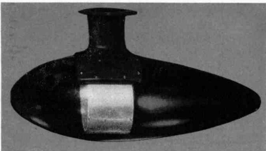
Fig. 1—Relative dimensions of streamlined housing for typical loop antenna as used in modern aircraft design. Housings for iron core loops may be considerably smaller
