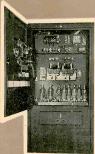
SEAM WELD TIMER with roller electrodes uses synchronously driven disc. Provides "On" and "Off" intervals.
