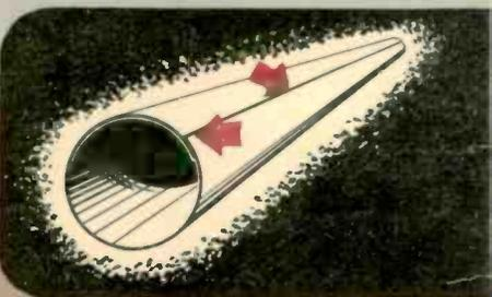
SEAM WELDED METAL FORM FOR CONCRETE PILING.
