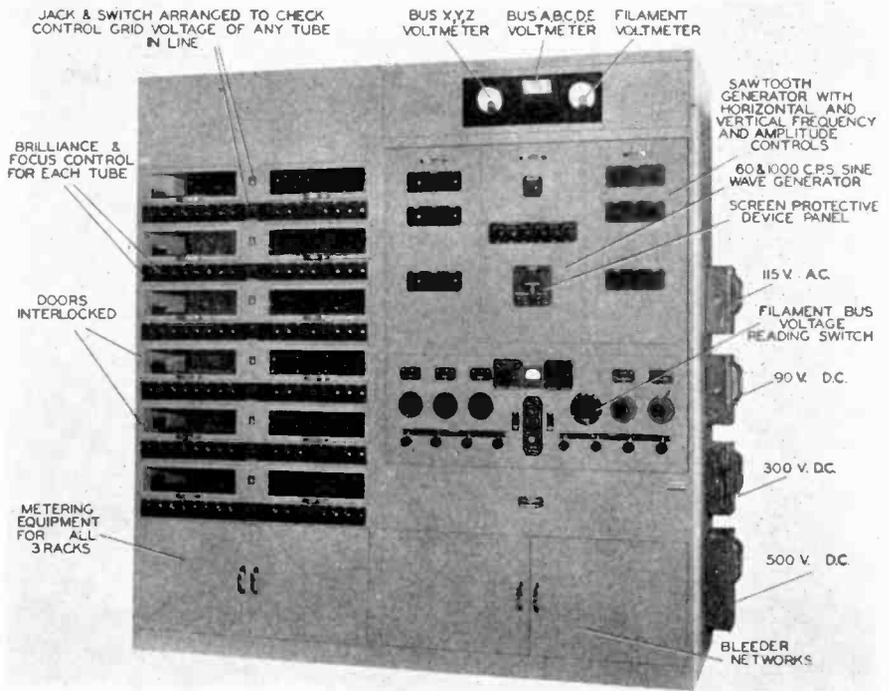
Fig. 6—18-position life test rack for electrostatic type tubes up to and including four-inch diameter
