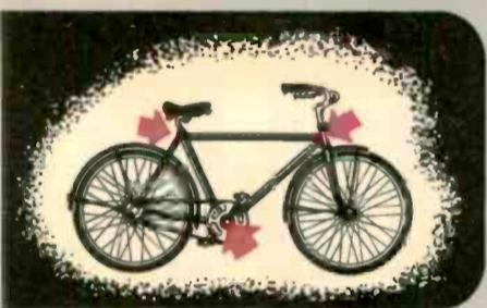
STEEL TUBING BICYCLE FRAMES BUTT WELDED.
