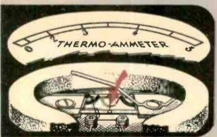
THERMOCOUPLE JUNCTIONS REQUIRE WELDING DISSIMILAR WIRES.
