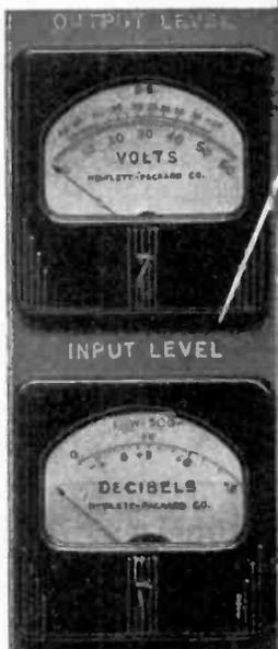
Separate input meter for making gain measurements
