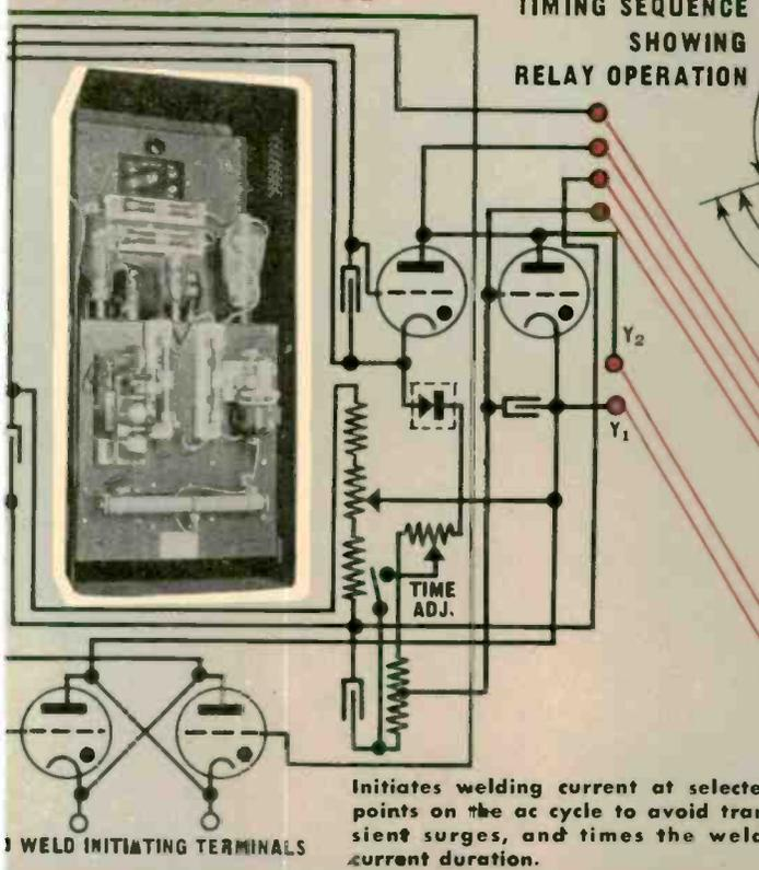
Initiates welding current at selected points on the ac cycle to avoid transient surges, and times the weld-current duration.
