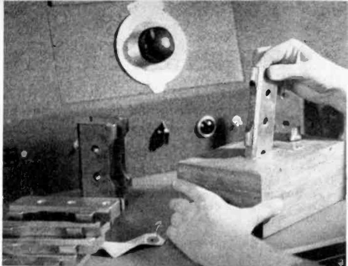
Testing case-hardening of gun breech blocks
