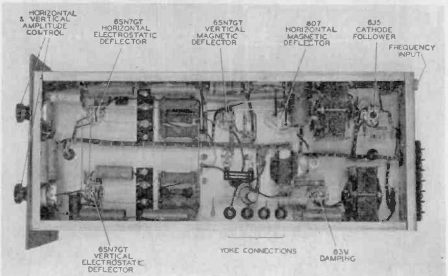
Fig. 4—Deflector chassis of sixteen-position rack
