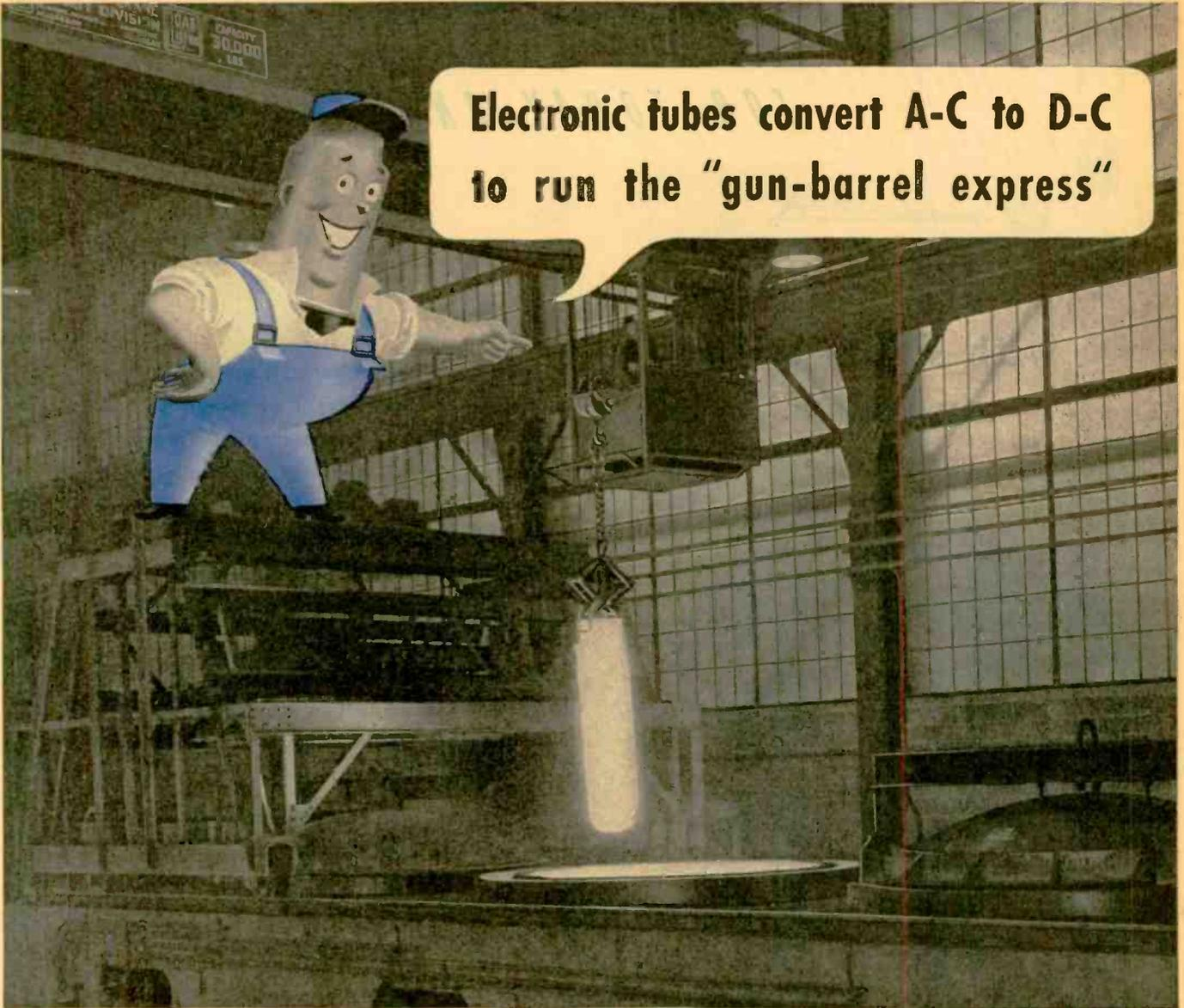
The General Electric sealed ignitron is used instead of rotating machinery
