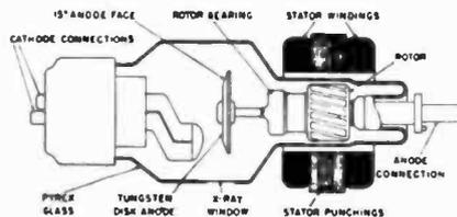
Rotating anode tube manufactured by Westinghouse
