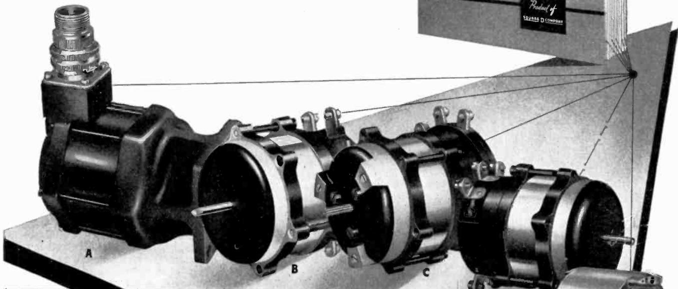
**A: KOLLSMAN TWO-PHASE GENERATOR**—High impedance, permanent magnet, two-pole generator, capable of operating at speeds up to 2500 R.P.M., delivering up to 83 volts. Compact, light in weight, and designed to operate under widely varying temperature and humidity conditions.
