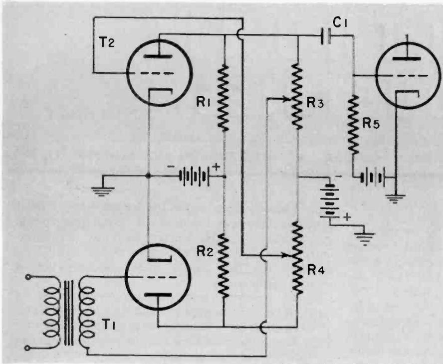
Fig. 1—Sine wave input to T<sub>1</sub> unbalances resistance bridge and produces square-wave output voltage of same frequency
