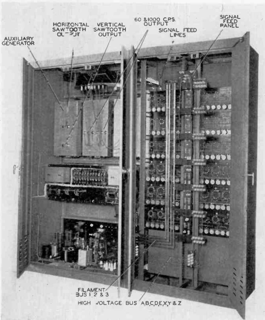
Fig. 7—Rear view of 48-position cathode ray life test rack illustrating interior wiring details and bus connections
