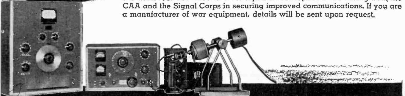
The Harmonic Wave Analyzer measures the presence of spurious frequencies introduced by microphone distortion. To the ear, such frequencies give the feeling of ragged and false speech quality that may be unintelligible under the stress and strain of battle.
