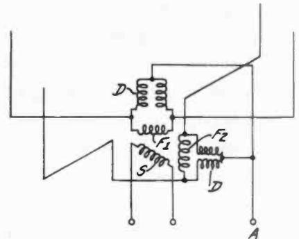
they have a very small inductance from the unjoined ends to the joined ends over the path provided for transmission of the non-directional antenna voltage. The inductance of chokes  $D$  is made to be high compared with that of coils  $F_1, F_2$ . K. G. Holsten, Allen Property Custodian, (F) July 5, 1941, (I) Aug. 17, 1943, No. 2,326,945.
