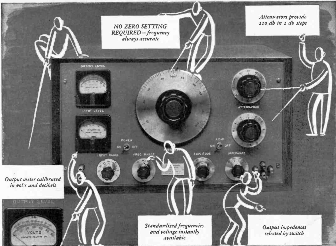
Output meter calibrated in volts and decibels
