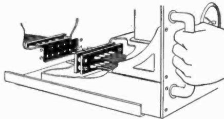
Both halves of this connector are mounted rigidly. One half mounts on the back of any electrically operated unit. The other half mounts on a rack or panel designed to hold the unit. By this means the excess weight of terminal strips and slack in the cable are eliminated.
