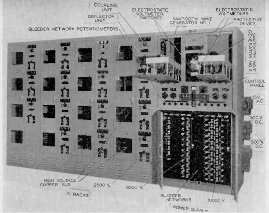
Fig. 2—Sixteen-position cathode ray tube life test equipment
