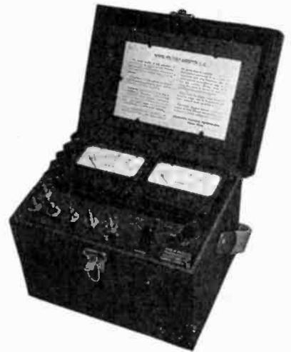
cover is hinged and contains space for a doughnut type transformer which is used in the higher ampere ranges.
