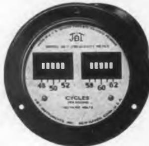
Model 30-F, double window, for ease in reading frequency in either range.
