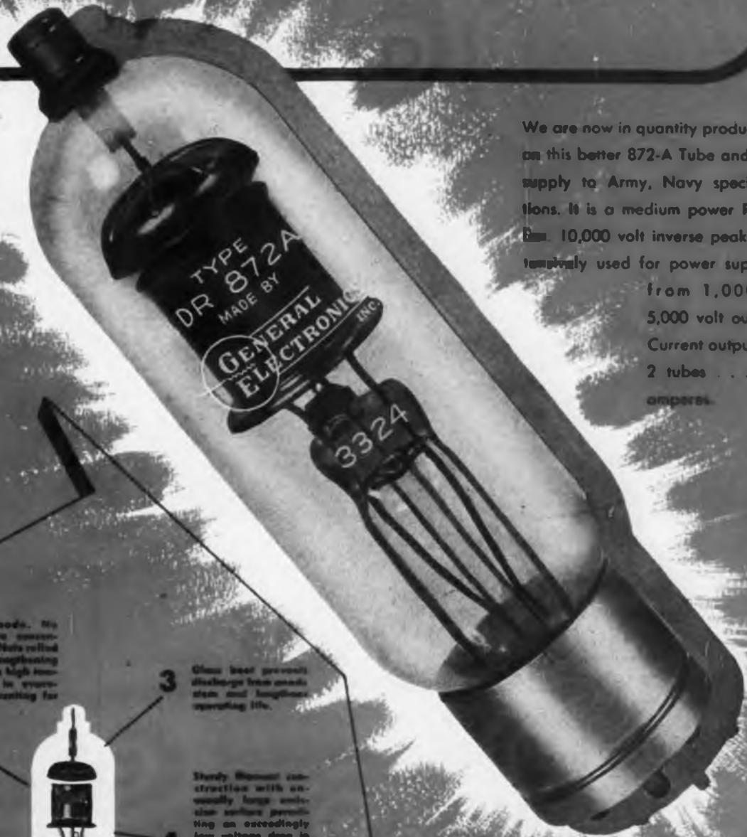
We are now in quantity production on this better 872-A Tube and can supply to Army, Navy specifications. It is a medium power Rectifier. 10,000 volt inverse peak. Extensively used for power supplies from 1,000 to 5,000 volt output. Current output . . . 2 tubes . . . 2½ amperes.
