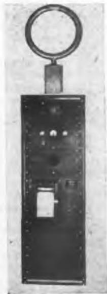
Radio range monitor constantly receives signals and automatically warns the control station of shift in radio course
