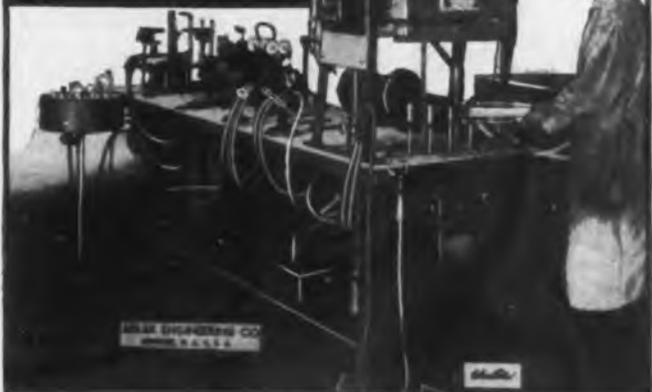
This electronic tube making unit fills the needs of schools, colleges, experimental and research laboratories for a compact machine complete in itself and capable of performing all operations required in the construction of incandescent lamps, radio tubes, electronic tubes and similar devices.
