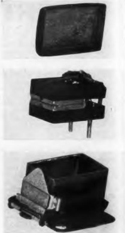
The recording and reproducing head removed from its case
