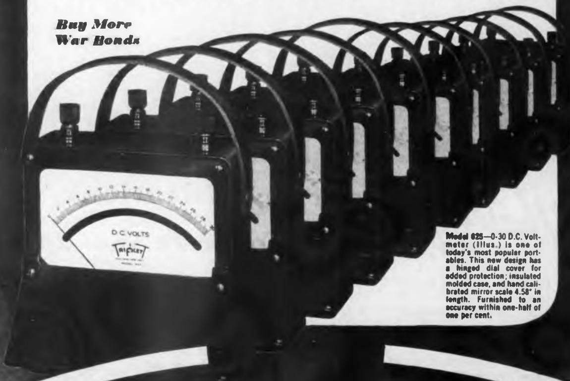
Model 625—0-30 D.C. Voltmeter (illus.) is one of today's most popular portables. This new design has a hinged dial cover for added protection; insulated molded case, and hand calibrated mirror scale 4.58" in length. Furnished to an accuracy within one-half of one per cent.
