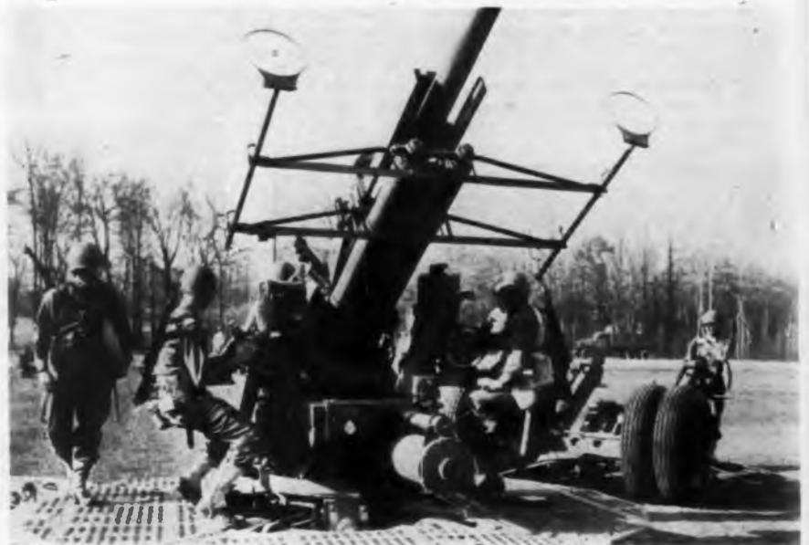
Gun pointers stand by but electronically controlled motors do the work
