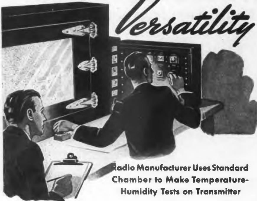
**Radio Manufacturer Uses Standard Chamber to Make Temperature-Humidity Tests on Transmitter**
