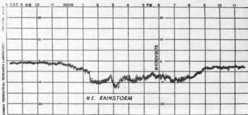
**10** ↑ Portion of record of October 26, 1943, showing point discharge between earth and sky during a rain-storm
