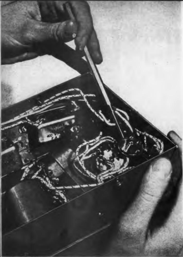
**2A** DENTAL MIRROR enables solder-girls and inspectors to see both sides of every connection at Electronic Labs., speeding wiring and eliminating rejects.
