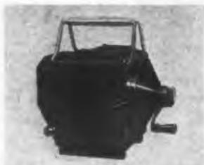
**THE NEW U. S.-MADE "MEGGER" INSULATION TESTER**—Consists essentially of a direct-reading true ohmmeter of the permanent magnet moving coil type mounted with a d-c hand generator in a plastic molded case. Ranges up to 1000 megohms, with hand generators up to 500 volts. Widely used in hard service. Variable-pressure ("Meg") and constant-pressure ("Super-Meg") types. Bulletin 1735-EI.
