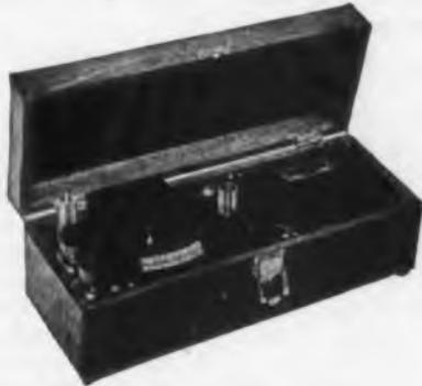
It operates with a barrier-lever photocell which is connected to a taut-wire suspension galvanometer. The instrument is built into a portable wooden case 5 x 6 x 15 in. and does not require any external power connection.
