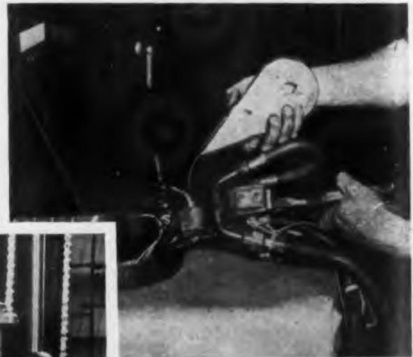
**4A** SILVER SOLDER dispenser, like old-time photoflash magnesium-ribbon holder, simplifies feeding solder to work being brazed and prevents waste. In old method, worker cut off a foot or two of solder and hand-held it. As it became short and hot, worker would drop scrap and get a new piece. Dispenser is a flat metal case containing roll of solder-ribbon and roller near tip over which solder is fed with thumb.
