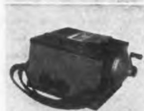
**THE "BRIDGE-MEG" RESISTANCE TESTER**—This instrument is a combined "Megger" Insulation Tester and a four-dial, multi-ratio Wheatstone Bridge. Will measure any ohmic resistance from .01 ohm up to 100 or 200 megohms; hand generators rated up to 1000 volts. A complete and compact resistance measuring unit that is ideal for power companies and industrial plants. Catalog 1685-EI.
