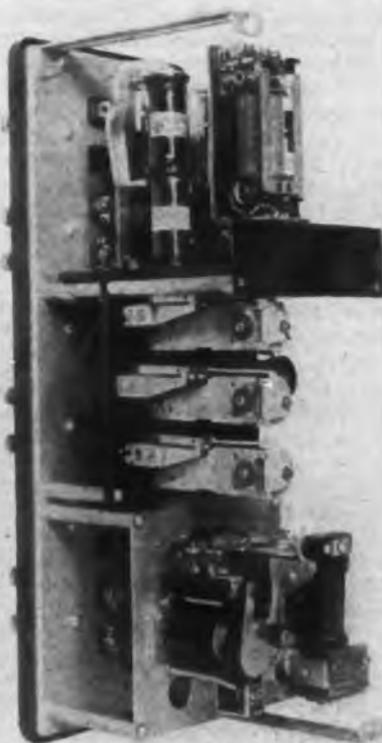
Fig. 12—Automatic synchronizer uses two low-power vacuum tubes
