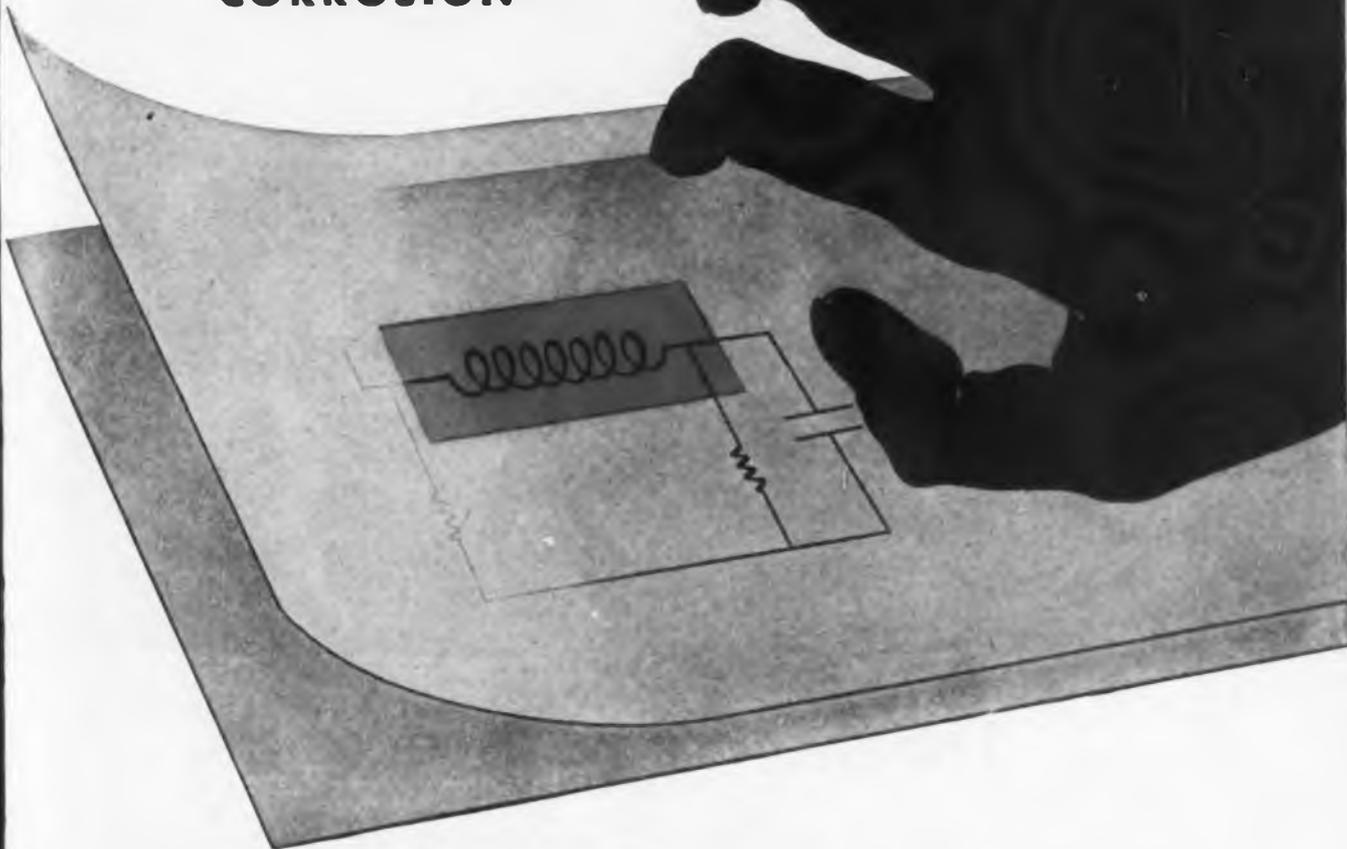
UNLIKE many dielectrics, Lumarith (cellulose-acetate base), when in contact with current-carrying copper wire, remains unaffected in the presence of moisture, and does not promote corrosion of the wire. In foil and film, it is used as an extra covering for bobbins and spools and as between-layer insulation in wire-wound coils—wherever the black hand of corrosion threatens.
