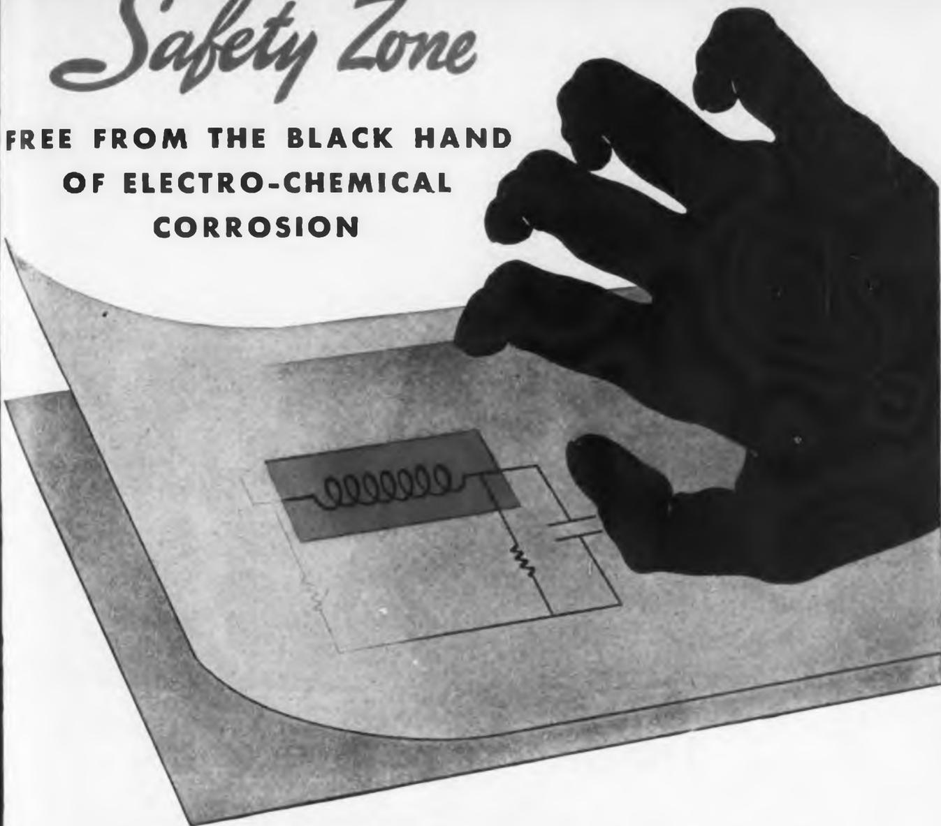
UNLIKE many dielectrics, Lumarith (cellulose-acetate base), when in contact with current-carrying copper wire, remains unaffected in the presence of moisture, and does not promote corrosion of the wire. In foil and film, it is used as an extra covering for bobbins and spools and as between-layer insulation in wire-wound coils—wherever the black hand of corrosion threatens.
