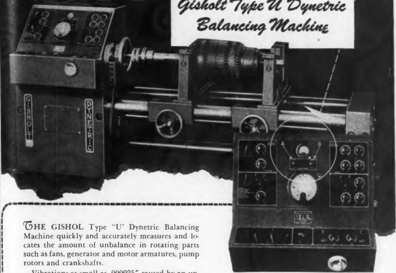
THE GISHOLT Type "U" Dynetric Balancing Machine quickly and accurately measures and locates the amount of unbalance in rotating parts such as fans, generator and motor armatures, pump rotors and crankshafts.
