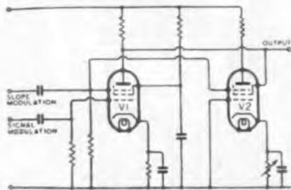
Controlling tube gain at constant dc current
