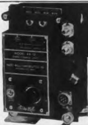
**LEFT** — Front of model AR-10-A with dust cover in place, showing Model AA-12 Channel and control selectors, loop and antenna connections.
