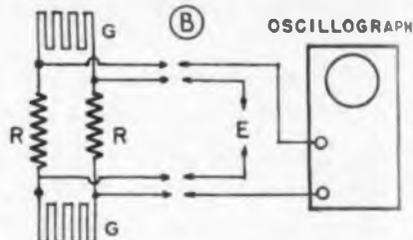
Fig. 4B—Where two strain gages are used, they may be connected to the oscillograph in this manner
