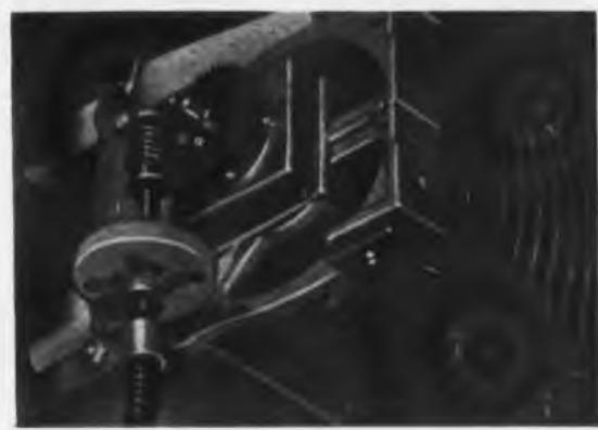
**S**EE how the use of these remote control flexible shafts enables you to put tuning elements in best positions for wiring and for optimum circuit efficiency and at the same time to centralize controls. The close-up shows how the shafts are connected through simple worm gearing which makes operation easy and gives very sensitive control.
