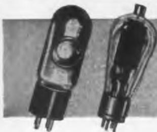
**The G-E phototube and G-E thyratron are the electronic tubes used in synchronizing the operation of this packaging machine.**
