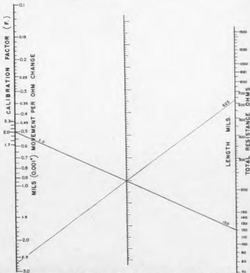
Fig. 3—Nomographic chart suitable for determining changes in length in gages of known characteristics corresponding to registered changes in resistance
