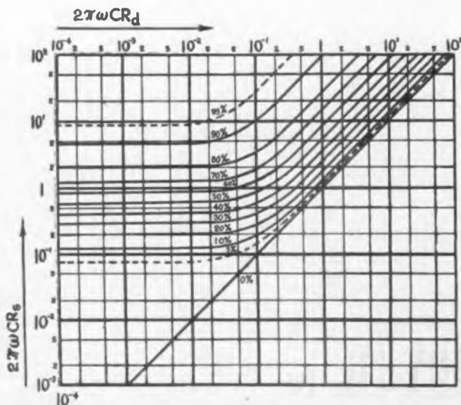
Average condenser output voltage  $e_o$  in percent of input voltage amplitude  $E_o$
