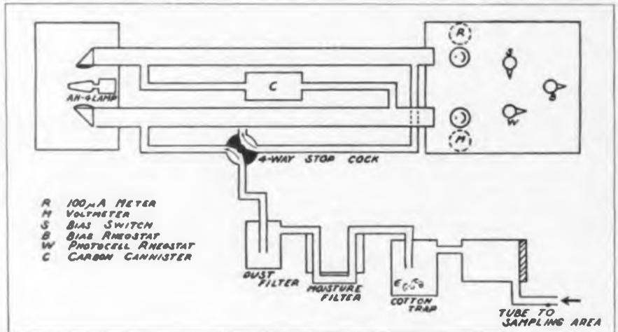
Diagram of gas analyzer. Air to be checked passes through one tube, then through carbon filter C. If gas is present, it is absorbed. Pure air then passes to second tube to upset balanced phototubes' response
