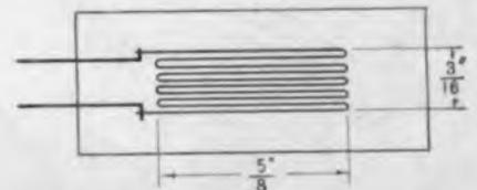
Fig. 2—Terminal heads connected to an accurately laid out grid of selected alloy wire, about 0.001 in. diameter
