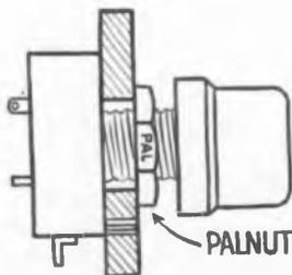
A Self-Locking PALNUT replaced heavier, more expensive jam nut and lockwasher on this volume control, saving weight and cost.
