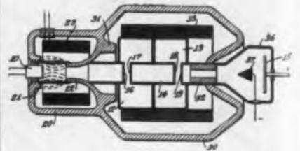
high intensity magnetic field converging in the direction of electron travel. This field is produced by electromagnets 20 and 30 having pole pieces, 21, 22 and 31, 32; 23 and 33 are the windings of these electromagnets. C. V. Litton, International Standard Electric Corp., (F) Dec. 22, 1942, (I) Nov. 2, 1943, Re. 22,389.
