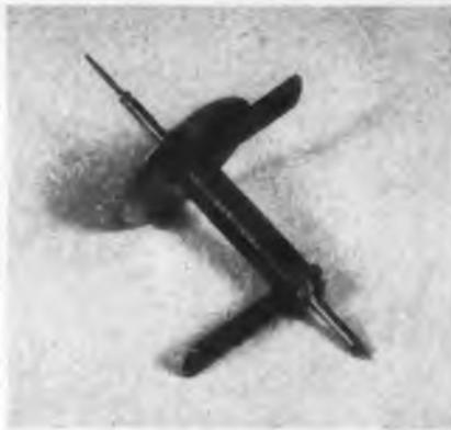
Rotor of the Circutrol is extremely light, almost inertialess
