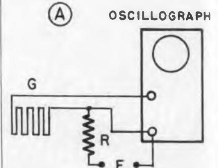
Fig. 4a—Method used to connect a strain gage to an oscillograph
