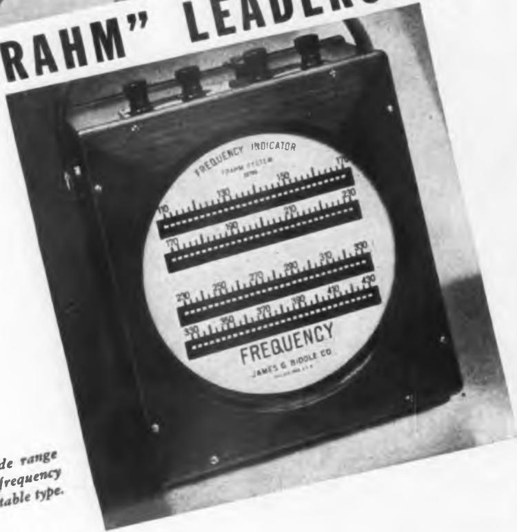
One job we were recently asked to perform was a tough one; namely, to design and build a special wide range portable frequency meter that would indicate from 110 to 430 cycles per second. Furthermore, it was required that simultaneous readings be obtainable at 2 or more points on the scale. . . . The instrument shown above is the successful answer to this unusual problem.
