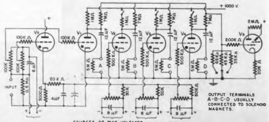
SOURCES OF BIAS VOLTAGES.  $10^{-4}$  to  $10^{-1}$  sec. time delay switch (K=kilo, M=meg.)
