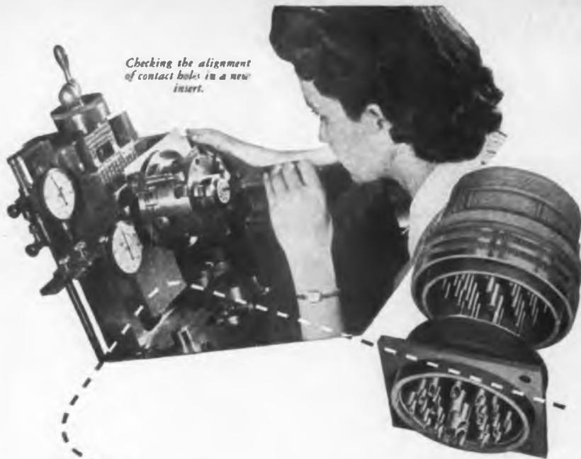
Checking the alignment of contact holes in a new insert.
