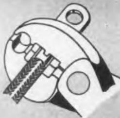
The jaws of the indenting pliers are then closed around the connector barrel.
