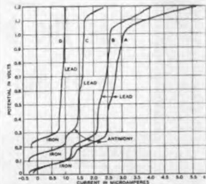
Fig. 4—Polarograms showing iron, antimony and lead content of the electrolyte of a commercial storage battery
