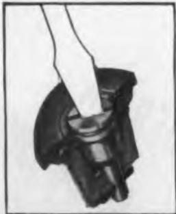
Camloc high speed fasteners operate with a quarter turn of the screwdriver. They secure doors and access panels in metal, plastic or plywood.
