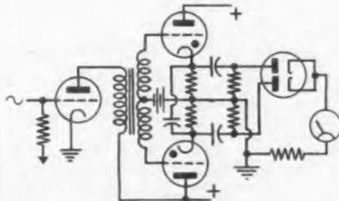
TYPICAL USES: Measuring frequency of signal generators, etc.; measurement and study of machine vibration; tachometer.
