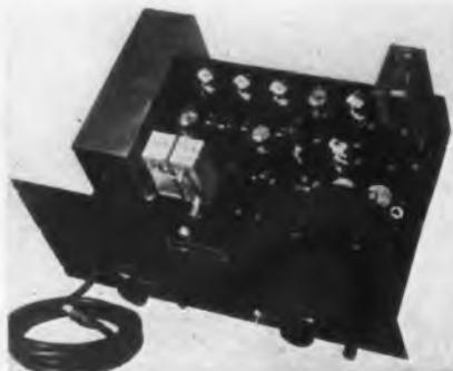
at ordinary indoor temperatures. Output voltage available is at least 30 volts for any frequency. Output impedance is 500,000 ohms maximum. The wave shape at all frequencies is sinusoidal and symmetrical within approximately 10 per cent. The unit is manufactured by American Time Products, Inc., 580 Fifth Ave., N.Y.C.
