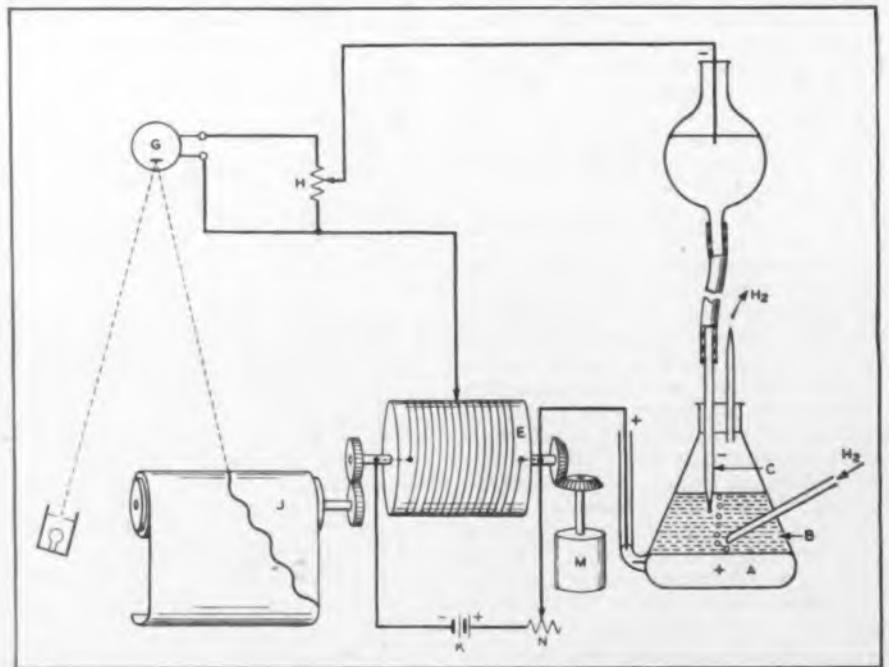
Fig. 1—Schematic of polarographic method of electrochemical analysis in which minute substances in solution are measured by a difference in potential as they are deposited on a dropping mercury electrode
