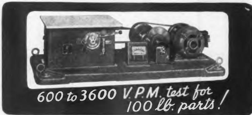
**E**LECTRONIC, aircraft and electrical parts and assemblies up to 100 lbs. in weight can be readily subjected to continuous or intermittent vibration fatigue test—the test that answers many questions about engineering, design and construction materials—on the Model 100A All American Vibration Fatigue Testing Machine.
