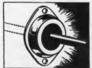
bulkhead. The device consists of an oil-resisting synthetic rubber disk with a radially extending slit and a cadmium plated steel retaining cup. They are made in several stock sizes from ¼th to 1½th in. hole diameter, and can be supplied to hold multiple lines.
