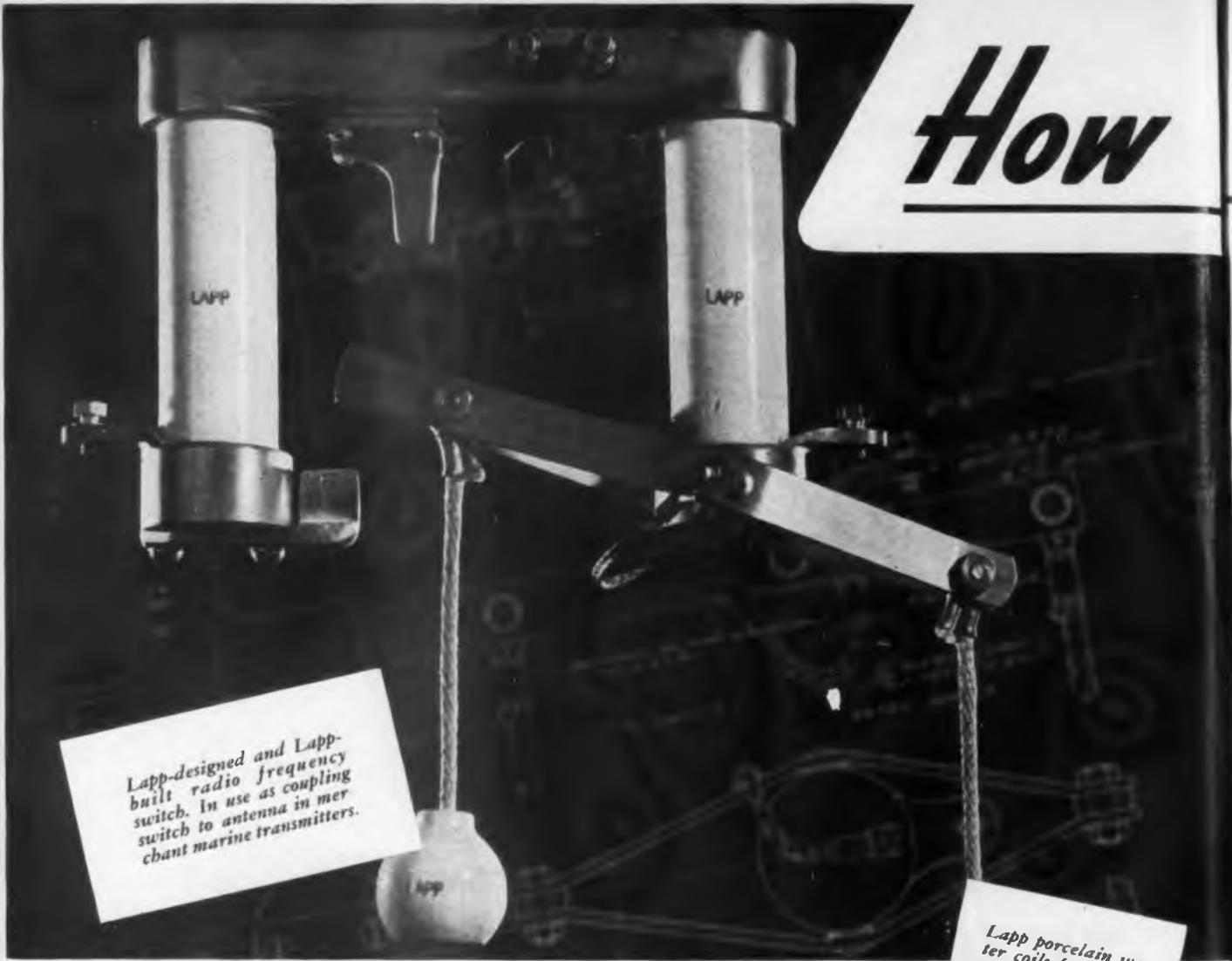
Lapp-designed and Lapp-built radio frequency switch. In use as coupling switch to antenna in merchant marine transmitters.
