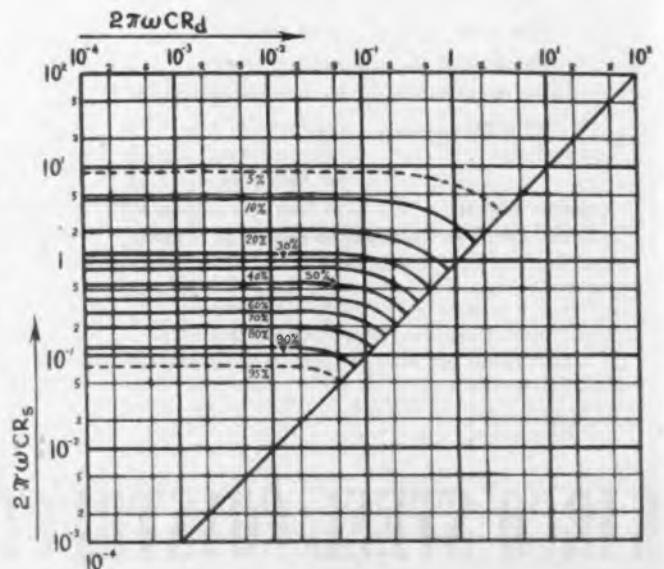
Peak ripple voltage  $\Delta e_o$  in percent of input voltage amplitude  $E_o$
