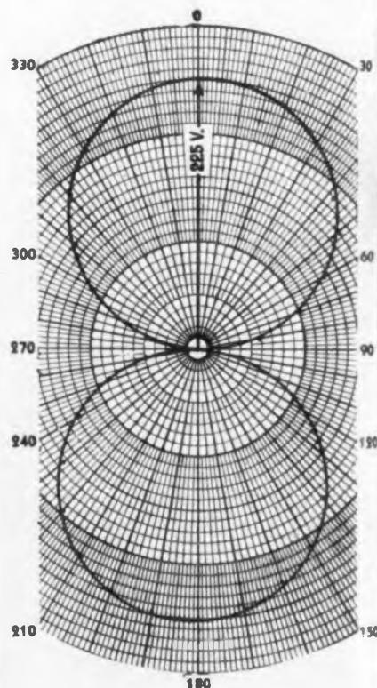
Fig. 4—Secondary voltage pattern of a Circutrol (782-02) for various positions of the shaft
