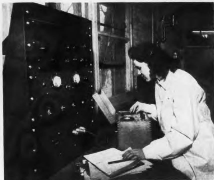
*Calibration of a Lavoie Precision Frequency Meter using a Crystal Calibrator developed in our Engineering Laboratory*
