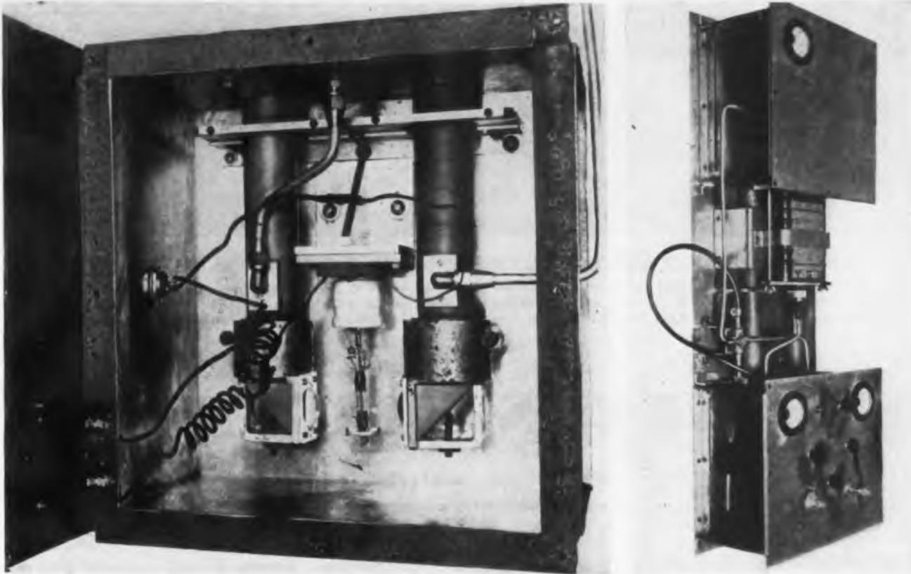
Left: Interior of light-source chamber, showing ultra-violet lamp with outer glass envelope removed; condensing lenses, and prisms. Right: Close-up of the analyzer. Chamber at top holds ultra-violet generator and quartz condensing lenses and prisms. Two large gas tubes connect to analyzing chamber, at bottom containing balanced phototubes and amplifier
