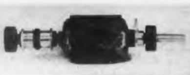
Rotor used in rotatable transformer and phase shift Circuitrol
