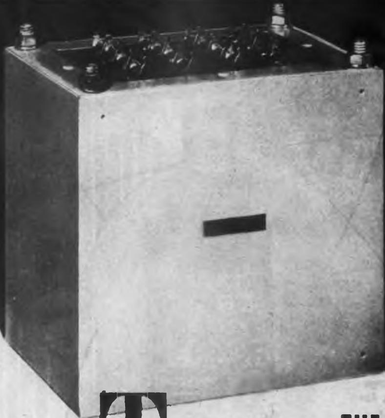
Illustrated at left, Type 300-A Output Transformer. Width  $4\frac{1}{4}$ ", length 6", height  $5\frac{1}{2}$ ". Utilizes Hypersil core in conjunction with Harvel 612-C Impregnation process. Mounting facilities  $\frac{1}{4}$ "-20 x  $\frac{1}{2}$ " studs on  $3\frac{1}{2}$ " x  $5\frac{1}{4}$ " centers. Weight 16 lbs.
