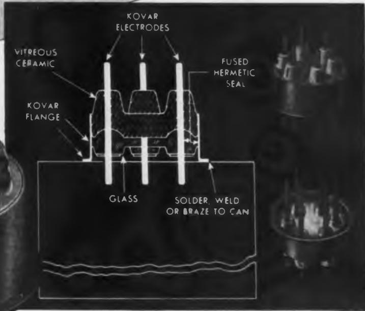
**H**ERMETIC transformer or capacitor seals of Kovar and glass may be made in a wide size range and with single or multiple electrodes. Electrodes may be solid or tubular.
