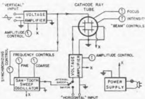
TYPICAL USES: Analyze oscillator, amplifier, and special purpose circuits; study many phenomena too rapid or too complex for other methods.
