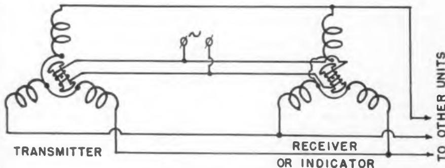
Fig. 1—In their commoner uses, rotors of all units in a group are excited from the same single phase source of ac
