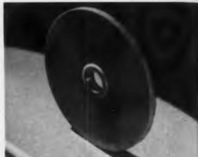
and paper base Synthane are combined. The paper base has usually better electrical properties while the fabric base furnishes added strength where the stress is greatest.
