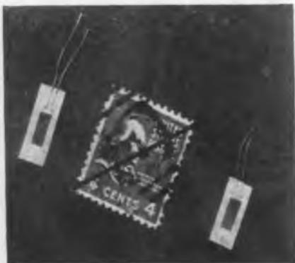
Fig. 1—Typical size of strain gages (not the smallest in use however) which are cemented flat against object being tested
