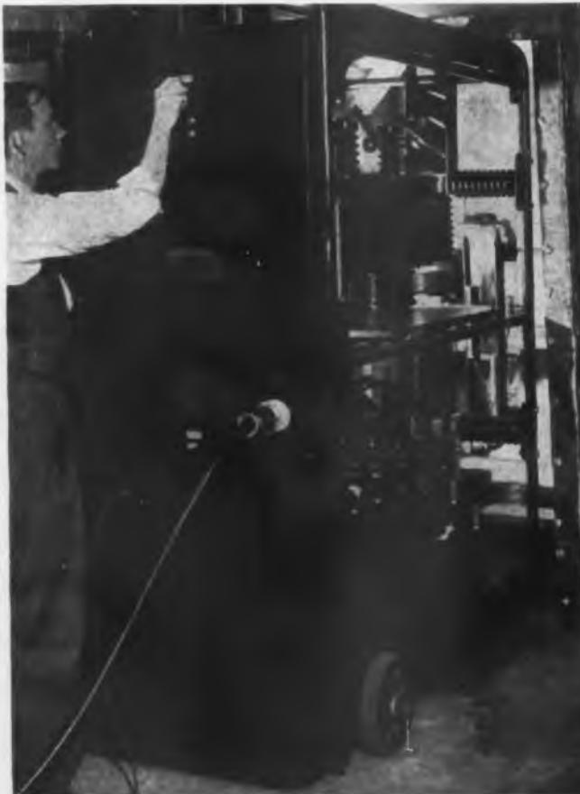
High-frequency dielectric heating equipment in use to sterilize packaged pancake flour
