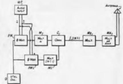
by the integer L. The output of mixing tube C then contains the original carrier, i.e., the difference frequency of its inputs, having a phase deviation equal to the combined retarded and advanced phase deviations of modulators PM and PM1, i.e., equal to  $2N \pm 1$  times the original phase deviations. This output component is multiplied, amplified and transmitted by the antenna. H. E. Goldstine, RCA, (F) June 10, 1942, (I) Dec. 7, 1943, No. 2,335,934.
