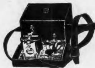
Main line telegraph combination set as supplied to the Signal Corps in 1898
