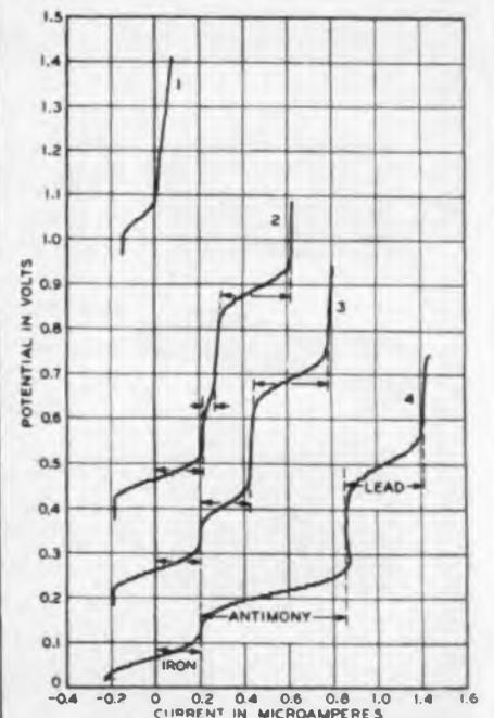
Fig. 3—Changes in current, as the potential applied to the electrodes increases, are recorded. To avoid superimposition of curves the vertical scale indicates voltage differences so that curves start at different points
