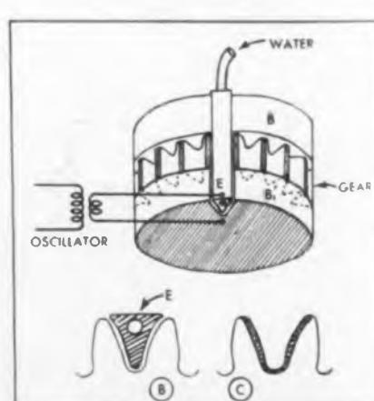
Fig. 15—Surface hardening gear teeth
