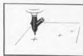
ON A VERTICAL MILL—locating and centering height gauge or size block layouts. Permits jig borer accuracy on more machines.
