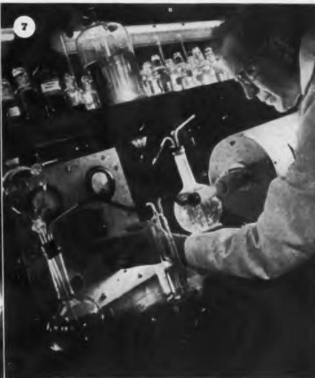
5. Set-up in the Kollsman electrical laboratory to test small drag cup motors. Operator measures inductance and the "Q" of the unit with a bridge
