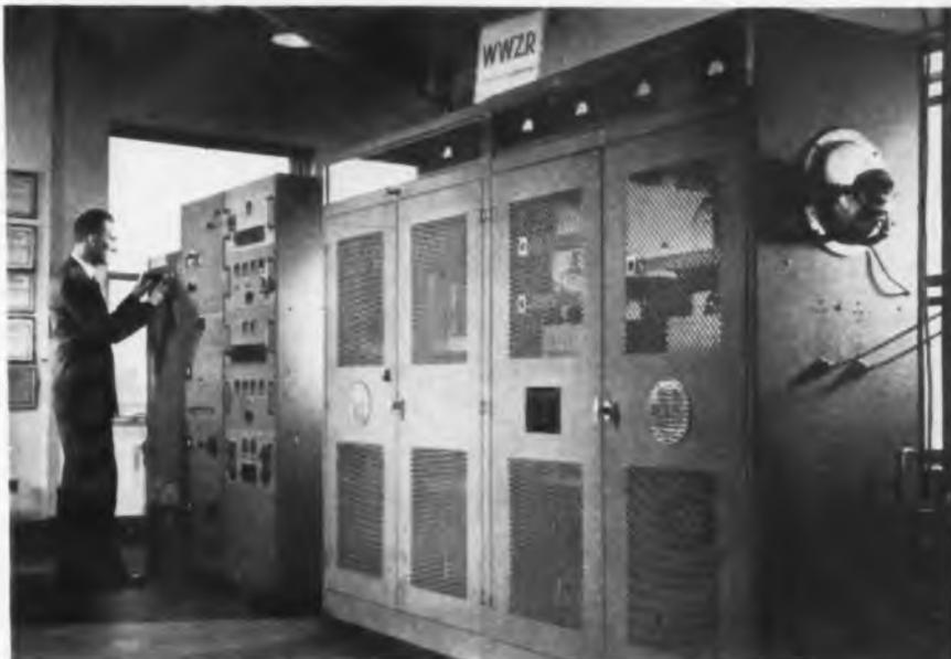
Modulation equipment and 1 to 5 kw rf amplifier stages of FM Station WWZR
