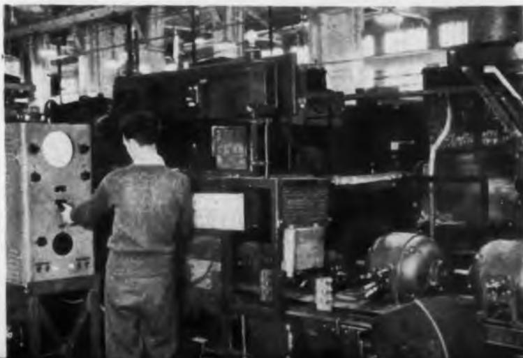
6. Top left: DC welder powered by storage batteries solves power line shock problem. Developed by Progressive Welder Company
