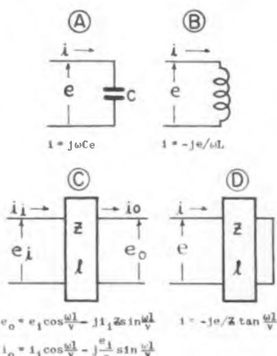
Fig. 1—Basic filter components with lumped C and L in (A) and (B). (C) is open line section, and (D) shorted line
