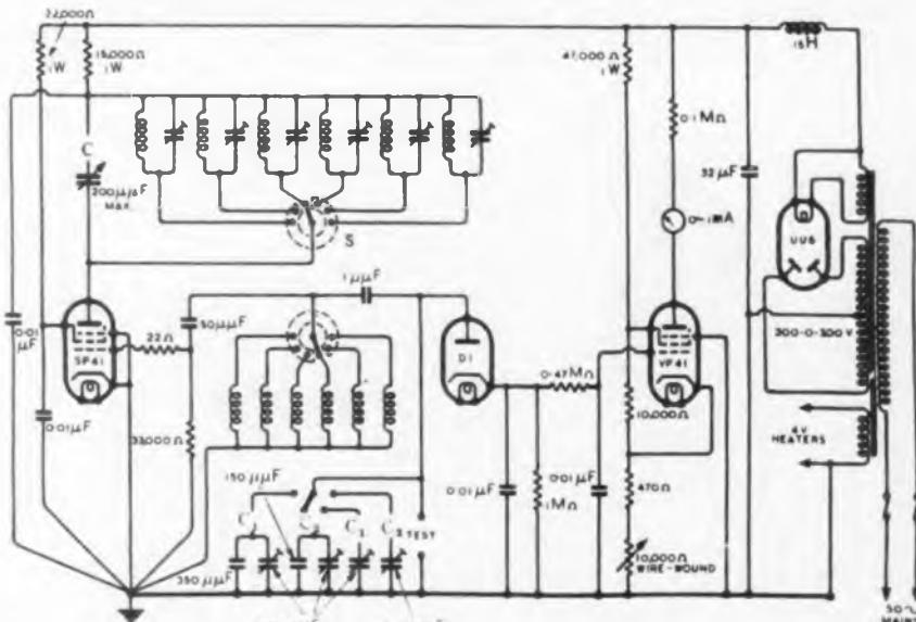
Scale connected to capacitor C in oscillator of inductance meter is so calibrated that unknown inductance is given by difference of two readings
