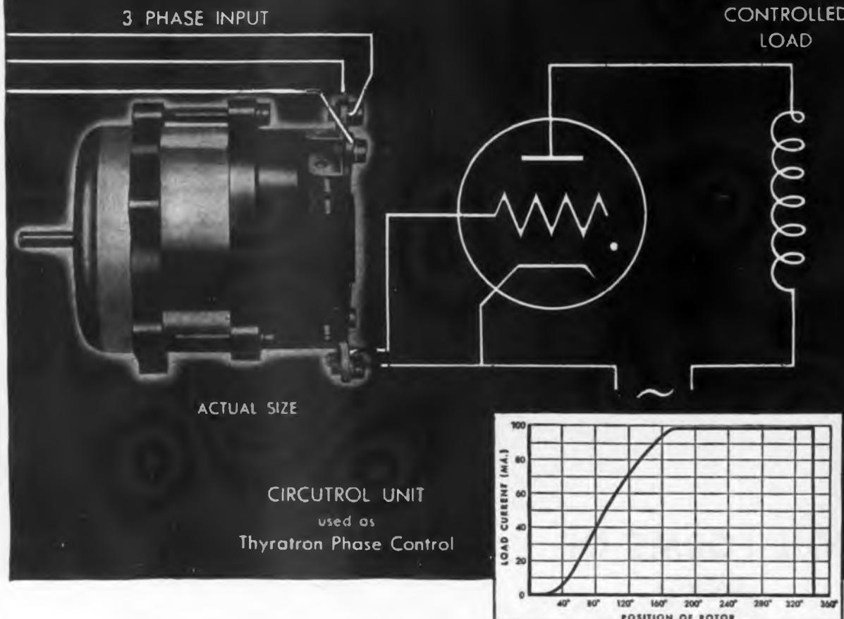
Typical of the many special applications for which design engineers have found the Kollsman Circutrol particularly suited, is phase control of Thyatron type units. In this application the unit offers accurate linear control, as shown by the above graph.
