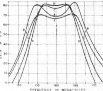
Fig. 12—Frequency response characteristics of amplifier of Fig. 11 showing effects of adjusting coupling impedance  $Z_L$  in Fig. 4. See text.
