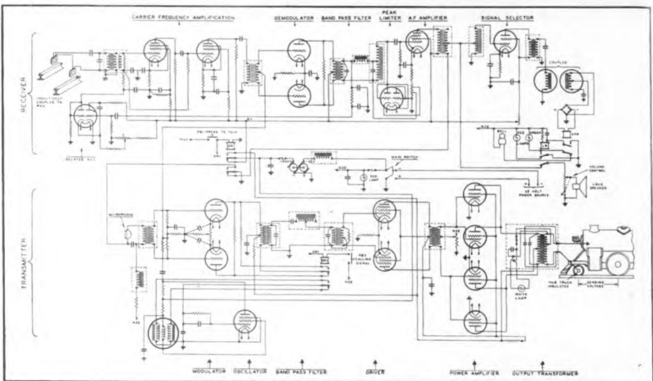
Fig. 2.—Complete circuit diagram of two-way carrier-telephone equipment for use on locomotive or caboose. "Signal Selector" (see text) provides closed circuit "proceed" signal. Way-station equipment similar except for power supply
