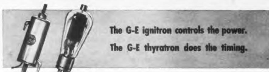
The G-E ignitron controls the power.
