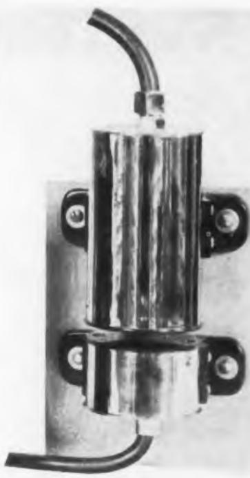
Fig. 3—Commercial thickness gage (G-E Co.) for metal foil measurements
