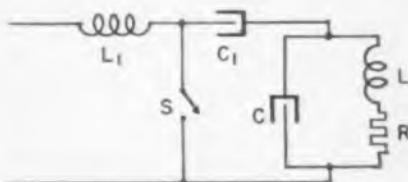
Fig. 3—Basic oscillating circuit with the function normally performed by a vacuum tube represented by the switch  $S$
