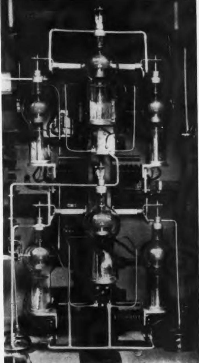
WE'RE a "have not" nation when it comes to tin. That's why a new plating method—developed by Westinghouse—makes big news! High frequency induction heating is the answer, and it not only fuses a uniform, corrosion-resisting tin coat on sheet steel five times faster than previous methods—it also uses only one-third as much tin!
