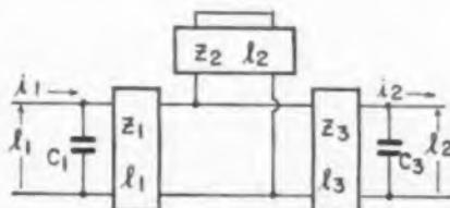
Fig. 4—Filter circuit using open lines at input and output coupled by section of shorted line
