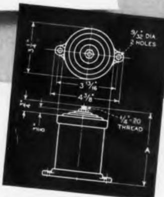
Type 1865 (no photo, but see drawing above) differs in the use of cast-aluminum case and steatite insulator to support terminal and withstand higher voltages. Dimension A is from 2 11/16 to 6 11/16".
