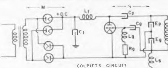
FIG. 8—Oscillator circuit with divided tank capacitor giving properly phased feedback voltages
