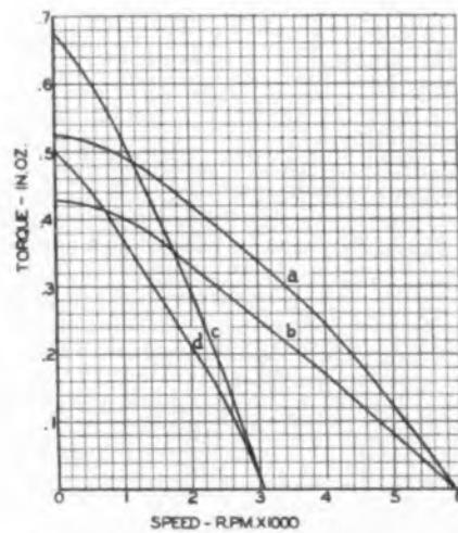
Fig. 2—Torque vs. speed relations for the type 776 drag cup motor. Curves a and c for 400 and 60 cycle copper cups, curves b and d for aluminum cups, at same frequencies
