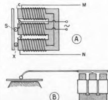
Fig. 2—Magnetic units used in production thickness-gaging applications
