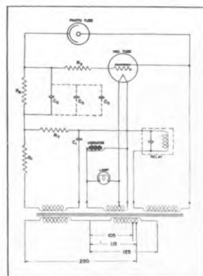
Fig. 4—Photoelectric control for automatic regulation
