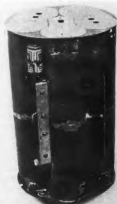
Fig. 11B—Side view of five stage amplifier. Each stage uses filter arrangement of Fig. 4 between tubes. Successive tubes are at alternate ends
