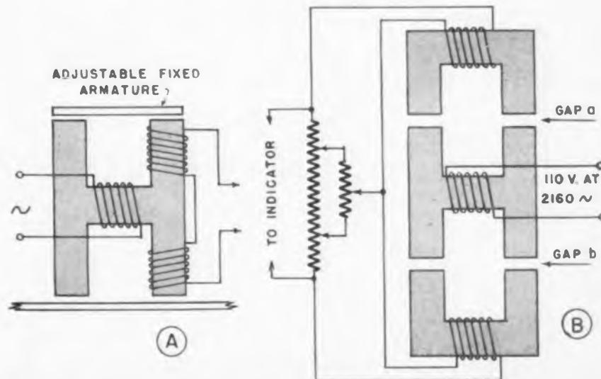
Fig. 4—Balanced-field type of thickness gages utilize changes in magnetic path, or else eddy current losses to alter a previously established null condition
