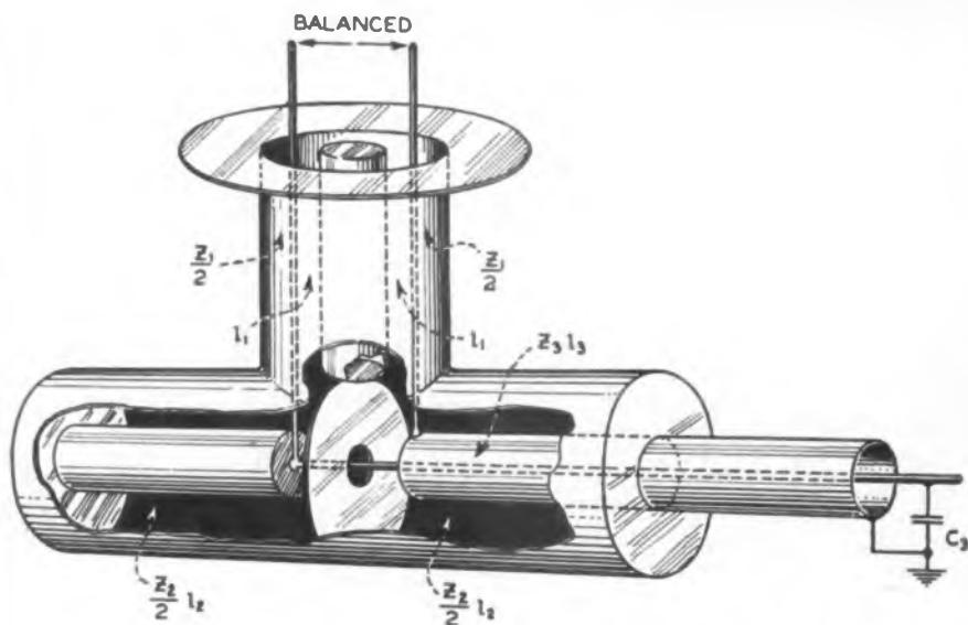
Fig. 6—Physical picture of coaxial line sections for filter in Fig. 5. Central spacing in illustration not in scale
