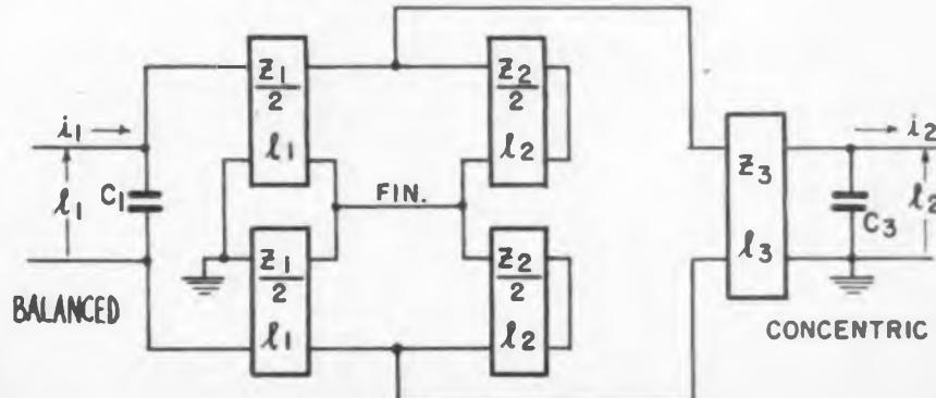
Fig. 5—Transmission line filter for conversion from balanced line to unbalanced concentric
