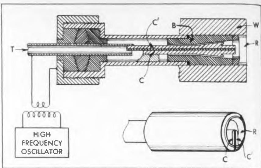
Fig. 11—Inside applicator for working in small bores
