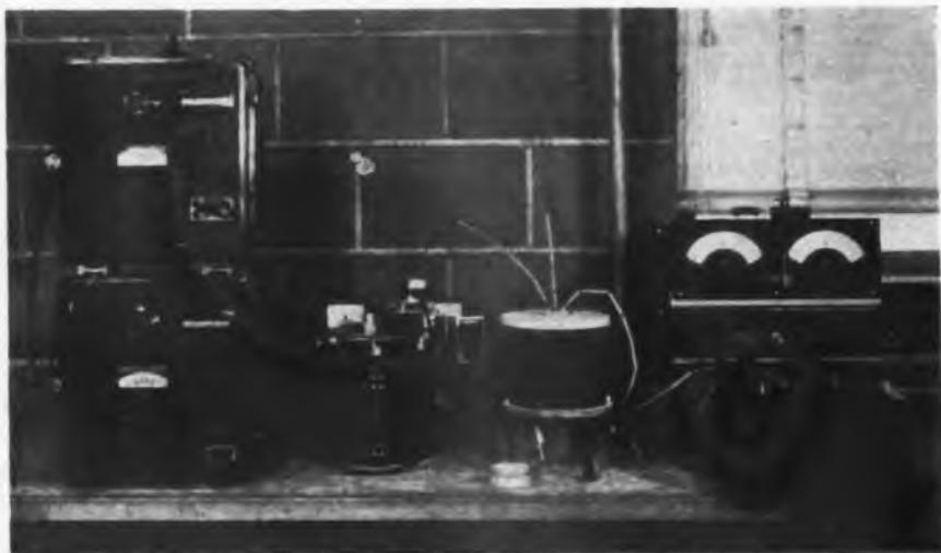
Fig. 2—Thermoanalysis apparatus, useful in determining temperatures at which chemical changes occur in metals and minerals
