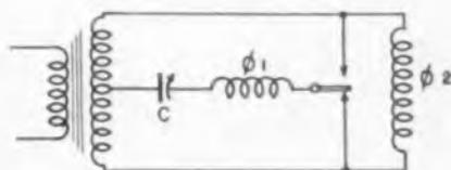
Fig. 6—Circuit with manual switch for speed reversal
