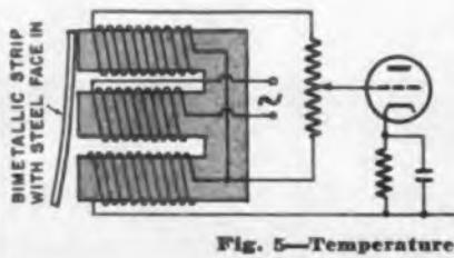
Fig. 5—Temperature-sensitive control unit
