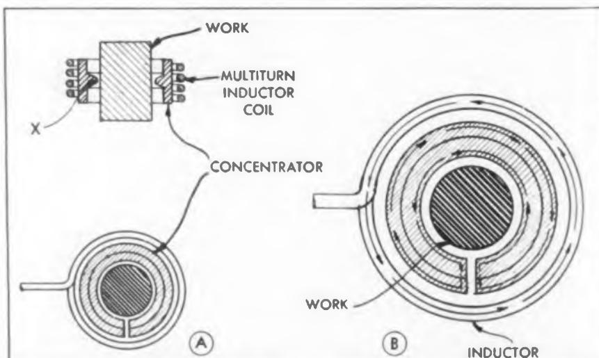
Fig. 13—Flux concentrators used to produce highly localized flux distribution
