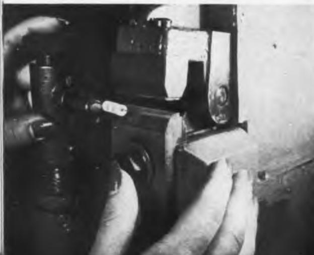
1. Above: Aligning jig for welding mount of 1.4-volt tube to base leads is a long arm pivoted at bench to swing tube into exact position between welder electrodes. Developed at Tung-Sol, Newark, N. J.
