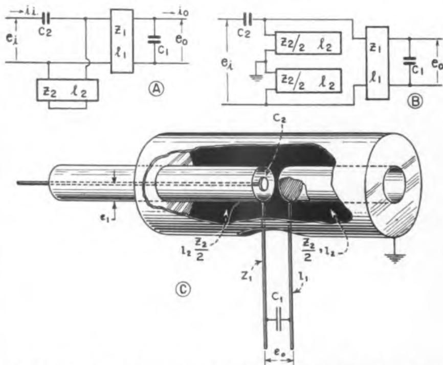
Fig. 7—Coaxial filter in block and physical forms for transition from low  $Z$  coaxial to high  $Z$  parallel lines. Spacing at center at  $C_2$  actually is smaller than shown
