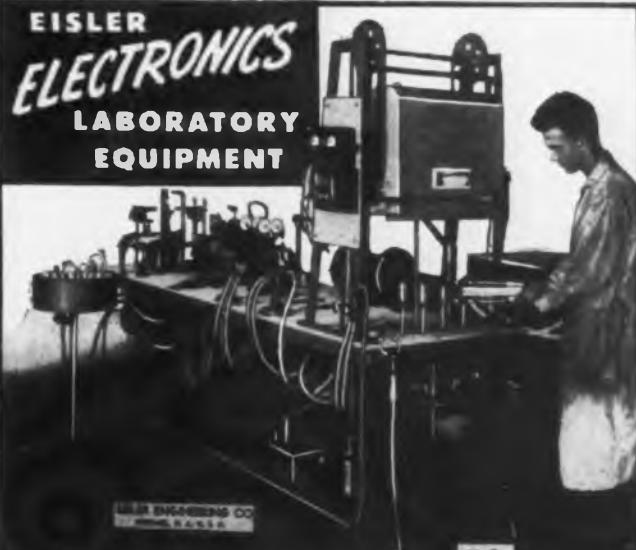
This electronic tube making unit fills the needs of schools, colleges, experimental and research laboratories for a compact machine complete in itself and capable of performing all operations required in the construction of incandescent lamps, radio tubes, electronic tubes and similar devices.
