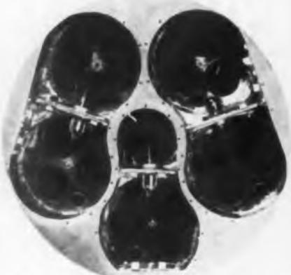
Fig. 11A—Top view of wide band amplifier using 954 acorn tubes shown through side walls of filter sections
