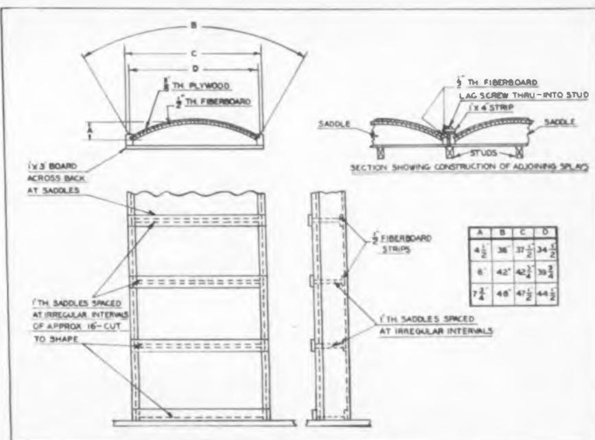
Fig. 1—This sketch shows the type of splay construction at present in use in the Walt Disney studios and also in the Paramount and Columbia stages
