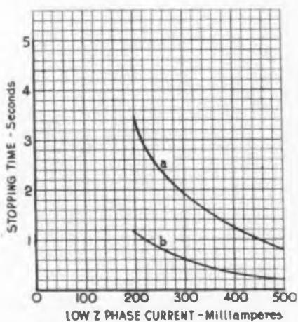
Fig. 4—Braking characteristics of an unloaded 400 cycle drag cup motor running at 6900 rpm. (a=copper, b=aluminum cup). Coasting time shown after opening the high impedance winding
