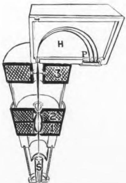
Diagrammatic cross-section showing inner construction of microanalyzer
