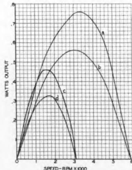
Fig. 3—Power output curves for same motor. The curves are for the same conditions listed in Fig. 2
