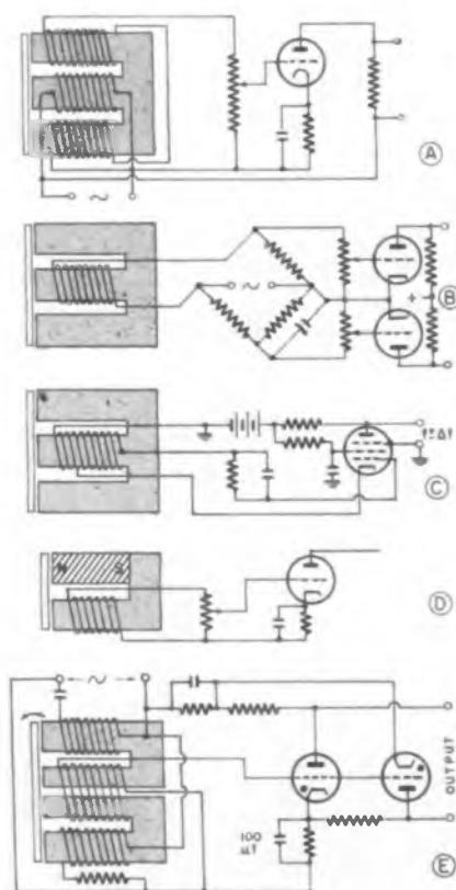
Fig. 1—Reluctance type units in five basic displacement measuring circuits
