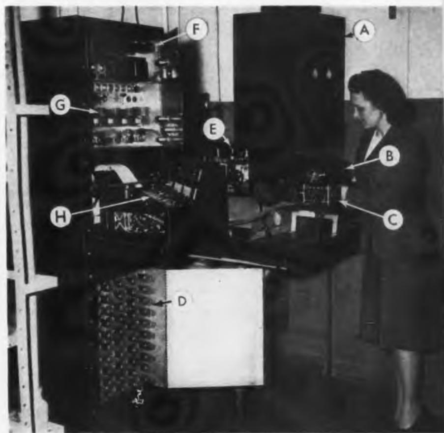
The Philco electronic recorder calibrating a Signal Corps frequency meter with completely automatic operation
