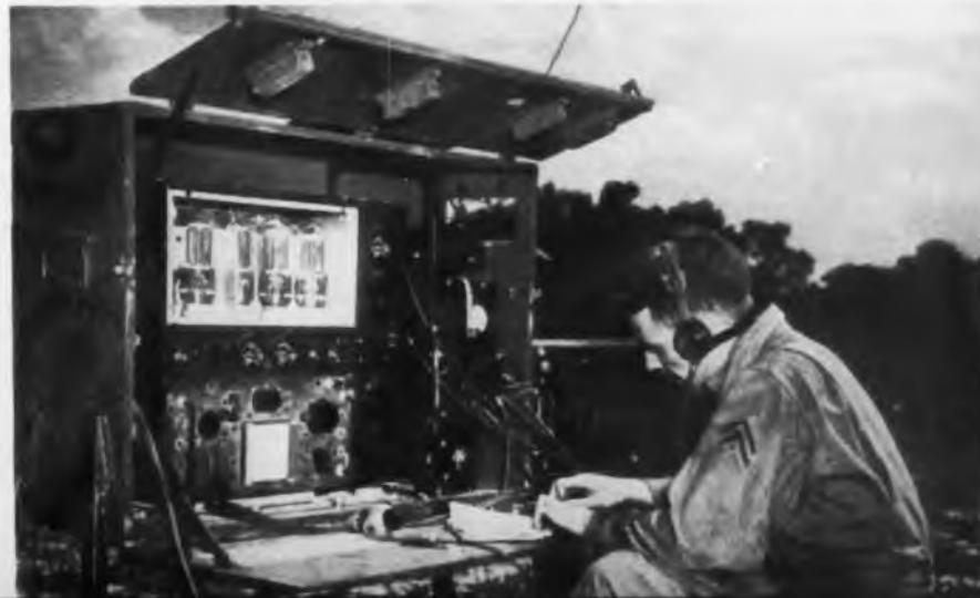
Upper—Part of the extensive radio equipment that is carried by AACCS ships. This particular installation shown the arrangement used in a Curtiss A-12
