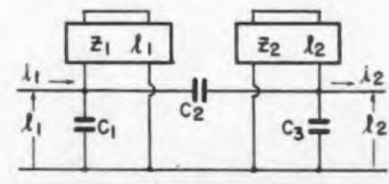
Fig. 3—PI filter using shorted line sections in shunt branches and C<sub>2</sub> for coupling
