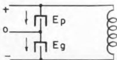
Fig. 6—Basic circuit of Colpitts oscillator
