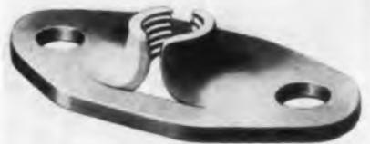
It is a light weight, one-piece integral unit with low installation torque that allows speedier insertion of screws and bolts. It is interchangeable with nut plate AN362, for high temperature applications in all structures. Retains its self-locking torque even after many removals.
