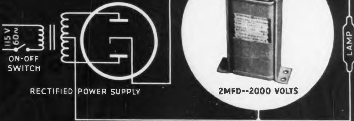
**IN THREE SECONDS** this small Pyranol capacitor accumulates enough energy to discharge 4,000,000 watts instantaneously, through a mercury lamp. This produces a four-microsecond flash which, at its peak, is one-fifth as bright as the sun's surface.
