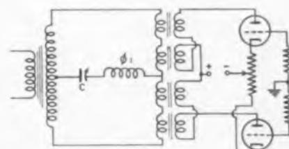
Fig. 7—Electronic circuit using saturating reactors to provide control of speed and direction. Second phase winding is connected across primary or secondary of transformer
