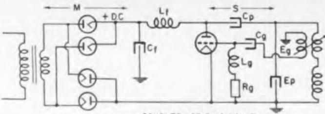
FIG. 7—Oscillator circuit with coupled grid coil for feedback purposes
