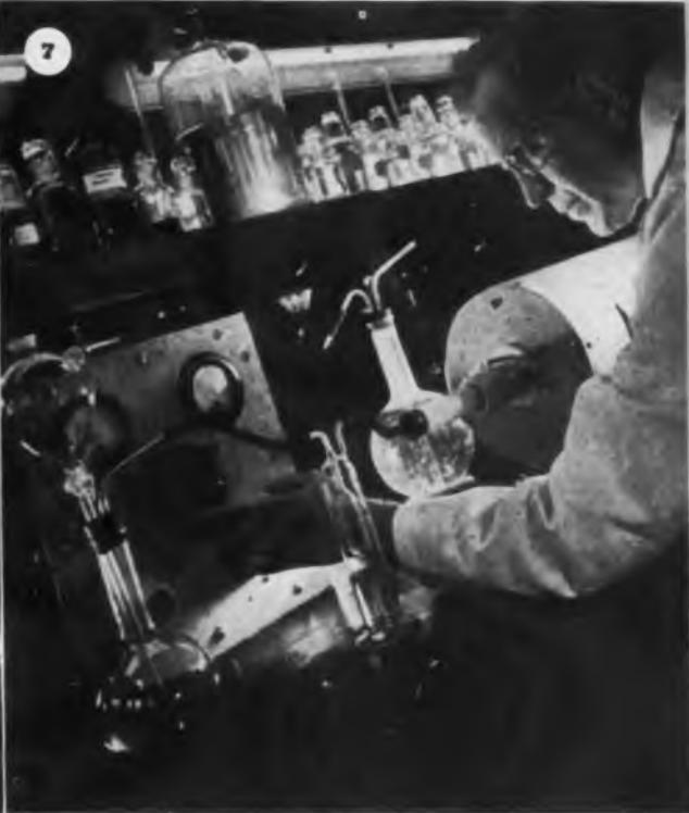
5. Set-up in the Kollsman electrical laboratory to test small drag cup motors. Operator measures inductance and the "Q" of the unit with a bridge
