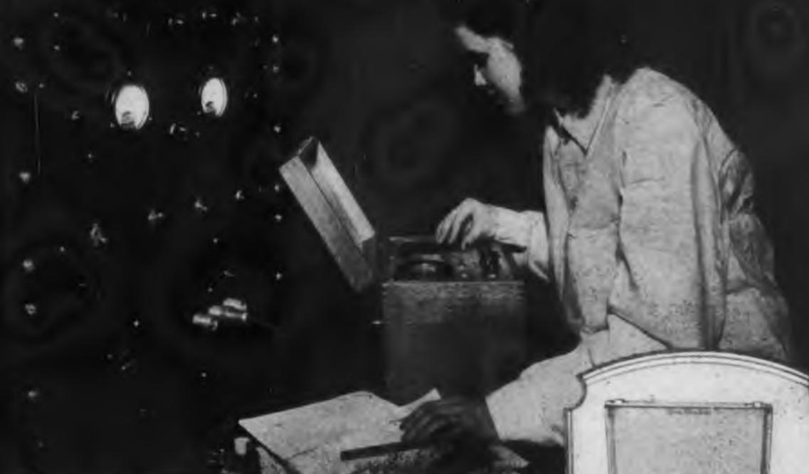
*Calibration of a Lavoie Precision Frequency Meter,
