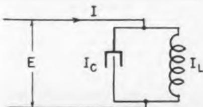
Fig. 1—Basic oscillating circuit
