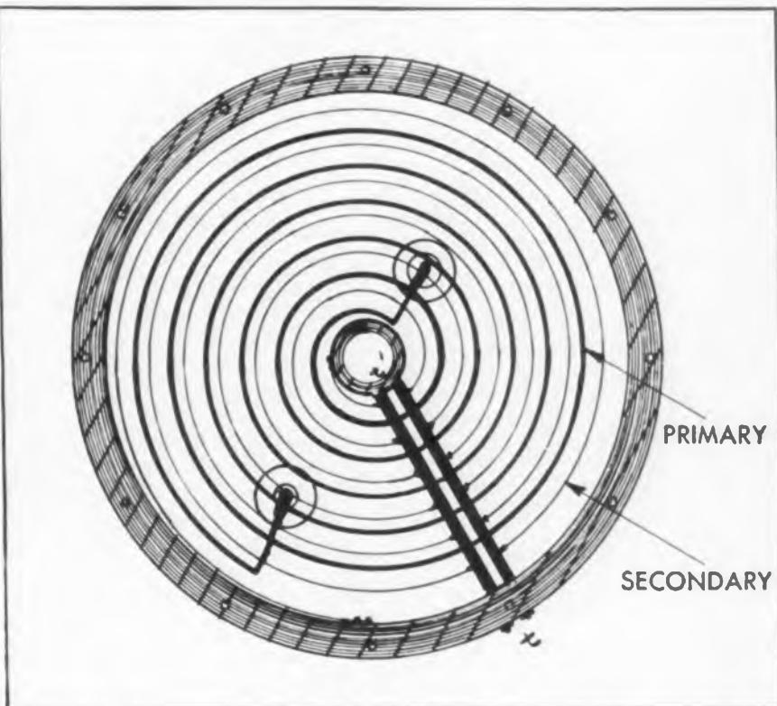
Fig. 2—Spiral type. Paralleled secondary loops interleave primary
