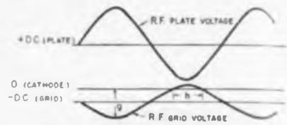
Fig. 5—Relation between anode and grid voltages in oscillator
