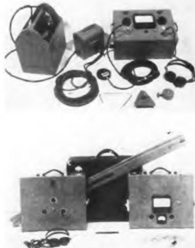
Above: Lead detector hears hiss of escaping water. Below: Transmitter-receiver type equipment for finding buried pipes and cables
