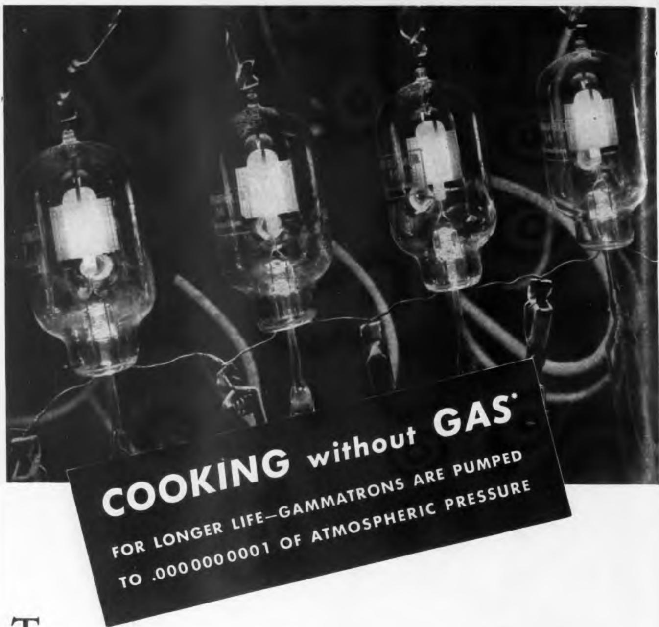
These Gammatron tubes are being submitted to an exhaust process so severe that only tubes made with tantalum elements can withstand it. They are "cooking" at 3,000° F, running at this temperature from 30 to 40 minutes. At the same time they are being pumped to create a vacuum equal to one ten-billionth of atmospheric pressure...the best commercial vacuum obtainable.
