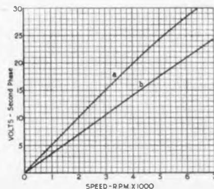
Fig. 5—Quadrature voltage and speed relations in drag cup motors when one phase is energized at 115 v. 60 cycles. a refers to a copper cup, b to aluminum
