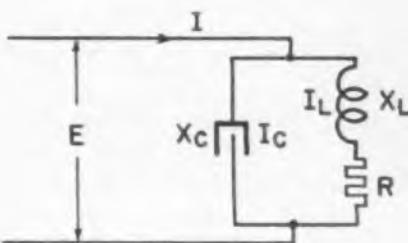
Fig. 2—Oscillating circuit with resistance
