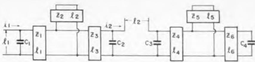
Fig. 9—Complex pass-band filter with good response characteristics for resistive load at output terminals  $l_1$ .
