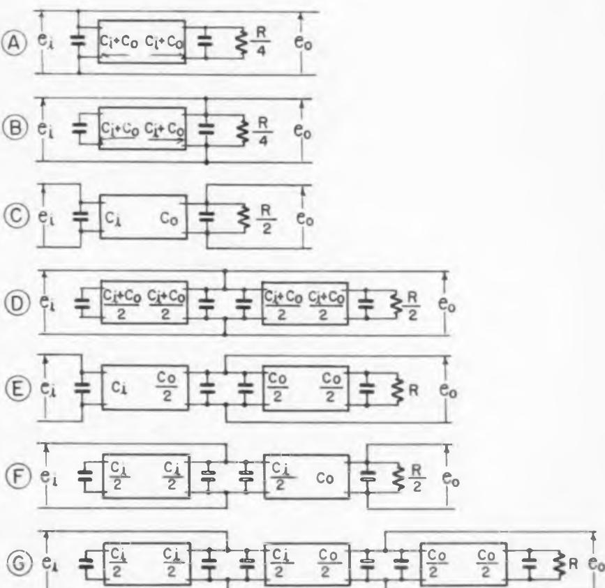
Fig. 10—Progressive filter arrangements, from simple at A to complex at G, for variety of circuit and load conditions
