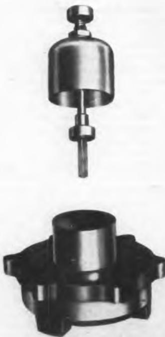
Fig. 1—The rotor and magnetic circuit of a drag cup motor
