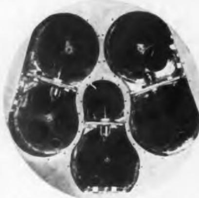
Fig. 11A—Top view of wide band amplifier using 954 acorn tubes shown through side walls of filter sections
