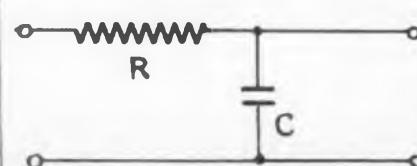
Fig. 6—Electrical Integrating network
