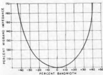
Fig. 8—Filter impedance variation over band pass for two shunt terminating elements
