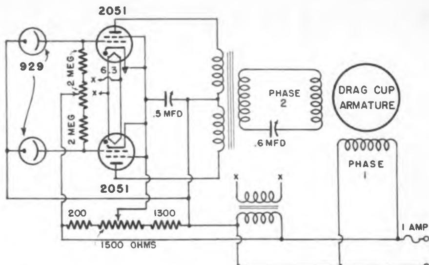
Fig. 8. Shifting the motor speed and direction, by photocells provides a versatile arrangement for the automatic control of numerous industrial processes
