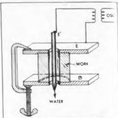
Fig. 14—Coaxial method of heating small bores
