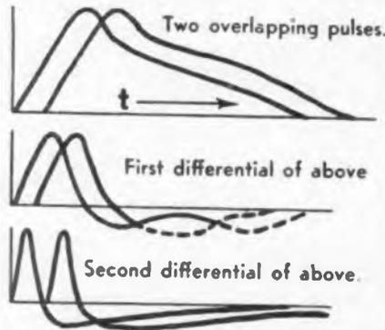
Fig. 8—Effect of multiple differentiator on overlapping pulses. Permits separation for control purposes
