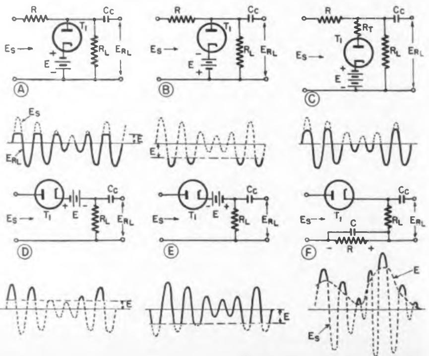
tube will conduct only when the positive swing of the incoming signal exceeds the negative voltage. Thus it is possible to control the threshold of action over wide limits.
