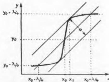
Fig. 2—Dependence of position of potential minimum ( $y$ ) on position short of ( $x$ )
