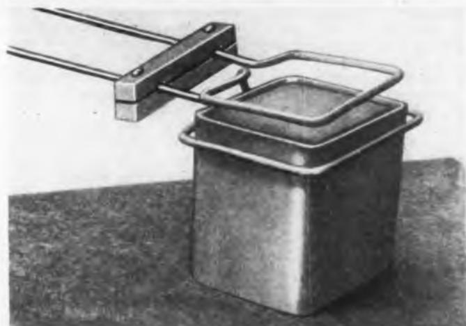
**SOFT SOLDERING LIDS TO CANS.** (Center). Rectangular tin transformer cans and lids;  $2\frac{1}{8}$  in. x  $2\frac{1}{4}$  in. Test set-up: Induction heating 2-turn coil  $\frac{3}{8}$  in. apart. Time: 7 seconds. Power input: 1640 watts. Results: Satisfactory; lids were soldered to cans smoothly and evenly.
