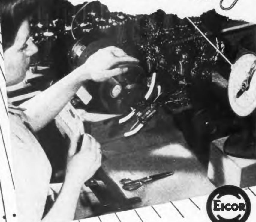
**This armature**, when completed, is destined for an important mission. It is being wound for one of hundreds of Eicor dynamotor designs—and may be used in one of scores of varied applications. *One factor alone remains constant—the requirement for complete reliability.*
