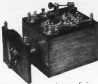
*Crystal wireless receiver as built for the Signal Corps in 1917*
