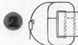
Core parts are butted together. Strap is threaded through seal and . . .
