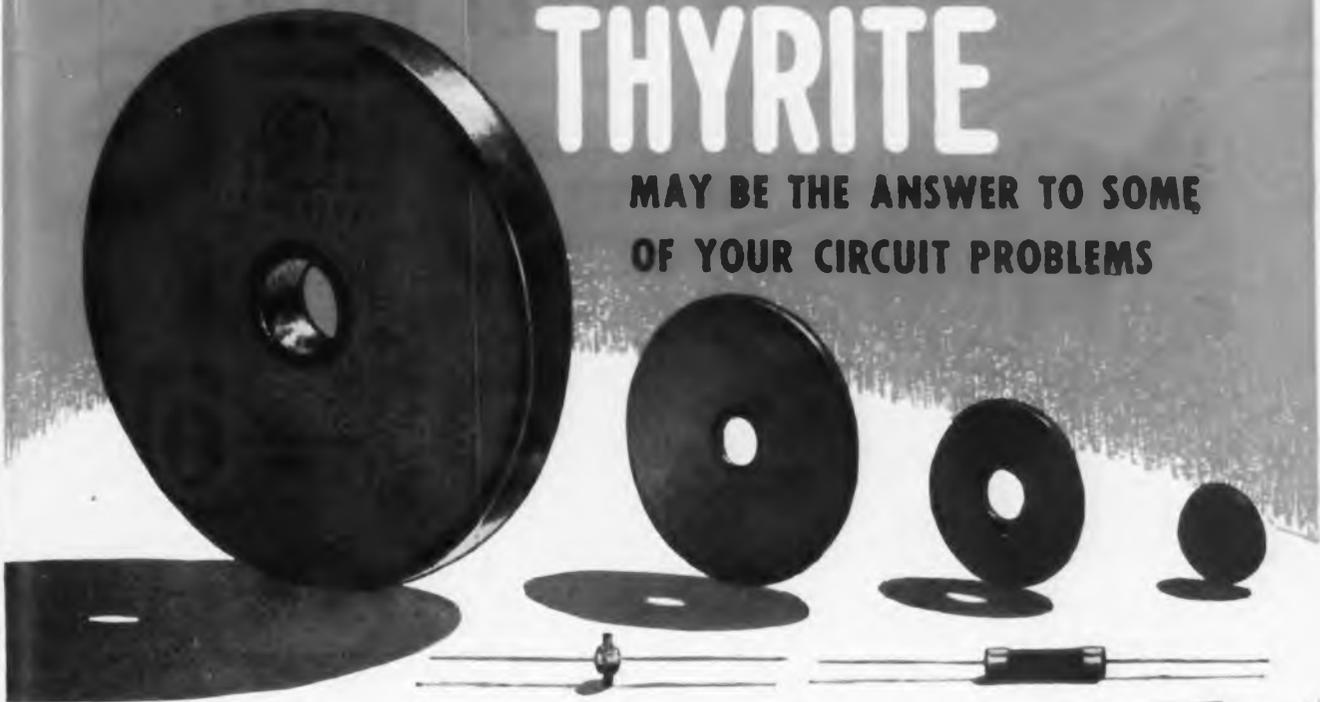
**THYRITE\*** is a silicon-carbide ceramic material, dense and mechanically strong, having nonlinear resistance characteristics—the resistance varying as a power of the applied voltage. Its resistance characteristic is stable, and substantially independent of polarity or frequency. Thyrite has been used for many years in many important applications, including electronic. Thyrite can be produced in various shapes and sizes (those which can be successfully molded).
