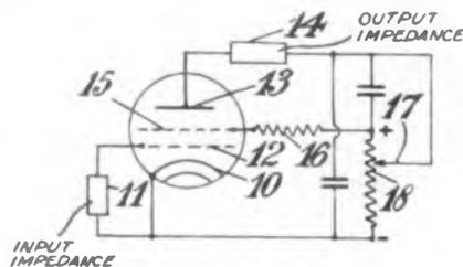
that it acts as by-pass for dc and no-signal-frequency space currents. Application to electron multipliers, amplifiers, and superheterodyne receivers is illustrated and described. F. J. G. van den Bosch, Vacuum-Science Products Limited, (F) June 16, 1941, (I) Feb. 29, 1944, No. 2,342,986.
