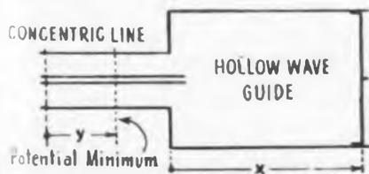
Fig. 4—Arrangement for measuring transfer characteristics at transition from concentric line to hollow wave guide
