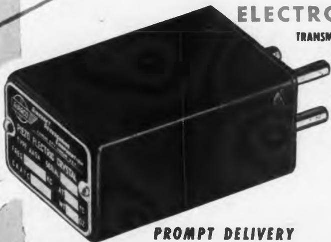
▶ Type AA9 Crystal, 2.5 parts/million temperature coefficient, accuracy of carrier frequency .01%. Made in three models—A, G and E, covering total fundamental frequency range of 200 to 10,000 kc. Internal adjustment screw permits small amount of frequency control in the single crystal units, AA9A and AA9G.
