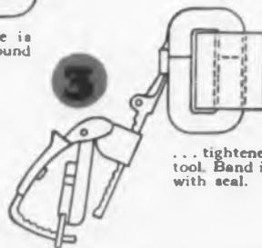
. . . tightened with banding tool. Band is locked in place with seal.
