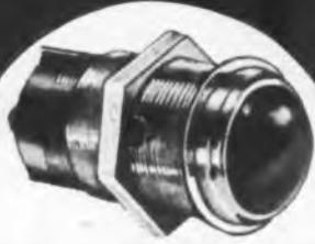
No. 600 . . . Molded Bakelite socket with special lamp gripping features, 6/32 terminal screws and 1/4" insulation barrier; high arched lens for side visibility; correct interior diameter to control lamp heat and to permit easy lamp removal without tools. Increased diameter flange for positive coverage of mounting hole; chromium plated; Underwriter: Approved for 120 V. (S6 type bulb). Patented 1931. (U.S. No. 185-8994).
