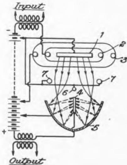
part of the anode 4, so that the secondary electrons go directly to the flat sides of the anode. The electron beams impinge on the inner surfaces of the secondary emission electrode 5 in such a way that substantially all secondary electrons pass directly to the anode without oscillating around or near it, and practically none of them return to the vicinity of the control grid 2. A. J. W. M. van Overbeek, Allen Property Custodian, (F) June 6, 1941, (I) Feb. 1, 1944, No. 2,340,631.
