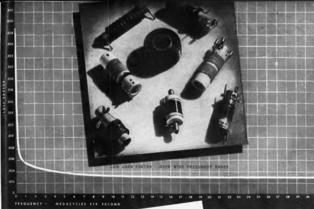
A typical group of H. F. radio coils insulated with Q-Max A-27 Lacquer
