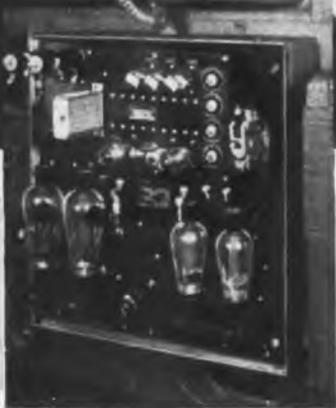
**The G-E thyatron tube is the "heart" of the G-E Thy-mo-trol unit which keeps the grinder going at uniform speed.**
