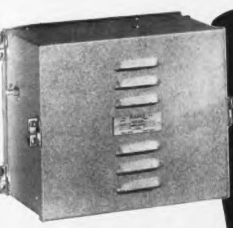
**1** The Kaar 11-X receiver is installed beneath the dash, and held securely by bolts through firewall.
