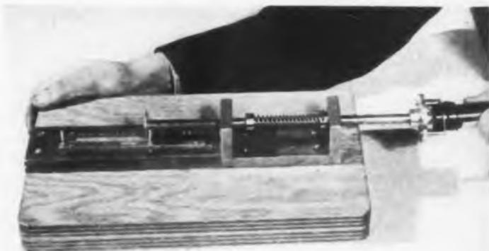
**ELECTRONIC TUBE CEMENT IMMERSION TESTER—(below).** This instrument measures in torque units, the force required to loosen or rupture the bond existing between the base and envelope of an electronic tube thereby providing a standard upon which a specification can be based
