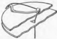
The TUNG-SOL Damper Bar construction is positioned to hold the filament tension spring to one side, thus taking the whip out of the filament above the mica disc. This whip would allow the filament to vibrate, the cause of low frequency pitch known as "howl".
