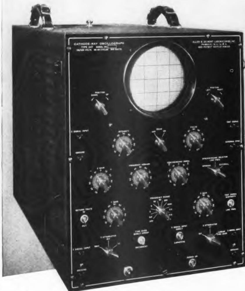
Uses new Army-Navy preferred Type 5CP1 cathode-ray tube with intensifier electrode operated at overall accelerating potential of 3000 v. High-intensity patterns. 5" dia. screen.
