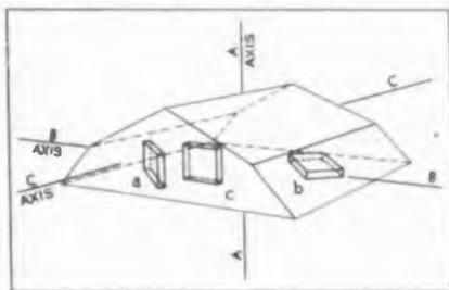
Fig. 2—Rochelle salt crystal exhibits greatest piezo-electric effect along axis 45 deg. from B and C perpendicular to A
