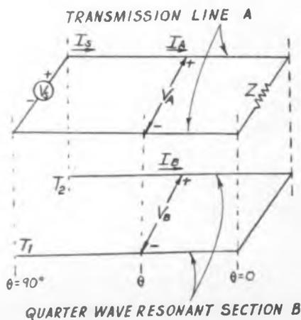
The coupled section blocks line A and power transfer at the frequency for which section B is a quarter wave length long is prevented.
