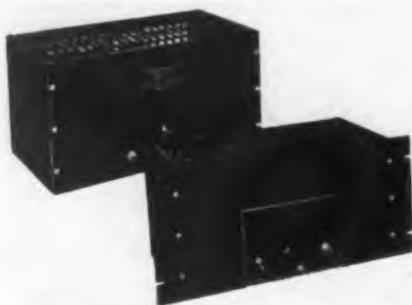
the sum of all ac components present in the output is less than 5 millivolts. The change in voltage output from no load to full load is less than one volt. The primary of the power transformer is tapped for use at 105 volts, 115 volts and 125 volts on a 50-60 cycle source. An unregulated heater supply winding of 6.3 volts at 5 amperes is furnished.
