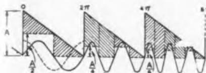
strip times the mean value of  $\sin n\omega t$  over the positive half cycles, i. e., it will be equal to  $2A_n$  and  $a_n$  will be equal to  $2A_n/\pi$ .
