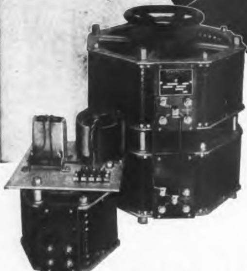
By simply turning a knob on the manually operated POWERSTAT Variable Voltage Transformer or by pushing the control button of the MOTOR-DRIVEN POWERSTAT the proper voltage is applied to infrared lamps to meet your heating requirements. The exact energy needed to process materials of varying thickness, color, or moisture content is conveniently and accurately obtained with POWERSTAT variable voltage control.
