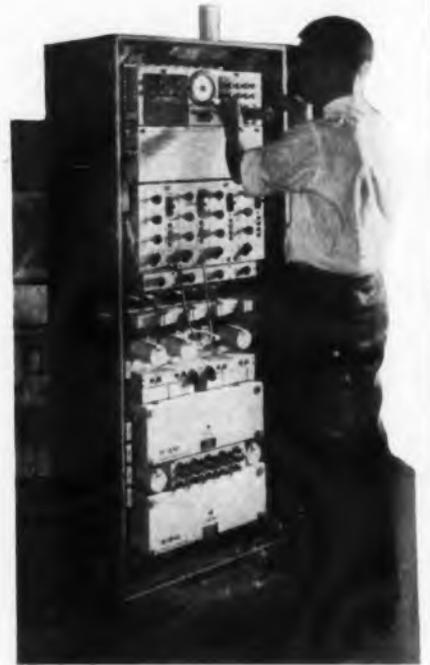
Carrier telegraph terminal unit for four duplex channels used on spiral-four system
