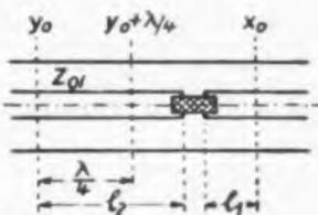
Fig. 5a—Concentric line with inner conductor partly replaced with ceramic piece
