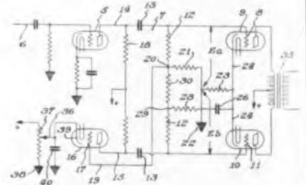
ingly there is less cancellation of the voltage on the inverter grid than in conventional circuits of the self-balancing type, and, for any given value of the gain of the inverter, the resistances 21, 30, 28 may assume values such that the voltages at the output grids 8 and 11 are substantially equal and 180 deg. out of phase under all conditions of operation. R. C. Sanford, RCA, (F) June 28, 1941, (I) Feb. 1, 1944, No. 2,340,617.
