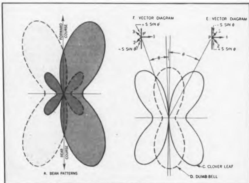
Fig. 2—Radiation pattern for localizer beam at left is composite of two patterns at right (Fig. 4). Course sharpness is 1.2 db per 1.5 deg. off-course. On-course signal approximately 2.75 db below maximum at 25 deg. off-course
