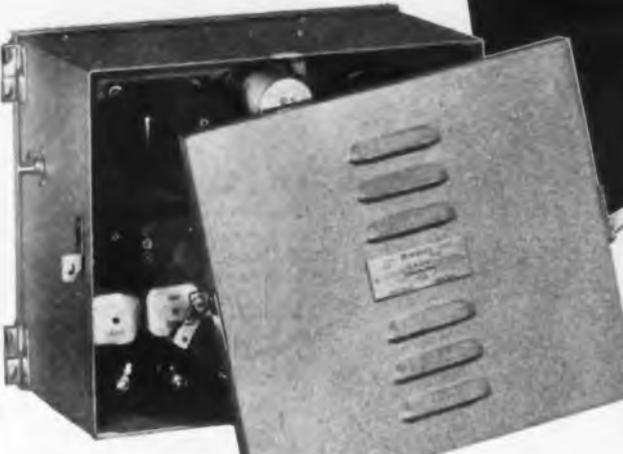
**2** For simple servicing, such as the replacement of tubes, the dust cover is removed by releasing two convenient snap catches. Takes but a moment.
