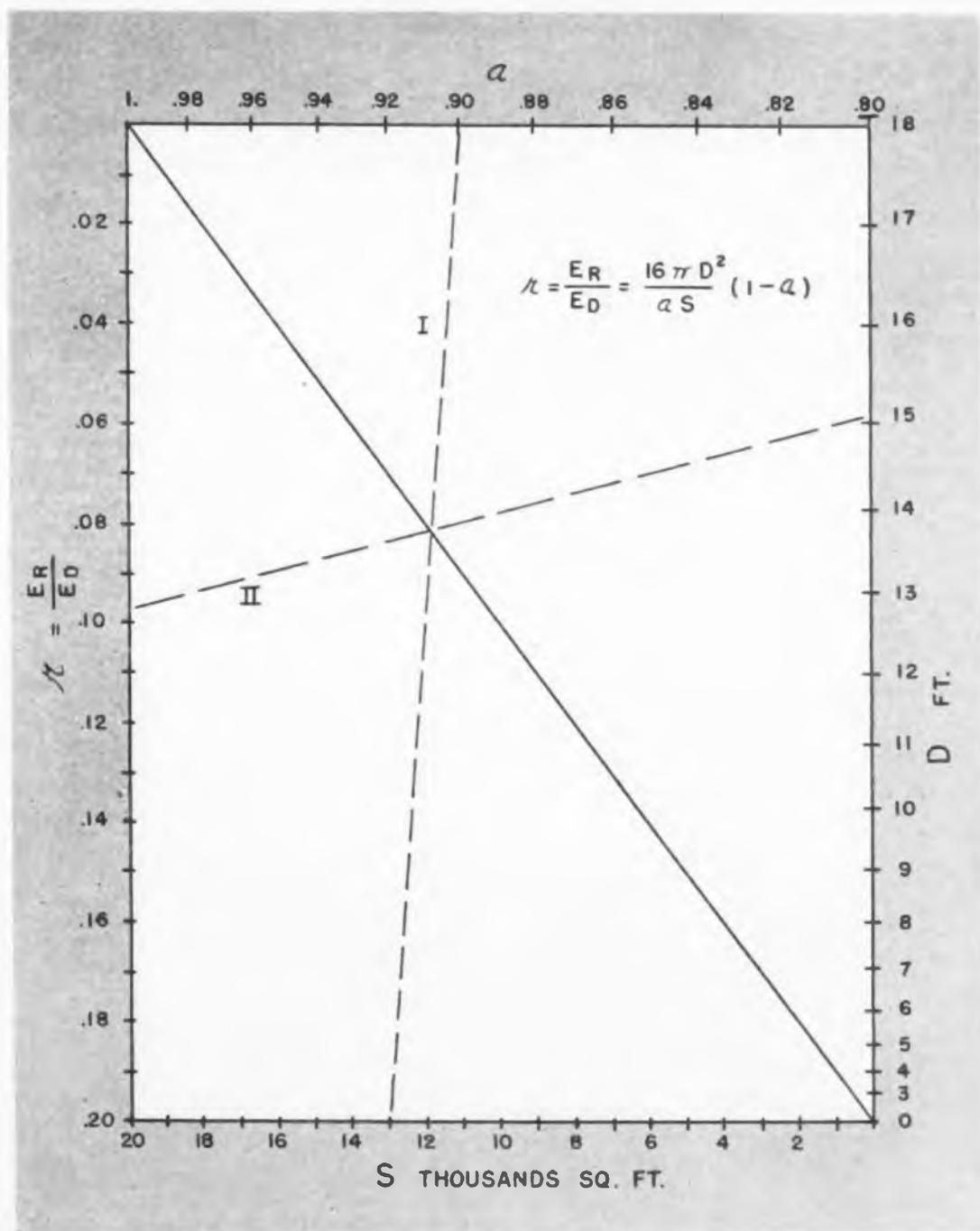
A formula for the ratio ( $r$ ) of the energy density  $E_R$  of reflected sound to  $E_D$ , that of the direct sound appears on the nomogram above.
