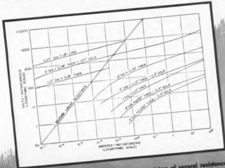
Typical volt-ampere characteristics of Thyrite resistors of several resistance levels and power ratings. Note that the nonlinear voltage-current characteristic extends over an extremely wide current range. Compare it with the characteristic (orange line) of a 1-megohm linear resistor.
