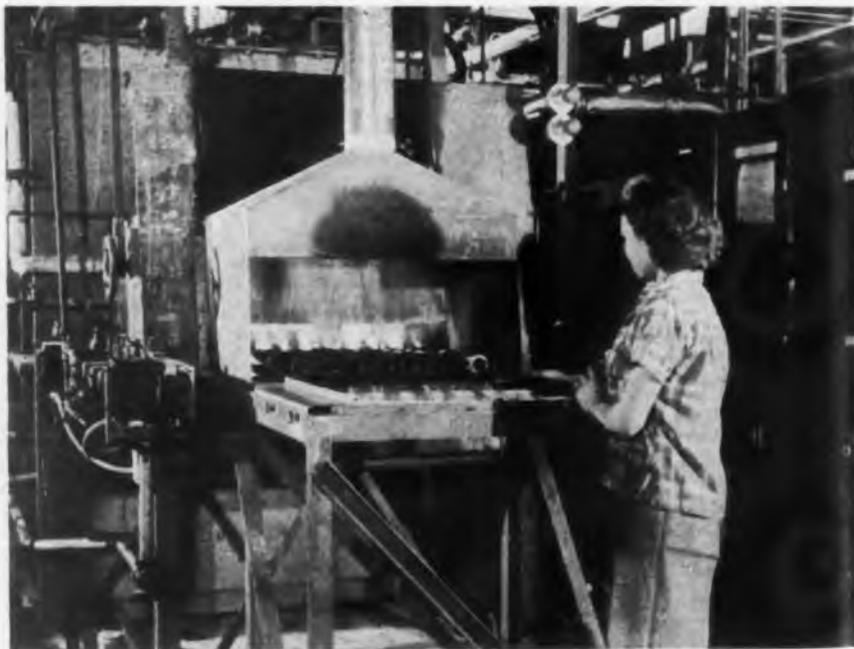
A new job for photoelectric door openers enables unskilled labor to do a good job in the plant of Burgess-Norton Mfg. Co., Geneva, Ill. The installation was made on a new-type, triple action, automatically controlled furnace which brazes, heat-treats, and quenches tank-track parts. The photo is a close-up of the furnace feed. A timer sets the feed-rollers in motion, carrying a tray of parts toward furnace door. The tray in-
