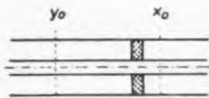
Fig. 5d—Concentric line with dielectric disk
