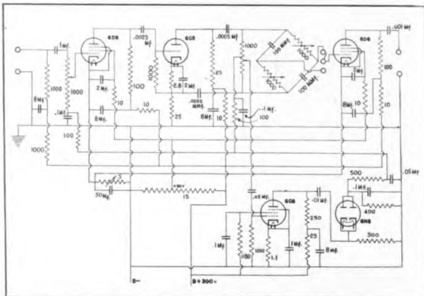
Fig. 5—Sonic flocculating unit capable of developing 2500 watts. Amplifiers at left
