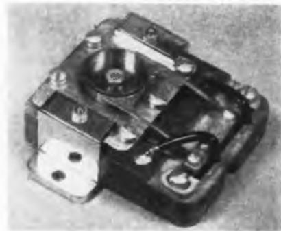
Fig. 6—Western Electric RA-355 vibration pickup with cover removed (above). Combines high-directional sensitivity and wide frequency range
