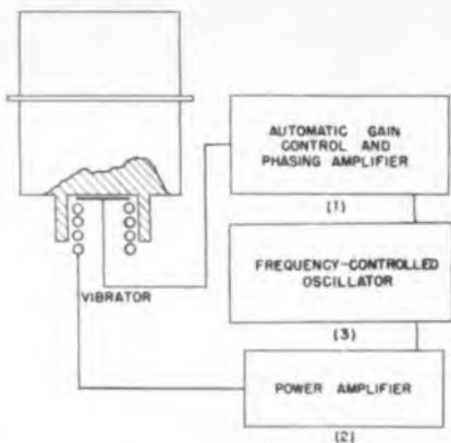
Fig. 2—Block diagram of self-controlled sonic generator using transducer in Fig. 1
