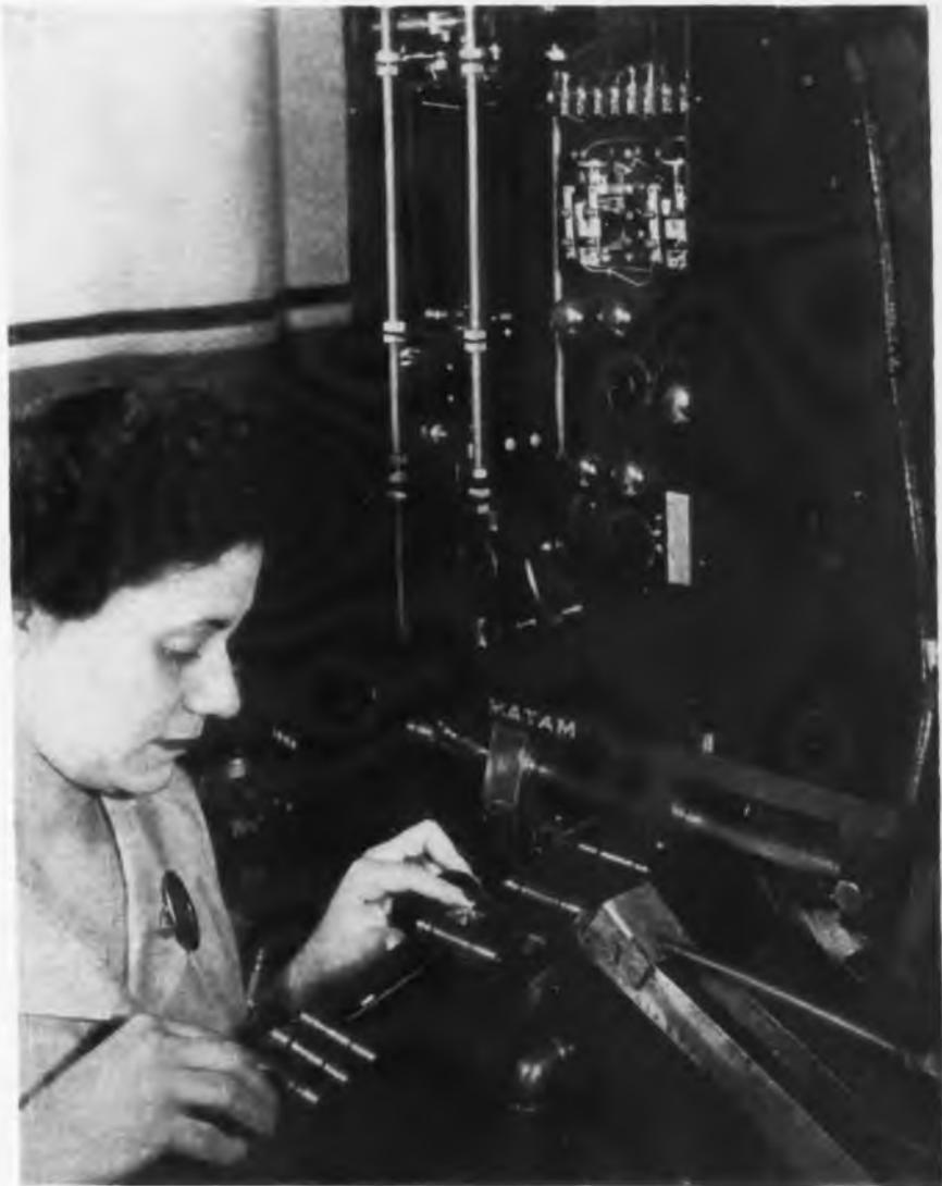
Close-up of delivery end of Matam Corporation's shell inspection machine. Note final measuring and ejecting positions
