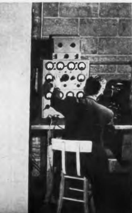
←3. Detonation detector equipment on engine in soundproof chamber. Photo shows tests in progress on improved detonation detector equipment being developed by the research laboratories at Sperry Corp. Tests involved are similar to the actual operation of the equipment as used in work on aircraft engines
