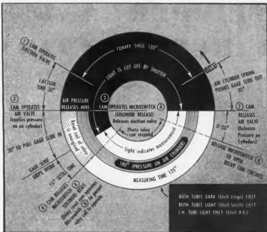
Timing diagram of the automatic shell inspection machine. Microswitches and solenoids referred to are shown in circuit diagram on the opposite page
