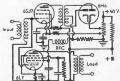
Fig. 4. Limiter circuit with increased control range uses separate amplifier tube (6SJ7) and rectifier (6H6) to control 6L7
