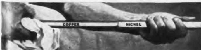
FIRST STEP IN MAKING "KULGRID" bi-metal wire is insertion of copper rod into Pure Nickel tube. The two-in-one wire has 70% of the conductivity of copper . . . is strong and corrosion-resistant, even at high temperatures.
