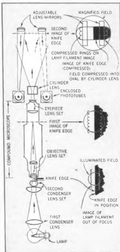
Fig. 1—Diagram of one of the 8 optical and photoelectric units. Knife edge takes a position determined by actual dimension being measured
