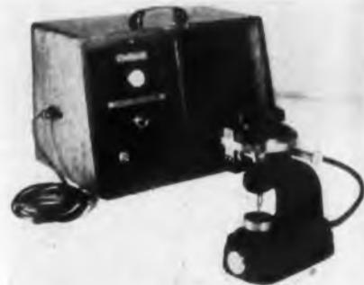
part being measured. The complete equipment, which operates on 110 v. 60 cycle power, weighs about 20 lb., requires no levelling or calibration. There are three models: 4½ in. dial with .00005 in. divisions; 3½ in. dial with .0001 in. divisions; and 2½ in. dial with .0001 in. divisions. Manufacturer is Carson Micrometer Corp., Little Falls, N. J.
