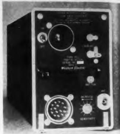
Fig. 10—Glide path receiver, type RUJ
