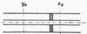
Fig. 5e—Concentric line with ceramic bolt
