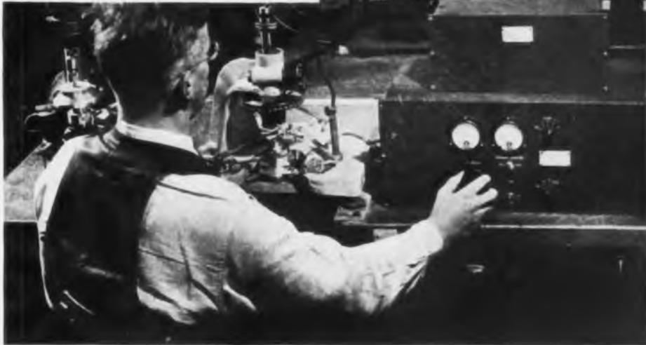
←3. Detonation detector equipment on engine in soundproof chamber. Photo shows tests in progress on improved detonation detector equipment being developed by the research laboratories at Sperry Corp. Tests involved are similar to the actual operation of the equipment as used in work on aircraft engines
