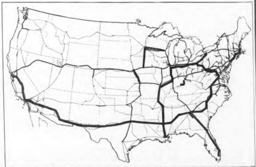
Heavy line indicates proposed coaxial cable routes. Shaded line shows existent coaxial lines
