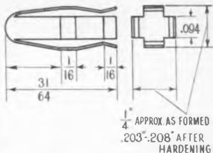
Beryllium-copper banana plug spring is formed from annealed strip and given desired spring properties by hardening after forming. Critical dimensions are held by fixture during the heat treating period
