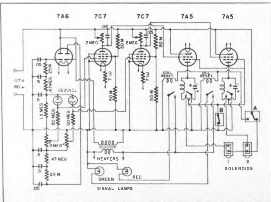
operated at 4.5 volts instead of at 6.3 volts. This has been found to be helpful when phototubes deliver very little current, as in the present case.
