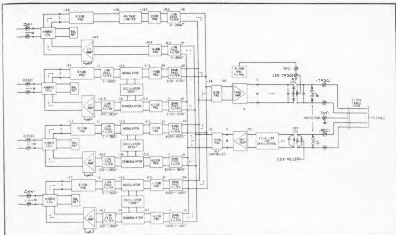
Block diagram of circuit elements at each CF-1-A carrier terminal on equipment location spiral-four system. Channel 1 at top is straight voice frequency while remaining three channels have carriers of 5900 cps, 8850 cps, and 11,800 cps each with pass band of 2600 cps
