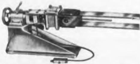
**Features:** Simple harmonic motion with variable amplitude. • Variable frequency from 20 to 70 C.P.S. • Vibration testing can be made in any direction through 360°. • Capacity up to 5 lbs. • Vibration acceleration is provided to 30 G. plus. • Only 75 watts are required for maximum test conditions. • Can be mounted on any bench without transmitting extraneous vibration. • Variable frequency direction provided. • No moving cranks, gears, or bearings in the vibration system.
