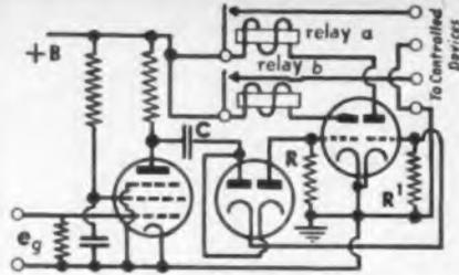
Fig. 7—Circuit to operate relays on positive and negative rates of change of applied voltage e.g. See Fig. 6
