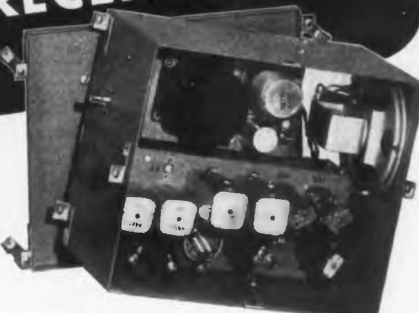
**3** For complete servicing, the entire chassis can be removed from the vehicle by releasing four snap catches. All wiring is instantly accessible.
