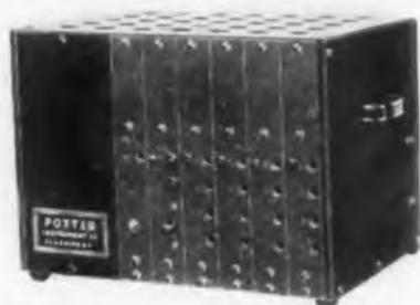
tubes are used for counting and indicating a scale of ten. The answers are indicated for each decade on four neon lamps designated 1-2-4-8. Combinations of these lamps indicate 0 to 9. The instrument operates from a line voltage of 100-125 v 60 cycles ac. The tube complement is 27 tubes. Plug-in construction of the units is used throughout. The counter chronograph interval timer's dimensions are 15 in. x 10 in. x 10 in., and the weight is approximately 39 pounds.
