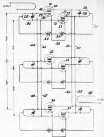
pull amplifier connected according to the invention. A system of two push-pull units, four tubes, may be arranged as a modulator by symmetrically applying the modulation frequency to the tank circuits of the units, and by transposing either tie-lines 44,45 or 50,52 so that the two units operate in phase opposition. The modulation is of the carrier-suppressed type giving only side bands. C. B. Watts, Jr., Federal Telephone and Radio Corp., (F) May 18, 1942. (I) Feb. 1, 1944, No. 2,340,352.
