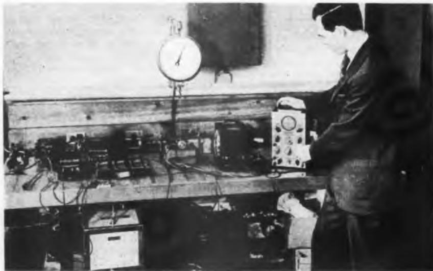
A miniature 400 cycle ac induction motor undergoing complete tests, including the brake test shown, at the laboratory of Eastern Air Devices, Brooklyn, N. Y. On such small motors an ordinary tachometer would be a partial load on the motor, so that speed is checked stroboscopically, while an oscillograph checks motor-current waveform. Line and phase am-
