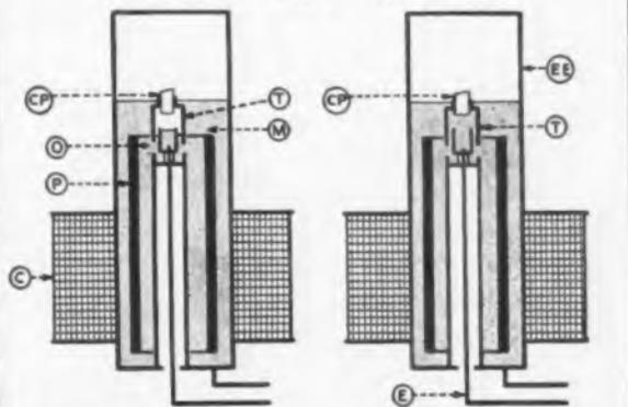
**ENERGIZED**—Coil C pulls plunger P down into mercury. Mercury thus displaced enters thimble T through orifice O. Inert gas in thimble gradually escapes through ceramic plug CP—thus producing time delay.
