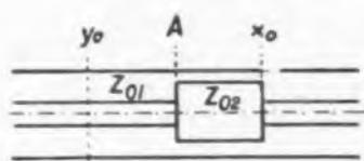
Fig. 5b—Quarter wave length transformer
