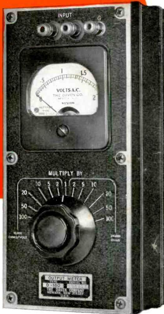
The DAVEN D-180 Output Meter is a combination of a high impedance voltmeter and a constant impedance output meter. The high impedance voltmeter range is particularly convenient when measuring transformer secondary voltages and as a bridging indicator where a high impedance is required. The constant impedance range serves as a null detector and as a beat indicator in the comparison of two frequencies.
