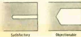
**HOLES PARALLEL TO LAMINATIONS**—Avoid large holes parallel to laminations where subsequent pressure, as from a screw, might injure the piece.
