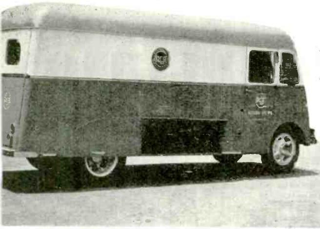
Battery compartment is located under the floor of the truck with batteries accessible through doors in side
