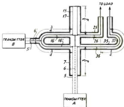
of the load has, therefore, a relationship with respect to the other, carrying phases  $P_A$  and  $P_B$  from the two transmitters, of  $P_A \pm 180^\circ \pm 90^\circ$  and  $P_B \pm 90^\circ$ . Line 15, 17 counterbalances any reactive component introduced into the lines due to the connection between the single-sided and push-pull circuits. Nils E. Lindenblad, RCA, (F) May 31, 1940, (I) Feb. 8, 1944, No. 2,341,408.
