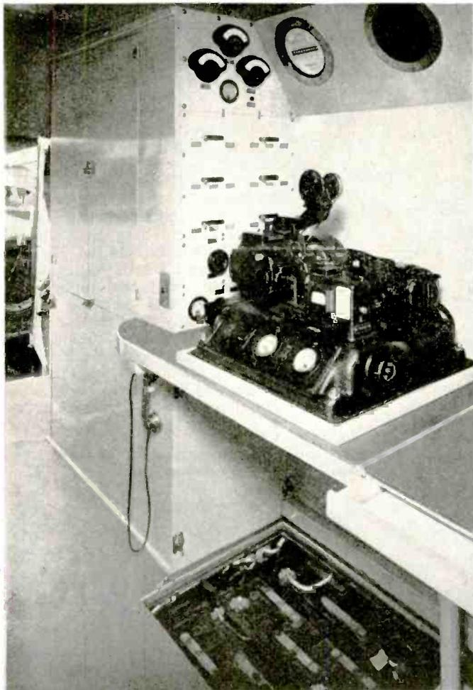
The sound film track recording equipment is mounted on a convenient shelf with its controls and meters built into the bulkheads adjacent to it. Beneath the machine one of the below-floor externally accessible battery compartments is shown with the floor up
