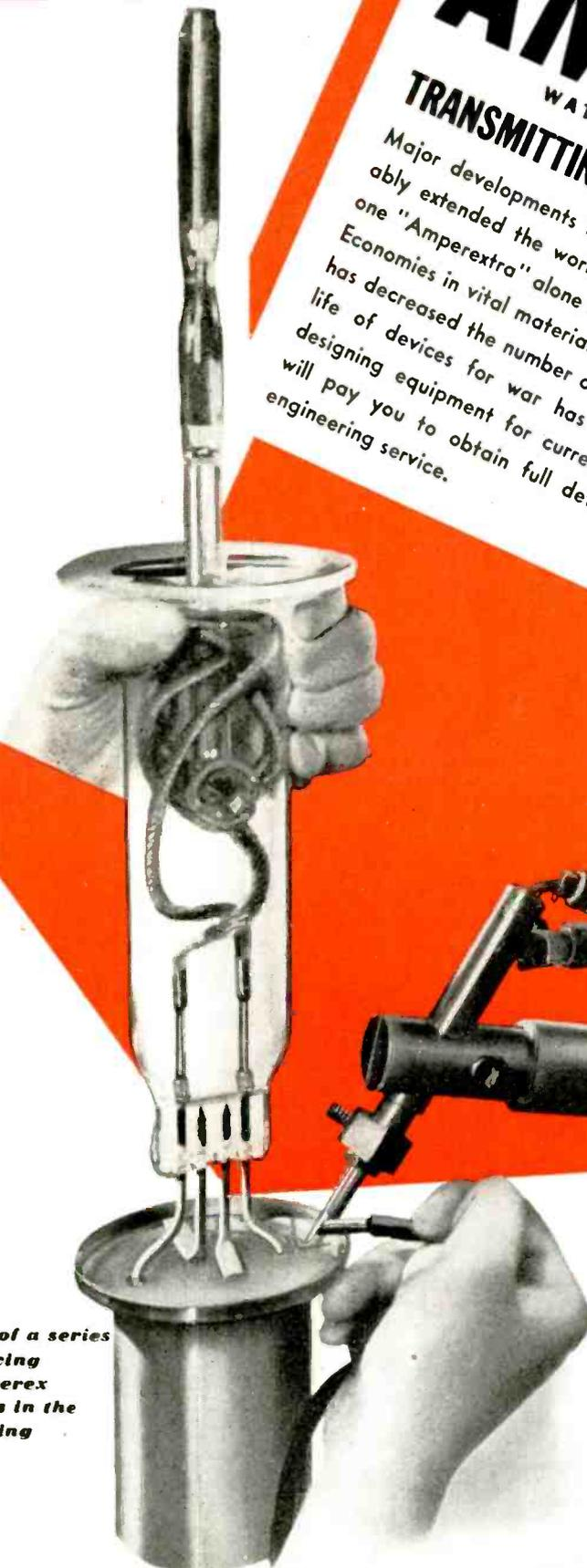
One of a series showing Amperex tubes in the making
