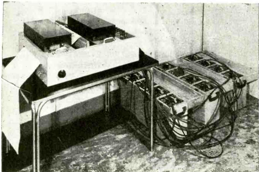
Illustrated above is a thirteen channel instantaneous direct recording oscillograph built to solve a specific recording problem.
