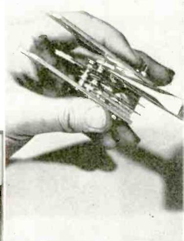
↑ **CROSS BETWEEN** tweezers and a pair of pliers, this tool is used by Electronic Labs., Indianapolis, Indiana, for removing broken screws or nuts from between reeds in vibrators. Just a pair of tapered half-round nose pliers with points ground down to be ultra-narrow, but a handy tool for any work in close, confined quarters. Sides must be ground slowly and carefully to avoid overheating and removing temper
