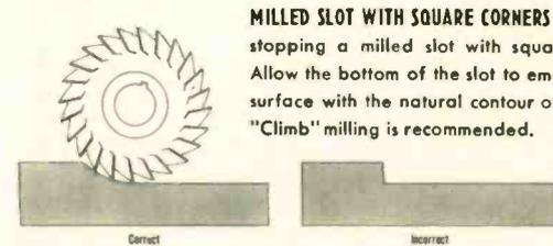
**MILLED SLOT WITH SQUARE CORNERS**—Avoid stopping a milled slot with square corners. Allow the bottom of the slot to emerge to the surface with the natural contour of the cutter. "Climb" milling is recommended.
