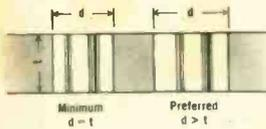
**DIAMETER OF PUNCHED HOLES**—The preferred ratio of hole diameter to thickness of material is not less than 1:1. That is, the diameter of a punched hole should not be less than thickness of sheet.
