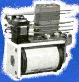
ABOVE—Type 108—Antenna switching contact combination with Mycalex insulation. Has a side contact mount to reduce capacity between antenna circuit and ground.
