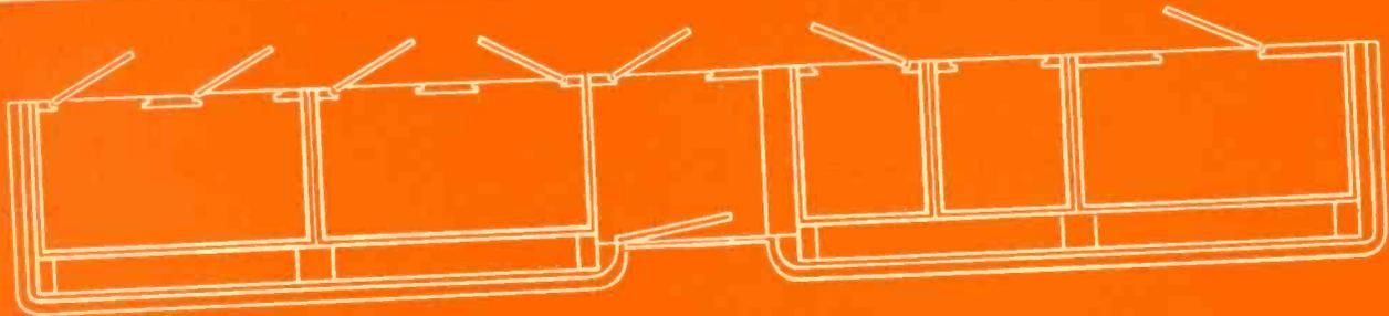
**FLOOR PLAN AND END ELEVATION.** The total length of the transmitter is 39' 6"; height 7' 6"; depth 6' 6". The transmitter proper consists of four cubicles, each 8' wide and 5½' deep. A wide passageway is provided in the center of the transmitter; and electric interlocks prevent transmitter from being placed in operation until all entrance doors are closed.
