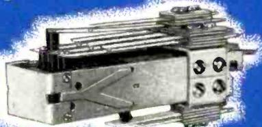
**BELOW—Type 300—**A double pole, double throw, latching relay arranged with two interlocking armatures. Either coil operates with a single impulse and contact remains until the other coil is energized.
