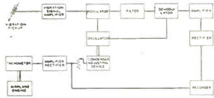
in separating very low frequencies, the full accuracy of the analyzer is not guaranteed below 5.5 cycles.
