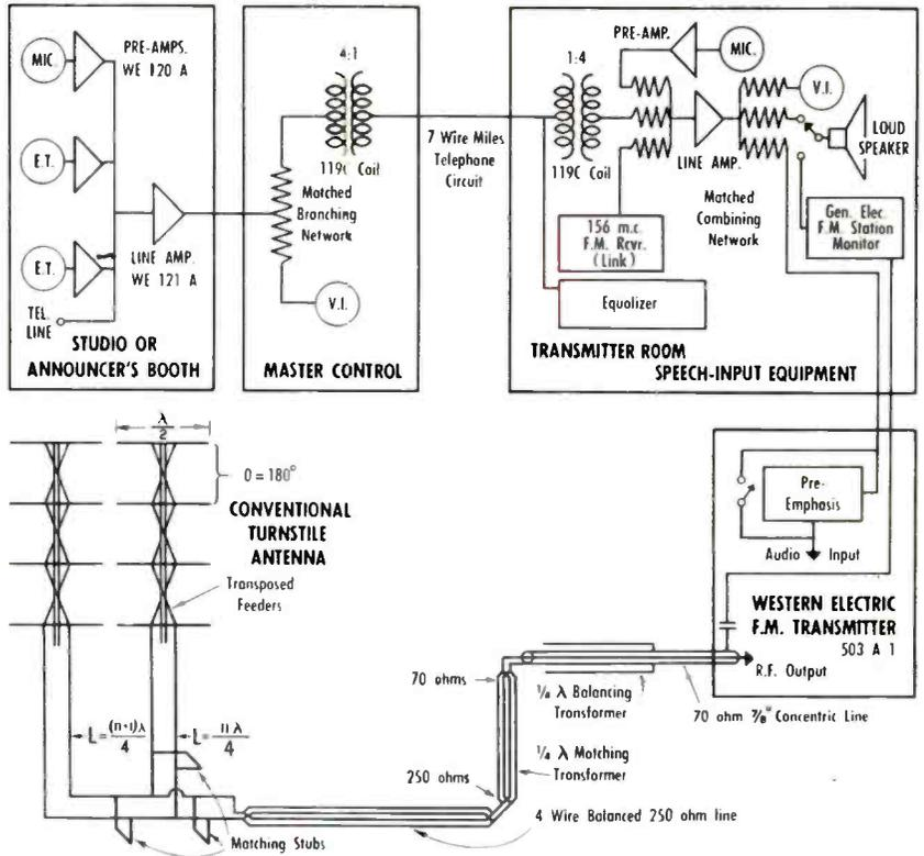
The model 503A Western Electric FM transmitter feeds antenna through coaxial line
