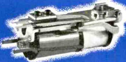
ABOVE—Type 102—Time delay relay of the slug type. Pure copper slug on heel end of core provides maximum of 300 milli-seconds delay in contact opening after circuit is broken.
