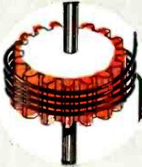
Electronic heat can surface harden gear teeth or localized areas in seconds instead of hours . . . with precise control over depth and degree of hardness.
