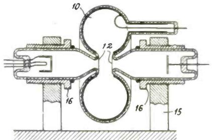
this type of tube from a glass pipe is extremely simple. To tune the resonator, pressure is exerted by turning screw 16 so that the two openings 12 come closer together. The glass yields sufficiently to permit tuning of the circuit within limits. Several resonant chambers may be blown consecutively in the same glass pipe. E. Steudel, General Electric Co., (F) Aug. 30, 1941, (I) March 7, 1944, No. 2,343,487.
