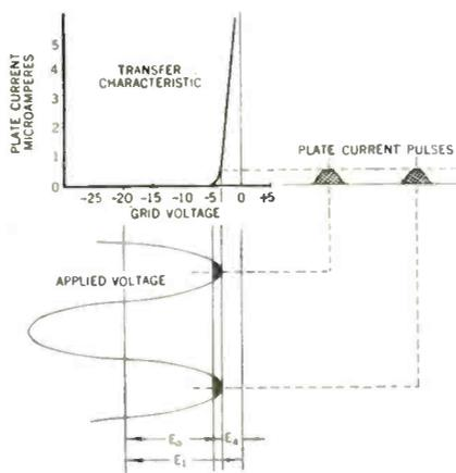
Fig. 2—Graphic presentation of operation. Transfer characteristic of the tube for the applied plate potential is plotted
