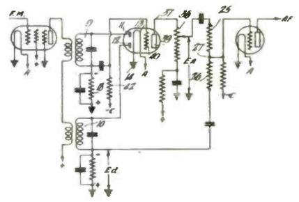
adjusting resistor 36 to output resistors 25 and 26. Output of diode 12,13 is connected directly to the other terminal of resistors 25,26. It will be seen that for suitable adjustment of the tap on resistor 36 amplitude modulation signals will be balanced out, while frequency modulation may be taken off point 27 between resistors 25 and 26. W. R. Koch, RCA, (F) July 31, 1941, (I) Feb. 8, 1944, No. 2,341,047.
