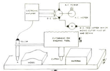
Tube-controlled tracer mechanism for intricate surface-machining
