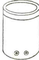
**APPARATUS ENCLOSED SOLDER-SEAL BUSHING**—combination insulator, cover and terminal board—has a hollow construction which permits placing small devices inside.
