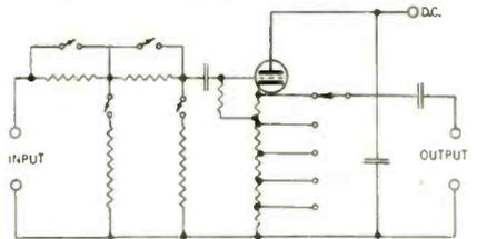
**Fig. 4. Input circuit of the low frequency VTVM, which uses a ladder type divider**
