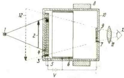
weak source. The latent image 4 of object 2 causes reactive layer 3 to give off charged particles or gamma rays which in turn release electrons within layer 3 or in an adjacent layer 5. The electron image so produced is reduced by an electron-optical lens system 6,8, so that the image 9 produced on screen 7 is much smaller than the latent image 4 and of comparatively high intensity. If 7 is a luminous screen, the image is
