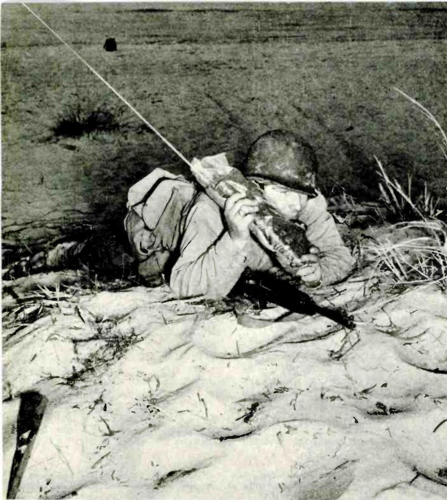
Even the ubiquitous "Handi-Talki" must be adequately waterproofed, here with a special type of covering put on as an expedient by the soldier himself to permit operation under all conditions
