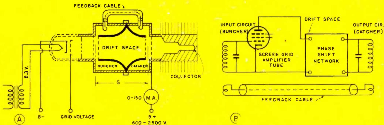
Fig. 7. Klystron tube at A showing bunching distance  $S$  and equivalent conventional tube circuit at B. Phase-shift network replaces drift space
