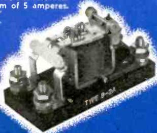
**ABOVE—Type E-2A—** Conforms to Army Air Force specifications for a 25 ampere contactor. Features pin type bearing, double break contact arrangement which eliminates the necessity for current carrying pig-tails. Adjustable residual and back-stop.
