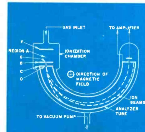
Fig. 2—Details of region A in Fig. 1. Electron beam ionizes gas sample by collision. Voltage V gives forward velocity to ions which in combination with magnetic field and their mass determine path radius
