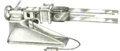
**Features:** Simple harmonic motion with variable amplitude. • Variable frequency from 20 to 70 C.P.S. • Vibration testing can be made in any direction through 360°. • Capacity up to 5 lbs. • Vibration acceleration is provided to 30 G. plus. • Only 75 watts are required for maximum test conditions. • Can be mounted on any bench without transmitting extraneous vibration. • Variable frequency direction provided. • No moving cranks, gears, or bearings in the vibration system.
