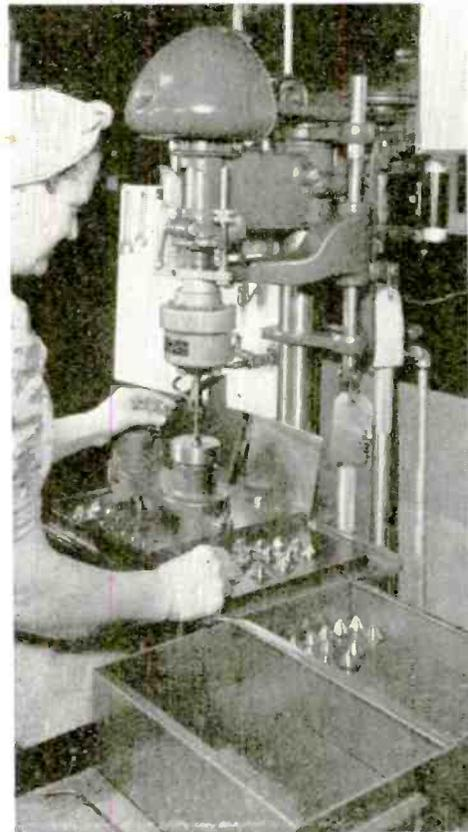
↑ **AIR OPERATED CHUCK** speeds precision work on small round parts and largely does away with need for special jigs and fixtures. Tapping operation illustrated. Air chucks, made by Redmer Air Devices Corp., Chicago, give collet capacity up to one and three-fourths inches
