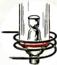
Electronic heat can bond glass to metal faster with finer control of heated area. Often increases production units from hundreds to thousands per hour.
