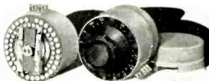
mechanism. Contacts and switches of the attenuators are tarnish-proof silver alloy. Cleaning and lubricating of the contact points has been eliminated. The new type steel cover provides improved magnetic shielding. The body of the cover forms an integral part of the attenuator assembly, protecting the resistors. A snap-on cap gives access to switch blades and contacts.
