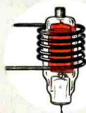
Electronic heat reaches through glass walls to degas metal elements in radio and fluorescent tubes without affecting the envelopes. Action is instantaneous.
