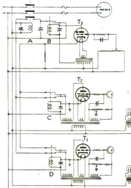
Schematic of revolving door control system
