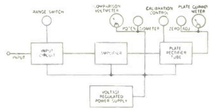
Fig. 3. Block diagram of the vacuum tube voltmeter designed to measure very low frequencies
