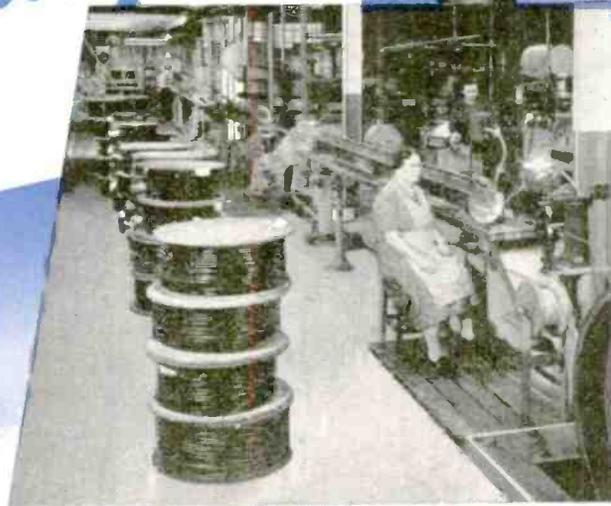
Clean, smooth, properly centered polyethylene covered wire is extruded by this machine.
