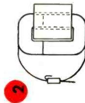
**2** Core parts are butted together. Strap is threaded through seal and . . .
