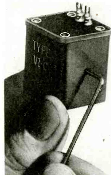
use in oscillators, (a model with 30 per cent tap for Hartley circuits is available), tuned amplifiers, equalizers and filters. It is housed in a die cast case, weighs approximately 5 oz. and the inductance is varied by means of an Allen wrench. There are nineteen standard types, from .0085 to 33.0 henries.
