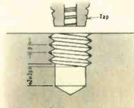
**TAPPING IN A BLIND HOLE**—When tapping in a blind hole, allow a depth of several threads from the bottom of the hole to first full thread for clearance.
