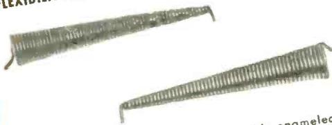
Formex wire (bottom) compared with enameled wire (top). The outer surfaces of the films have been elongated by stretching around a tapered mandrel and heating the samples to 150 C. Note the cracks on the enameled wire.
