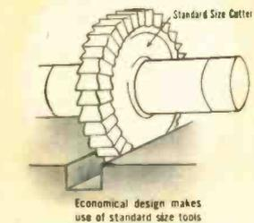
**DESIGN FOR MACHINING WITH STANDARD TOOLS**—Try to design parts so that machining can be done with standard tools or cutters. Specify standard size holes and slots wherever possible to avoid special tooling.
