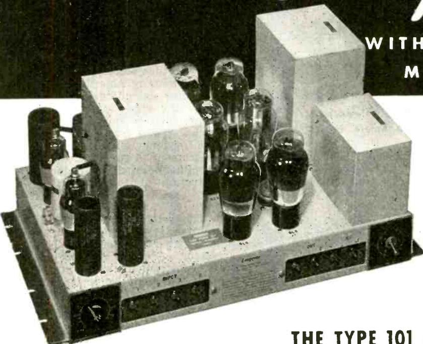
Input impedance 600 ohms and bridging. Gain 600 ohm input 61 db., bridging input 46 db. Frequency response 30 to 16,000 c.p.s. either input—600 ohm output  $\pm .5$  db., 30 ohm output  $\pm 1$  db. Power output—production run average: +47 V.U. with less than 3% RMS harmonic content.
