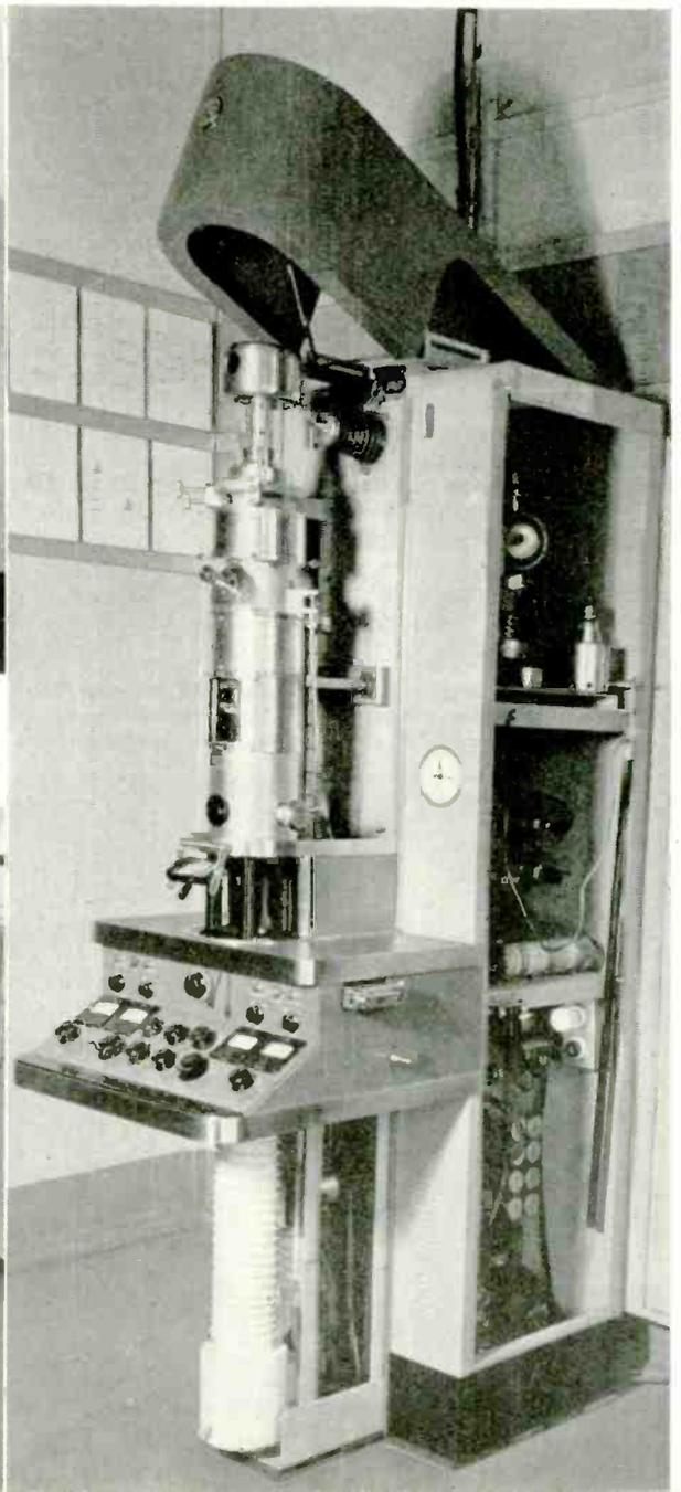
RCA's type EMC electron microscope is a simplified version of the larger model in console form intended primarily for industrial use
