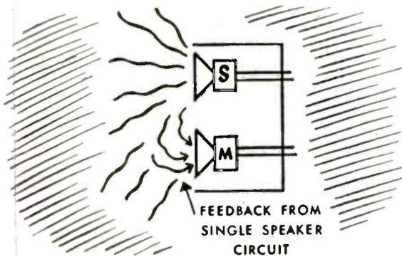
The Dalmo circuit commercially eliminates sound feedback by the use of two speakers and a microphone, symmetrically located and connected out of phase, like this . . .
