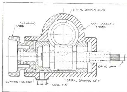
Fig. 7—Phase shift control is effected by advancing minor shaft using spiral gears
