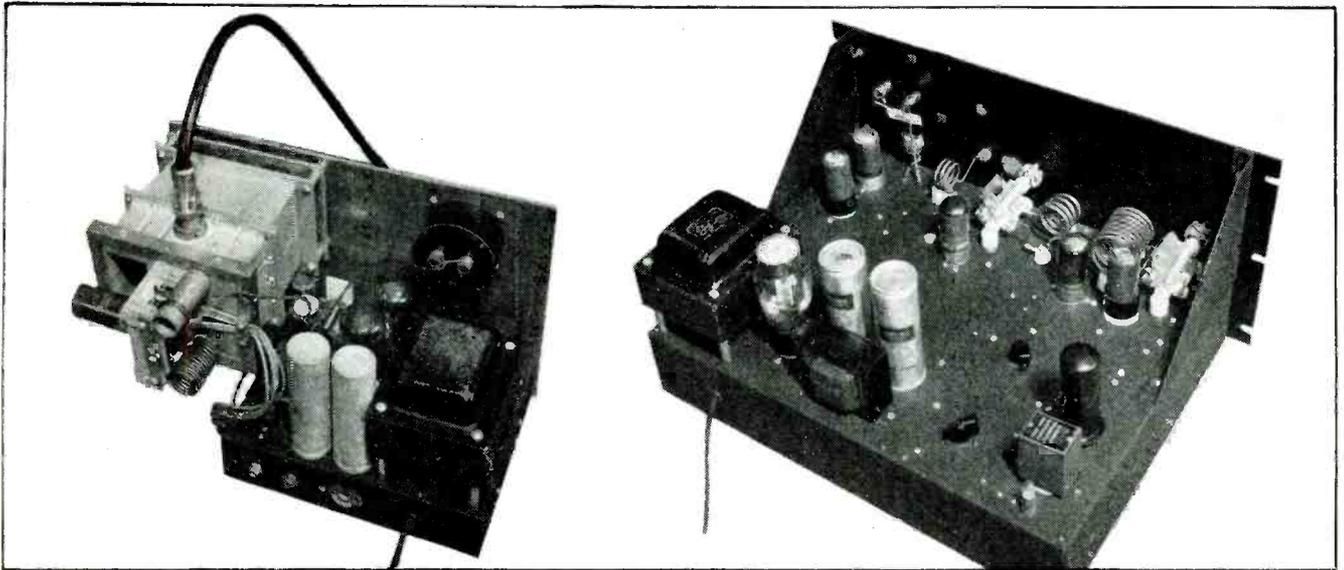
Fig. 4—At left, original model with power supply and modulator. At right, secondary standard for operation above 1,000 mc using 5 mc crystal
