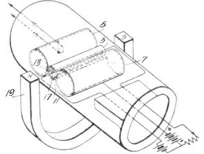
force or establish standing electromagnetic waves within the cavities. The device may be used as detector, amplifier or generator of uhf waves. E. G. Linder, RCA, (F) Oct. 24, 1940. (I) May 16, 1944, No. 2,348,986.
