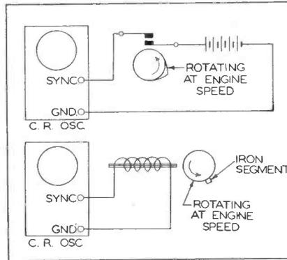
Two methods for getting a cathode-ray oscillograph to follow the variations in speed of the engine. Fig. 1 (above) uses a cam-driven contactor to initiate the synchronizing pulse. Fig. 2 uses a magnetic pulse generator
