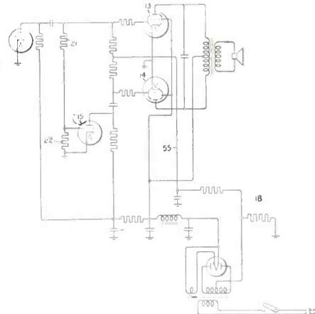
power supply 18. Bias is supplied over conductor 55 to the control electrodes of amplifier tubes 13 and 14. The result is that the hum voltages supplied to the grid of tube 14 from the bias source cancels that supplied thereto from the phase inverter circuit, leaving in the output circuit only the hum supplied to the grid of tube 13. J. A. Worcester, General Electric Co., (F) March 27, 1943, (I) June 6, 1944, No. 2,350,858.
