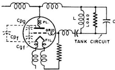
Fig. 7—In uhf operation the inductance and capacitance of the leads, shown here as lumped values, become important circuit components
