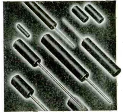
applications at broadcast band frequencies. Similar side-molded cores are now available for short wave frequencies including television and frequency modulation. Conventional cores molded by applying pressure to the ends, result in a dense grouping of iron particles at these points, thus interfering with uniform permeability. In side-molded cores, however, any density resulting from molding pressure extends
