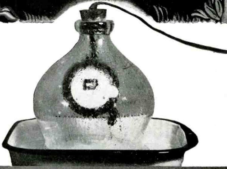
Jungle Conditions—One of the laboratory tests simulating field use is a minimum run of 120 hours at 120° F, 95 RH. Component parts have previously been tested at 180° F.
