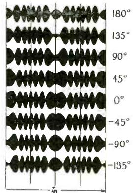
Fig. 3—Oscillograms for various phasing between modulated and unmodulated carrier
