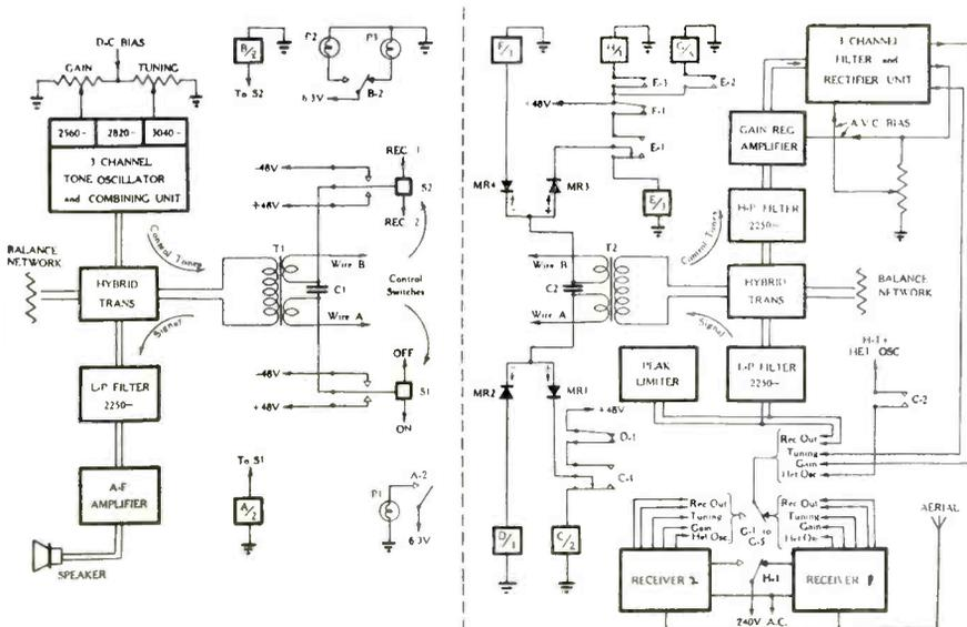
Fig. 2—Remote control installation for two receivers
