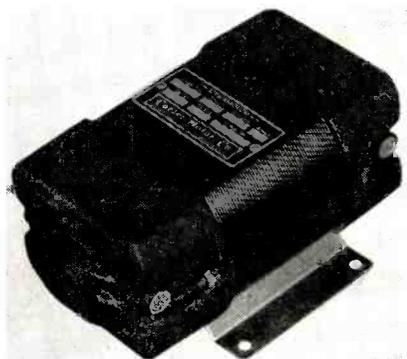
Units are available with inputs ranging from 6 to 115 volts dc and outputs up to 600 volts at .25 ampere. The size of the largest dynamotor is 7 1/4 in. long by 4 1/2 in. wide by 3 1/2 in. high, and without the filter (available on order) weighs 9 lb.
