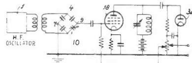
compensating means for this non-linearity. For this purpose, part of the output of rectifier tube 32 is fed back in phase opposition to the input wave, thereby reducing the excessive change in input voltage at high pressures. P. H. Dijksterhuis, Alien Property Custodian, (F) April 9, 1941, (I) May 9, 1944, No. 2,348,245.
