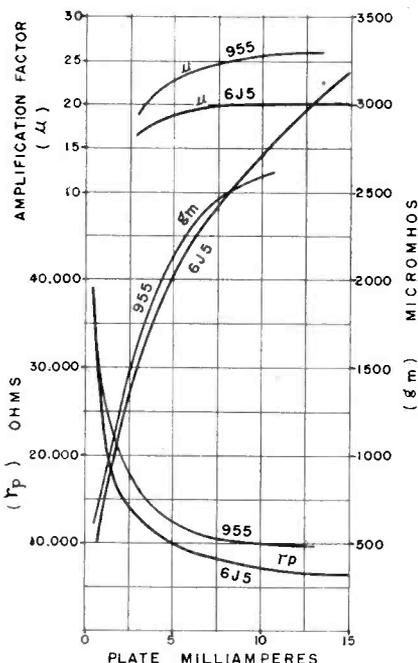
Fig. 9—Comparison of transfer characteristics of the Type 955 acorn and the commonly used octal type tube 6J5
