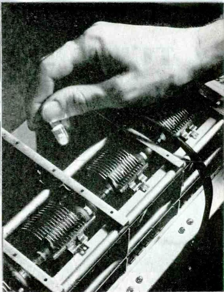
Time—even a lot of it—spent on a jig or fixture is quickly repaid in labor savings on the production line. This two-sided steel dimension gage checks accuracy of fifteen dimensions in two simple go, no-go operations. The ceramic plates are end pieces for variable condensers. If hole placements after firing aren't kept within close limits, strains cause gradual changes in characteristics of finished condensers
