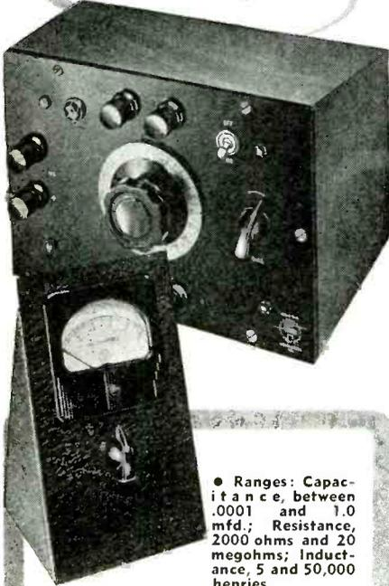
• Ranges: Capacitance, between .0001 and 1.0 mfd.; Resistance, 2000 ohms and 20 megohms; Inductance, 5 and 50,000 henries.
