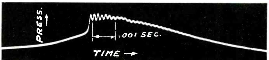
Fig. 11—High frequency detonation waves show up on high speed pressure diagram taken with new oscillograph
