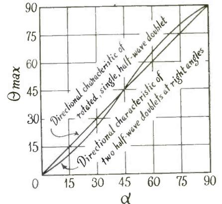
Direction of rotating coil for max. induced voltage as function of direction of wave propagation
