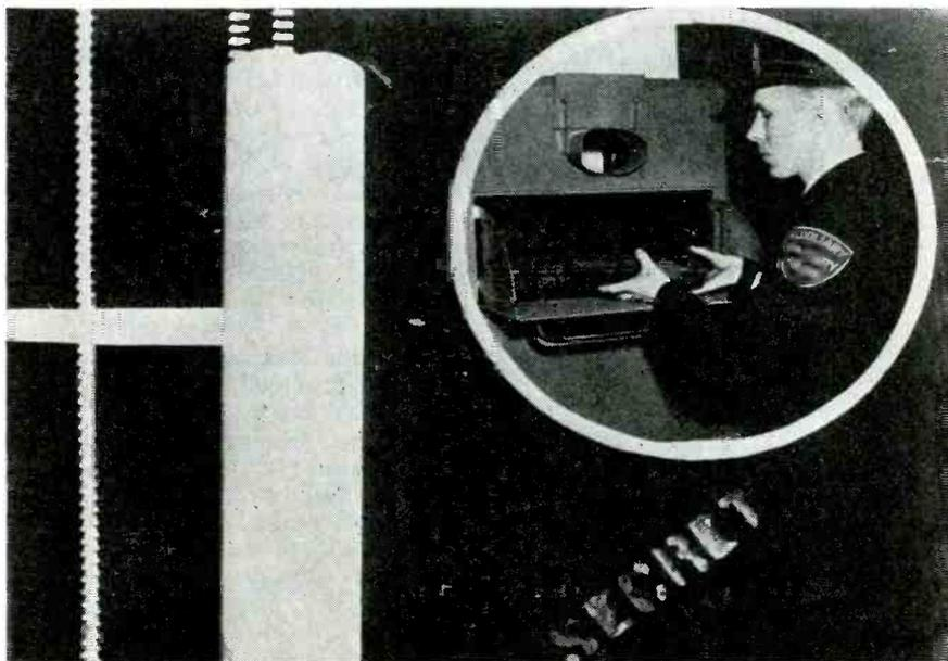
A new marking compound, developed by North American Philips Company, Inc., New York, is used to mark secret documents. The photo shows how such a paper, marked with the compound, looks in the Searchray machine—the secret paper was hidden in a stack of literature 1 1/2 in. thick and was enclosed in a zipper bag. The insert view shows a plant guard placing the bag into the compartment of a Norelco industrial X-ray unit where he will view it by means of a fluoroscope
