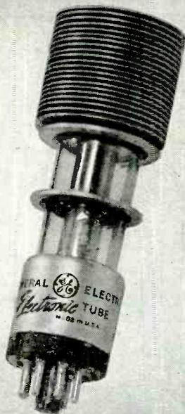
The G-E disk-seal tube — a development that makes ultra-high frequency relaying possible.
