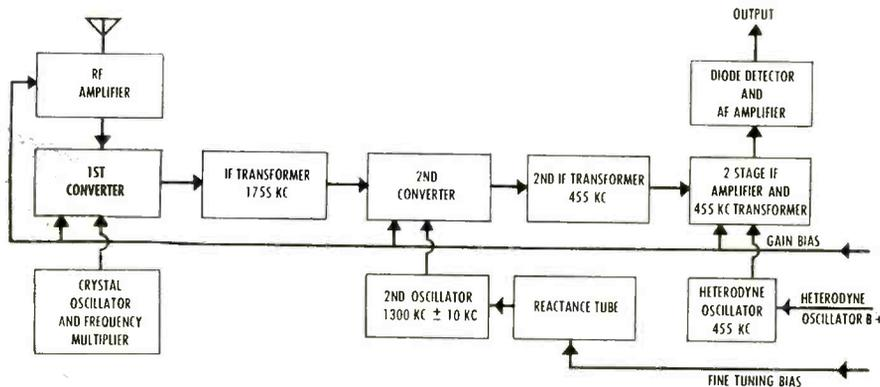
Fig. 1—Double-conversion superheterodyne receiver in remote control circuit
