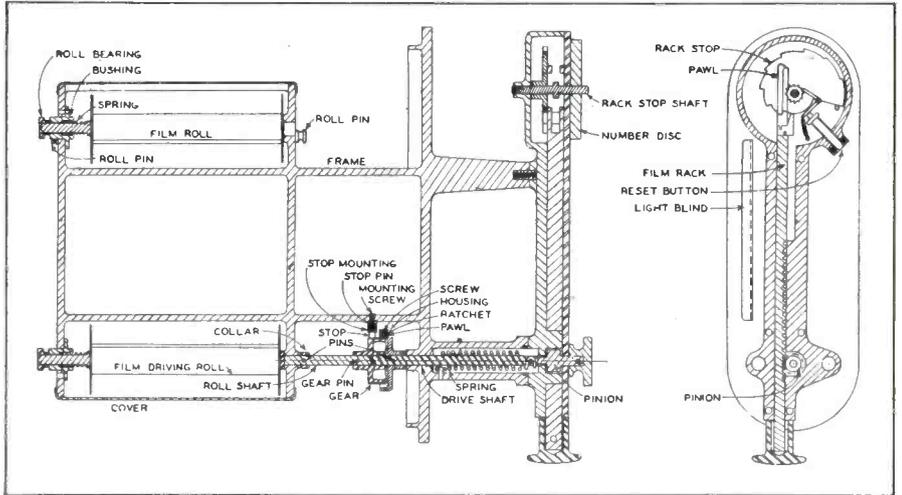
Fig. 9—Shows the controls and indexing details of the film holder. Standard roll type film used
