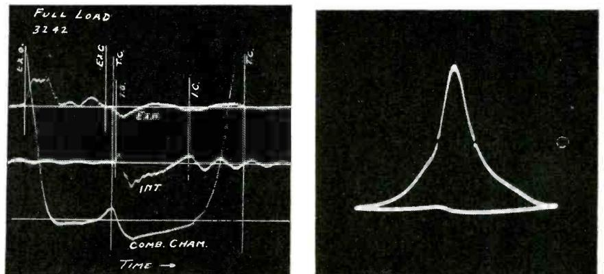
Fig. 10—A typical oscillogram with three pressure effects shown simultaneously (left). At right, a regular indicator diagram with calibration marks appearing at a predetermined level
