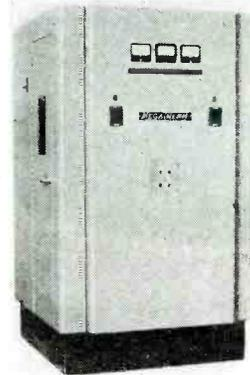
aluminum alloy pieces as well as the usual steel parts. The heating fixture is a simple coil of from one to five turns which can be constructed readily from standard copper tubing. The unit is designed to deliver 25 kw of output continuously at frequencies adjustable within the 2-5 million cycle range and measures 4 x 4 x 7 ft.
