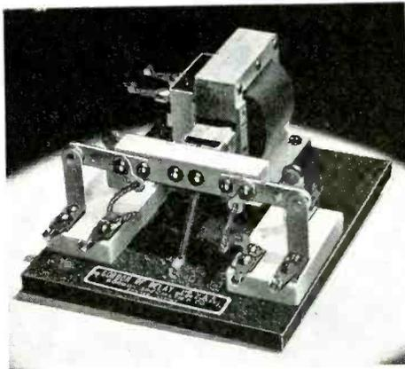
• A heavy duty D.P.D.T. relay providing many desirable electrical and mechanical characteristics. Alsimag 196 insulation which, because of its extremely low power factor of .04, shows negligible losses even at frequencies up to 300 mc.
