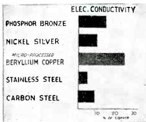
Before heat treatment, the conductivity of Beryllium Copper is the same as phosphor bronze. Conductivity increases during heat treatment, and response varies with each lot of material. Micro-processing is the only sure way of obtaining the value shown above, and at the same time reaching maximum overall spring properties. Still higher conductivity values are obtainable at some sacrifice in other properties.
