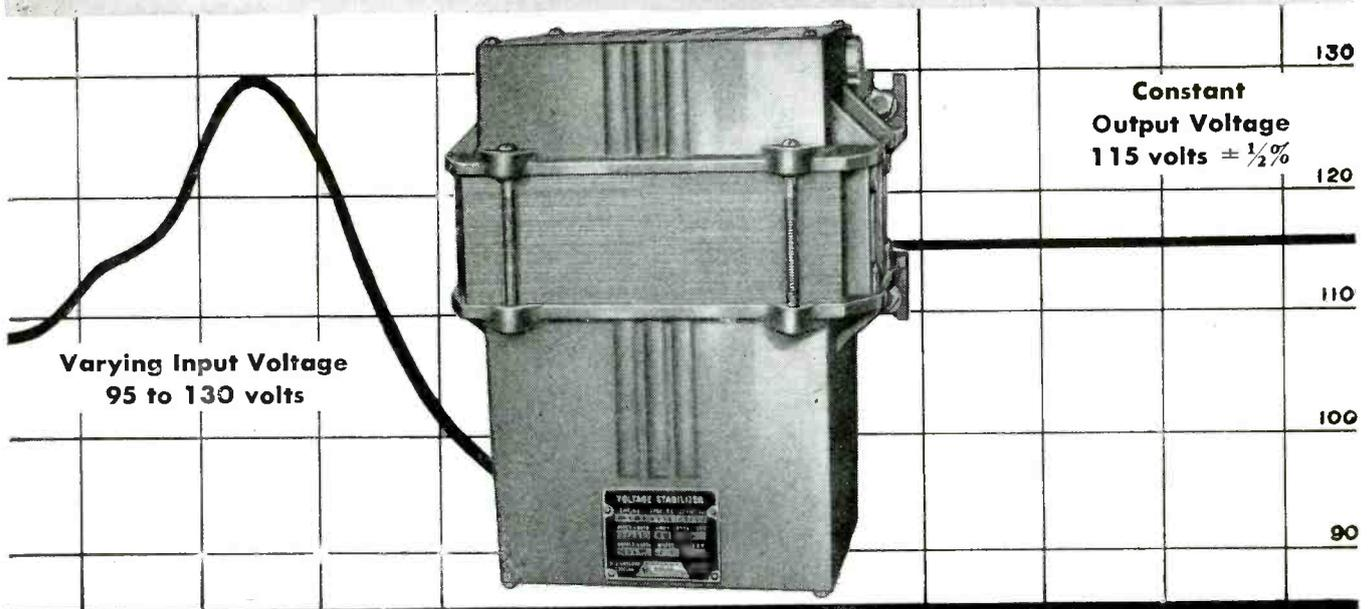
Precision operation of a wide variety of factory testing, production and laboratory electrical equipment requires uniform, stabilized AC input voltage. A Raytheon Voltage Stabilizer, incorporated in the product, permanently eliminates fluctuating voltages by assuring constant output voltage of 115 volts  $\pm 1/2\%$ . They are available in three designs to meet practically every installation requirement. Bulletin DL48-537 gives the complete story. Write for your copy.
