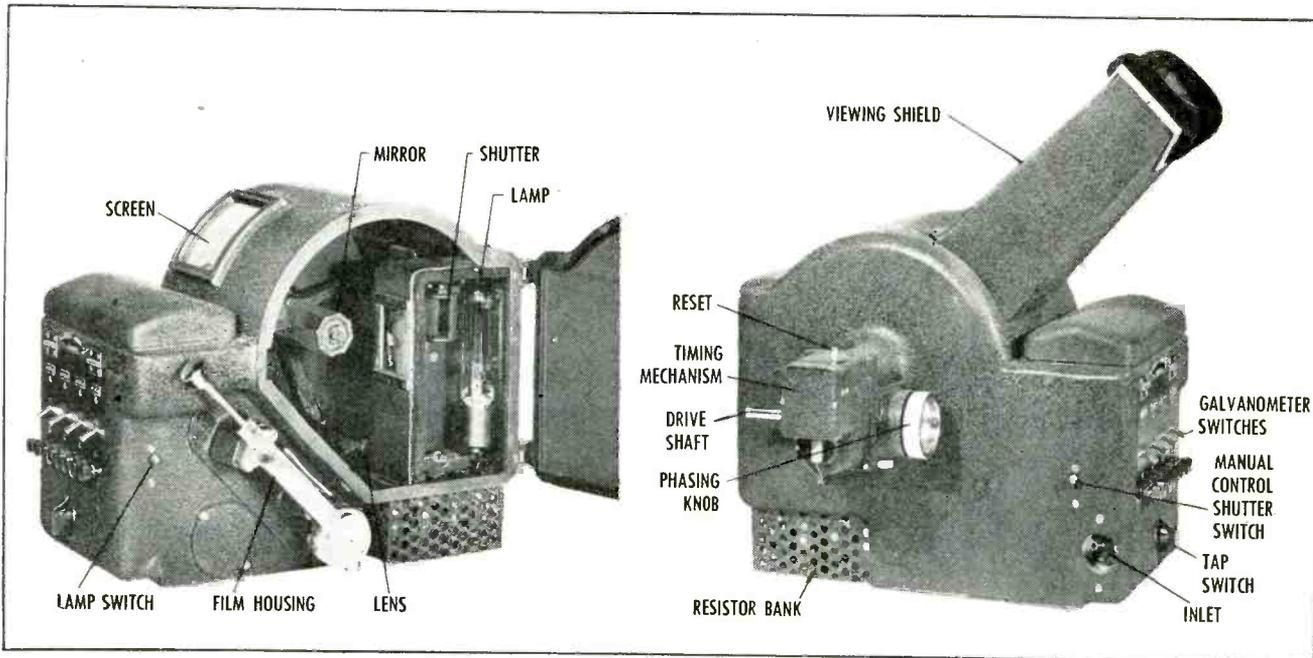
Fig. 6—Shows two views of the General Motors oscillograph with components primarily developed for the study of the combustion engine research problems of that organization in the viewing and recording of engine indicator diagrams
