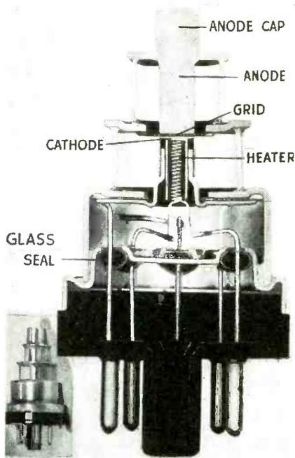
the war. The new tube eliminates the conventional type of grid, anode and cathode. Instead of components being fitted around one another as in the past, they are now constructed in simple, parallel planes or layers, with glass and metal fused together in rigid, inseparable units. This design permits an extremely compact over-all tube structure, while providing high frequency and high power output.
