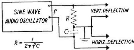
Fig. 3—Basic form of circular time base "rotating" circuit
