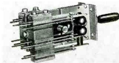
bounce. Coil springs are used on both sides of the cam so that equalized pressure is assured regardless of the number or arrangement of contact assemblies. The switch is static shielded and is of non-corrosive construction. All contacts can be removed from frame by removing a single bolt. Control knob can be supplied with light or stiff action. Contact rating is 10 amps., 125 volts ac, and 2 amps., 125 volts dc.
