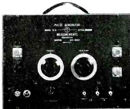
Fig. 2—Panel controls of generator regulate pulse frequency and duration
