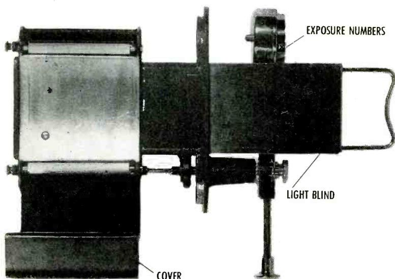
Fig. 8—View of indexing mechanism associated with film holder
