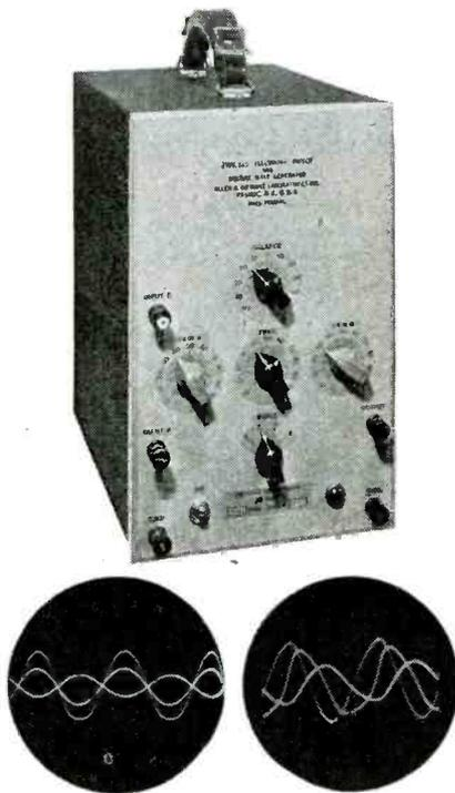
Fig. 1 shows a form of electronic switch providing a method of superimposing two different factors with correct phase relations. To show three factors simultaneously, requires two of these switching circuits, illustrated in the oscillograms. The connections needed are shown in Fig. 2, below
