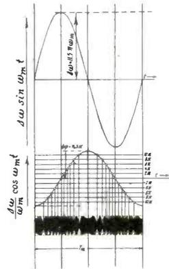
Fig. 1—Constructing phase angle and shape of modulating wave from oscillogram
