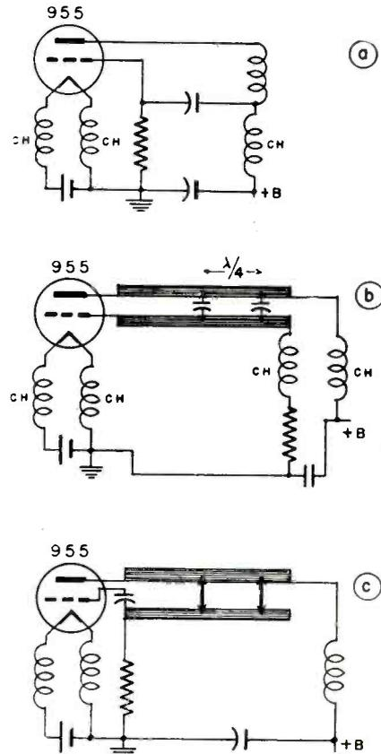
Fig. 10—Typical oscillator circuits using acorn tubes
