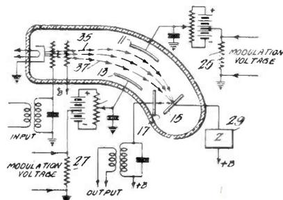
If a square wave voltage is applied to resistors 25 and/or 27 alternate response to two different frequencies is obtained, and by applying a sawtooth modulation wave the response curve may be continuously shifted through a desired frequency range. If the sawtooth frequency is very high, a band pass characteristic will result.
