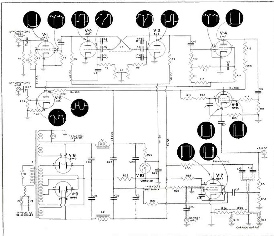
$V_5$  to a low current value and the incoming positive pulse as shown at pin 5 of  $V_5$  causes an increase in plate current and a corresponding output wave across  $R_{19}$ .
