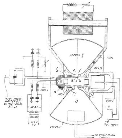
pair of magnetic lenses constituted by gaps c-d and e-f. The threads on sleeves 14 and 15 enable the variation of the length of the magnetic gap c-d. The band width of this type of tube is much greater than that of conventional types because of the higher shunt impedance possible at the gap. F. H. Kroger, RCA, (F) Sept. 22, 1939, (I) June 6, 1944, No. 2,350,907.
