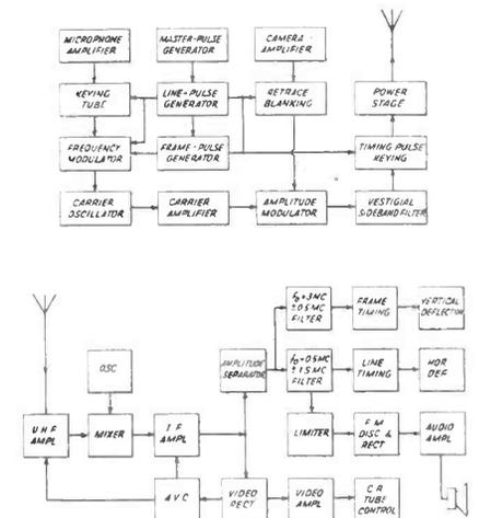
but over a wide frequency range of 2 mc. Periodically at the end of each frame the carrier is shifted to a third frequency to provide the frame synchronizing pulses. The amplitude of both synchronizing signals exceeds the black level. The figures, block diagrams of a transmitter and a receiver, respectively, are self-explanatory. H. E. Kallmann, RCA, (F) Aug. 27, 1941. (I) June 6, 1944, No. 2,350,902.
