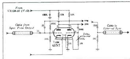
Fig. 3—Flip-flop circuit which can be used to give sliding pulses
