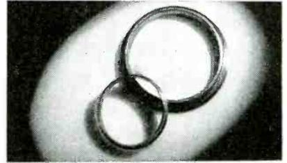
Inner bearing-races, perfectly machined, for an amazing instrument that speeds Allied progress and hastens total victory. They must be held to very close tolerances and carefully finished—and they must be turned out by the thousands on a mass-production basis.
