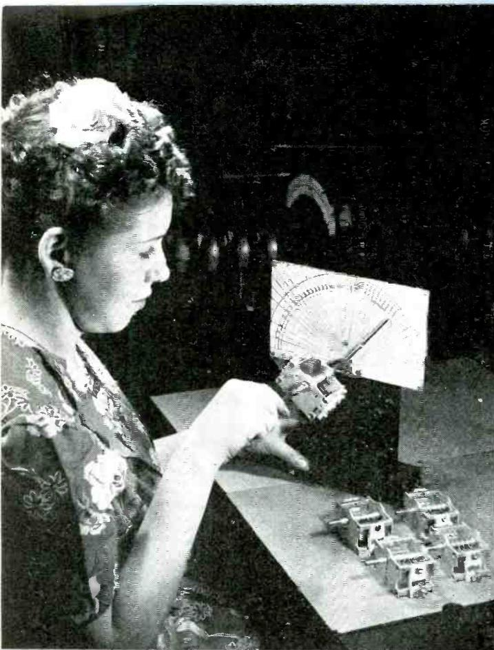
Simple torque gage for transmitting condensers consists of a weight-loaded spindle carrying a pointer and calibrated scale. Test is for smoothness of action as well as torque inch-ounces. Lower front plate is provided with stops to limit travel of weights (behind plate) for rapid inspection of condenser types where specs do not require extremely close torque-tolerances
