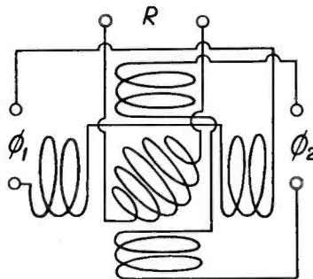
Fig. 5—Internal connections of rotatable transformer with two-phase output
