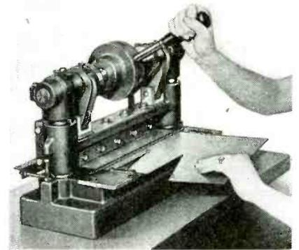
to be used for a wide variety of slitting and notching operations to close tolerances. The unit is equipped with a stripping guide and a delivery chute to allow sheared parts to be automatically loaded into a receptacle. The shear weighs approximately 150 lb. Manufactured by O'Neil-Irwin Mfg. Co., Minneapolis 15, Minn.
