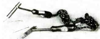
places. The extendable tip turns straight through the center barrel, making the tool quick heating and reducing current consumption. Heating element coils are sealed in ceramic insulation. There are three sizes, 65, 100 and 125 watts, the smaller size weighing 8 oz.
