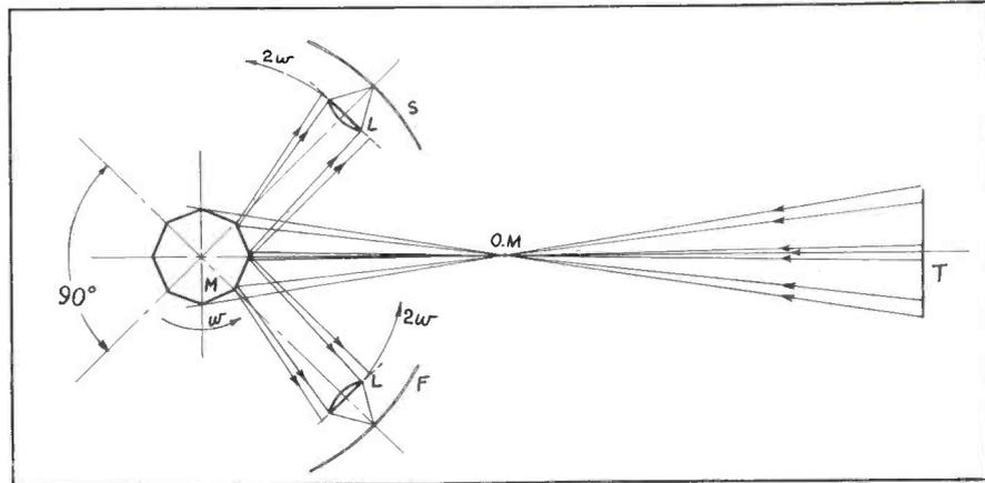
Fig. 4—(above). The rotating mirror system provided in the oscillograph provides simultaneous viewing and recording. The complete optical system is shown in Fig. 5 below
