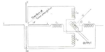
Schematic of half-wave doublet goniometer
