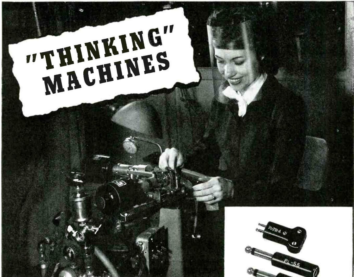
Machines designed by Remler to perform multiple operations: automatic slotting; indexing; drilling; milling and reaming.
