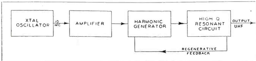
Fig. 3—Simplified schematic diagram of the frequency multiplier
