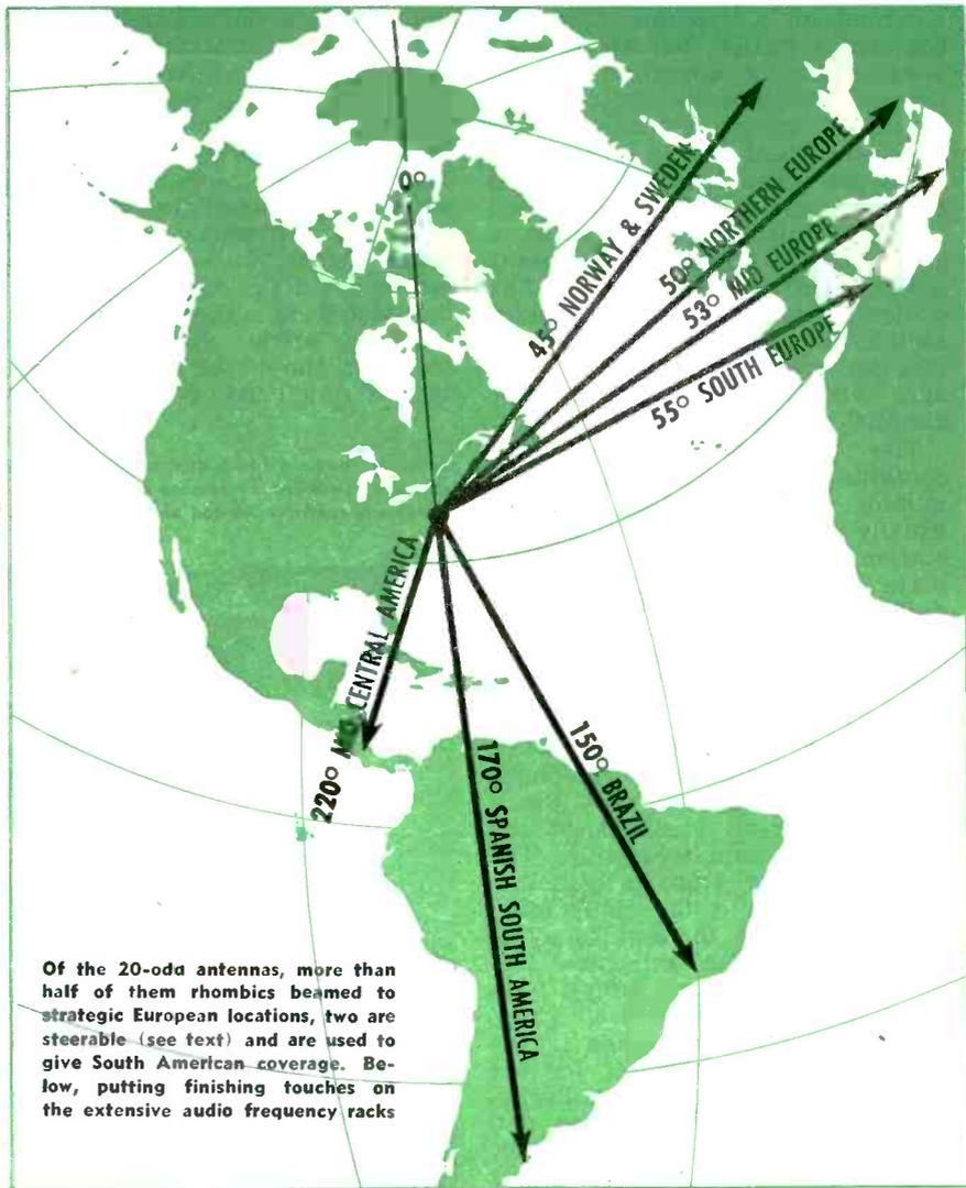
Of the 20-odd antennas, more than half of them rhombics beamed to strategic European locations, two are steerable (see text) and are used to give South American coverage. Below, putting finishing touches on the extensive audio frequency racks
