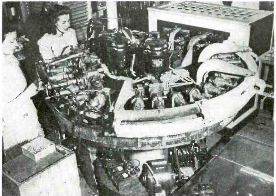
Fig. 3—The automatic exhaust machine (original with Sonotone) controls the evacuating and degassing processes and then seals up the tube. Fig. 4—(below) Effect of a scale size reduction on operating characteristics of tubes
