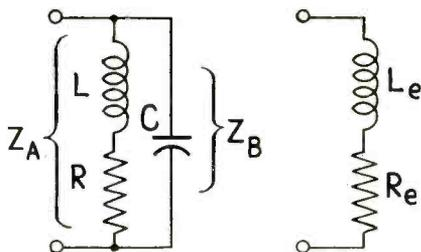
Figs. 1 and 2—Equivalent networks that a resistor introduces in high frequency circuits
