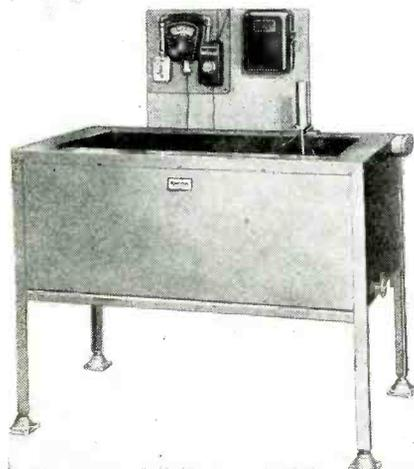
fast, efficient and economical wax coating of coils, resistors, condensers, panels and other electrical parts. This unit can also be used to wax-coat wrapped packages. Electrically heated by low density type strap-on heating elements, the bath temperature is automatically controlled by adjustable thermostats fitted with dial thermometers. The bath temperature can be adjusted from 100 deg. to 550 deg.
