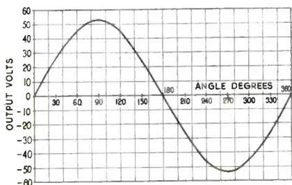
Fig. 7—Output characteristics of one of phase windings for the Kollsman type 787-01 rotatable transformer with an input of 32 volts
