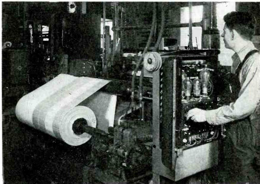
Photoelectric control regulating the feed of a roll of printed labels passing through a slitting operation in a Western label plant
