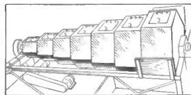
Tubes are put into the various sized angular chambers and tumbled. The larger the chamber the greater the shock. Thus the amount of abuse each tube will withstand is determined, giving our engineers accurate data for design and construction improvements.
