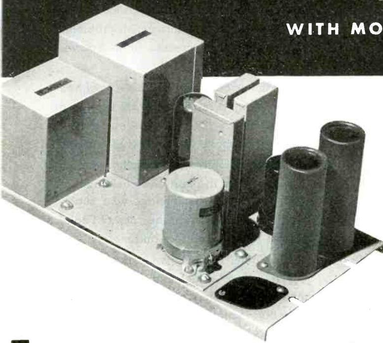
TYPE 102-A—Two stage—Fixed gain 55 db. Input impedance 30, 250 or 600 ohms; output impedance 600 ohms. Frequency response 30-16,000 Cycles  $\pm$  .5 db. Power output  $\pm$  26 VU with less than 1% harmonic content. Requires external power supply 275 Volts DC 30 M.A., and 6.3 Volts AC .75 Amps. When a 102 Series Amplifier is used in conjunction with a 101 Series Amplifier, the latter is capable of supplying the necessary power.
