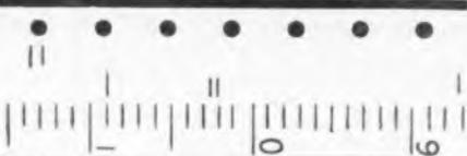
The tape is graduated in hundredths of a minute — Values accurate to .0025 minutes are read easily and directly.
