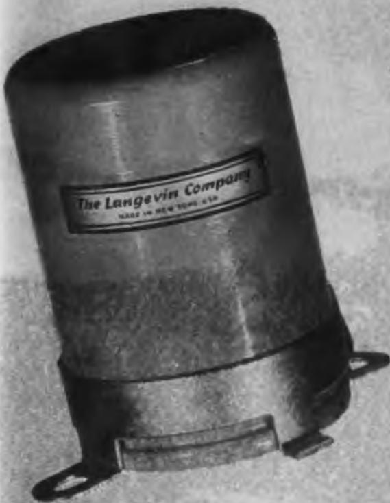
**D**esigned to occupy minimum space with excellent frequency response, the 400 Series Input Transformers are intended for high quality amplifier requirements. Combines high permeability shield with rotatable strap mounting for minimum stray field pick-up. Equipped with 10" Surprenant color-coded leads. 2" center to center mounting, 1 1/2" O.D. x 2 1/4" high. Baked gray enamel finish. Available for immediate delivery.
