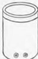
**APPARATUS ENCLOSED SOLDER-SEAL BUSHING**—combination insulator, cover and terminal board—has a hollow construction which permits placing small devices inside.
