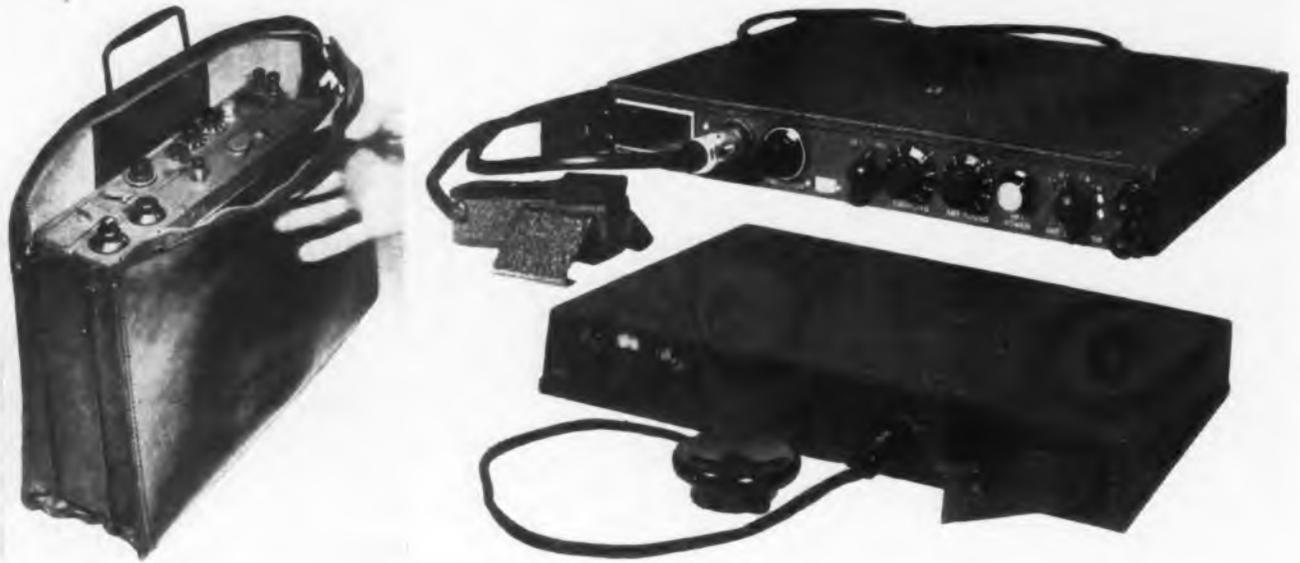
Relative size of the equipment and the reason for its designation as a "Brief Case" set become apparent from these pictures which show the extremely compact construction of transmitter and receiver, shown separately at the right and packed together in a brief case of ordinary dimensions
