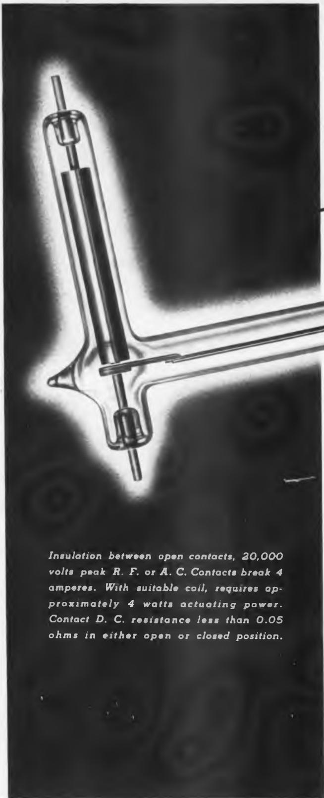
*Insulation between open contacts, 20,000 volts peak R. F. or A. C. Contacts break 4 amperes. With suitable coil, requires approximately 4 watts actuating power. Contact D. C. resistance less than 0.05 ohms in either open or closed position.*
