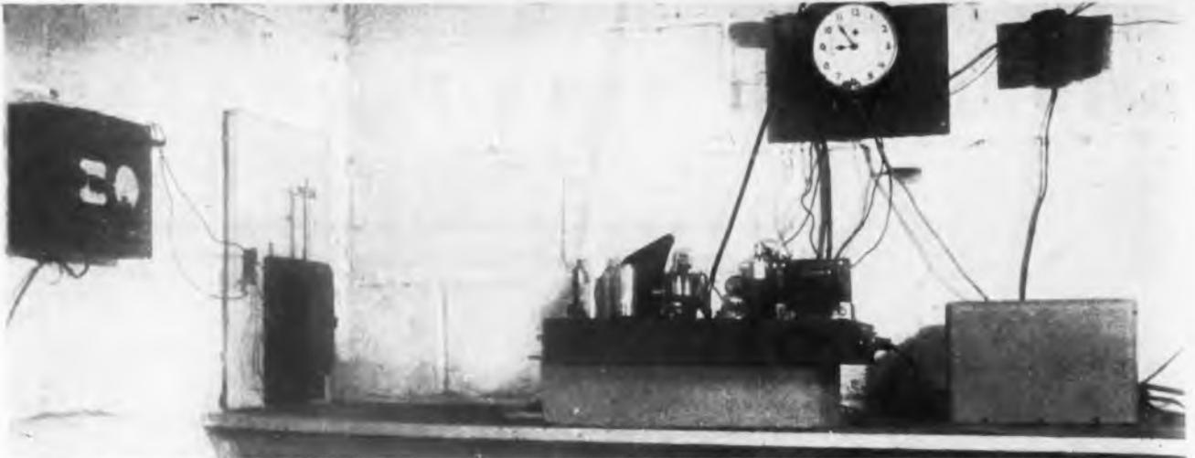
Earthquake recorder is set up in six by twelve foot room in basement of residence. Photo shows galvanometer, amplifier, voltage regulator and timer
