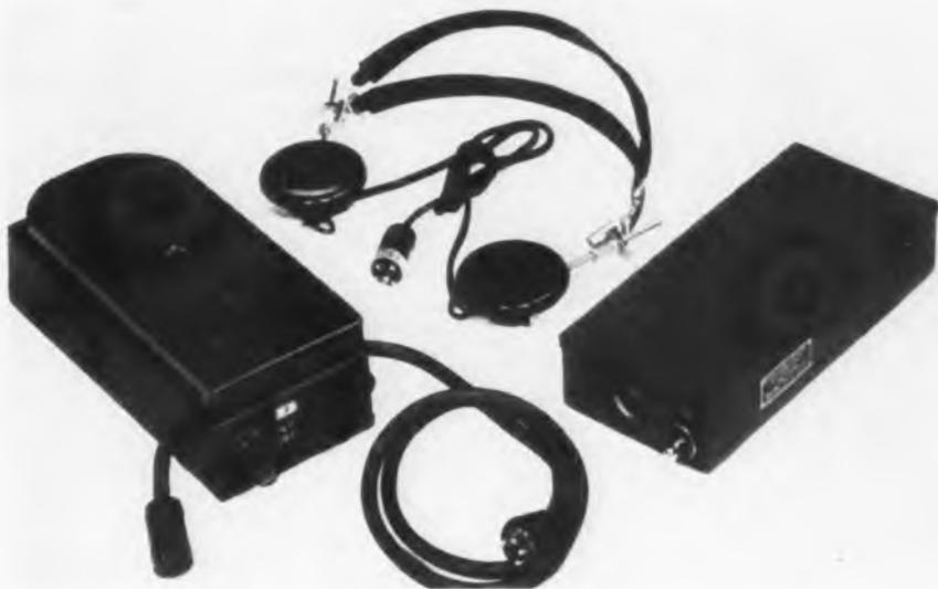
Two models originally were made, this being one of the first in which the battery was carried in a separate case that could be slipped into a slightly over-sized pocket. Note loop on receiver.
