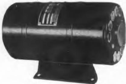
very high voltage without breakdown. It is possible to furnish the unit with two 1,500-volt, 0.05 ampere outputs, instead of the 3,000-volt one. Because of the high voltage and the tendency towards sparks and corona effects, the ends of the unit, where the brushes are located, are enclosed in explosion-proof covers enabling the use of the unit in gaseous locations such as near airplane engines, in mines, and other similar positions.
