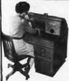
**NEW COMPACT, G.E. ELECTRON MICROSCOPE** distinguishes objects as small as 1/1,000,000th of an inch...magnifies them up to 5,000 or 10,000 times actual size. Photographic enlargements are wanted. Photos can be made to show objects at 100,000 times their true size. Can be plugged into a regular 110-volt A.C. line.
