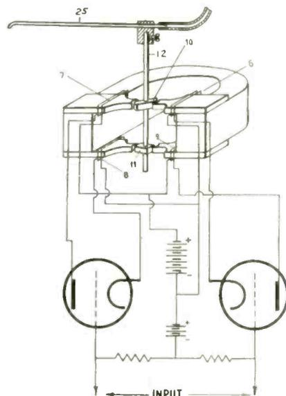
trols the current through coils 6, 7, 8, 9 which in turn modifies the magnetic flux in the gaps. Consequently, if an alternating voltage is applied, the shaft 12 will oscillate back and forth at a frequency equal to the applied frequency and at an amplitude proportional to the amplitude of the applied voltage.
