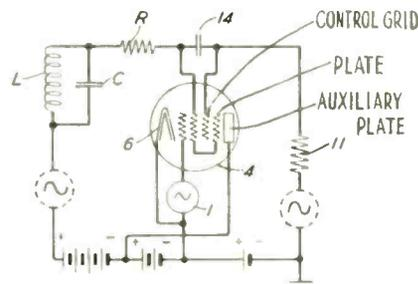
tor 14 and will cause it to be less negative; plate current will decrease to a minimum. The tube will then discharge the electric charge on capacitor C and another cycle will start.
