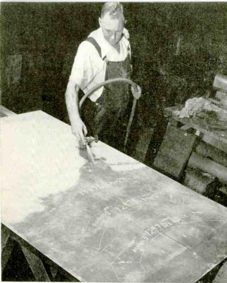
**1**—Flat metal work is speeded up by Eastman Kodak Co., Rochester, N. Y. Kodak Layout Paint is sprayed on. Black ink drawing is photo-printed on metal by exposure to arc or mercury vapor lights. Print is "developed" by warm, weak, ammonia water and washed
