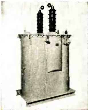
Single phase, half wave rectifier plate transformer, 60 cycles, 220 volts primary, 110,000 volts secondary.
