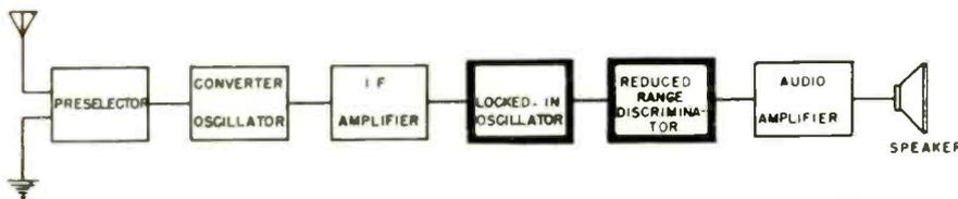
Fig. 1—Block diagram showing the arrangement of locked-in oscillator and discriminator units
