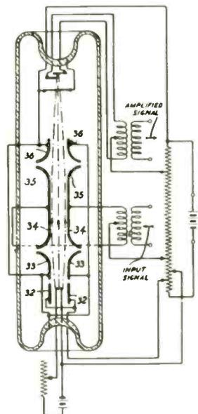
the plates as shown in the drawing. The adjacent portions of each pair of plates 33, 34 and 35, 36, respectively, are flared outwardly; an abrupt flare is required.
