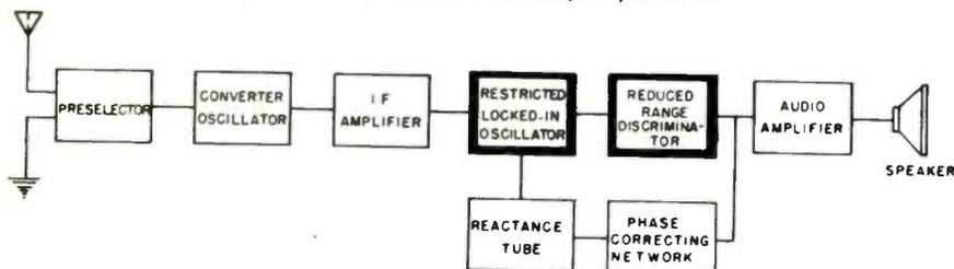
Fig. 5—Modification of a receiver to include the locked-in oscillator and reduced range discriminator as well as a reactance tube and phase correcting network indicated that such an arrangement provided superior noise reducing and adjacent channel selectivity
