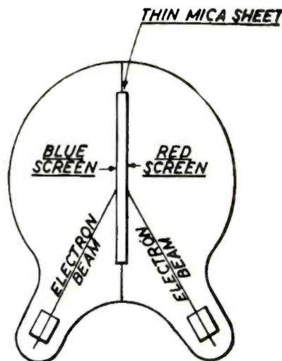
Fig. 1—Diagram of double screen cathode ray tube for viewing television images in two colors
