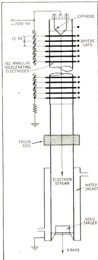
At left, R. R. Machlett, president of Machlett Labs., holds new 2000 kv X-ray tube. Cathode end is at top and water jacketed target at bottom. At right is outline of accelerating column, focus coil, target and water jacket. X-rays are transmitted directly through target
