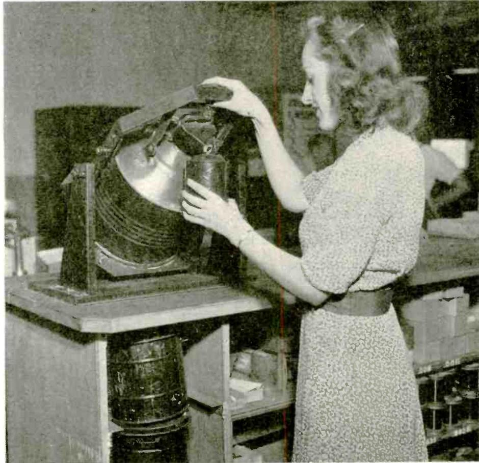
10—Idea for handling inflammable or corrosive solvents eliminates manual lifting, promotes safety, and speeds entire process of filling girls' individual containers at a Westinghouse plant. The safety can-tilting stand incorporates lever to pull stopper automatically
