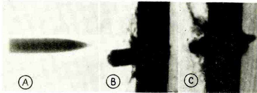
Fig. 4—High speed X-ray picture of bullet piercing armor plate. (A) Stationary X-ray picture of cal. .30 armor piercing bullet. (B) High speed X-ray picture of this bullet penetrating 1/2 in. thick armor. (C) High speed X-ray picture of same bullet 20 millionths of a second later
