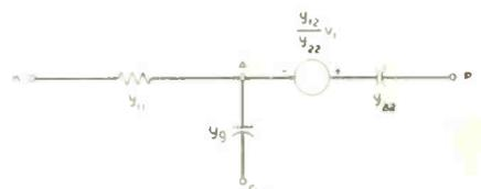
Fig. 6—Complete diagram of triode
