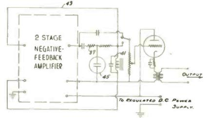
Lead 43 provides positive feedback for the oscillator. Current limiting resistance 37 is made sufficiently large compared to the low output impedance of the amplifier so that any variation in the resistance of the glow discharge tube during the cycle of operation does not affect the amplifier gain.
