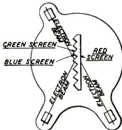
Fig. 2—Diagram of tube for television reproduction in three colors, the mica screen being stepped on one side as shown
