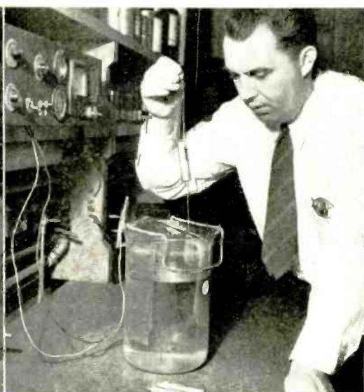
Experimental set-up for determining methods and procedure in developing rhodium plating processes
