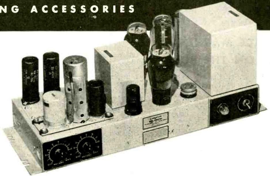
**TYPE 108-B** two-stage Amplifier provides transformer input impedances for either 30 or 250 ohms with nominal output impedance 500 or 8 ohms. Variable gain 65/105 db. with electronic volume control. Frequency response better than  $\pm 1$  db. 30/16,000 c.p.s. Power output +43 V.U. (20 watts) with less than 5% RMS harmonic content. Noise level full gain 56 db. below full output.
