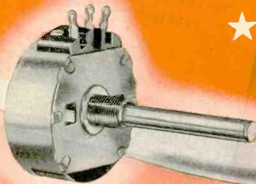
★ Chicago Telephone Supply Company now offers a new 1 5/8" diameter, wire wound variable resistor, 352 Series, with resistance value up to 20,000 ohms linear and with the same bakelite housing and grounded metal construction as the popular 1 1/4" 252 Series. This potentiometer may be used with switches attached and in tandem construction.
