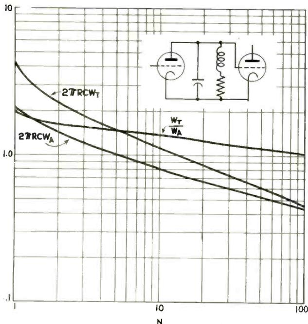
$W_A$ , as defined above, is the most useful single number measuring the amplitude response other definitions have been used. Probably the most common is the width to the  $g = .707$  point. It is fortunate that in almost all cases of practical interest the width to the 71 per cent point and  $W_A$  are only very slightly different. For example, for a number of RC coupled stages the difference is 6 per cent, for a number of shunt peaked stages .5 per cent, etc.
