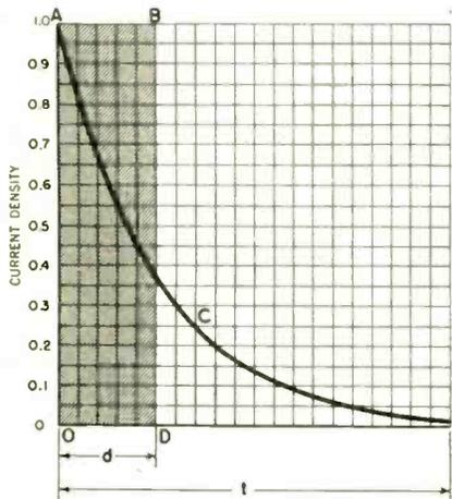
Fig. 3—Decay curve of current density distributed in sheet of conducting material
