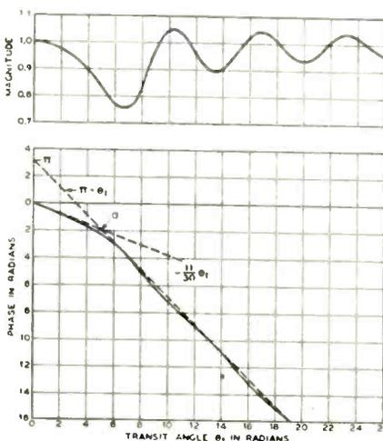
Fig. 8—Phase of transadmittance as function of  $\theta_1$
