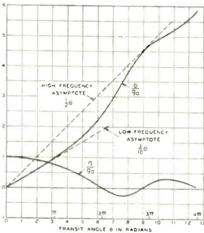
Fig. 3—Diode admittance with complete space charge
