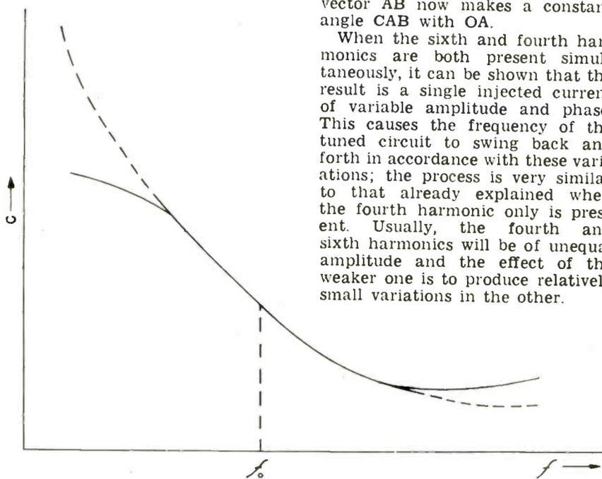
Fig. 4—Solid line is falling input capacitance of discriminator; dashed line is variation of capacitance needed to keep the oscillator in tune as the frequency is varied
