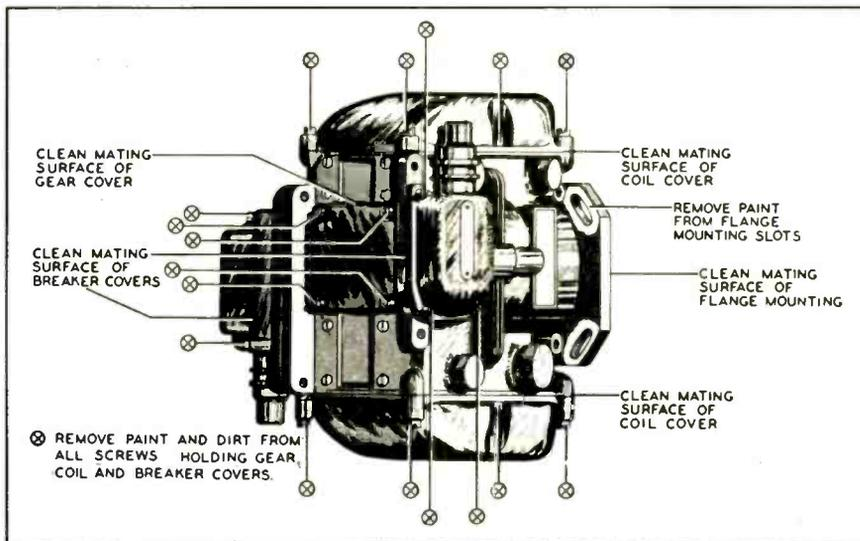
Fig. 6—Striking illustration of care necessary to insure "bottling up" VHF ignition noise. Note that all mating surfaces must make perfect contact. Paint on screws or flanges is fatal
