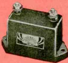
**TYPE 6** Medium Power Mica Transmitter Capacitor. Designed for a wide variety of r. f. applications where size and weight must be kept to a minimum. Patented series mica construction; vacuum impregnated—resulting in low loss, high insulation—no air voids; special low-loss filler reduces stray losses.
