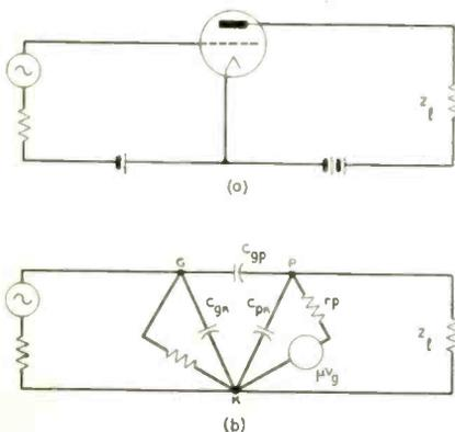
Fig. 1—Conventional representation of vacuum tube network
