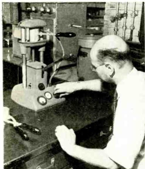
Mounting a specimen of iron powder in a suitable resin for subsequent examination
