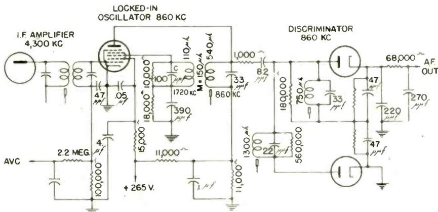
Fig. 2—The local oscillator is locked-in with and modulated by the received signal at one-fifth the intermediate frequency. The discriminator is designed for the reduced frequency
