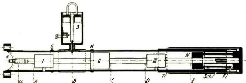
Wavemeter for 140 mm. waves detects changes of 0.0007 mm.
