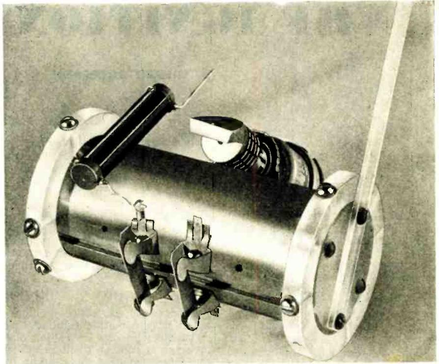
Cylindrical circuit covering the frequency range from 10 to 500 megacycles in four bands. The two strips between the contacts form the highest frequency "coil"
