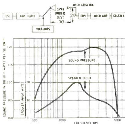
Fig. 5—Sound pressure/frequency curve for one style of unit designed for PA work. Pressure measured with input voltage constant with measured distortion at 1 kc was 12%
