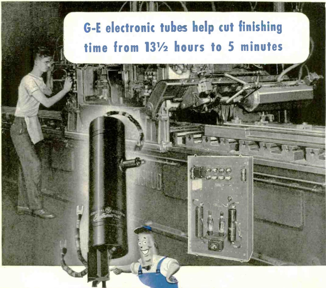
The G-E all-metal thyatron tube is the "heart" of the Thy-mo-trol unit that maintains correct machine speed for every load.
