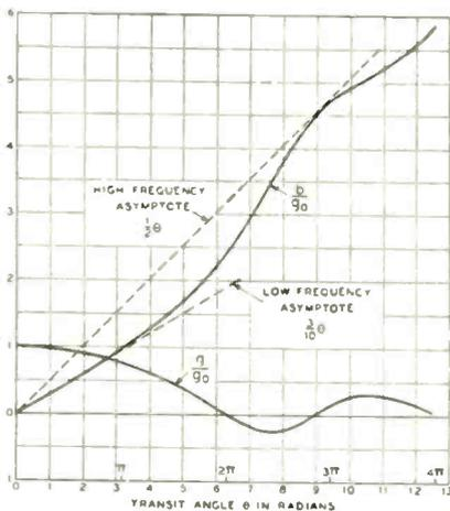
Fig. 3—Diode admittance with complete space charge
