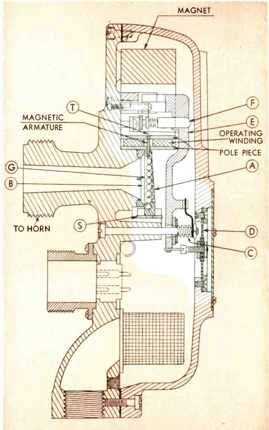
Fig. 3—Cross-sectional view of Dilks fluid flow unit. The automatic adjustment-stabilizing arrangement is shown in the white central section
