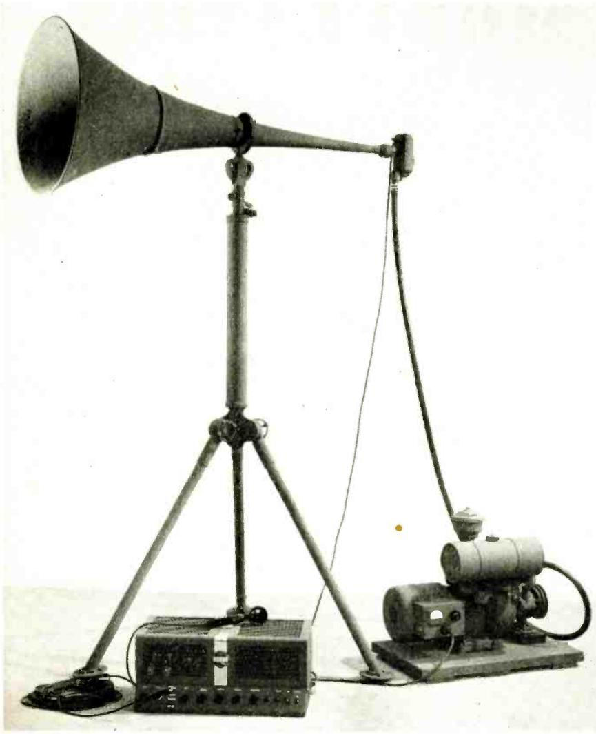
Portable units are operated by either electric or gas engine drives. Fig. 4 shows a form of the latter, with source of power for amplifier and air compressor mounted integrally on the gasoline engine base, Fig. 5
