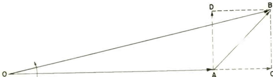
Fig. 3—Vector diagram showing phase relationship when the oscillator locks in with the incoming signal; vector AB then makes a constant angle CAB with OA
