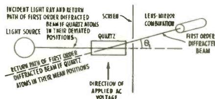
Measuring light velocity with ultrasonic diffraction grating
