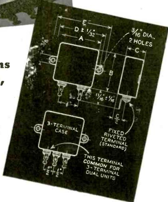
metal case with soldered bottom plate. Terminals are constructed with the Aerovox-originated "double-rubber" bakelite insulators permanently riveted to the case, making a sturdy, absolutely immersion-proof assembly. Terminals on side, top, bottom or ends to suit mounting and wiring requirements.
