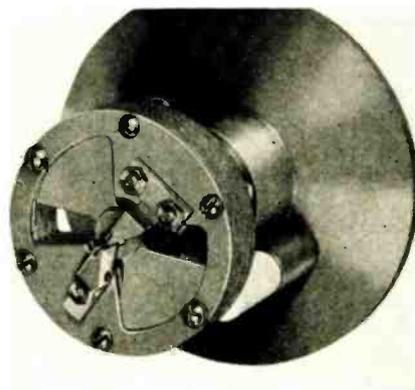
stator sections. These devices can be designed with a wide variety of characteristics, and with tuning ranges as high as 12:1 and with Q values of 300-650. Another form of tuning arrangement found of value is the cylindrical circuit also shown. A special shaped split cylinder rotates inside to produce the tuning variations.
