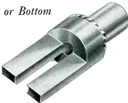
A .050" hole through the shaft permits wiring from top or bottom side of the terminal board without time lost drilling holes. They're firmly anchored and swiftly set by a simple swaging operation. Knurling at base of Lug prevents twisting or turning.
