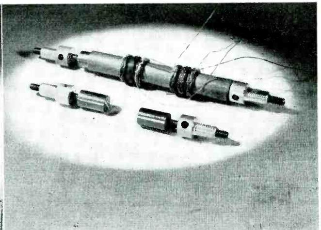
coils. In the case of if transformers where permeability tuning is substituted for the usual capacity tuning, the iron-core unit is cheaper than the air-dielectric type, much more stable than the compression mica condenser, and provides higher gain and selectivity. In single-tuned or untuned if transformers, iron cores can be used to increase the coefficient of coupling.
