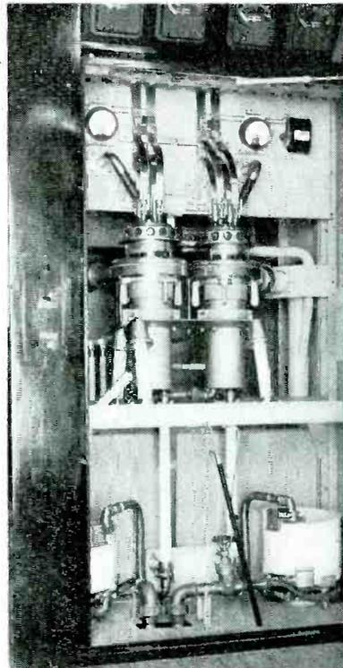
Back of the RCA 150 kw electronic power generator, which puts out 150 kw at 400 kc or 125 kw at 13.7 mc, and (right) a side view of the generator arranged for 27.4 mc
