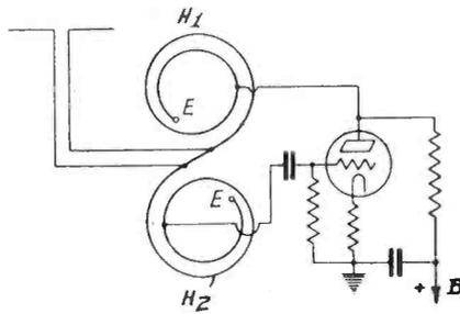
The figure shows two ribbons  $H_1$  and  $H_2$  connected in series in a balanced transmitter or receiver. To provide tuning facilities, the ends E of the ribbon may be adjusted by a winch, screw or cord for altering the space between the turns of the spiral and changing its distributed capacitance.
