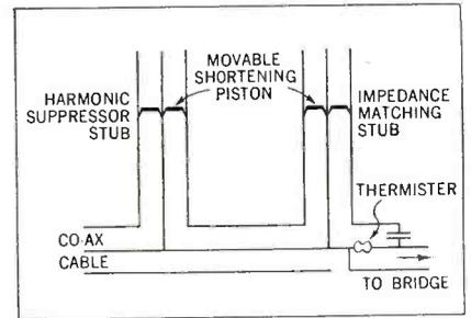
Fig. 5. Application of bridge to coaxial cable output. Stubs used to eliminate harmonics
