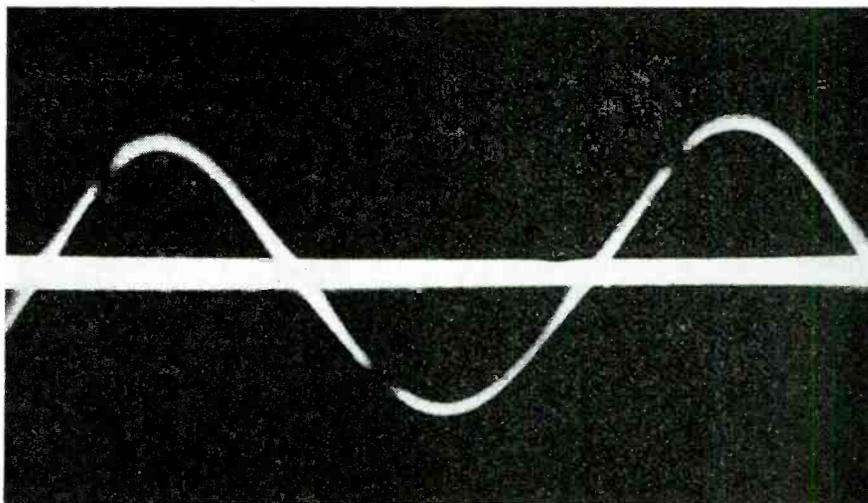
Fig. 7. Oscillogram of 1000 cycle 1500 amp. current in induction heating load coil of mercury arc converter. Resonant condition in load circuit produces sine wave output from shock excitation produced by block waves from tubes
