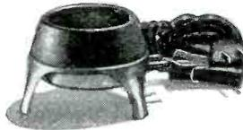
Available in two sizes—Model 200 with 1¾ pound capacity and Model 250 for 2 pound melts. They are particularly adapted to tinning small wires and leads, and similar operations. A single-heat, porcelain nickel-chrome heating element heats the pot. Element can be quickly and inexpensively replaced when necessary. Can be had for 220 V. operation. Low Cost! Economical! Efficient!
