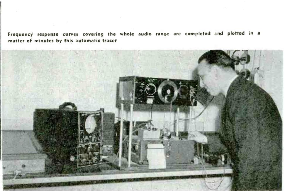
Frequency response curves covering the whole audio range are completed and plotted in a matter of minutes by this automatic tracer
