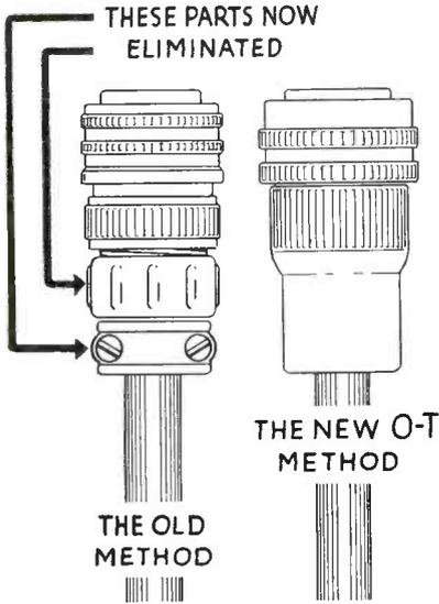
Assembly time and number of parts cut to a minimum by new simple compression type.
