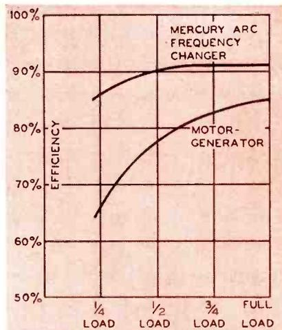
Fig. 6. Efficiency comparison between mercury arc and motor generator high frequency equipment. Mechanical windage losses reduce efficiency of MG sets at low output
