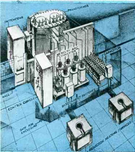
Fig. 1. At left is sketch of typical frequency converter installation of the Mercury Arc type
