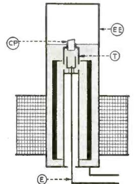
ENERGIZED—Mercury now fills thimble T, is completely leveled off and mercury-to-mercury contact established between electrodes E and EE. Degree of porosity of ceramic plug CP determines length of time delay.
