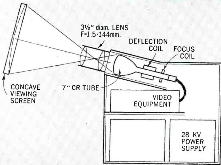
Fig. 1. Cross section and working model of television receiver. The image is projected on concave viewing screen by lens system
