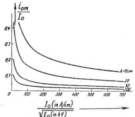
Fig. 3. Maximum efficiency of fundamental wave; modulating index is 0.1
