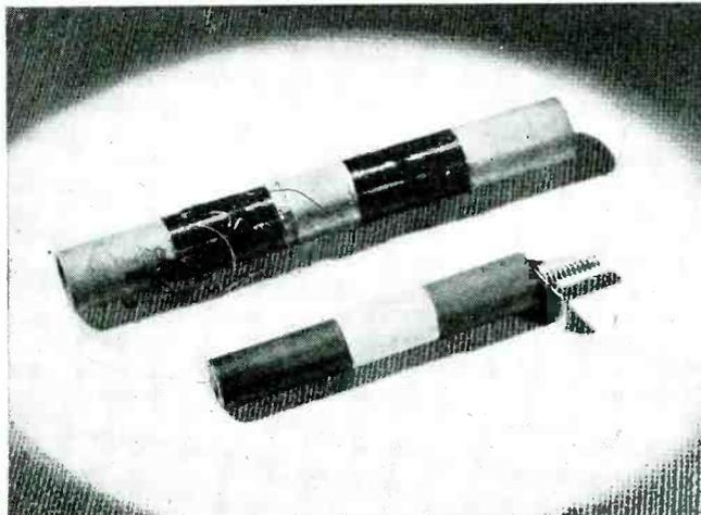
Typical multi-pi iron if transformer. Each core is adjustable in its winding by means of the extended screws
