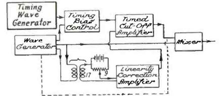
The timed cut-off amplifier is introduced to permit correction of the sawtooth wave only during the major portion of the rising wave; obviously no linearity control is to be introduced close to the minimum and maximum values of a sawtooth wave. The timing bias control provides suitable interruption of the timed cut-off circuit; it may be operated by the wave generator or by an additional timing wave generator synchronized with the wave generator.
