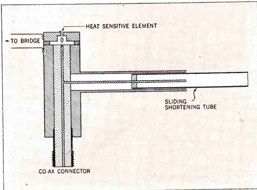
In order to avoid reflections, the Thermister must be placed in a mount which can be matched to the wave guide so that there is no change of surge impedance at the junction point.
