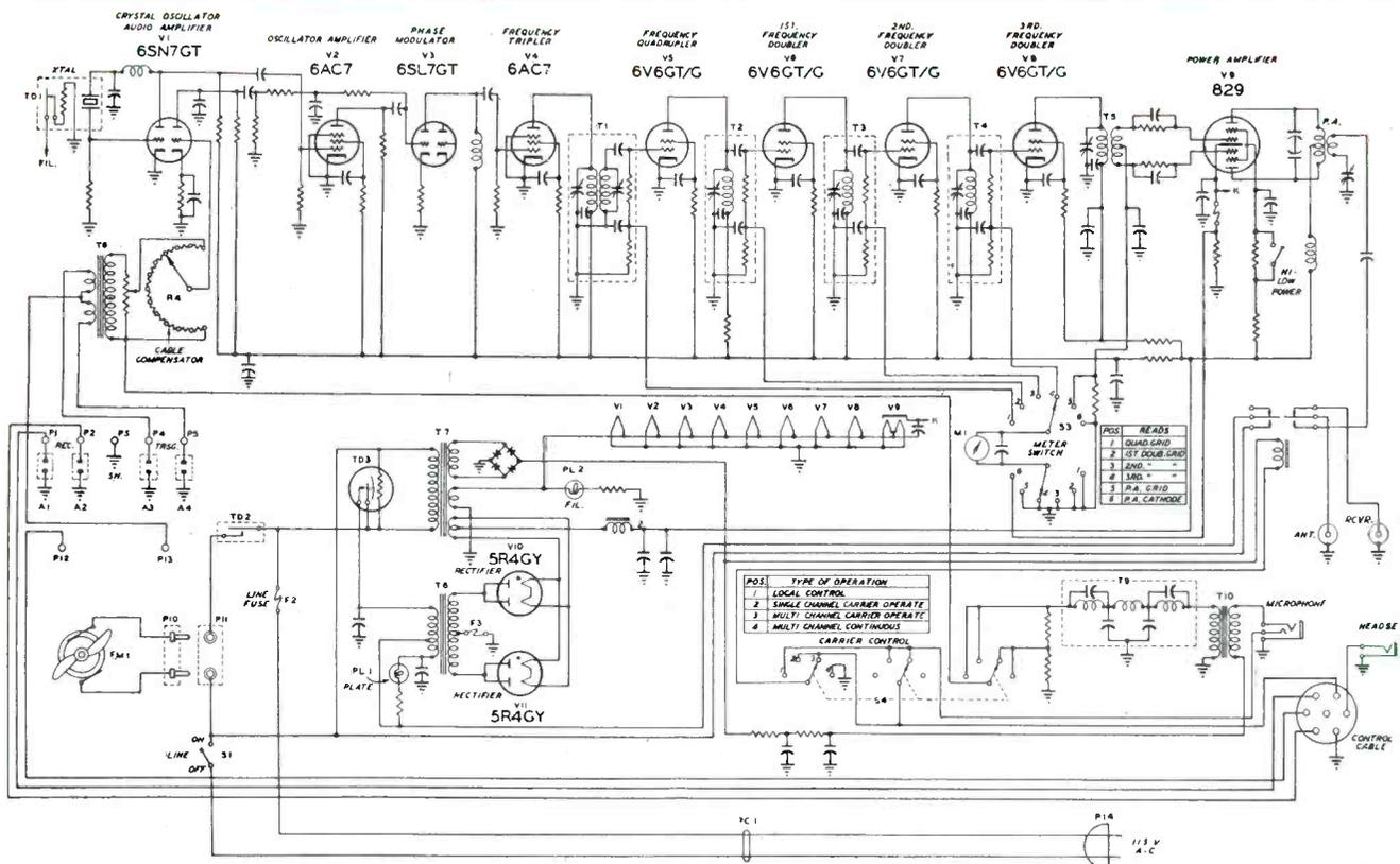
Circuit diagram of transmitter. Balanced push-pull output used with 829 power tubes. High-low switch limits power to permit tuning without damage by lowering the screen voltage. Spiral-four cable connections are p1 to p3.
