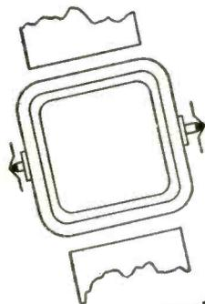
External pivots (above)—used in the design of DeJur 1½" Meters—provide greater accuracy in mounting the moving element between the jewel bearings. For this reason internal pivots (below) are not used in DeJur meters.
