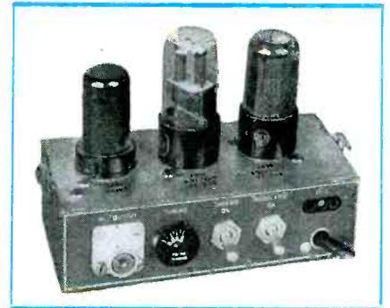
The oscillator (without cover) tunes receiving sets for any desired frequency
