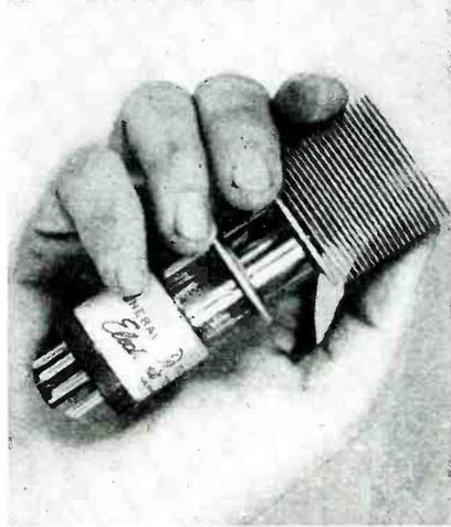
Disc seal transmitting tube used in shf range. Cooling fins increase power
