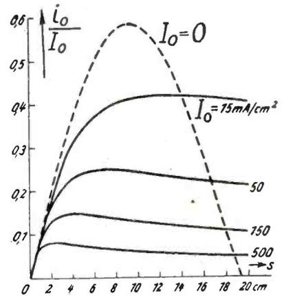
Fig. 2. Relative amplitude of fundamental as function of distance from modulating grids
