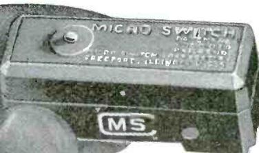
The basic switch is a thumb-size, feather-light, plastic enclosed, precision, snap-action switch. Underwriters' listed and rated at 1200 V.A., at 125 to 460 volts a-c. Capacity on d-c depends on load characteristics. Accurate reproducibility of performance is maintained over millions of operations. Basic switches of different characteristics are combined with various actuators and metal housings to meet a wide range of requirements.
