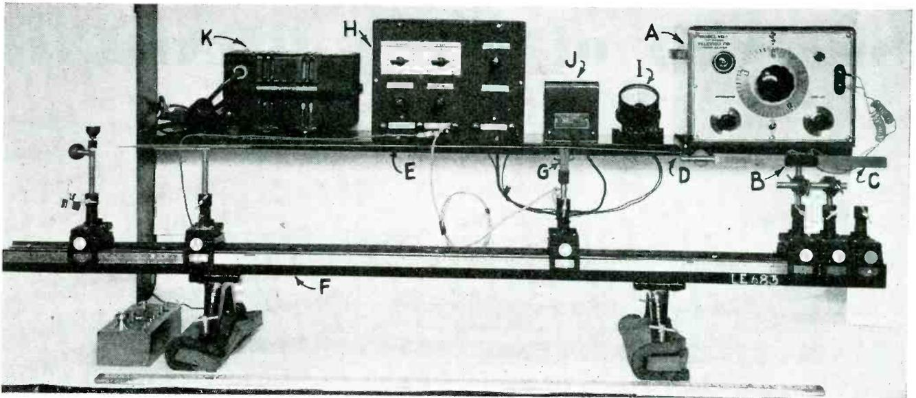
Apparatus used for determining Young's modulus of elasticity for fibers and sounds by velocity measurements. (A) audio oscillator; (B) rochelle salt crystal; (C) steel resonating bar; (D) yarn clamp; (E) yarn sample; (F) optical bench mounting; (G) crystal pickup; (H) amplifier; (I) out-put meter; (J) filter to remove 60 cycle from I; (K) voltage regulating transformer for power supply
