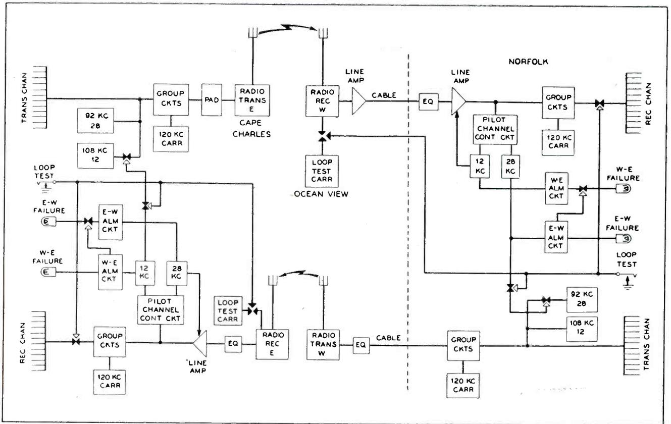
Block diagram of the Cape Charles to Ocean view relay link now in use for two way transmission of 12 simultaneous messages. System operates at 156.3 and 160.65 mc. Proposed radio relays will use FM and much higher frequencies
