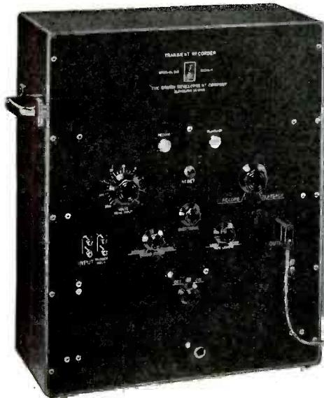
Brush Transient Recorder with oscilloscope. (Any good quality oscilloscope with low-frequency sweep may be used.)
