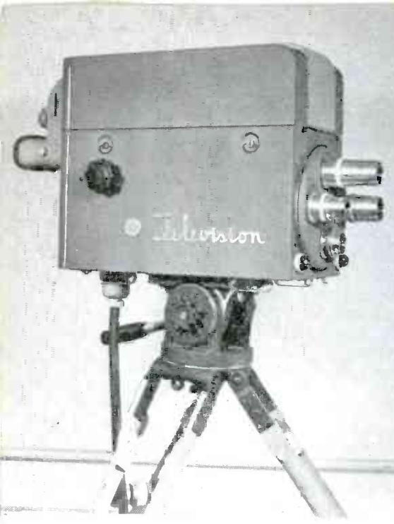
Close-up of the new RCA model TK-30A Image Orthicon camera which carries four lenses in a turret. Below, addition of telephoto
