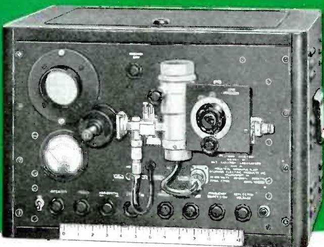
The Sylvania Spectrum Analyzer offers a convenient means of studying the energy spectrum of microwave generators operating as pulsed oscillators or modulated or unmodulated C. W. oscillators. The output of magnetron, klystron, rocket and similar UHF and SHF tubes can be conveniently investigated.
