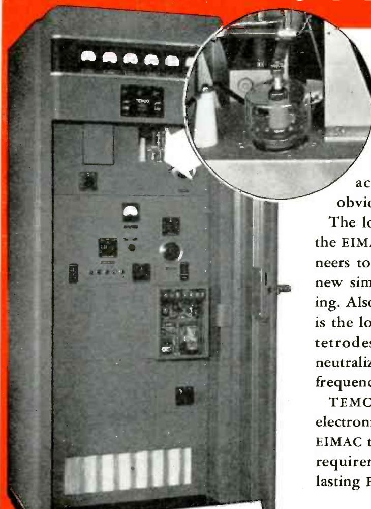
In the power amplifier of the 1000-GA transmitter, TEMCO employs two EIMAC 4-250A tetrodes to obtain a kilowatt input on CW and high level modulated radio telephone. The characteristics of this tube make it the obvious choice for this assignment.
