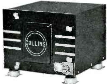
**THE 180K-1** antenna loading unit efficiently transfers the power output from the 18S-1 to any standard commercial fixed antenna. Remote controlled, pretuned operation for ten channels is provided. The nominal input impedance is 50 ohms. Weight, 10 lbs. Size,  $7\frac{1}{2}$ " h,  $10\frac{1}{2}$ " d, 12" l.
