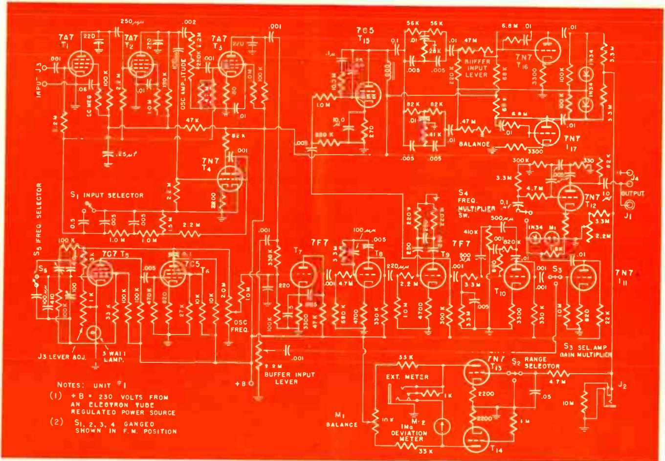
Above shows schematic of the pitch perceptor and below is the low frequency voltmeter and wave analyzer circuit
