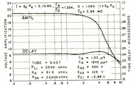
Fig. 3: Theoretical curves of compensation characteristics. See text for full details
