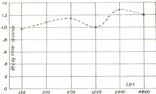
Decay time over frequency range at one pair of speaker-microphone positions. Each point is decay average at that frequency
