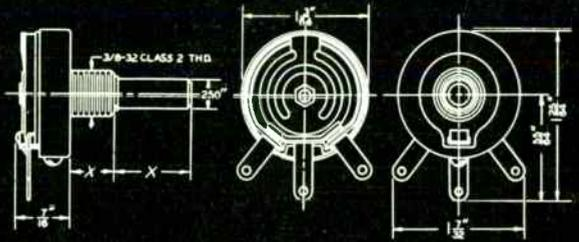
TYPE C IS A SMALL 2 WATT UNIT, USED AS A METER COMPENSATOR, MINIATURE MOTOR CONTROL AND LIGHT DIMMER.
