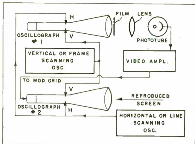
Fig. 2: Showing block diagram of the flying spot video-signal generator system for slide transparencies used in studio telecasting
