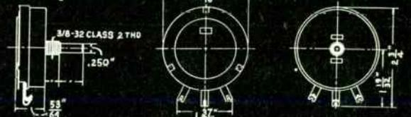
TYPE E, RATED AT 7 WATTS, IS WIDELY USED IN PRECISION INSTRUMENTS, RESISTANCE BRIDGES AND OTHER CIRCUITS REQUIRING ACCURATE SETTINGS.
