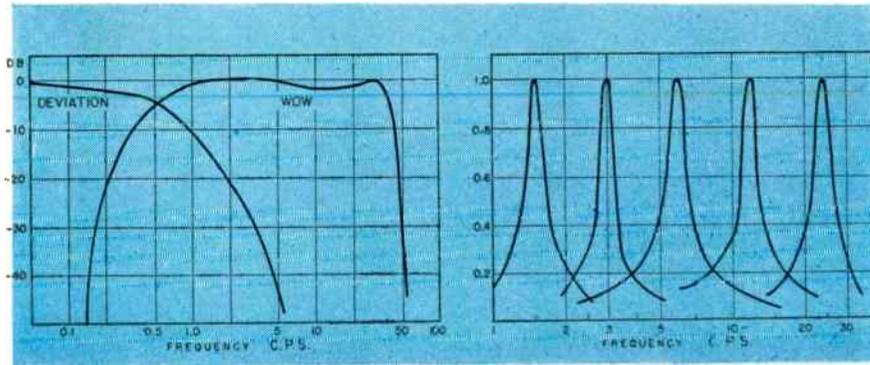
Fig. 1: Showing wow and deviation circuit responses recorded by equipment used with Esterline-Angus recording milliammeters
