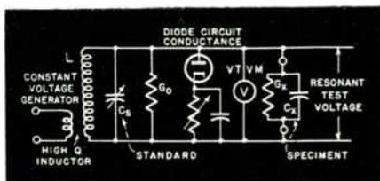
Fig. 1: Basic measuring circuit. Here,  $G_0$  represents the diode circuit conductance
