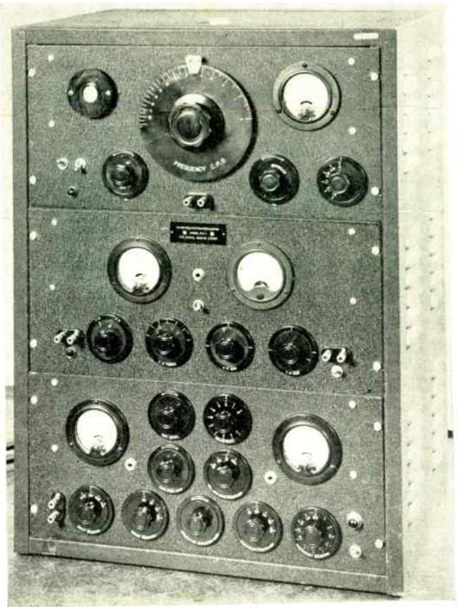
Photo shows rack with beat oscillator at top; center unit takes signal through discriminator; voltmeter and analyzer at bottom
