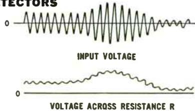
Used to good advantage as second detectors at frequencies to over 60 mc. They have much lower impedance than vacuum tube diodes, and are particularly effective in low-impedance circuits. The 1N47 is tested for operation at 100 mc.
