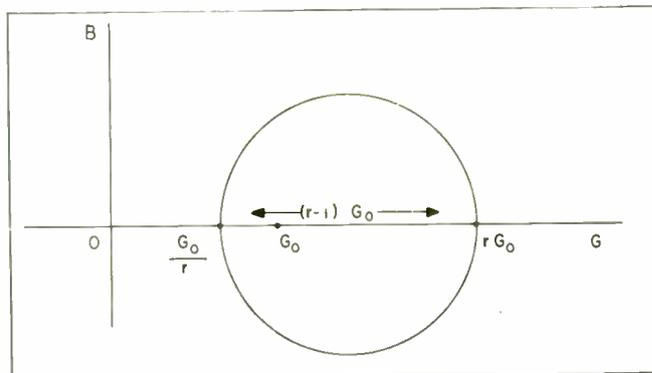
Fig. 6: This drawing illustrates the admittance variation with the change in position of the standing wave minimum
