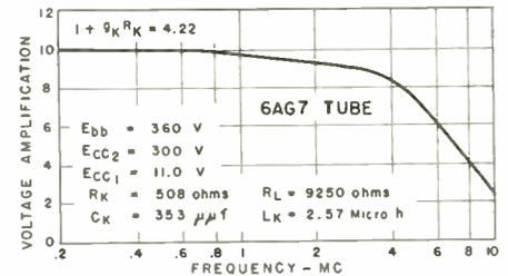
Fig. 4: Compensation curve of amplifier indicates good input and output linearity
