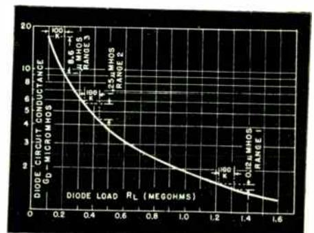
Fig. 5: Diode circuit conductance curve with selected operating range points indicated
