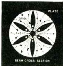
**SYMMETRY OF DESIGN** . . . enables manufacture of a mechanically rugged tetrode, with self-supporting internal elements. Gassy, inactive, internal insulators, shields and ineffective portions of the elements are eliminated.
