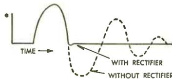
Unit damps out the oscillation after one-half cycle, producing a single pulse shaped similarly to half of a sine wave. This pulse may be clipped, provided clipper is isolated from pulse-producing tuned circuit to prevent damping out desired half cycle.
