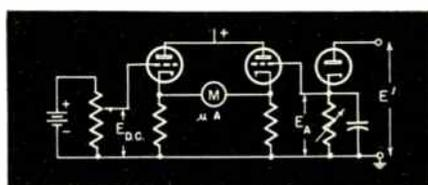
Fig. 2: Diagram of differential voltmeter. DC load voltage  $E_A$  is balanced by  $E_{D.C.}$  The
