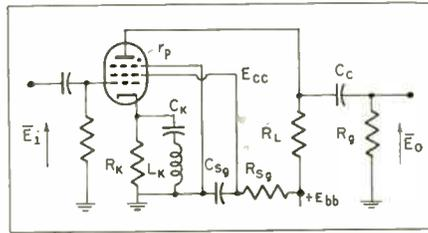
Fig. 1: Basic video amplifier stage with cathode compensation for high frequency loss
