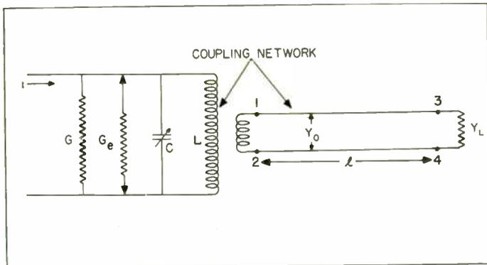
Fig. 5: In equivalent circuit of loaded oscillator,  $G_c$  is equivalent conductance coupled into oscillator circuit
