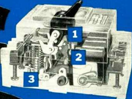
**1.** The HIGH SPEED LATCH operates with minimum friction and maximum speed. It functions only under overload or short circuit conditions, but it does that even if the handle is held in the "ON" position during overload. The rotation of the latch releases contacts which are under heavy spring pressure.
