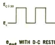
Circuit shows d-c restorer applied to a network widely used for coupling successive amplifier stages. The germanium crystal prevents output voltage from swinging below  $E_C$ ; thus negative peak of wave is established at  $E_C$ .
