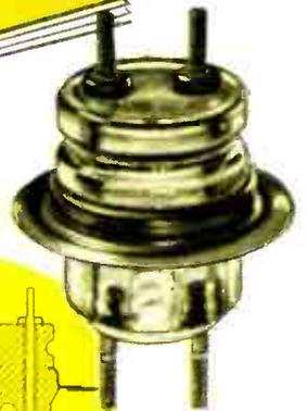
Glass bushings are currently available to meet dry, 60-cycle, flashover values of from 10 to 50 kv, and in current ratings of 25 and 50 amperes (large sizes up to 800 amperes). They may be single or multi-conductor and can be provided with a top flange to permit mounting tube sockets directly on the bushings. Diameters range from 1 1/8 to 3 3/8 inches and weight from 2 1/2 oz. to 4 lb.
