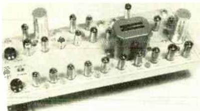
and at transmitters as a picture line amplifier, or as an amplifier for remote line and radio relay links. It will remove low-frequency interference from the signal, stretch and clip supersync, and restore DC to improve low-frequency response. A signal as small as 0.2 volt, peak to peak, can be raised to a standard picture line signal of 2 volts. The unit is mounted on an aluminum relay rack chassis, 7-in. wide, which fits into a standard 19-in. relay rack.—General Electric Co., Syracuse, N. Y.
