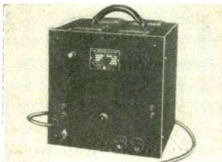
the 1E51002, the regulator measures approximately 11½ x 11½ x 10¼-in. and is fitted with carrying handles. It is rated at 95 to 135 volt input and its output is adjustable between 110 and 120 volts. The load power factor range is 0.5 lagging to 0.9 leading; waveform distortion is claimed never to exceed 3%.—**Superior Electric Co., Bristol, Conn.**
