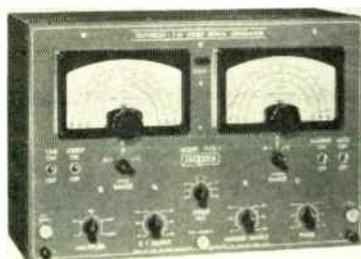
graph for visual alignment of television or FM radios. It provides a complete range of frequencies for the alignment of RF, oscillator, IF and trap circuits. Sweep frequencies are from 2 to 216 MC in 3 convenient ranges, all on fundamentals. Sweep width is adjustable from 100 KC to 12 MC bandwidth, ample width for the alignment of badly detuned circuits.—**Jackson Electrical Instrument Co., 18 South Patterson Blvd., Dayton 1, Ohio.**
