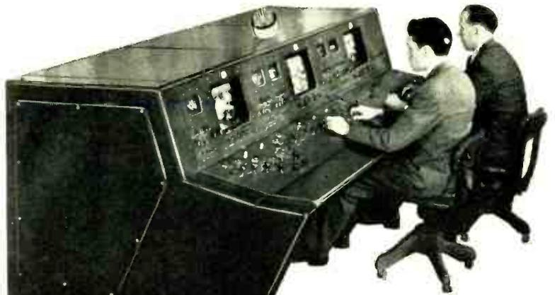
Du Mont Type TA-105-A Film Pickup Control Console. Includes saw-tooth, parabola and sine-wave shading with 5" waveform monitors for both line and frame. 12" picture monitor. Instantly accessible chassis. Integral design with the Du Mont Type TA-108-B Video Mixing Console and associated equipment which will handle four separate video or composite input channels with automatic or manual "fades" and "lap dissolves" between any video input channels.
