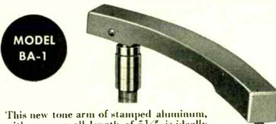
This new tone arm of stamped aluminum, with an over-all length of 5 $\frac{1}{2}$ ", is ideally suited for use on player units designed for playing the new 7" records, either 33 $\frac{1}{3}$  or 45 RPM. It incorporates the model A-1 miniature cartridge exerting a tracking pressure of only 7 grams without use of spring counterbalance.
