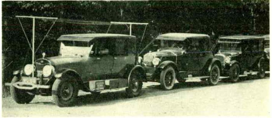
The 50-watt broadcast transmitter carried on the first car was assigned call-letters WGMU and operated on 63 meters. It was used as a remote pickup for the old Grebe station WAHG, in Richmond Hill, L. I., N. Y. Also designed by Ralph R. Batcher, author of the nostalgic article on preceding pages, was the receiving installation on Batcher's own car, second in the line, which used as antenna a four-turn loop surrounding the car.
