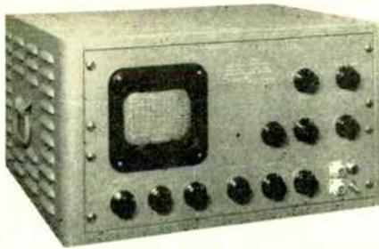
Incorporating completely new design features — such as continuously variable resolution and variable scanning rates—the SB-8 and SA-8 enable highly detailed analysis of signals extremely close in frequency, yet offer all the time saving advantages of wide scan Panoramic displays.
