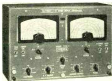
graph for visual alignment of television or FM radios. It provides a complete range of frequencies for the alignment of RF, oscillator, IF and trap circuits. Sweep frequencies are from 2 to 216 MC in 3 convenient ranges, all on fundamentals. Sweep width is adjustable from 100 KC to 12 MC bandwidth, ample width for the alignment of badly detuned circuits.—**Jackson Electrical Instrument Co., 18 South Patterson Blvd., Dayton 1, Ohio.**
