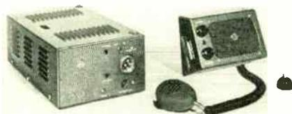
possible by the highly selective circuits which are part of the new RCA Carfone. The complete transmitter-receiver is contained in a single metal-shielded unit only slightly larger than a shoebox. Frequency range is between 152 and 174 MC. An automatic modulation control circuit locks the voice input level at a constant amplitude.—RCA Victor Div., Radio Corporation of America, Camden, N. J.
