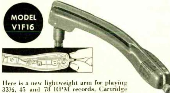
Here is a new lightweight arm for playing 33 $\frac{1}{3}$ , 45 and 78 RPM records. Cartridge rotates 180° to present the proper needle for standard or long-playing records, and locks in position. Tracking pressure is 7 grams in either position. The illustration shows method of turning cartridge.
