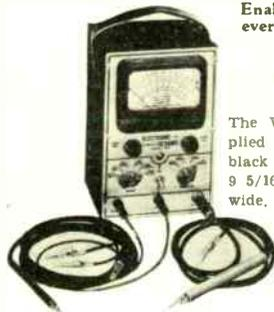
Enables laboratory engineers and radio service technicians to measure every voltage required in the design laboratory and radio servicing.
