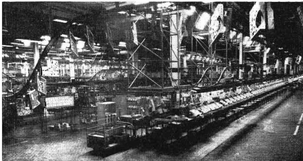
Starting point for the three main assembly lines. Overhead conveyor carries chassis from sub-assembly area where tube sockets and terminal strips are riveted into place
