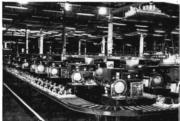
Alignment and Testing area. Generators providing test signals to stations are centrally located in air-conditioned room
