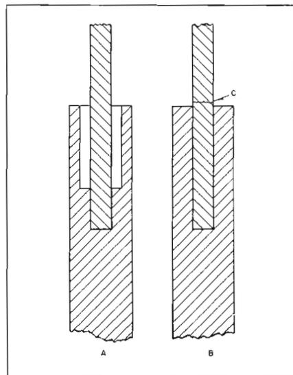
Fig. 9: Diagram showing filament-to-filament support junctions. (A) illustrates present and (B) illustrates previous constructions
