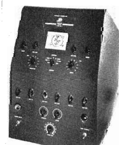
cast transmitter, an RF TV signal generator or for direct test of video portions of TV equipment. This model includes the following circuit units: monoscope sweeps; video pre-amplifier and mixer amplifier; monoscope and CR blanking; CR monitor sweeps; video and switching; regulated power supply; high voltage power supply. Operation is from standard 115/120 v., 60 cycle line.—Television Projects, Inc., 3660 Coral Way, Miami 35, Florida.
