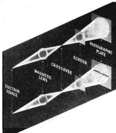
Left: Drawing showing the principle of electron-optical shadow measurement technique. In the upper illustration a magnetic lens converges an electron beam, forming a reduced image of original source at crossover point. This reduced image acts as a virtual source and produces an enlarged shadow image of the wire screen on the photographic plate.
