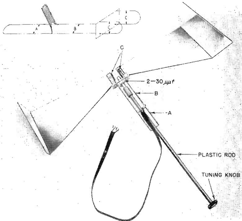
Fig. 1: Physical appearance of cabinet antenna. Details of coil structure at upper left
