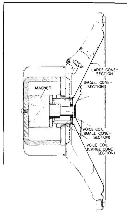
Fig. 1: Cross sectional view of the new loudspeaker showing magnet construction and mounting of large and small cone sections
