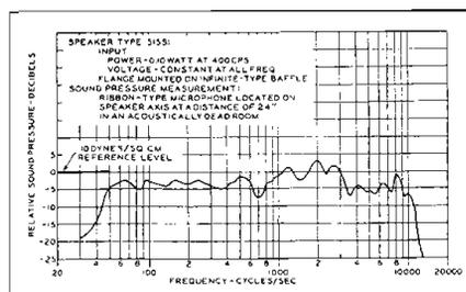
Fig. 2: Frequency response characteristic of 515S1 speaker mounted in infinite baffle
