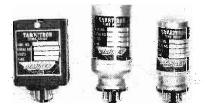
multiple contact arrangements, fast switching and also automatically relieves the time delay heating element of the necessity of continual excitation after performing the prescribed delay. Tarrytrons are hermetically sealed or strappaxed with inert gases which completely protects them from altitude, moisture, dust or other atmospheric conditions. Units are supplied with timing ranges from 2 to 150 seconds.—Cook Electric Co., 2700 North Southport Ave., Chicago 14, Ill.
