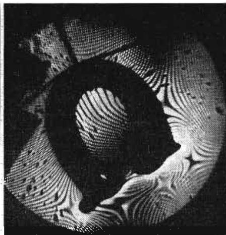
Right: Photo of magnetic field about horseshoe magnet 1/4 in. wide. New method of measurement is expected to find extensive application in study of space-charge fields, fields produced by contact potentials, waveguide problems, and properties of dielectrics
