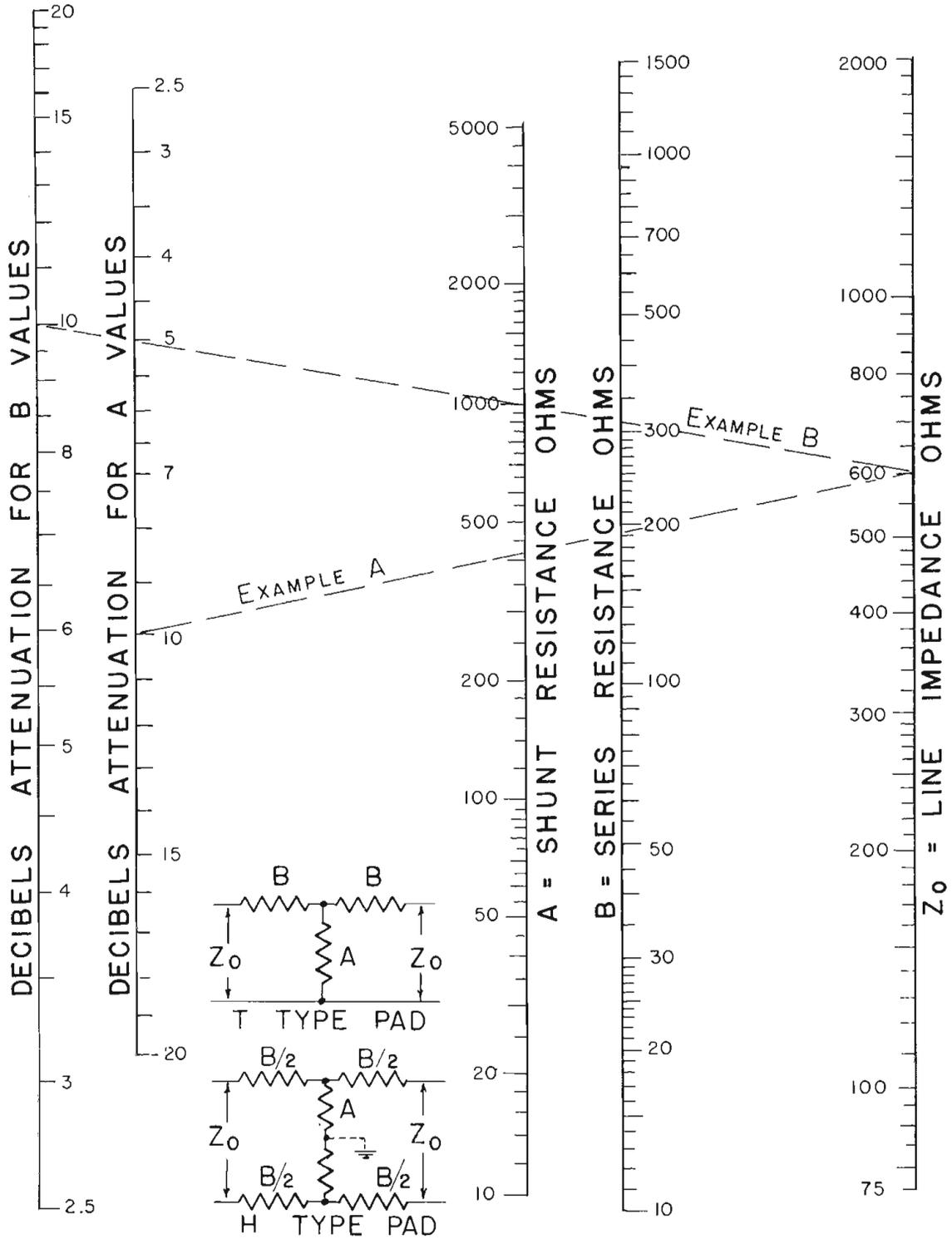
"T" and "H" type attenuators are simple standby pad circuits where fixed units of various sizes are permanently installed in the line. In using these values the terminal impedances "in" and "out" must be the same. Two lines from the db point on each of the scales at left to the  $Z$  scale at right will cross the A and B
