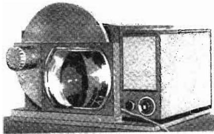
Probable appearance of standard receiver fitted with disk converter for CBS color
