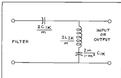
Fig. 4: m-Derived terminating half section
