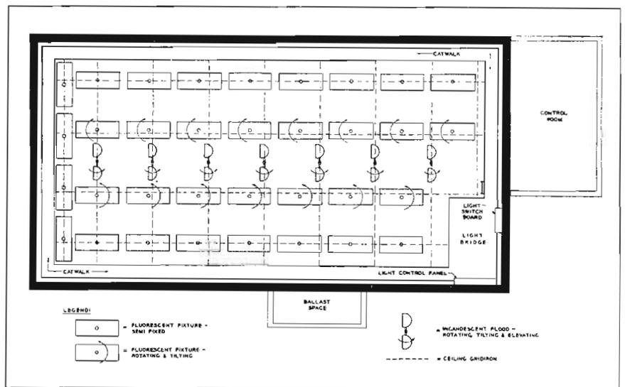
Fig. 9: Diagram of a typical lighting layout for a moderately sized television studio
