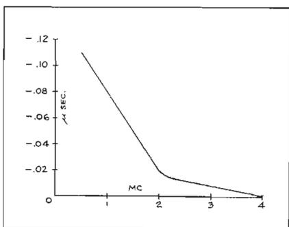
Fig. 9: Time delay vs. frequency for composite filter. (shown relative to delay at 4 MC)
