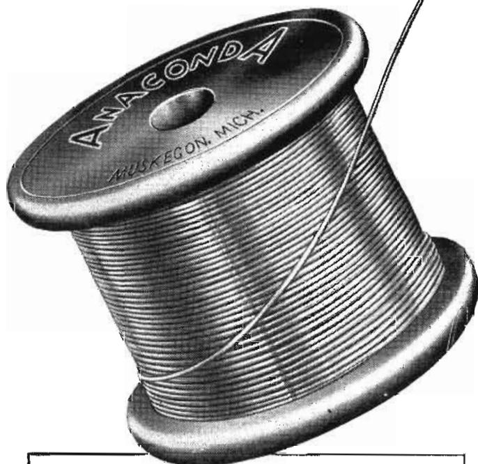
TO WITHSTAND temperatures up to 130° C, Vitrotex magnet wire is insulated with alkali-free glass fibres. This inorganic textile is soft and luxurious—with a tensile strength comparable to that of steel. The servings are bonded with a high grade insulating varnish, to give Vitrotex a smooth abrasion and moisture resistant surface.
