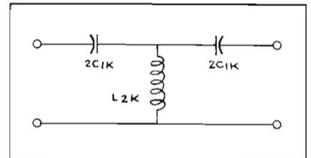
Fig. 3: Constant K high pass T section
