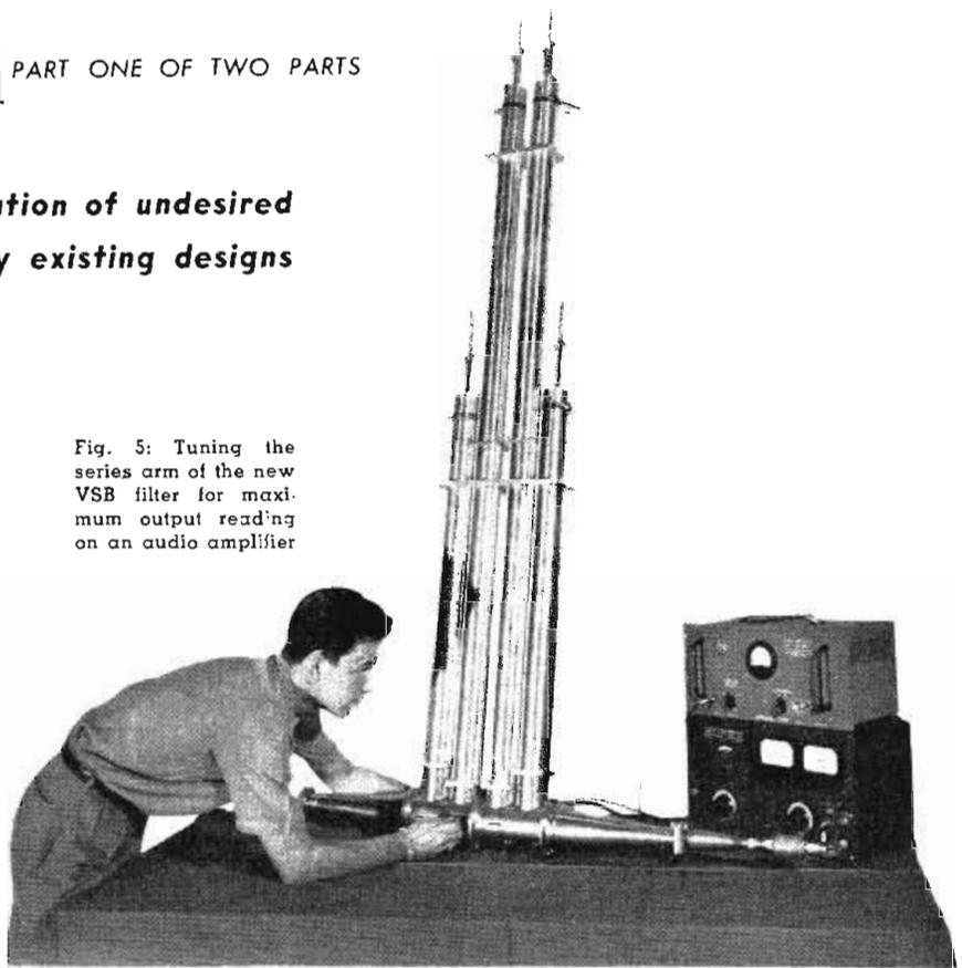
Fig. 5: Tuning the series arm of the new VSB filter for maximum output reading on an audio amplifier
