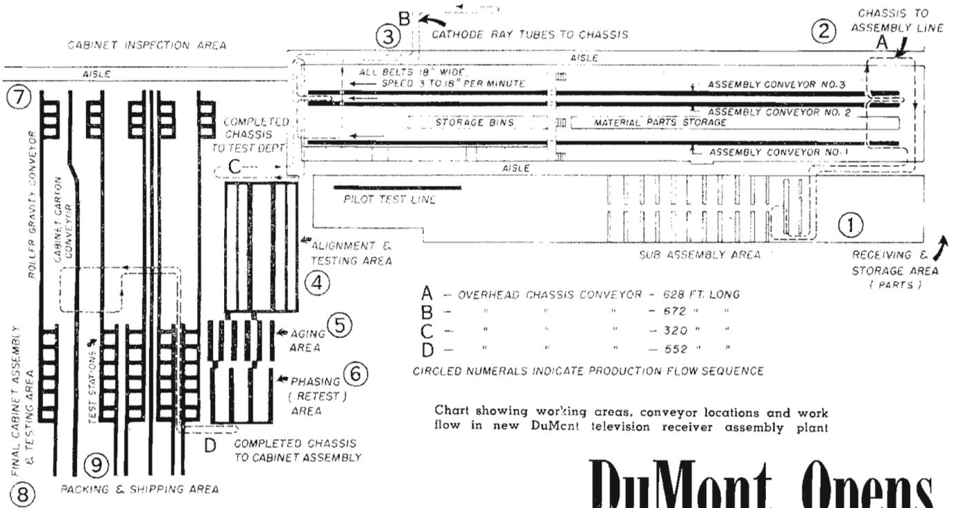
Chart showing working areas, conveyor locations and work flow in new DuMont television receiver assembly plant
