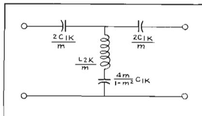
Fig. 2: m-Derived high pass T section
