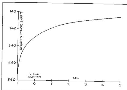
Fig. 8: Phase shift curve of composite filter
