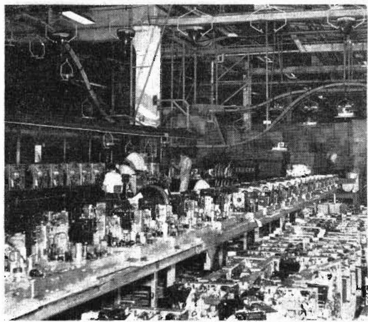
Mounting cathode ray tubes on the completed chassis at end of assembly lines. Receivers are then aligned and tested
