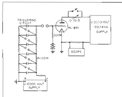
Fig. 2: Circuit used for surge current tests
