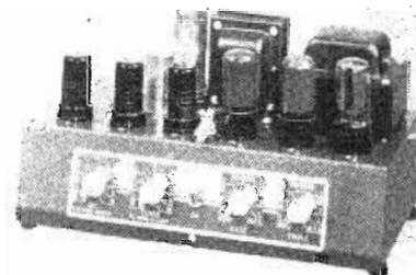
sponse with ten controls normal is  $\pm 1$  DB, 20 cps to 20 KC. Peak power output is 18 watts and power consumption is 70 watts. 110/120 v. AC, 60 cycle, fused. Separate bass and treble controls, each having boost and attenuation ranges, provide flexible compensation of frequency response for individual preference.—Precision Electronics, Inc., 611 Milwaukee Ave., Chicago 22, Ill.
