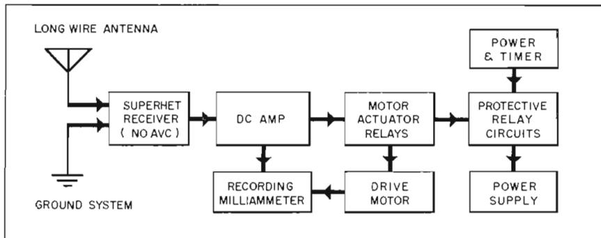
Fig. 2. Block diagram of apparatus at monitoring point shows functions of equipment
