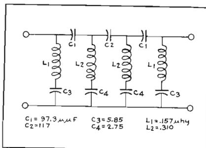
Fig. 7: Typical composite high band filter
