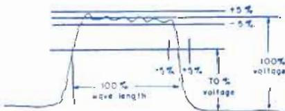
Specially designed G-E Type-E networks will produce impulses which have definite, known energy contents and durations, and thus are ideal for converting a-c or d-c charging voltages into approximately rectangular square waves. These networks consist of capacitor and coil sections adjusted to close tolerances and hermetically sealed in single metal containers.
