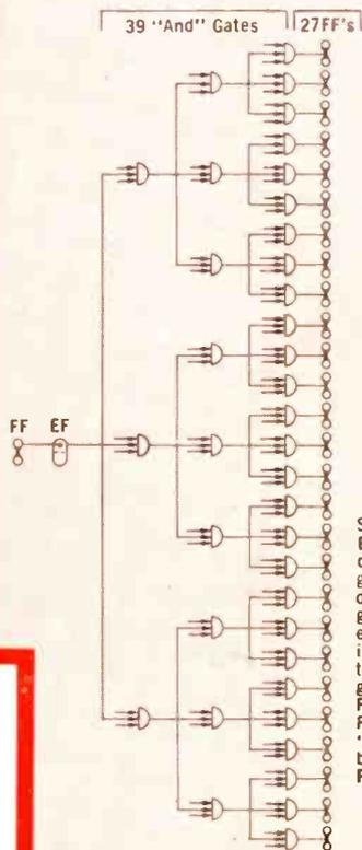
SCHEMATIC II—One Emitter Follower will drive three fully loaded gates, each gate driving three more gates in parallel and each of these gates, in turn, loaded with three more parallel gates, each driving a Flip-Flop. Total: 27 Flip-Flops and 39 "And" gates all driven by a single Emitter Follower.
