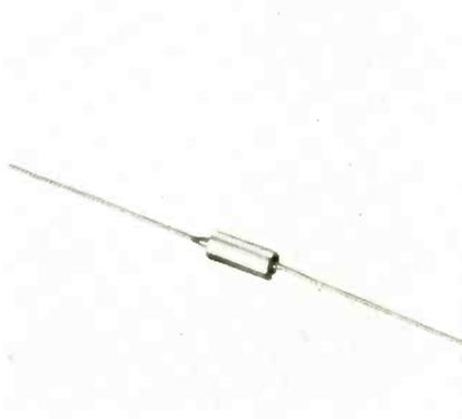
rosion. Capacitors have good stable capacity and dissipation factor over the range from -80° to +85°C. Shelf life is indefinite. They have axial lead construction, with hermetic glass-to-metal end seals. Leads are approximately 1½ in. long—of .020 in. wire, nickel-tinned. Available in standard EIA capacities. P. R. Mallory & Co., Inc., Indianapolis, Ind.
