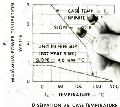
ohms at 25°C plus an operating range of -65°C to +200°C. Both are encased in short, round welded packages. The 2N497 is a 60 v. transistor for use with 28 v. power supplies in military aircraft. The 2N498 is a 100 v. device for use in higher voltage applications. Texas Instruments Incorporated, P. O. Box 312, Dallas, Texas.
