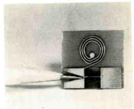
"Persistor" consists of bi-metallic loop which is maintained near absolute zero
