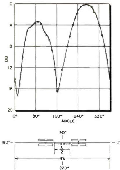
Fig. 6: Radiation is restricted to the portion confined by the suppressor chokes.
