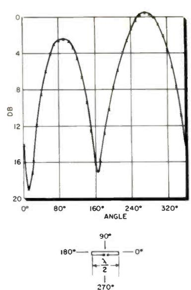
Fig. 7: Folded dipole pattern verifies feed system as cause of Fig. 6 lobe unbalance.
