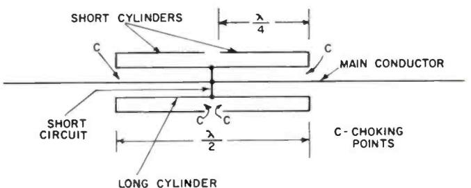
Fig. 4: By shorting the main conductor and the long cylinder at its mid-point, the element can be used as an effective radiation choke.
