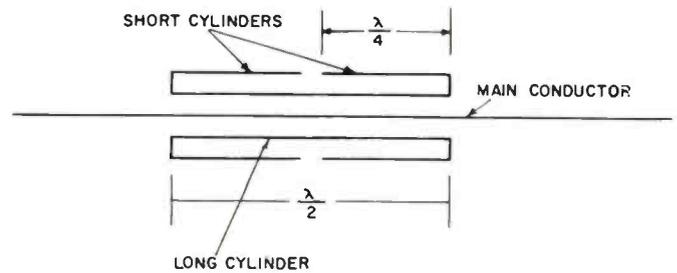
Fig. 1: One form of the element: various cylinders mounted over main conductor are connected to produce cooperative choking conditions.
