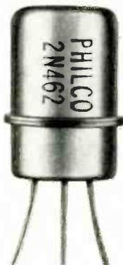
complementing circuits, bi-directional switches, bi-directional amplifiers, and phase detectors. It has good high voltage, current, and gain ratings. Maximum collector (or emitter) voltage is 40v; maximum collector current is 200 ma. DC current amplification factor ( $h_{FE}$ ) is typically 45, in either direction. Philco Corporation, Philadelphia, Pa.
