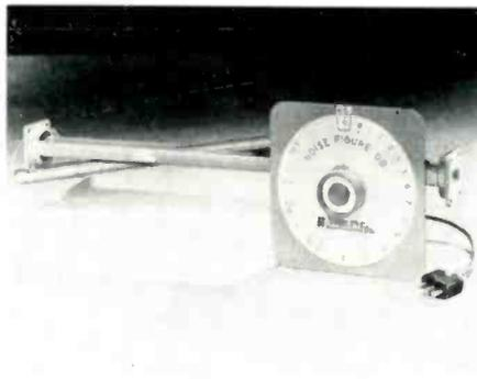
power supply, provides a noise generator designed for direct reading noise figure measurements which facilitates laboratory and production testing. These tube mounts utilize Argon gas tubes to provide a 16.0 db level of noise which is controlled by a precision attenuator section. Wave-line, Inc., Caldwell, N. J.
