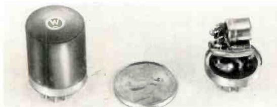
Fig. 2: Entire circuit can be potted in tiny case.
