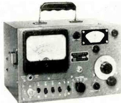
UHF converter expands signal readings to the complete UHF television range. Exact signal strengths can be read from 10  $\mu$ v. to 3 v. It includes a phone jack, front panel attenuator switches, pilot light, handle & carrying strap, db and percentage AM modulation scales. Blonder-Tongue Labs., Inc., 9-25 Alling St., Newark 2, N. J.
