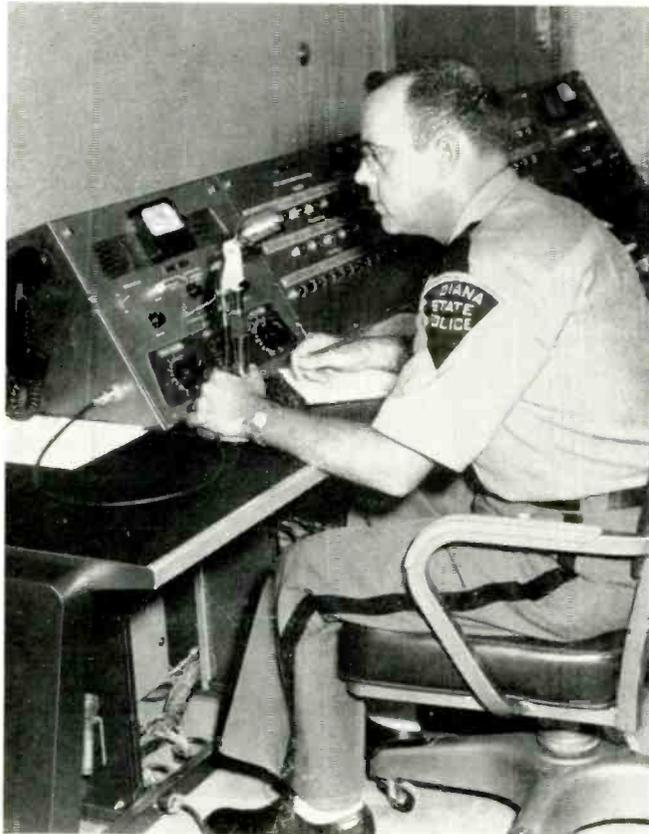
(Right) Two separate duplex VHF systems serve the Indiana State Police and turnpike maintenance personnel. The two transmitters are connected to one antenna, through tuned cavities. The receivers are similarly cavity-linked to one antenna. Interaction is negligible.
