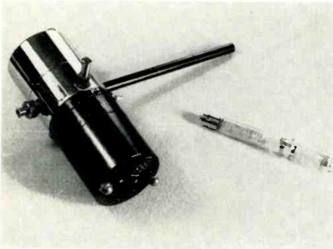
Fig. 4 (above): Cuvette photometer is used with an oximeter to measure the amount of oxygen in the blood.
