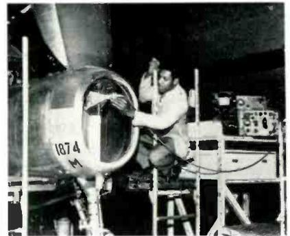
The radar system of Republic's F-84F Thunderstreak has its waveguide transmission line tested. Use of the Narda test adapter gives quick and accurate evaluation of the entire waveguide transmission line.
