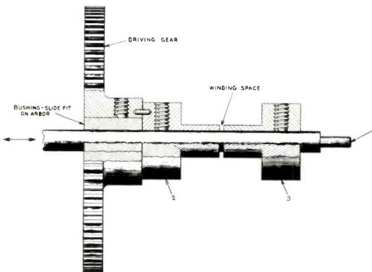
Fig. 4: Transformer cup is placed on stud at the end of the arbor and the coil is then pushed into slot by retracting the arbor.
