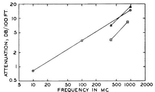
Fig. 4: Attenuation vs frequency of experimental silicone rubber coaxial cables.
