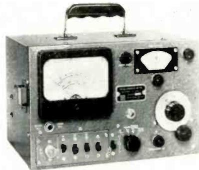
UHF converter expands signal readings to the complete UHF television range. Exact signal strengths can be read from 10  $\mu$ v. to 3 v. It includes a phone jack, front panel attenuator switches, pilot light, handle & carrying strap, db and percentage AM modulation scales. Blonder-Tongue Labs., Inc., 9-25 Alling St., Newark 2, N. J. Circle 243 on Inquiry Card. page 103
