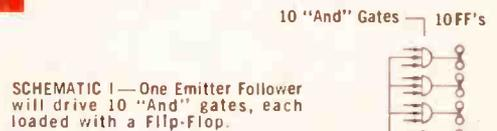
SCHEMATIC I—One Emitter Follower will drive 10 "And" gates, each loaded with a Flip-Flop.
