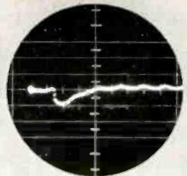
The MAGAMP has a surge capacity of 400% overload for 2 seconds. Regulation at the load is 1% or better. Recovery time is less than 50 milliseconds. Overshoot and undershoot are less than 25%, with a 30% change in load. (Scale in above photos: 5V/CM and 10MS/CM.)
