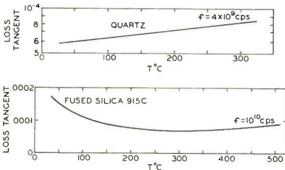
Fig. 6: Loss tangent vs temperature for quartz and fused silica—same sources as Fig. 5.
