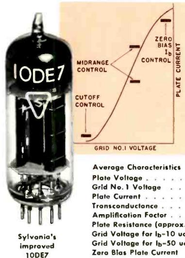
The transfer characteristics in the new 10DE7 are rigidly controlled for proper vertical deflection operation.
