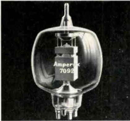
ment. Does not require water cooling. Heavy-duty anode is able to withstand large overloads. Envelope is constructed of extra-thick, hard glass for ruggedness. Used in continuous class C operation, 2 kw. power into industrial loads can be obtained. The thoriated-tungsten filament is rated at 6.3 v. Amperex Electronic Corp., 230 Duffy Ave., Hicksville, L. I., N. Y. Circle 225 on Inquiry Card, page 103
