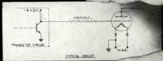
Heater voltage is only 1 volt, 30 ma, AC or DC. The anode will draw only 0.5 ma from a 50 volt DC supply during the zero-bias "on" condition. A 3.0 volt DC voltage is sufficient to cut-off plate current and light. Write for data sheet to Semiconductor and Special Purpose Tube Division, Amperex Electronic Corp., 230 Duffy Avenue, Hicksville, L.I., N.Y.
