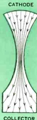
Sperry's Space-Charge Focus principle of beam control eliminates need for heavy, unwieldy magnetic structures. New Sperry tube design using this principle cuts weight, size, power consumption and cooling requirements.
