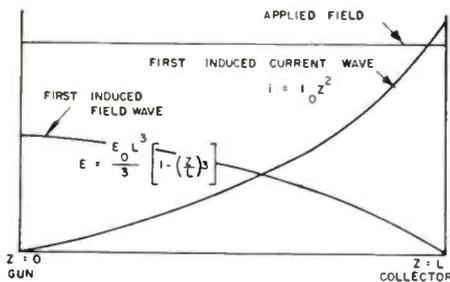
Fig. 4: Field and current component amplitudes obtained from simplified BWO theory.
