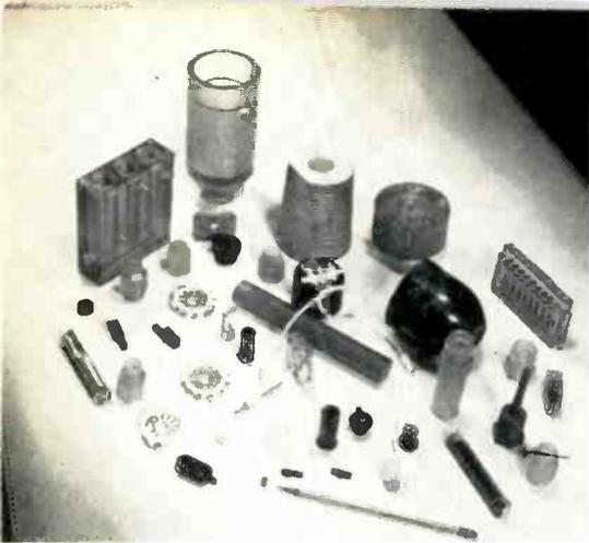
← A parade of a few of the 200 parts made by compression or injection molding, casting, and encapsulation at L&N.
