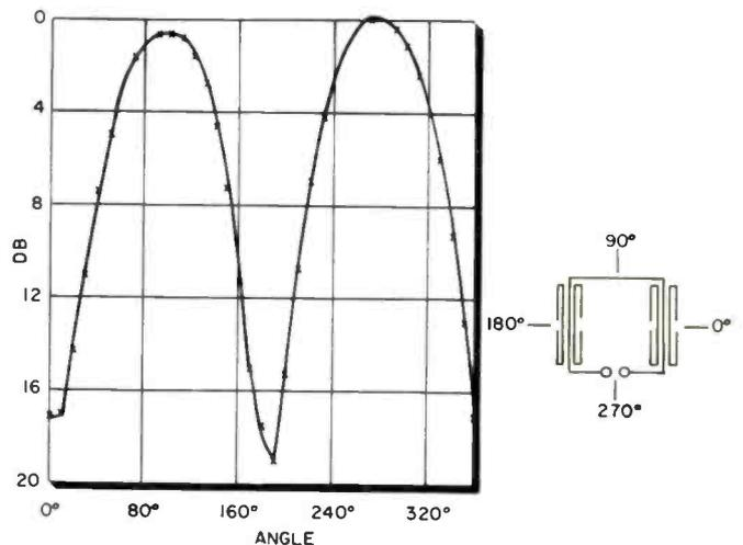
Fig. 3: E-plane pattern of the same square loop but with 2 suppressors added.
