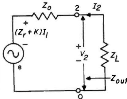
Fig. 5: Automatic elimination of internal function-sources by forming of transfer function representing a Thevenin generator.
