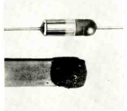
$-20^{\circ}\text{C}$  to  $+50^{\circ}\text{C}$  with adequate storage life. Of polar construction, the capacitor case and attached lead form the cathode terminal. Available in insulated and non-insulated construction. The anode tantalum wire extends through the teflon bushing to which a solderable lead is attached. It is encapsulated in a thermosetting resin. Aerovox Corp., New Bedford, Mass.
