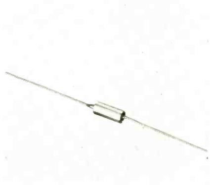
rosion. Capacitors have good stable capacity and dissipation factor over the range from -80° to +85°C. Shelf life is indefinite. They have axial lead construction, with hermetic glass-to-metal end seals. Leads are approximately 1½ in. long—of .020 in. wire, nickel-tinned. Available in standard EIA capacities. P. R. Mallory & Co., Inc., Indianapolis, Ind.
