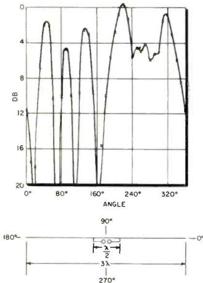
Fig. 5: Folded dipole with extended arms and its attendant multilobe pattern.
