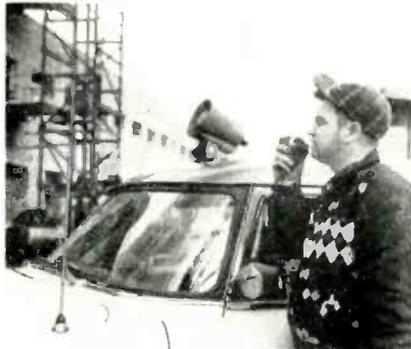
driver will hear all messages even when working away from his parked vehicle. And by turning a control, speaker is converted into a powerful public address system with a half a mile or more range. Speaker provides up to 15 watts power output at 12 volts. Motorola Inc., 4501 W. Augusta Blvd., Chicago 51, Ill.
