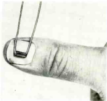
wire wound resistors. The NS6AZ (.125 x .250) is one in a line of over 15 sizes encapsulated to meet MIL R93A characteristic "A" and MIL R9444. Available with resistance values up to 125K with tolerance to 0.1%. This resistor will dissipate 0.1 watts at 125° C with no derating. Eastern Precision Resistor Corp., 675 Barbey St., Brooklyn 7, N. Y. Circle 223 on Inquiry Card, page 103
