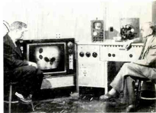
Fig. 9 (right): The UTCM, which instantly translates u-v absorption data of living cells into colors, uses pulsed radiation to help prevent lethal damage to cells.
