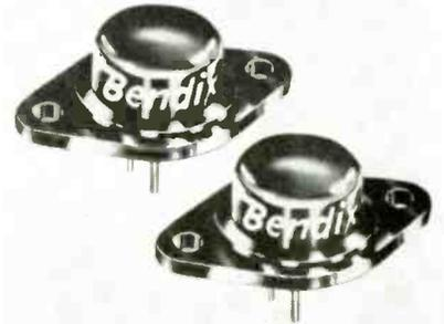
able. The 2N399 and the 2N401 can readily dissipate up to 25 w. Typical Class B undistorted output power for both types is 8 w. The 2N399 is a high gain transistor and the 2N401 is a medium gain power output transistor. Both feature welded construction with a vacuum-tight seal. Red Bank Div., Bendix Aviation Corp., 201 Westwood Ave., Long Branch, N. J. Circle 209 on Inquiry Card, page 103
