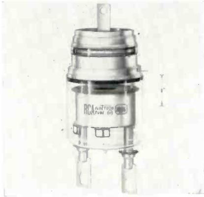
tube operation, is available. The RCA-7086 can also be used for grid-controlled rectifier or inverter service. Capable of withstanding a maximum peak forward and inverse voltage of 650 v. at a maximum peak anode current of 400 ampere in intermittent service, or 160 ampere in continuous service. Radio Corporation of America, Harrison, N. J.
