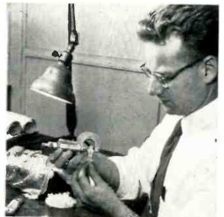
← Possibly the only epoxy casting in the Phila. Metropolitan area, a ph flow assembly component is being poured. It will then be baked in the large Dispatch Oven, Model Y-29-2 (\$650), in rear.
