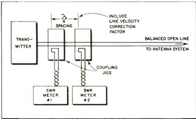
Fig. 2: Matching antenna with two SWR indicators on open balanced line. When both meters read the same, flat line conditions exist.
