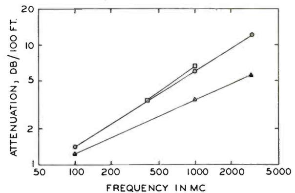
Fig. 3: Manufacturers data on 50-ohm "High-Temperature" coaxial cables—attenuation vs frequency.
