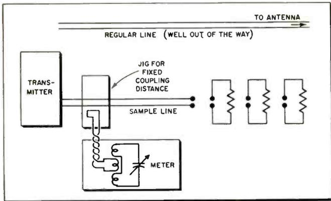
Fig. 4: Set-up for open line system, using one meter to obtain a fixed reference level for flat line condition.
