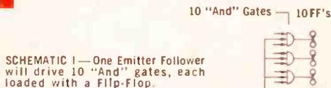
SCHEMATIC I—One Emitter Follower will drive 10 "And" gates, each loaded with a Flip-Flop.
