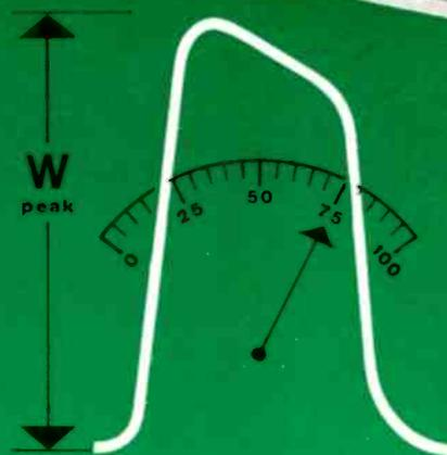
Meter indicates actual peak of power pulse, regardless of width, shape, rate, or duty cycle.
