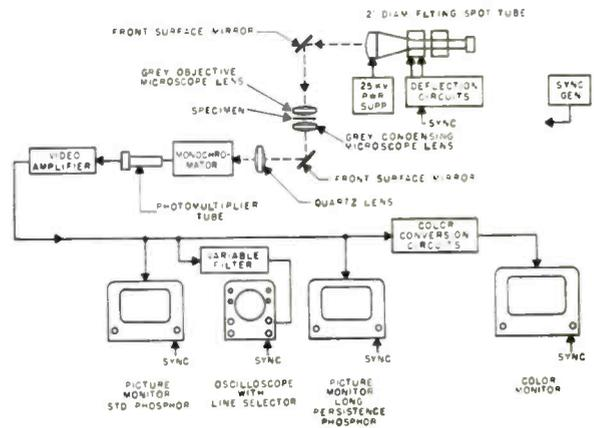
Fig. 2: This u-v microscope uses the flying spot technique.
