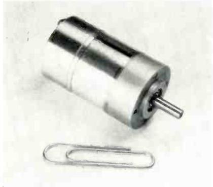
rated at 0.01 hp at 12,000 RPM, and Model 6A2 rated at 0.001 hp at 4,000 RPM. Model 6A2 is designed for continuous duty and requires a 0.22 amperes maximum current, while Model 6A5 is for intermittent service and requires 0.9 amperes maximum current. Western Gear Corp., P. O. Box 182, Lynwood, California.
