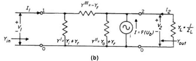
Fig. 2: Active TEE (a) and active PI (b) networks, which may represent transistor amplifier. Input and output immittance to be determined
