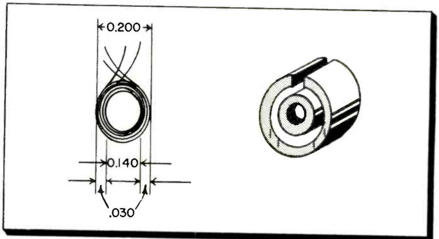
Fig. 1: I.D. of this coil is 0.140 in. With ferrite cup it forms subminiature transformer.
