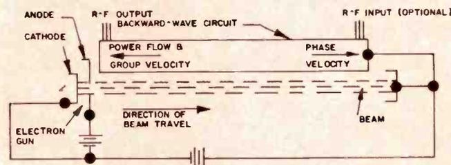
it has decreased in phase by  $90^\circ$ , and is therefore  $180^\circ$  out of the phase with  $dE_2$ . There is not a perfect cancellation because the inducing current grows with distance.
