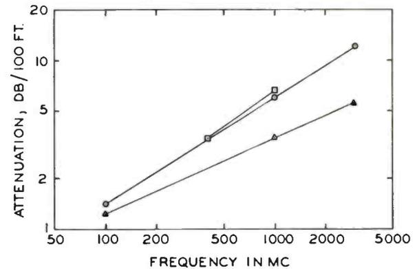
Fig. 3: Manufacturers data on 50-ohm "High-Temperature" coaxial cables—attenuation vs frequency.
