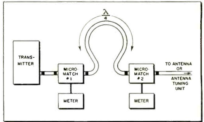
Fig. 3: Matching antenna with two SWR indicators spaced electrically  $\frac{1}{4}\lambda$ -wavelength. Line is flat when meters read identically.
