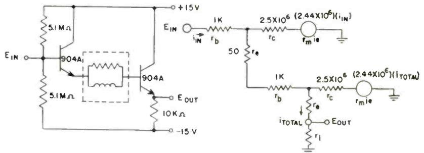
Fig. 1: Schematic and equivalent circuit for the transistor impedance changer.
