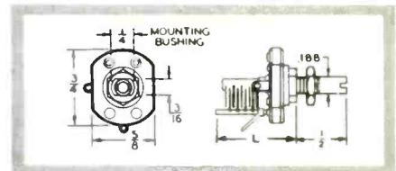
**SPECIALS**—Johnson Miniature Air Variables are available in production quantities with the following features: 1. Locking bearing. 2. 180° stop. 3. Various shaft extensions. 4. High torque. 5. Silver or other platings.
