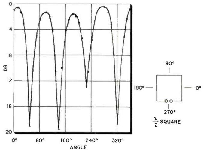
Fig. 2: The E-plane pattern of a square loop with sides a half wavelength long.
