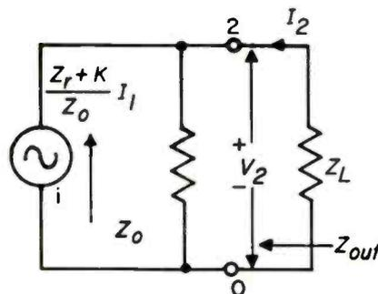
Fig. 4: Automatic elimination of internal function-sources by forming of transfer function representing a Norton generator.
