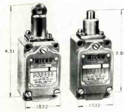
tact arrangements are double-throw 2-circuit, single-pole double-break. The electrical rating is: 10 a., 120, 240 or 480 volts ac; 0.8 a., 115 vdc. Micro Switch, Freeport, Ill.
