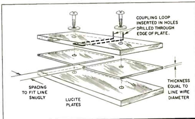
Fig. 5: Jig assembly. Reliability of readings will depend on the stability of coupling between the line and the measuring loop.
