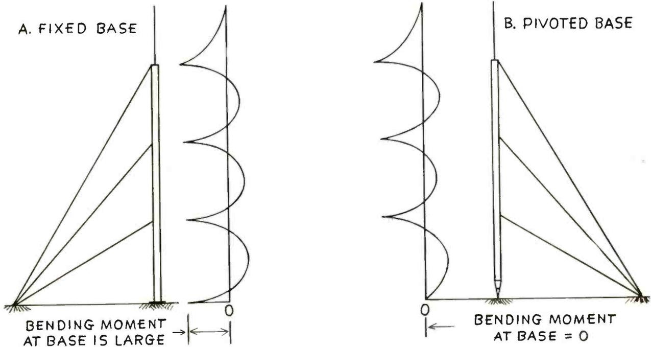
A guyed tower may be designed to come straight down at the base pier or to a pivot. Either method is satisfactory providing the conditions encountered are properly resolved and engineered.
