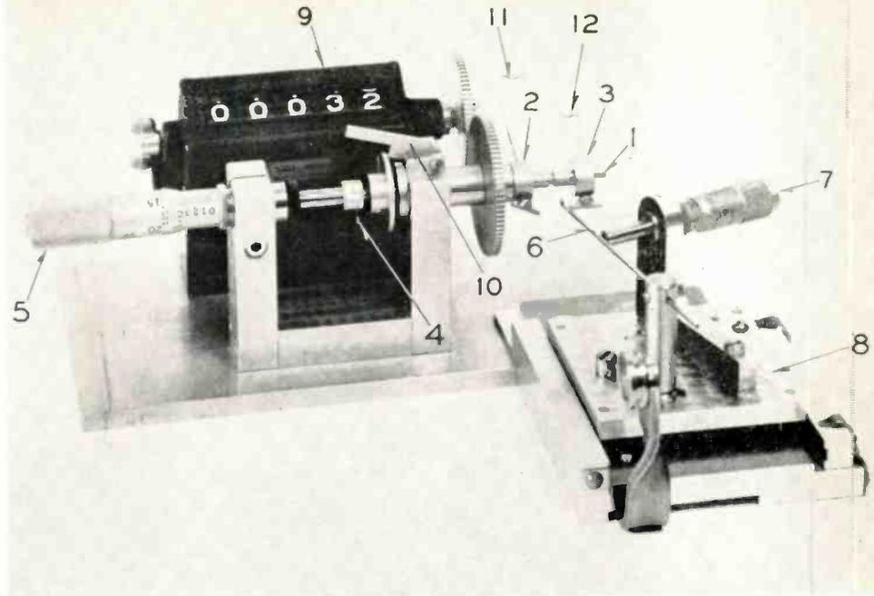
Fig. 2: Principal parts of winding machine are: (1) arbor, (2 & 3) adjustable collars, (4) coupling between adjusting micrometer (5) and arbor, (6) wire guide, (7) micrometer to control guide, (8) movable platform for wire guide, (9) counter, (10) lock for arbor, (11 & 12) outriggers.
