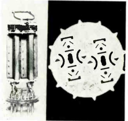
nections, freedom from cathode interface and interelement leakage and long life characteristics. Structurally, it makes use of a protective shield mica to prevent deposition of getter material on micas and electrodes. Plate dissipation is 4.5 w. per plate with a total of 8 w. for the 2 sections. Sylvania Electric Products, Inc., 1740 Broadway, New York 19, N. Y. Circle 219 on Inquiry Card, page 103
