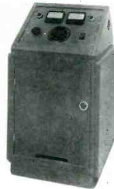
tained. Output is 5 kw at 1000 or 5000 v rms. Operates from 220 v rms, 60 cps, single phase line. Output voltage is continuously adjustable. Has instantaneous trip type circuit, breaker rated to trip at 25 amps. Voltage and current are simultaneously metered. Industrial Transformer Corp., Gouldsboro, Pa.
