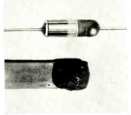
$-20^{\circ}\text{C}$  to  $+50^{\circ}\text{C}$  with adequate storage life. Of polar construction, the capacitor case and attached lead form the cathode terminal. Available in insulated and non-insulated construction. The anode tantalum wire extends through the teflon bushing to which a solderable lead is attached. It is encapsulated in a thermosetting resin. Aerovox Corp., New Bedford, Mass.
