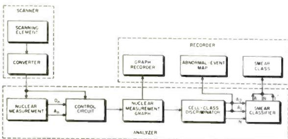
Fig. 6 (above): The function diagram of a cytoanalyzer.
