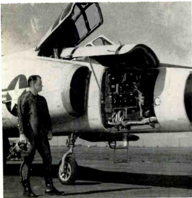
Test pilot inspects prototype test model of "Digitair," first airborne digital computer in actual production. Shown here installed in an F-102A all-weather interceptor, the computer is small enough to fit into a 21-inch table model TV cabinet.
