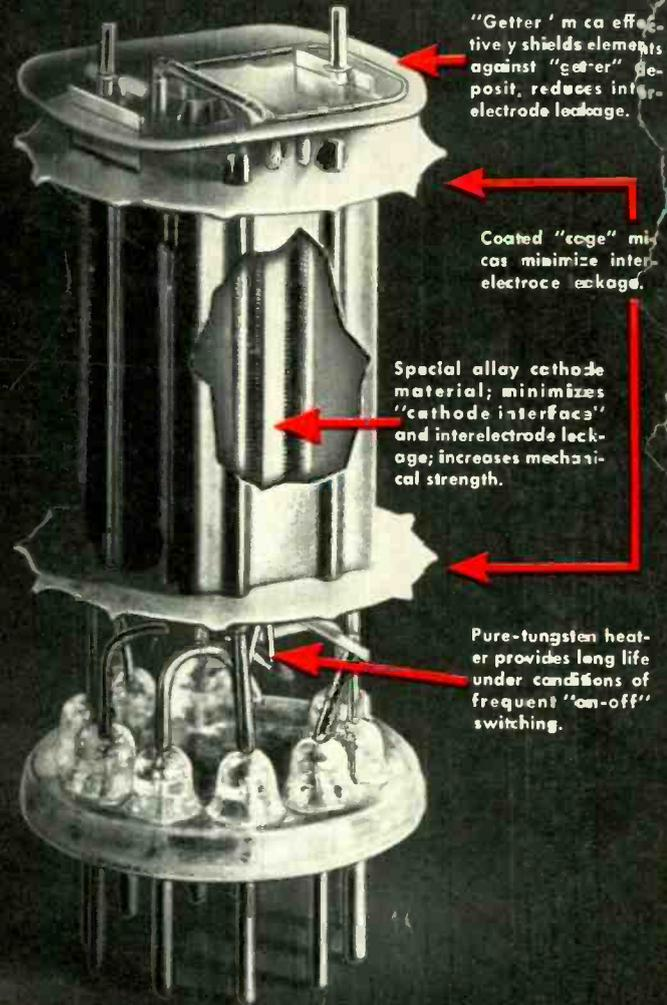
"Getter" mica effectively shields elements against "getter" deposit, reduces inter-electrode leakage.
