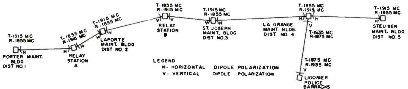
Each patrol car is linked to all offices of the toll system, and with all other mobile units by the system of base stations and microwave links. All calls on the patrol circuit are constantly monitored by all other units in the system.
