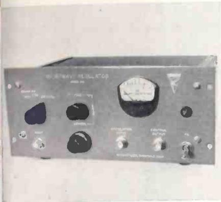
square wave modulated constant power source. The device itself operates at an audio frequency, hence, is completely independent of microwave power and frequency. By utilizing constant power, systems are more versatile and some measurements heretofore long and laborious, if not impossible, are done swiftly and with high accuracy. Brocker Labs., Dept. TT, P. O. Box 967, Sunnyvale, Calif.
