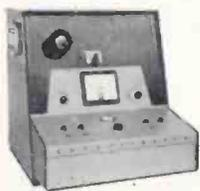
24-210... Low cost. Portable with no sacrifice of reliability. Detects at least  $1 \times 10^{-9}$  atm cc/sec of air. Weighs 145 lbs. Available with mobile workstand. Operates on 115 volts, 60 or 50 cycles. Bulletin CEC 1830-X32.
