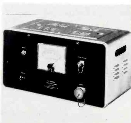
It has a meter and neon light for visual warning. Sensing unit can be either an alpha scintillation probe or a GM tube. The Victoreen Instrument Co., 5806 Hough Ave., Cleveland 3, O.
