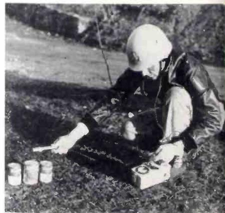
A N. Y. Civil Defense Warden checks food cans for radioactive contamination with new transistorized beta-gamma survey monitor manufactured by Universal Atomic Div. of Universal Transistor Products Corp.
