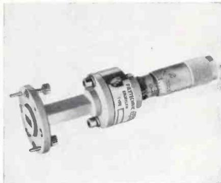
they are the most useful terminating impedances in waveguide measurements, apart from matched loads. The units consist of a section of waveguide in which a short-circuiting plunger can be moved by means of a micrometer drive. This is a non-contacting short of the two-section coaxial-filter type. Five types are available. Polytechnic Research & Development Co., Inc., 202 Tillary St., Brooklyn 1, N. Y.
