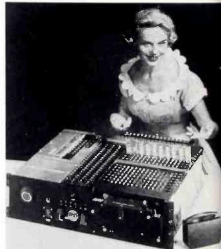
The "APAC" computer developed by Northrop Div., Northrop Aircraft, is designed for airborne applications and features full transistorization. APAC (Airborne Parabolic Arc Computer) is packaged into 1½ cu. ft., has magnetic memory drum.
