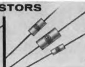
**METAL GRID PRECISION RESISTORS**—Hermetically sealed. Non-inductive. 1, 1/2, and 1/4 watts at 100°C. Tolerances 0.1% to 1.0%. Temp coef.  $\pm 25$  PPM/°C.
