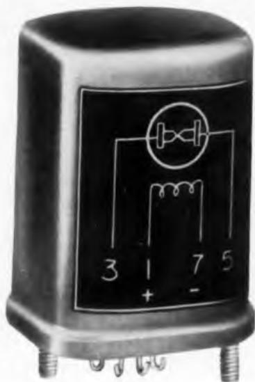
Isolated coil circuit allows switching of many independent circuits within one unit.
