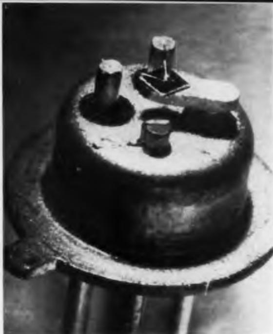
Fig. 5: Photo close-up. Shock limit is determined by the .04 mil gold wire.
