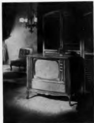
Philco's radically new TV line features a striking departure in this portable picture tube which is connected by 25 feet of cable to the main chassis, can be positioned where the viewer chooses.
