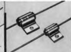
**COPPER CLAD**—Metal panel mounting, insulated composition resistor supplied in two ratings: 3 and 4 watts at 70°C, and 4 and 5 watts respectively at 40°C.
