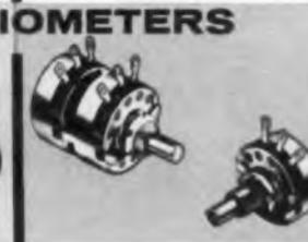
**HIGH TEMPERATURE**—Type K. Similar to Type J but rated 3 watts, 70°C; 2 watts, 100°C; and 1 watt, 125°C—derate to zero at 150°C. Many types and tapers.
