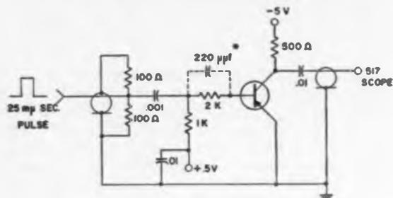
\* CAPACITOR ADDED FOR STORAGE AND FALL TIME MEASUREMENT
