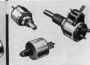
**MINIATURE**—Type G. Solid molded element. Only 1/2" in diam. Plain or lock bushing; also with line switch. Rated 0.5 watt at 70°C. Values to 5 megohms.
