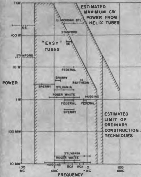
Fig. 2: Power vs. frequency for O-type forward wave cw amplifiers. Commercially available tubes are indicated by solid lines.
