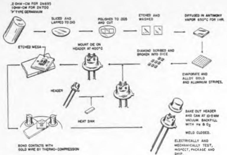
entirely germanium. That is, there are no alloys involved in the formation of the collector junction. Thus, thermal runaway in power dissipation modes of operation is far less dangerous.
