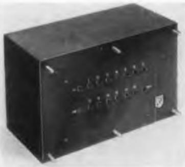
a delay line. Wider bandwidth enables it to handle closely-spaced pulse groups. The unit measures 3 x 4 1/2 x 8 1/2 in. ESC Corp., 534 Bergen Blvd., Palisades Park, N. J.
