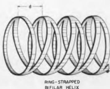
Fig. 9: Ring-strapped bifilar helix offers advantages over single helix at high voltages
