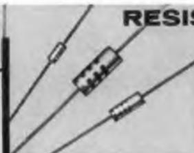
**HERMETICALLY SEALED** in ceramic tubes. Solid, hot molded resistor. Less than 1% resistance change after 250 hr, 95% rel. hum., 40°C. Resistance values to 22 megohms.
