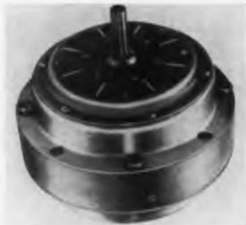
performance with long-life reliability. Horsepower ratings are from 1/200th to 1/20th, with a running torque of 2.8 in.-oz. to 28-in.-oz. Different rpm's can be selected by varying input frequency. It reaches full speed in 1 revolution and maintains synchronous speed at rated load. Motor is totally encased. Dale Products, Inc., Box 135, Columbus, Nebr.
