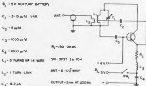
Fig. 11: 200-300 MC variable frequency oscillator
