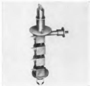
1.4/1 range of frequencies from 685 to 985 Mc. It is a 4 cavity amplifier klystron requiring about 1 w of drive power. The 4 internal cavities tune with individual drive shafts. It needs only a dc power supply, cooling and mounting magnet to form a complete microwave amplifier unit. Varian Associates, Palo Alto, Calif.
