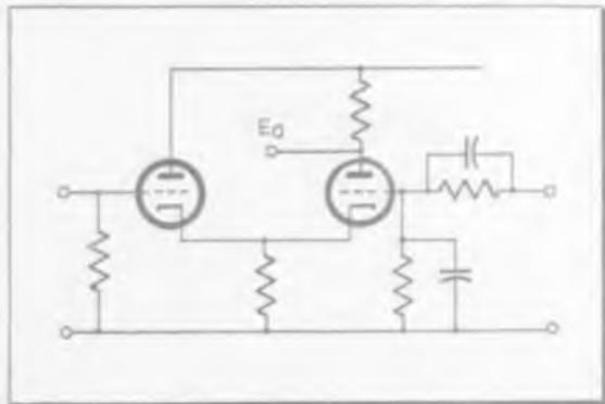
Fig. 2: Alternate method balances without need for an attenuator.
