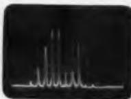
Relative lack of sidebands to left of carrier (centered on Panalyzer screen) indicate limited deviation on clipped and of oscillator swing
