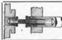
Coupling is used for the transmission of power or control of movement between parts located close together in a piece of equipment. It is not a separate type of flexible shaft but rather an added application of flexible shafting.
