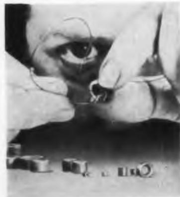
Rigid structure of the cap of these new "Polly Cap" tape wound bobbin cores by Magnetics Inc. will not distort with temp. changes, allows easy handling during assembly.
