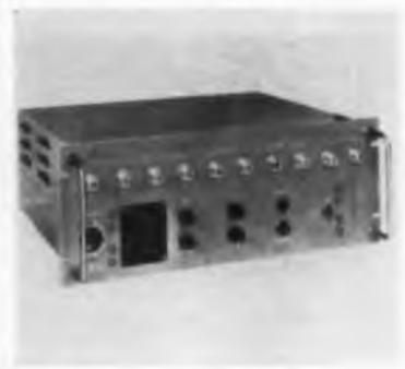
tenuation of intermodulation components, and a 6 db noise figure. Modular isolator circuits attenuate receiver local oscillator signal by more than 90 db. Degradation of weak signals by a 1 v. signal is limited to 1 db over the band. Selection between input impedances is made by patch cord. CGS Labs., Inc., Ridgefield, Conn.
