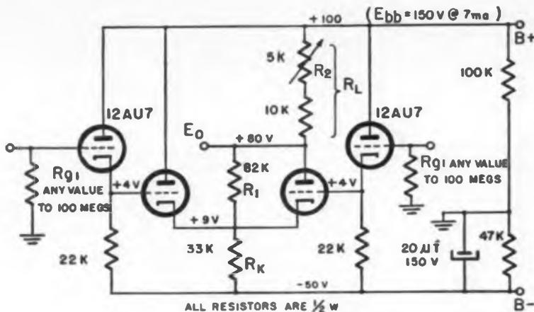
Fig. 3: Final circuit of the transformerless bridge null detector.
