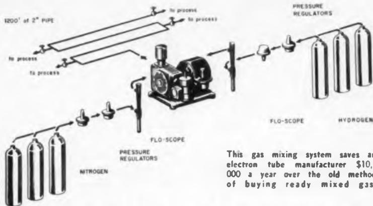
This gas mixing system saves an electron tube manufacturer \$10,000 a year over the old method of buying ready mixed gas.
