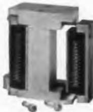
**GAP-MOUNTED**—Multi-channel head cartridges, easily removed and replaced with no close adjustment necessary. Bracket and cartridges have lapped surfaces providing reference positions to gap perpendicularity, azimuth and contact adjustment.
