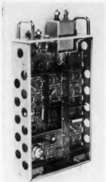
Unitized plug-in modules permit change from direct recording to frequency-modulated or PWM telemetering in seconds.
