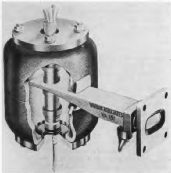
Fig. 4: Commercial O-type X-band BWO employing PM focusing.
