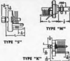
**TYPE “S” CAPACITORS**—The Type “S” Capacitor falls midway between the type “M” and “K” capacitors in physical size. Peak voltage rating 850 volts—plate spacing .013; other spacings available on special order. Square mounting studs tapped 4-40 on 17/32” centers.
