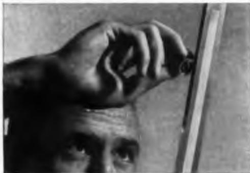
**Electromagnetic positioning** of cutting edges is directed by this etched metal bar, a significant innovation which aided in the Hughes Products development of the first all-electronically controlled machine tool line.
