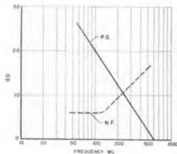
Fig. 9: Neutralized power gain and noise figure vs. frequency
