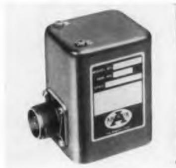
TME-2 SD are for use with fast-response, 100-ohm-resistance temperature transducers to produce a full 5 volt output for a span of only 75° F. TME-1 SD is a single-channel unit; TME-2SD, a dual-channel unit. They meet Specification MIL-E-5272A. Arnoux Corp., 11924 W. Washington Blvd., Los Angeles 66, Calif.
