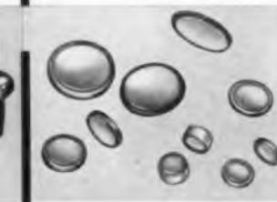
**BARE DISC** ceramic capacitors for direct mounting in printed circuit boards. Mechanically strong to avoid breakage in handling, installing, and soldering.
