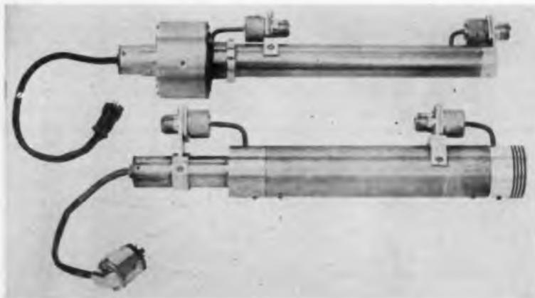
Fig. 5: (1) Two O-type X-band forward wave amplifiers, using periodic magnetic focusing.
