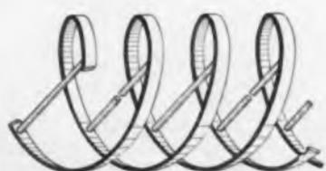
Fig. 10: Diametrically strapped bifilar helix (with gaps) with alternate straps broken
