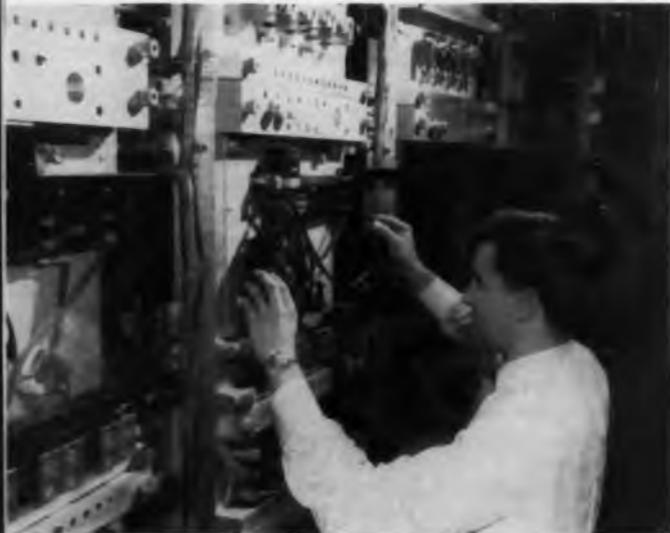
Computers are the heart of much systems planning. Here, at Raytheon, an engineer threads "Raydac" tape-handling mechanism
