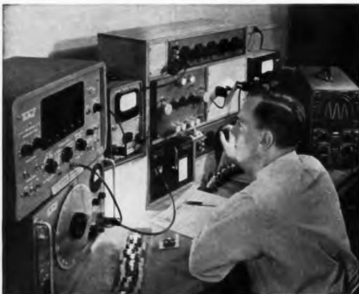
Test set-up devised to check low induction permeability.
