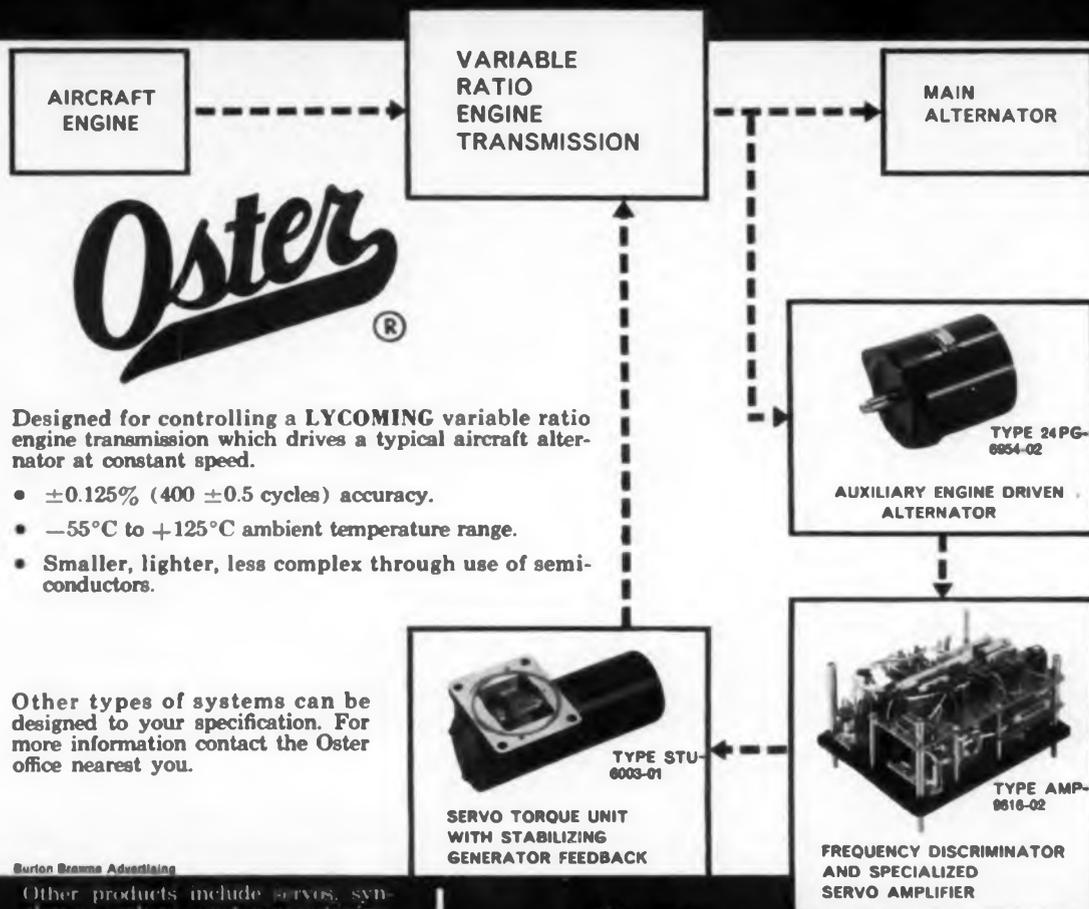
Designed for controlling a LYCOMING variable ratio engine transmission which drives a typical aircraft alternator at constant speed.
