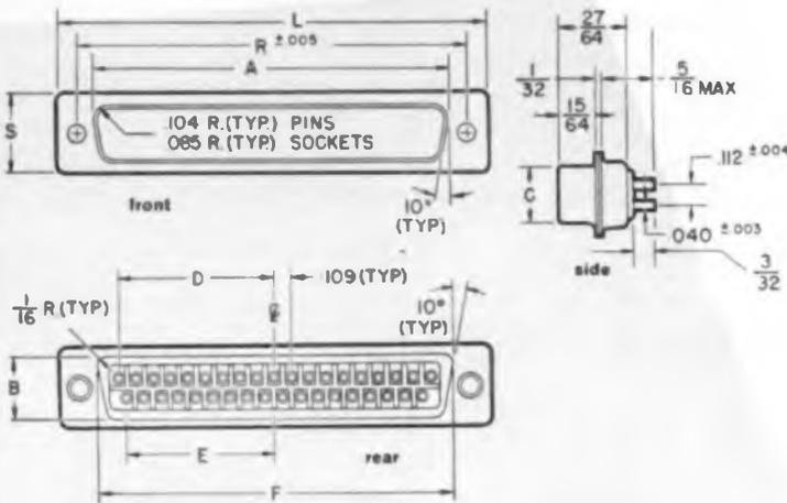
D Sub-Miniature plugs and sockets with printed circuit pin and socket inserts are now available as listed for immediate delivery.
