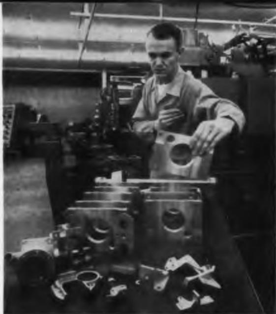
At Hughes Aircraft these precisely machined parts are turned out on a numerically controlled machine tool
