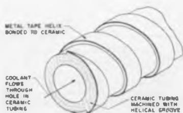
Fig. 8: Properly cooled tape helix circuit yields high cw power and wide bandwidth
