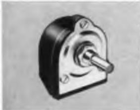
**INDUSTRIAL**—Type H with solid, hot molded resistor element. Quiet, improves with use. Life over 100,000 cycles. Rated 5 watts, 40°C; and 3 watts, 70°C.
