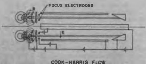
Fig. 11: Promising line of development in beam focusing involves the Harris flow and improved modifications by Cook.
