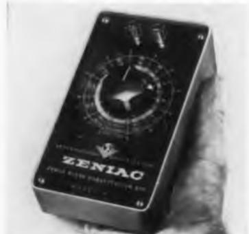
cuit. A turn of the selector switch rapidly determines the exact diode required. International Rectifier Corp., 1521 E. Grand Ave., El Segundo, Calif.
