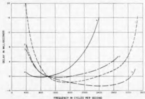
Fig. 6: The delay characteristics of some typical phone channels.
