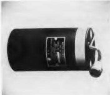
Small light weight motor-generators for the missile and aircraft industry are available. A series of models are available operating from a 400 cps, single or multi-phase supply and delivering 250 w. of continuous power at frequencies from 1000 to 5000 cps. D & R, Ltd. Booth 635.
