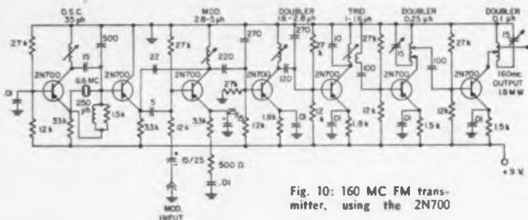
Fig. 10: 160 MC FM transmitter, using the 2N700
