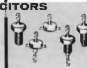
**FEED-THRU & STAND-OFF** discoidal capacitors for VHF and UHF range. No parallel resonance effects at 1,000 Mcps or less. Nominal values 4.7 to 1,000 mmf.
