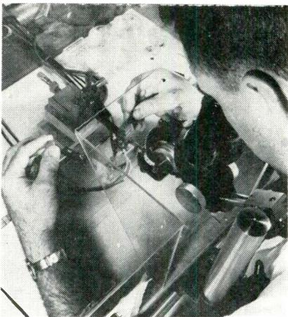
At Bell Telephone Labs T.B. Light is using a newly developed method of compression bonding to join gold leads to a transistor.
