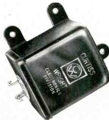
to shock and vibration. Preset time delays between 20 and 180 sec. are available. The relay is voltage compensated from 22 to 32 vdc with a nominal 28 v. rating. Temperature compensation is from -65°C to +125°C. Operating power is less than 3 w. after the timing interval and 10 w during timing. Various contact arrangements are available. Curtiss-Wright Corp., Wood-Ridge, N. J.
