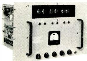
MODEL 201 for Tape Indexing generates numerically coded timing signals which are recorded on the magnetic tape throughout the data recording periods, providing a precise digital index in terms of elapsed time.
