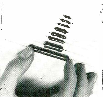
has eight sizes, with a selection of five wattage ratings:  $\frac{1}{8}$ ,  $\frac{1}{4}$ ,  $\frac{1}{2}$ , 1 and 2 watts. Resistance range is from 1 ohm to 50 megohms, depending on size and type. Standard tolerance is 1%. Typical derating is 100% power to 70°C. derating to 0% at 150°C. Dielectric strength is 1000 vac on the V-block test. All resistors have axial leads. Dale Products, Inc., Columbus, Nebraska.
