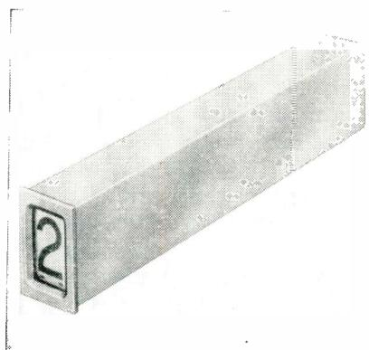
Numbers 0 through 9 and two blanks are displayed in sequence in response to four bit binary coded decimal input. Operating on an open circuit principle, complete code agreement of both binary ones and binary zeros is checked to assure positive and correct positioning of the indicator. Westinghouse Air Brake Co., Union Switch & Signal Division, Swissvale, Pa.
