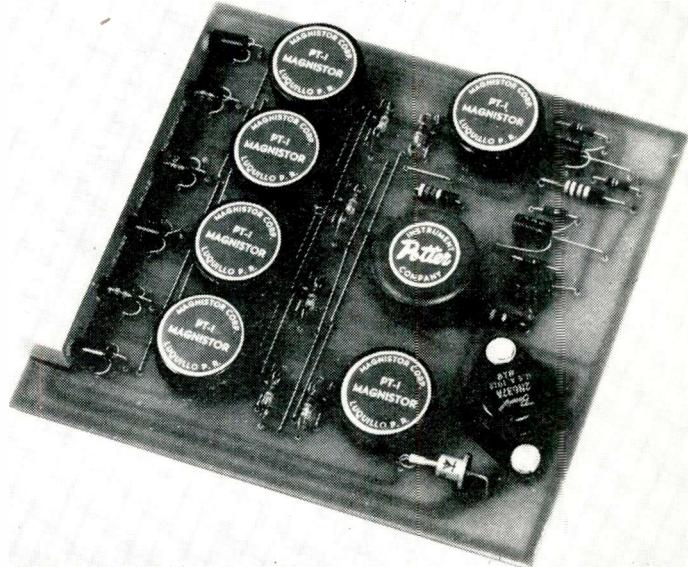
actuated dissipates the stored magnetism. The alternate states of magnetism resulting is evidenced by a two state change of inductance of an R.F. signal winding.
