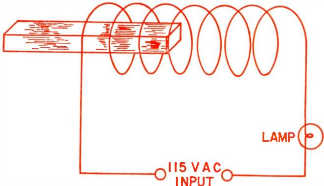
Fig. 1: A simple demonstration of magnetic amplifier principles
