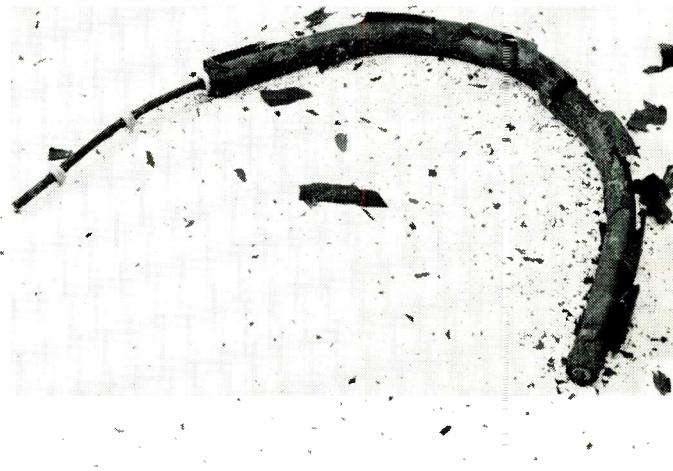
Fig. 9: Copper sheathed beaded cable after 15 min. at 650°C.
