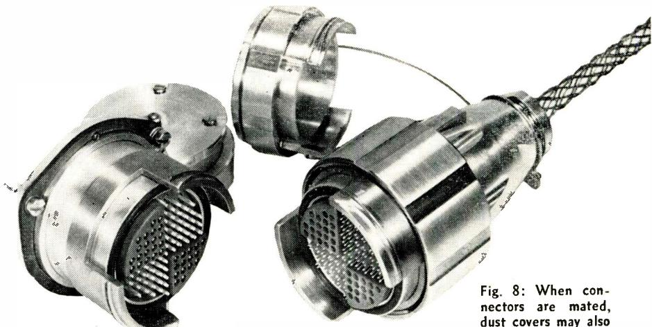
Fig. 8: When connectors are mated, dust covers may also be mated.
