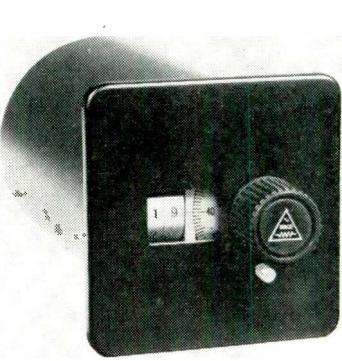
is supplied in the standard resistance value of 10,000 ohms and in other resistance values on special order. Full scale resistance accuracy is  $\pm 0.05\%$ , linearity  $\pm 0.01\%$ , resolution 0.002%. Power rating is 5w and the operating frequency range is dc to 10 KC. Rinco Inc., 7962 S.E. Powell Blvd., Portland, Oregon.
