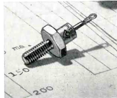
These silicon power rectifiers are designed for conduction cooling by mounting directly onto the chassis. Ratings from 400ma to one amp. are possible at PIV ratings of from 50 to 600 volts.
