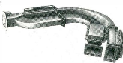
usual dual polarized horn requires a coax input. This feature has the advantage of providing the same center of radiation for both signals. Maximum power transmission is obtained in both polarizations. The horn handles 10 kw with more than 30 db decoupling between the signals. The horn has been produced in the frequencies of 1700-2400 MC, 755-985 MC and 400-560 MC, but the design is available in other frequencies. D. S. Kennedy & Co., Cohasset, Mass.
