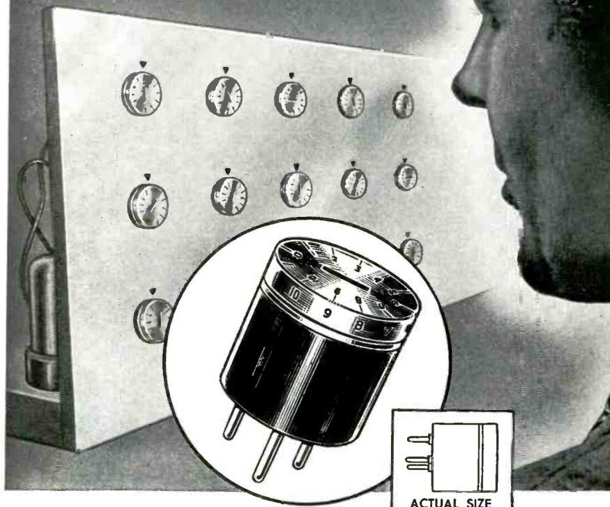
**Plugged into printed circuits or mounted on control panels,** this new  $\frac{1}{2}$ " pot speeds adjustments by letting you see what you've set. Its dual-calibrated dial tells at a glance slider location, shaft angle and voltage percentage. The  $300^\circ$  winding angle is equally graduated from 0 to 10. Zero on the dial lines up with a scribe line on the side of the pot at  $0^\circ$  rotation. Terminals are located on a standard 0.1" grid, as used in printed circuits.
