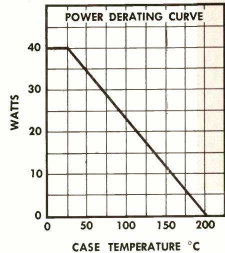
NEW TI silicon intermediate power transistors have bridged the gap between high and medium power devices...TI 2N1047, 2N1048, 2N1049, and 2N1050 guarantee 20 watts at 100°C.
