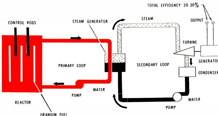
Fig. 5: Simplified diagram of a pressurized water system illustrates energy conversion.
