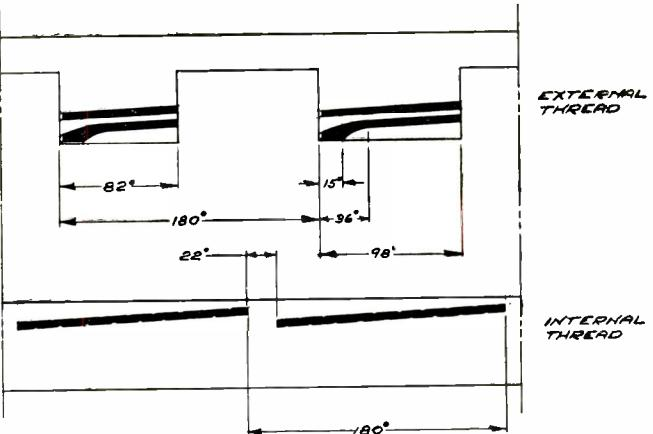
Fig. 10: Connector double thread with coarse lead-in is shown.
