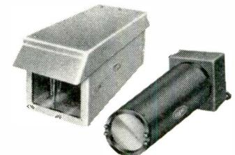
**SPECIAL HOUSINGS** make GPL cameras weatherproof, explosionproof, dustproof. Extremes of weather and climate cannot affect camera operation in housing (l). Fans and thermostatic heaters control inside temperature, while windshield wipers—inside and out—keep viewing window free of condensation, rain and snow.
