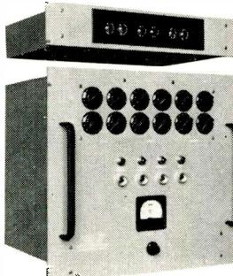
MODEL 202 for Tape Searching operates during data reduction periods. This instrument automatically locates and selects for controlled playback the tape data included between a "sequence start time" and a "sequence end time" specified by panel dial settings. Model 202 may be modified to search for timing formats other than those originated by Model 201.
