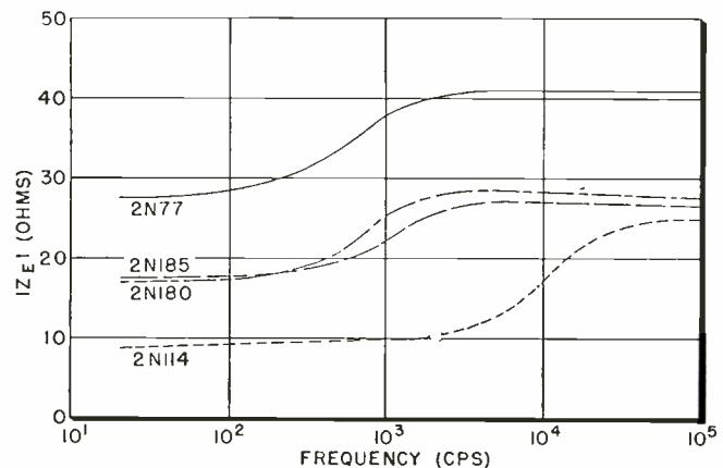
Fig. 1 (left) and Fig. 2 (right): Over I-f range, magnitude of equivalent T-parameters of certain audio transistors change radically.
