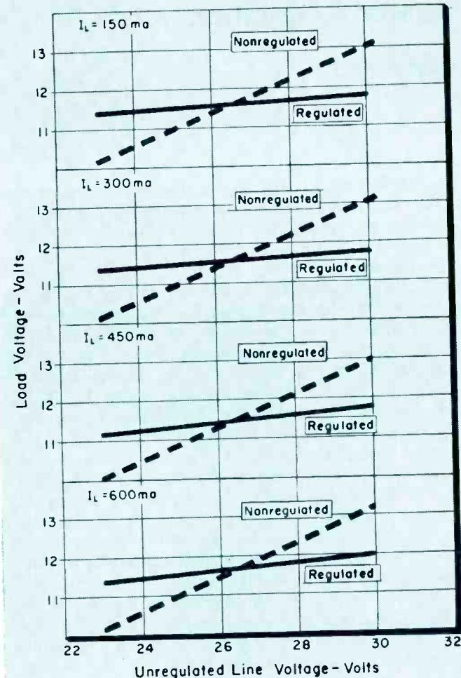
Fig. 2: Load-input voltage of dc regulated heater voltage
