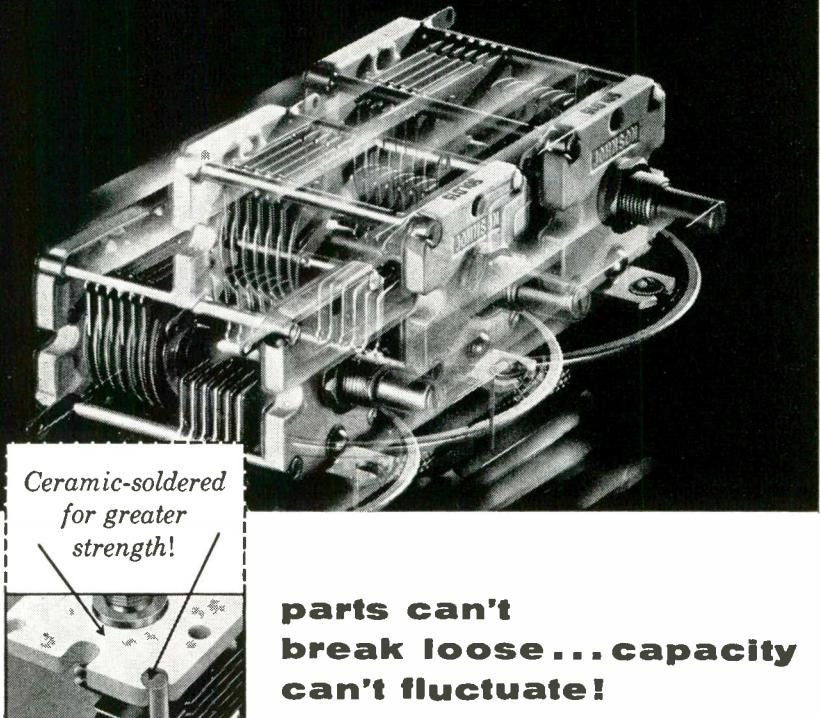
These ceramic-soldered Johnson Type "L" capacitors are an ideal choice for applications requiring extreme stability and strength. Rotor bearings and stator support rods are actually soldered directly to the heavy  $\frac{3}{16}$ " thick steatite ceramic end frames. Impervious to shock and vibration, parts can't break loose . . . capacity can't fluctuate.
