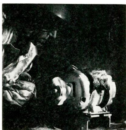
Cooking a steak on the motor's shell shows dramatically the high temperature characteristics of Westinghouse's new "red hot" motor.
