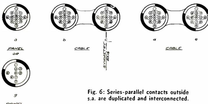
Fig. 6: Series-parallel contacts outside s.a. are duplicated and interconnected.
