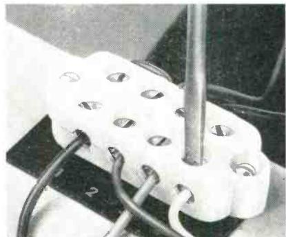
time required by older methods. Available with any number of stations from 2 through 20, these terminal blocks take wire sizes up to #18, handle up to 15 amps and withstand heat up to 220°F. Dielectric strength is 2500 v between terminals, 3000 v from terminal to base. Camblock Corp., 825 Bronx River Ave., New York, N. Y.
