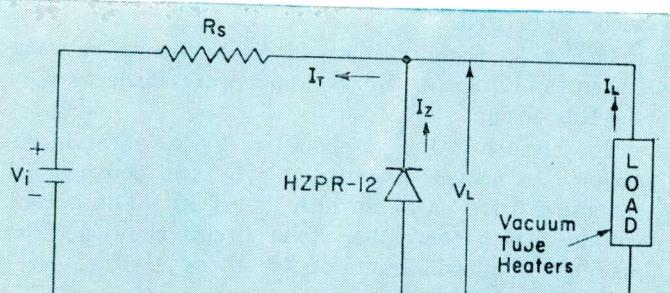
Fig. 1: Typical zener diode regulation of dc heater voltage
