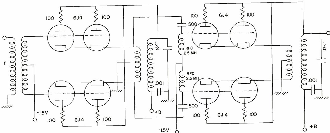
Fig. 2: This model is presently used to divide by four. Note that the output transformer of the first section is input for the second.
