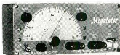
a continuously variable source of modulating frequencies from 15 CPS to 15 KC. It includes an accurate beat-frequency audio oscillator. R-F input voltage is 2.0 v RMS, input impedance is 50 ohms, and insertion loss is approx. 15 db. For the Audio Oscillator: frequency calibration accuracy is  $\pm(1.5\% + 8$  CPS), harmonic distortion is 1.5%, output voltage is 1.0 v RMS at 600 ohms, and output flatness is  $\pm 0.5$  db over its range. Kay Electric Co., 14 Maple Ave., Pine Brook, New Jersey.
