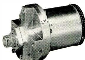
These instruments feed signals from 2-100 watt transmitters into a single missile antenna system and are designed to satisfy military requirements for use in test missiles and supersonic aircraft. Frequency Range: fixed-tuned between 215 to 250 Mc/s; Attenuation: less than 0.3 db; Size: each cavity approx. 3" x 4"; Weight of total system: 3.7 pounds, (2 diplexers + circuitry).
