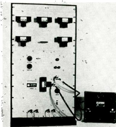
second traced on a Smith chart. The unit consists of an AMCI Hybridge, Polar Display and auxiliary components. It utilizes a standard r-f oscillator, regulating power supply, dc oscilloscope and/or X-Y recorder. Available frequency ranges are 2.5-250 MC, 30-400 MC and 180-1100 MC. Unknown impedance is compared with a 50 ohm Standard Load impedance. Alford Mfg. Co., 299 Atlantic Ave., Boston, Mass.
