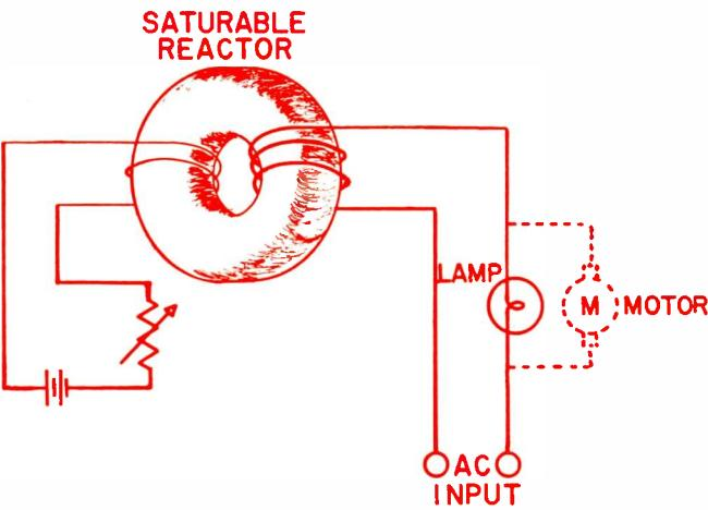
Fig. 2: With little current in control circuit lamp is dim
