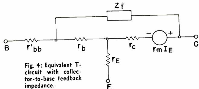
Fig. 4: Equivalent T-circuit with collector-to-base feedback impedance.
