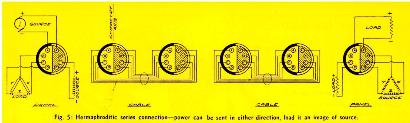
Fig. 5: Hermaphroditic series connection—power can be sent in either direction, load is an image of source.
