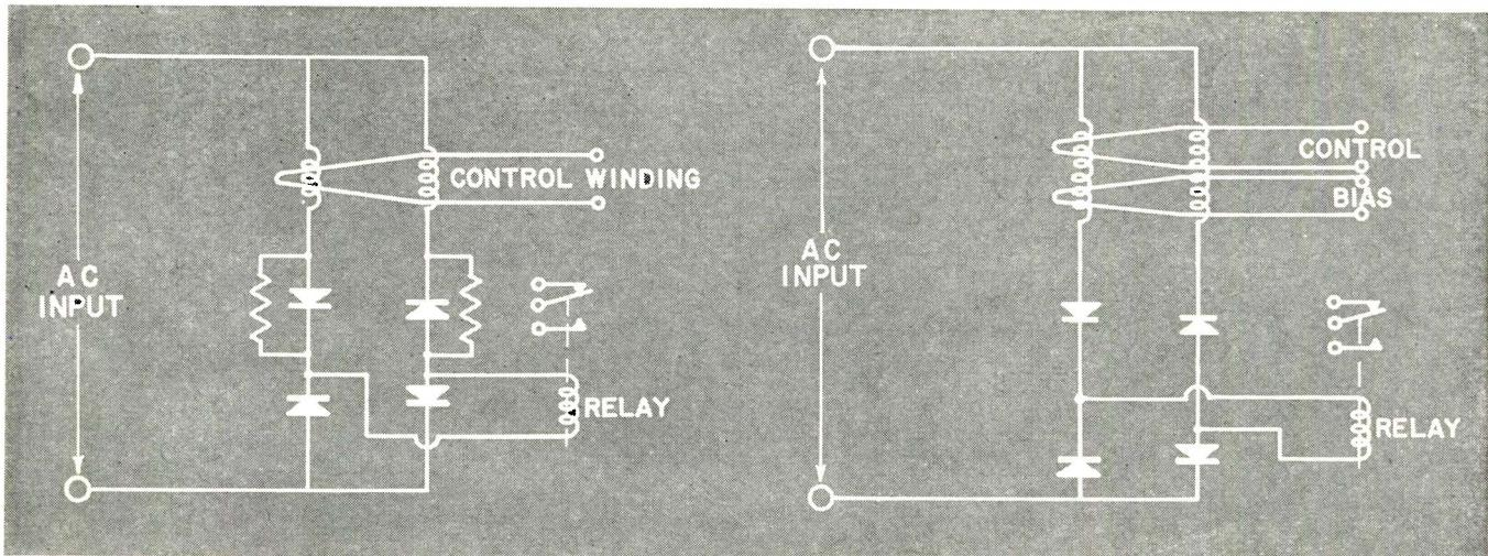
Fig. 5: Resistors keep relay de-energized with no control pwr.
