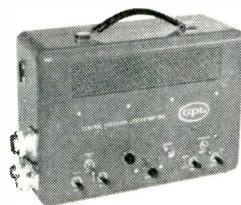
**AUTOMATIC IRIS AND TARGET CONTROL UNIT** automatically adjusts lens aperture and target voltage, compensates for light changes up to 16,000 to 1. Selects smallest possible apertures to give greatest resolution, contrast, and depth of field.
