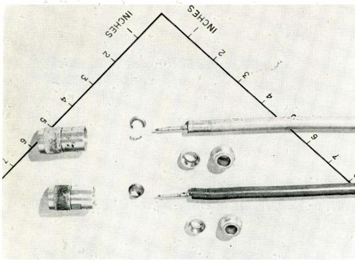
Fig. 7: Sheath fracture of beaded cables caused by subjection to longitudinal vibration while using UG-1149 & UG-1150 connectors.
