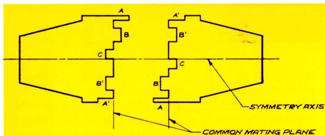
Fig. 3: Portions above mating plane have a counterpart below opposite symmetry axis; portions below mating plane do not.
