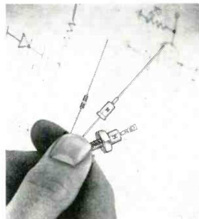
power categories ( $\frac{1}{4}$  w, 1 w, and 10 w). The zener voltage in each power rating ranges from 5.6 v through 200 v in 10% steps. The units are offered in a  $\pm 10\%$  zener voltage tolerance and  $\pm 5\%$ , up to 56 volts. Dynamic impedance ranges from 1400 ohms for 200 v -  $\frac{1}{4}$  watt zener regulator type, down to 1 ohm for the 5.6 v - 10 w unit. Hoffman Electronics Corp., Los Angeles, Calif.
