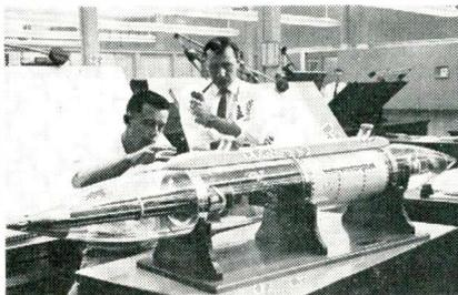
The Air Forces new 7.62 mm. Vulcan is shown in its mockup stage at GE's Missile & Space Vehicle Dept., Burlington, Vt. The new Gatling-type weapon will fire 3,000 rds/min.
