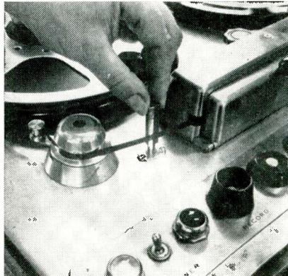
¾ inches by ¼ inch in size with a small energized area. The bar fits over a ¾ inch base plate permanently installed on a tape transport over which passes the moving tape. The package consists of two erasers each with a different power of energized area. Audio Devices, Incorporated, 444 Madison Avenue, New York 22, N. Y.
