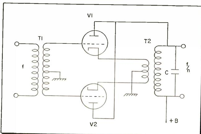
Dividers using regeneration and modulation overcome many of these difficulties but are necessarily complex. They are not always self-starting and may require some auxiliary circuit to insure starting. In addition, they are narrow-band devices.
