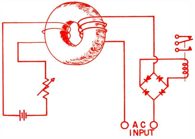
Fig. 3: An elementary magnetic amplifier operated relay
