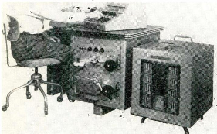
Fig. 2: This tube type computer consumes 18 kw and requires a heat sink. Its transistorized version is shown in
