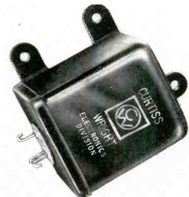
to shock and vibration. Preset time delays between 20 and 180 sec. are available. The relay is voltage compensated from 22 to 32 vdc with a nominal 28 v. rating. Temperature compensation is from  $-65^\circ\text{C}$  to  $+125^\circ\text{C}$ . Operating power is less than 3 w. after the timing interval and 10 w during timing. Various contact arrangements are available. Curtiss-Wright Corp., Wood-Ridge, N.J.
