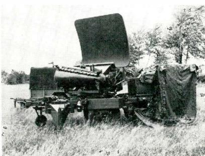
Special design MPQ-4A Mortar Locator Radar developed for the Signal Corps by G.E. detects mortar shell in flight and computes the location of the enemy's mortar installation.
