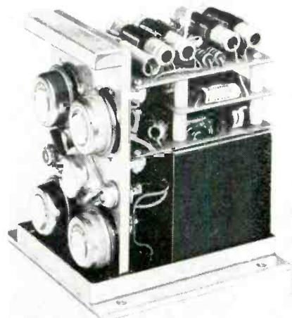
puts of different voltage levels or frequencies. The devices offer up to 5 w per cubic inch output and efficiency is 80% for input voltages greater than 23 volts dc. For the series 760 and 770, output power is up to 1 kw at 0.1% regulation, and for the 780 series, output power is up to 200 w at 0.5% regulation. Spectrol Electronic Corp., San Gabriel, Calif.
